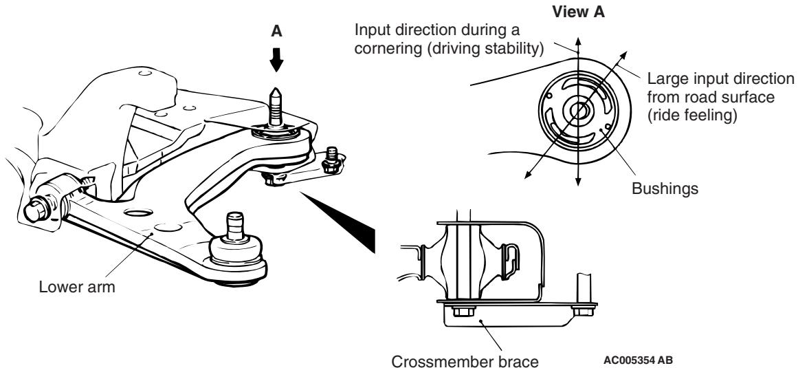
Enlarging the size of mounting bolts at the front and rear sides of crossmember mounting section on lower arm has increased reliability. In addition, bushings with soft spring characteristic at the rear side for the large input direction from road surface and with hard spring characteristics for the input direction dur-
