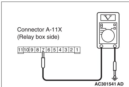
(2) Voltage between A-11X front-ECU connector terminal No.7 and body earth
