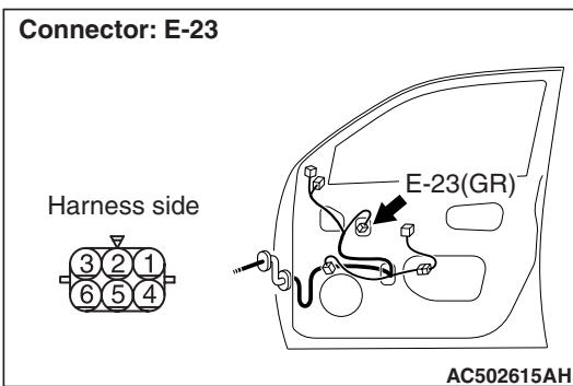
(1) Disconnect the connector, and measure at the wiring harness side.
