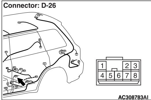
*Prior to the wiring harness inspection, check intermediate connectors E-09 and D-26, and repair if necessary.*
