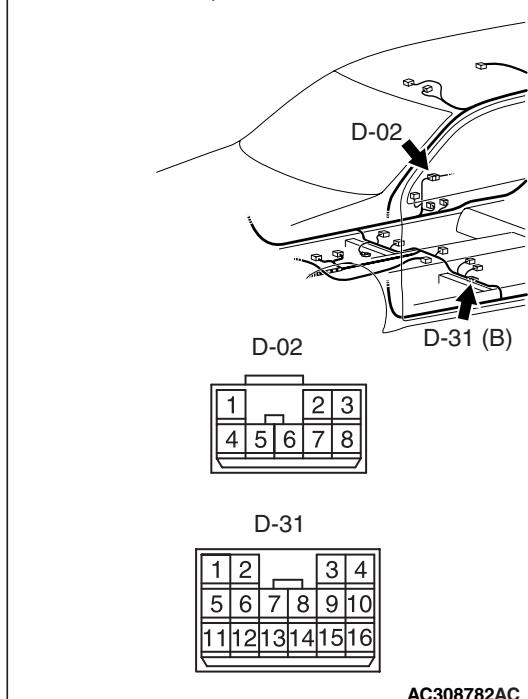
*Prior to the wiring harness inspection, check intermediate connectors D-02, D-31 and junction block connector C-209, and repair if necessary.*
