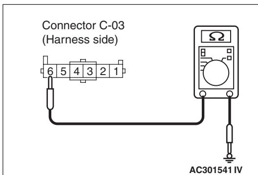
(2) Resistance between C-03 fog lamp switch connector terminal No.6 and body earth
