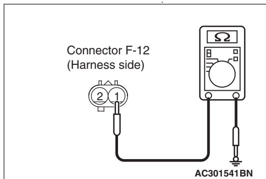
Resistance between F-12 rear fog lamp relay connector terminal No.1 and body earth
