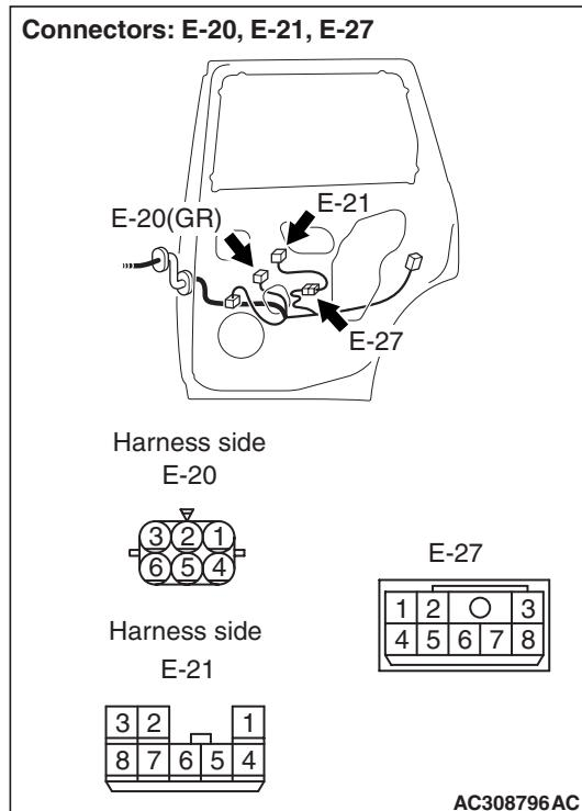
*NOTE: Prior to the wiring harness inspection, check intermediate connector E-27, and repair if necessary.*
