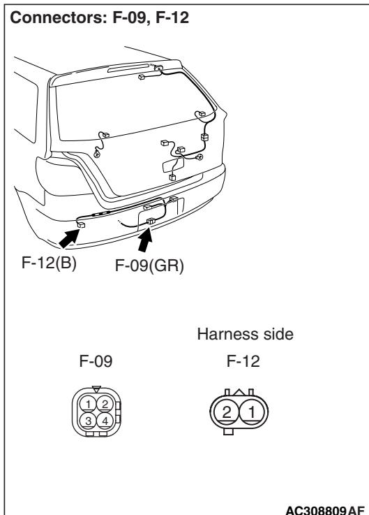
*NOTE: Prior to the wiring harness inspection, check intermediate connector C-117 <rear fog lamp>, F-09 <rear fog lamp> and junction block connector C-201, and repair if necessary.*
