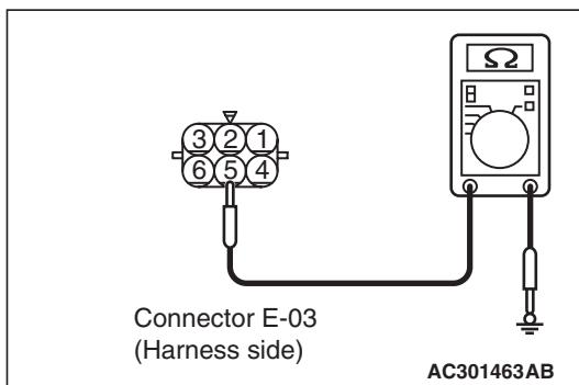
(2) Resistance between E-03 power window motor (rear: LH) connector terminal No.5 and body earth.
