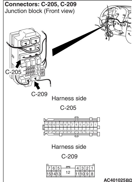
*Prior to the wiring harness inspection, check intermediate connector F-05 <tailgate> or C-13 <RH> and junction block connector C-205 <RH> or C-209 <LH and tailgate>, and repair if necessary.*
