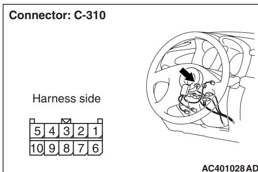
(1) Disconnect the connector, and measure at the column switch side.
