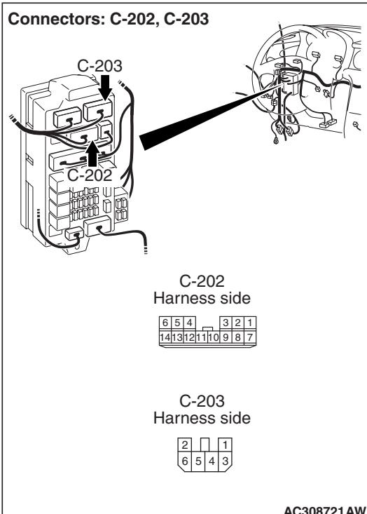
*Prior to the wiring harness inspection, check intermediate connector C-106, junction block connectors C-202 and C-203, and repair if necessary.*
