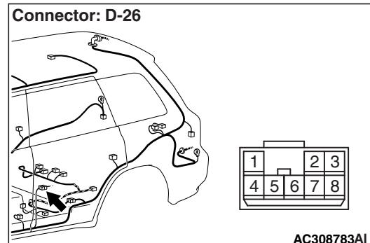
Prior to the wiring harness inspection, check intermediate connectors C-117, D-26, E-09 and junction block connector C-203, and repair if necessary.
