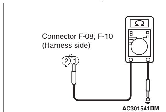
Resistance between F-08 <licence plate lamp, RH> licence plate lamp connector terminal No.1 and body earth
