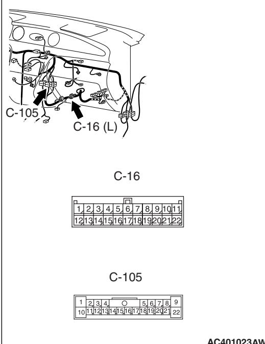
*Prior to the wiring harness inspection, check joint connector C-02, C-16 <2000> and intermediate connector C-105, and repair if necessary.*
