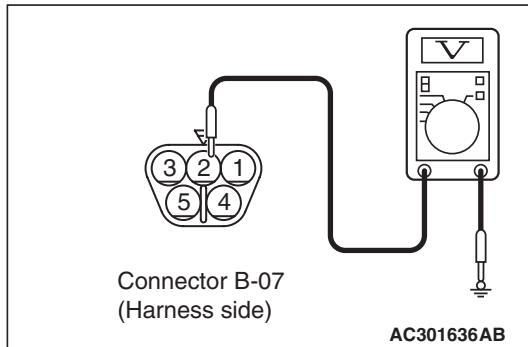
(3) Check the voltage between the B-07 windshield wiper motor connector terminal No.2 and body earth.
