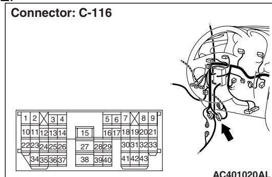
*Prior to the wiring harness inspection, check the intermediate connector C-116 and repair if necessary.*
