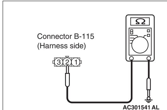
(2) Resistance between B-115 vehicles speed sensor connector terminal No.2 and body earth
