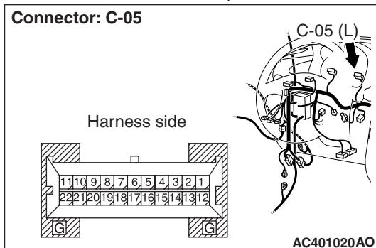
Resistance between C-05 <rear fog lamp indicator lamp> combination meter connector terminal No.12 and body earth
