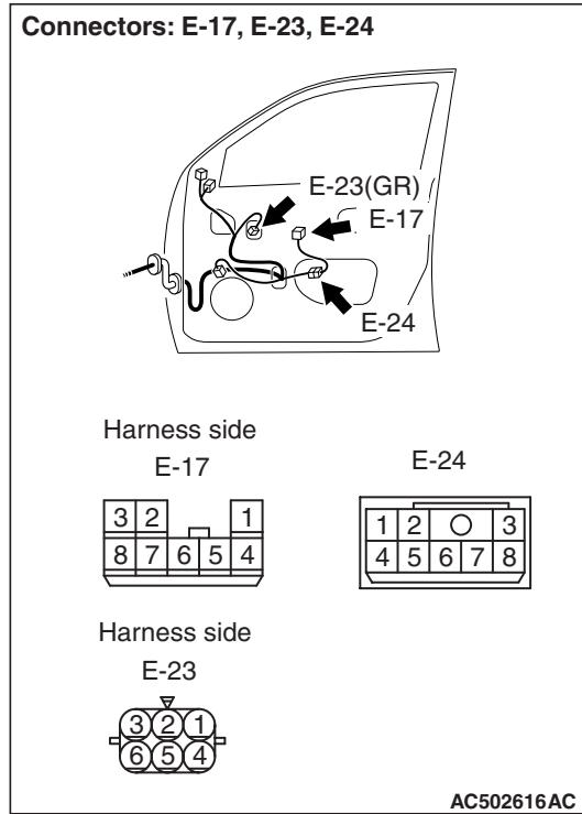
*NOTE: Prior to the wiring harness inspection, check intermediate connector E-24, and repair if necessary.*
