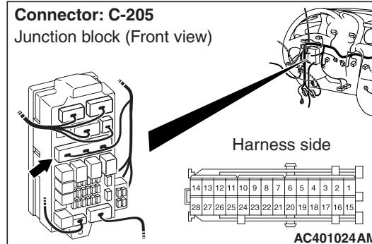
*Prior to the wiring harness inspection, check junction block connector C-205, and repair if necessary.*
