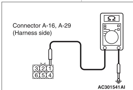
Resistance between A-29 <front turn: RH> headlamp assembly connector terminal No.1 and body earth
