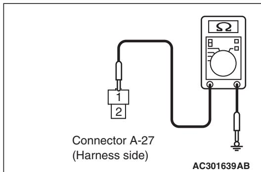
(2) Resistance between A-27 rear washer motor connector terminal No.1 and body earth
