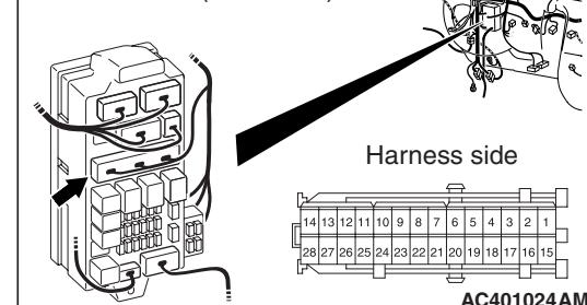
*Prior to the wiring harness inspection, check intermediate connector C-118 and junction block connector C-205, and repair if necessary.*
