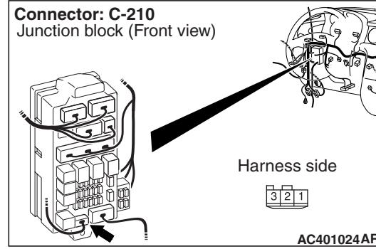
*Prior to the wiring harness inspection, check junction block connector C-210, and repair if necessary.*
