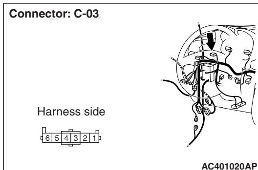
(1) Remove the fog lamp switch, and measure at the wiring harness side.
