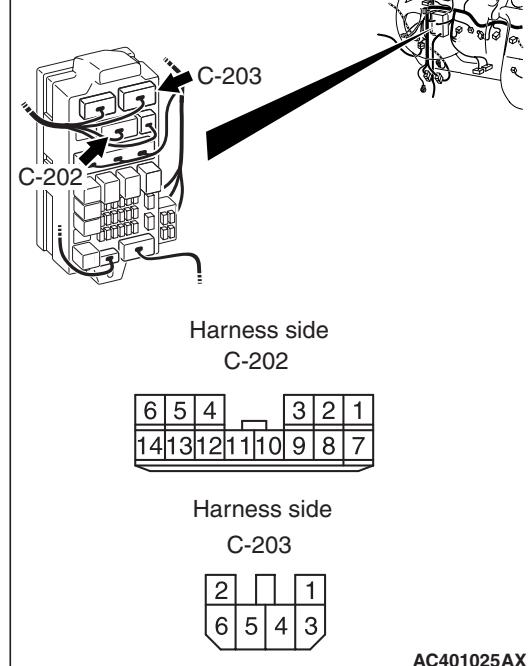
Prior to the wiring harness inspection, check the junction block connectors C-202, C-203 and intermediate connector C-116 and repair if necessary.
