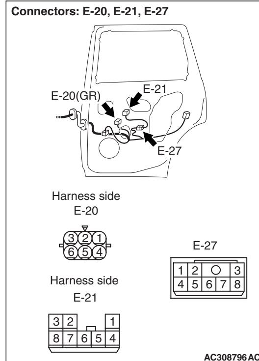
*Prior to the wiring harness inspection, check intermediate connector E-27, and repair if necessary.*
