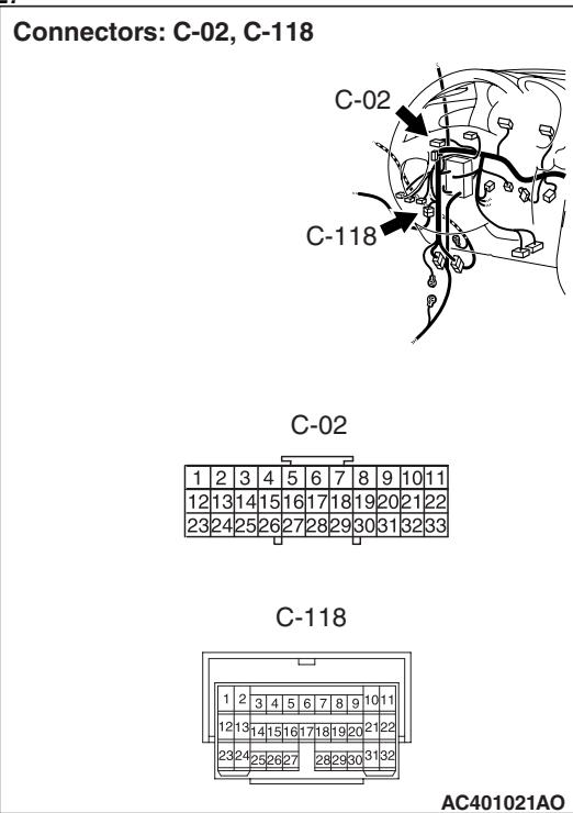
*Prior to the wiring harness inspection, check intermediate connectors, C-118, E-12, and joint connector C-02, and repair if necessary.*
