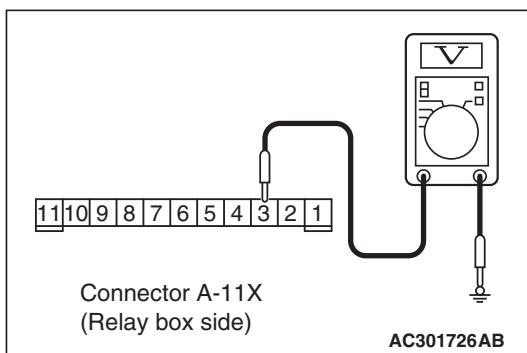
(3) Check the voltage between the A-11X front-ECU connector terminal No.3 and body earth.
