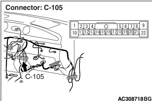
*Prior to the wiring harness inspection, check joint connector C-02 and intermediate connector C-105, and repair if necessary.*
