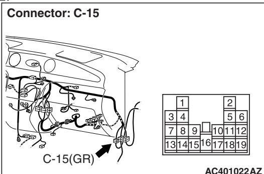
*Prior to the wiring harness inspection, check intermediate connectors C-15 and E-24, and junction block connector C-203, and repair if necessary.*
