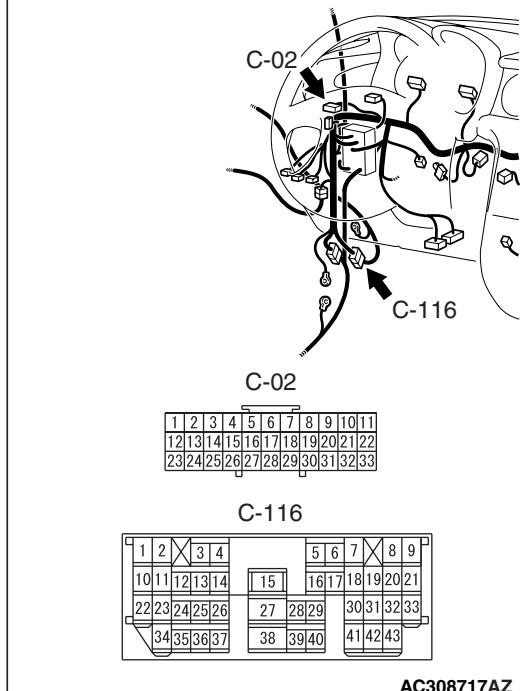
Prior to the wiring harness inspection, check intermediate connector C-116 and joint connector C-02, and repair if necessary.
