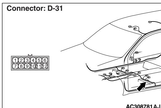
Prior to the wiring harness inspection, check intermediate connector C-14 <side RH>, C-116 <front or side LH> or D-31 <rear turn: RH>, C-209 <rear> or C-205 <turn-signal indicator lamp>, and repair if necessary.
