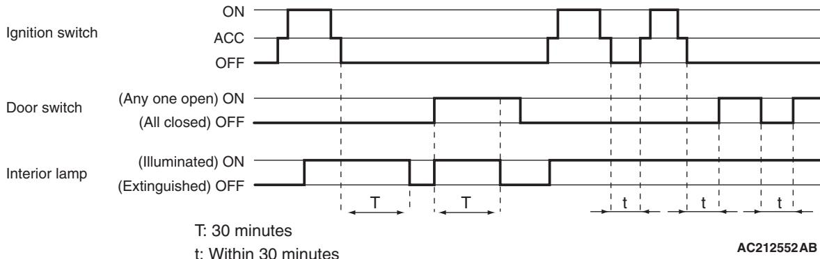
When the interior lamp such as the room lamp [all interior lamps connecting to the room lamp fuse (the front room lamp, the map lamp, the rear room lamp, and the ignition key cylinder illumination lamps)] is lit, but either one of the conditions is met, the interior lamp is turned off automatically for preventing the battery discharge caused by the unattended operation or the door-ajar.
