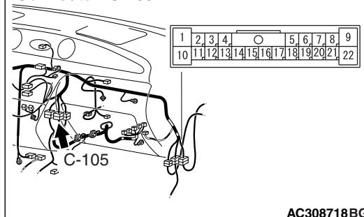
Prior to the wiring harness inspection, check joint connector C-02, and intermediate connector C-105, and repair if necessary.
