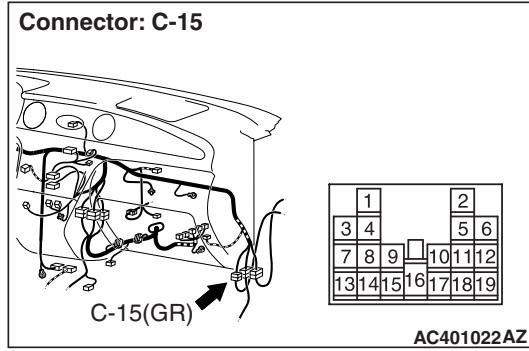
*Prior to the wiring harness inspection, check intermediate connector C-15 and E-24, and repair if necessary.*
