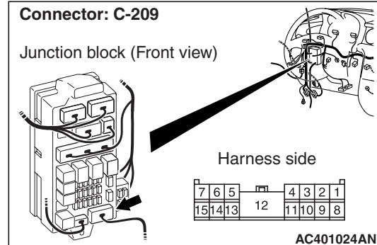
*Prior to the wiring harness inspection, check joint connector C-209, and repair if necessary.*
