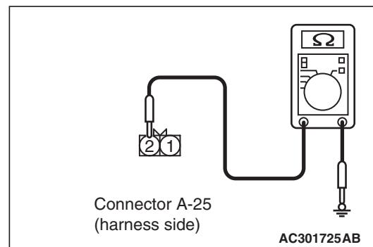
(2) Continuity between A-25 headlamp washer motor connector terminal No.2 and body earth
