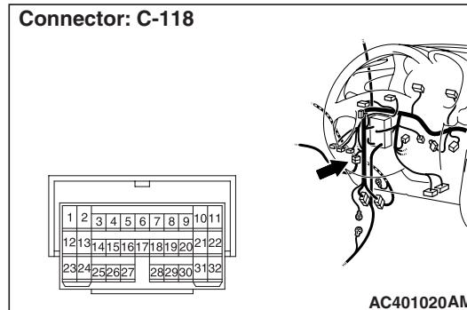
Prior to the wiring harness inspection, check intermediate connectors C-15, C-118, E-12 and E-24, and repair if necessary.
