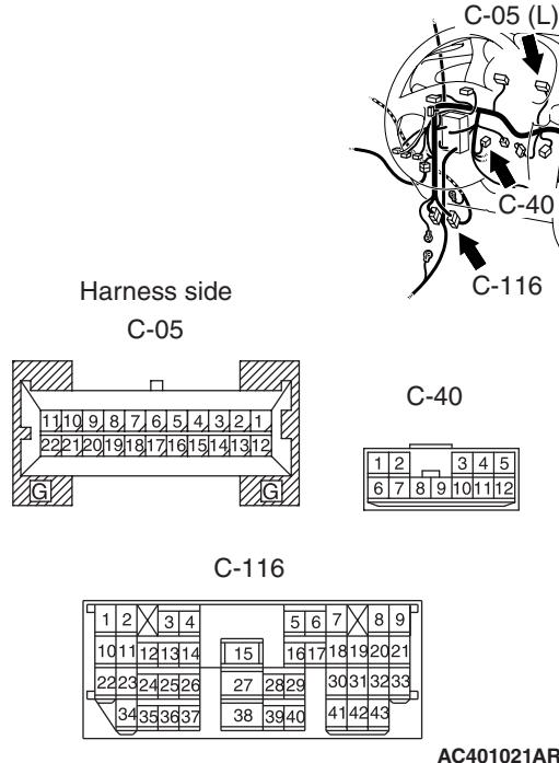
**NOTE: Prior to the wiring harness inspection, check intermediate connector C-116 and joint connector C-40 (high beam indicator lamp), and repair if necessary.**
