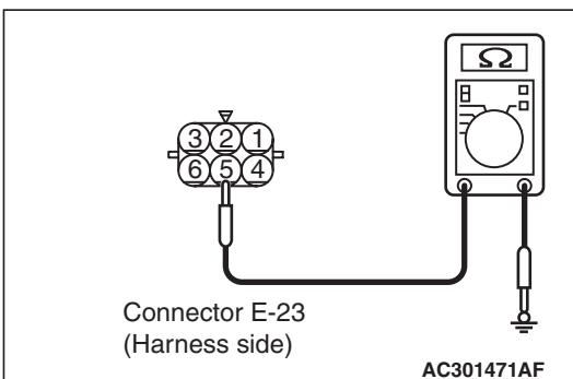
(2) Resistance between E-23 power window motor (front: RH) connector terminal No.5 and body earth.
