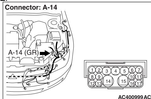
*Prior to the wiring harness inspection, check the intermediate connector A-14, and repair if necessary.*
