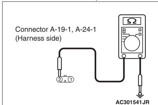
Resistance between A-24-1 <RH> front fog lamp connector terminal No.2 and body earth
