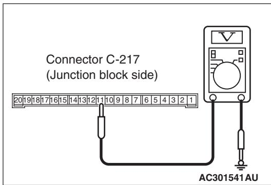
(2) Voltage between C-217 ETACS-ECU connector terminal No.11 and body earth
