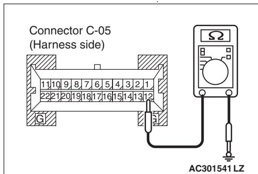
Resistance between C-05 <front fog lamp indicator lamp> combination meter connector terminal No.12 and body earth
