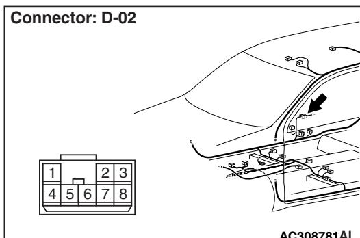
Prior to the wiring harness inspection, check intermediate connectors C-13, C-118, D-02, E-12 and E-27, and repair if necessary.
