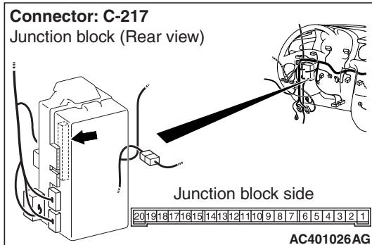
**Step 7. Check the wiring harness from C-217 ETACS-ECU connector terminal Nos. 5 and 6 to D-11 rear room lamp connector terminal Nos. 2 and 1.**
