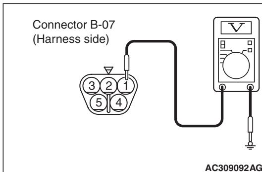
(4) Check the voltage between the B-07 windshield wiper motor connector terminal No.1 and body earth.
