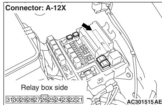
When A-12X front-ECU connector is disconnected, check that diagnosis code No.21 is not reset. However, diagnosis code No.13 will be set at this time.
