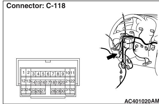
*Prior to the wiring harness inspection, check intermediate connector C-118, and repair if necessary.*
