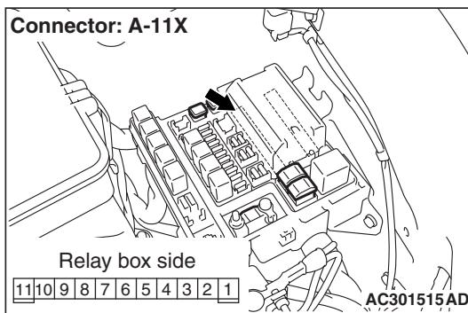
(1) Remove the front-ECU, and measure at the junction block side.
