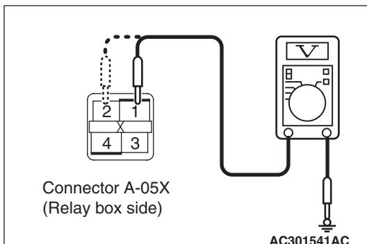
(2) Check the voltage between the front fog lamp relay connector and body earth.
