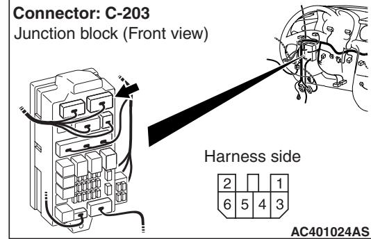
*Prior to the wiring harness inspection, check junction block connector C-203, and repair if necessary.*
