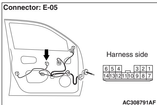
When E-05 power window main switch connector is disconnected, check that diagnosis code No.21 is not reset.
