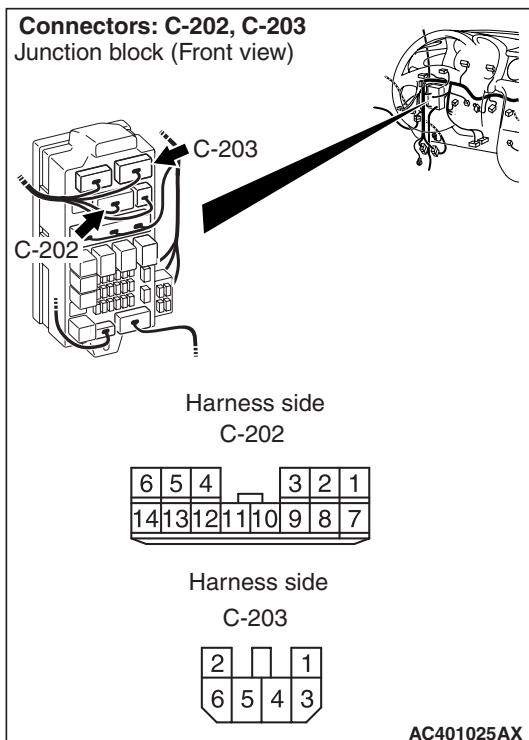
Prior to the wiring harness inspection, check A/T control relay connector B-16X, joint connector C-16, intermediate connector C-106 and junction block connectors C-202 and C-203, and repair if necessary.
