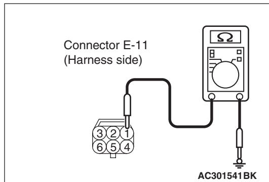
(2) Resistance between E-11 door lock actuator (front: LH) connector terminal No.1 and body earth
