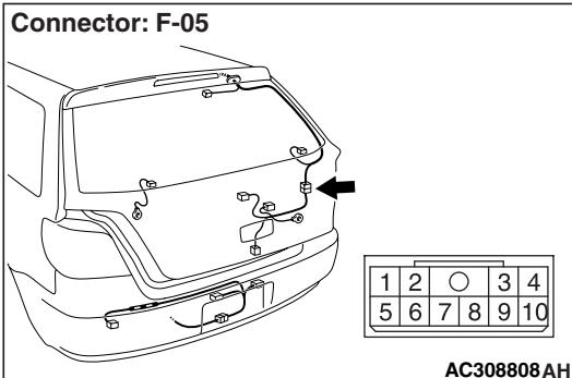
*Prior to the wiring harness inspection, check intermediate connector F-05 and junction block connectors C-209, and repair if necessary.*
