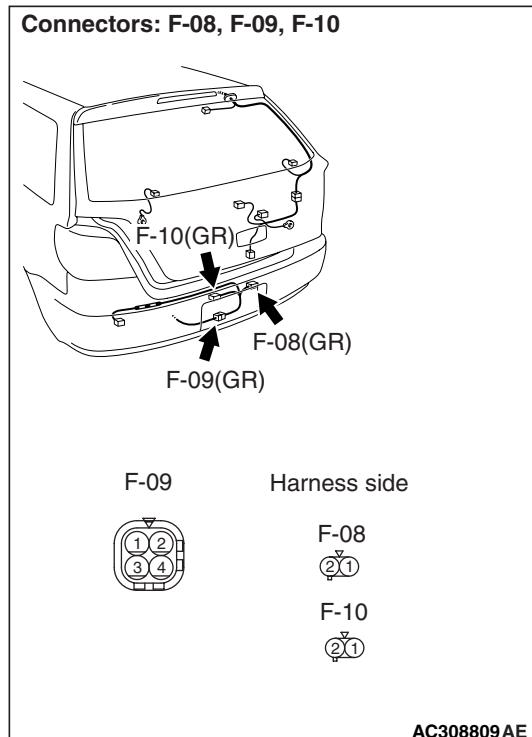
**NOTE: Prior to the wiring harness inspection, check intermediate connector F-09 <licence plate lamp>, and repair if necessary.**
