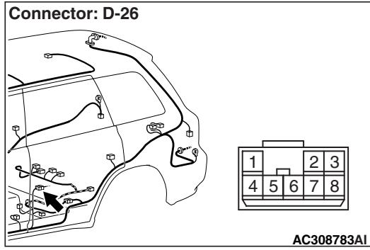
Prior to the wiring harness inspection, check intermediate connector D-26, and repair if necessary.
