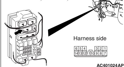
*Prior to the wiring harness inspection, check junction block connector C-202 and intermediate connector C-116, and repair if necessary.*
