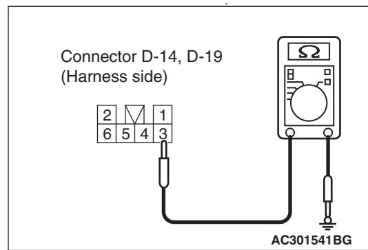
Resistance between D-14 <right tail lamp> rear combination lamp connector terminal No.3 and body earth
