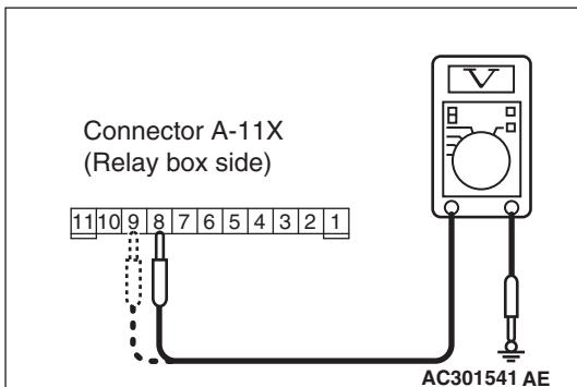
(2) Voltage between A-11X front-ECU connector terminal Nos. 8, 9 and body earth
