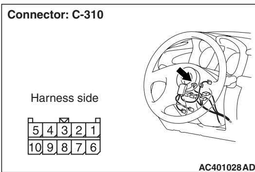
(1) Remove the column switch, and measure at the wiring harness side.
