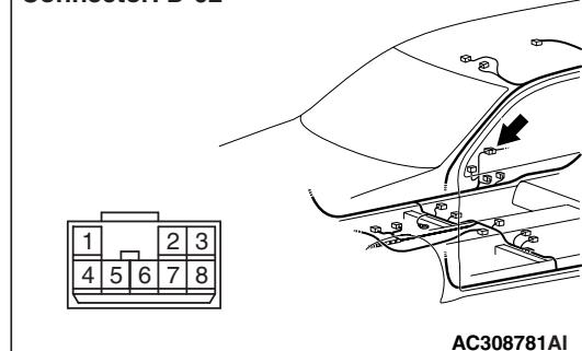
*Prior to the wiring harness inspection, check intermediate connectors C-13, D-02, E-27 and junction block connector C-203, and repair if necessary.*
