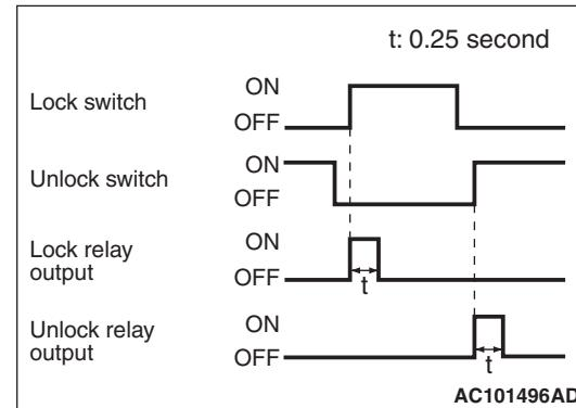
When the front doors are locked (when the lock switch turns ON after turning OFF the unlock switch in the driver's door lock actuator), ETACS-ECU turns ON the lock relay output for 0.25 second, and locks all doors (including the tailgate). When the front doors are unlocked (when the unlock switch turns ON after turning OFF the lock switch on the driver's door lock actuator), ETACS-ECU turns ON the unlock relay output for 0.25 second, and unlocks all doors (including the tailgate).
