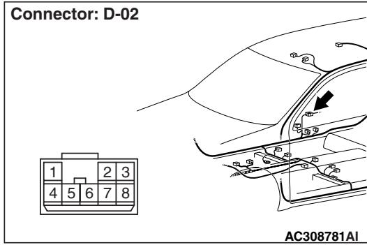
*Prior to the wiring harness inspection, check intermediate connector D-02, and repair if necessary.*
