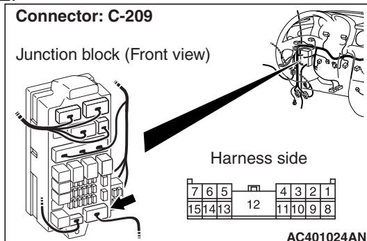
*Prior to the wiring harness inspection, check intermediate connector F-05 and junction block connector C-209, and repair if necessary.*
