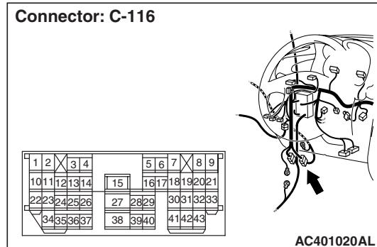
*Prior to the wiring harness inspection, check intermediate connector C-116 and repair if necessary.*
