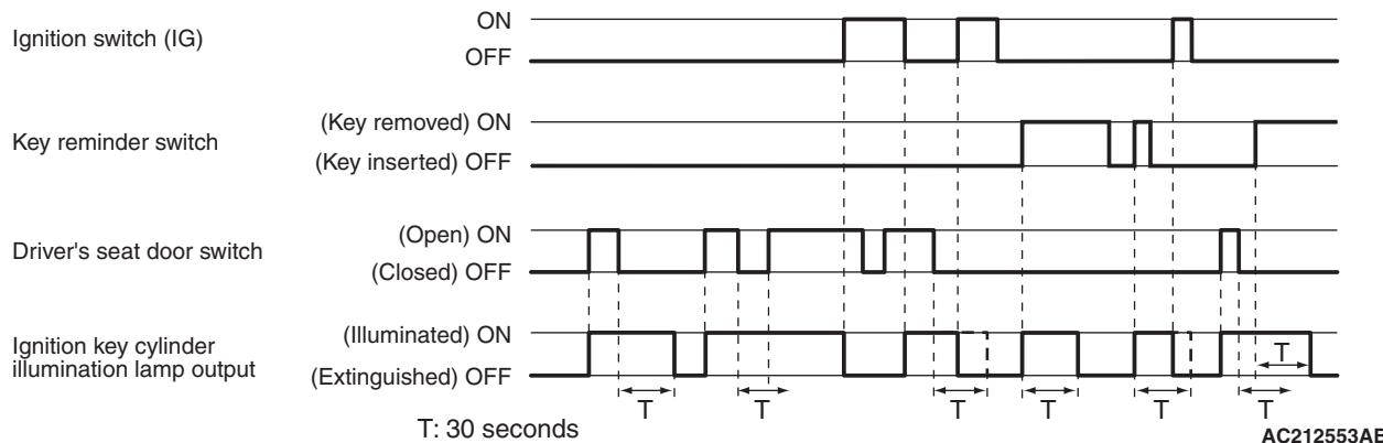
The ignition key cylinder illumination lamp turns on for 30 seconds when the driver's door is opened/closed with the ignition switch OFF. Also when the ignition key is removed from the ignition key cylinder, the lamp turns on for 30 seconds. In any cases, the ignition key cylinder illumination lamp turns ON when the ignition switch is turned to ON.
