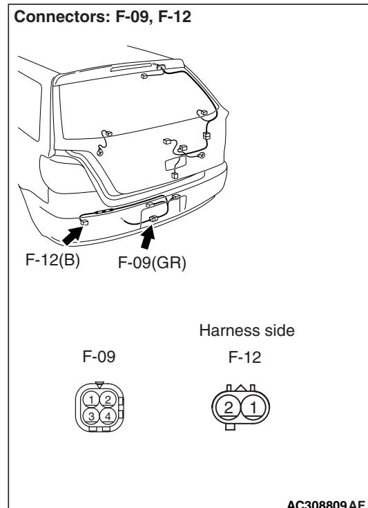
*NOTE: Prior to the wiring harness inspection, check intermediate connector F-09 <rear fog lamp>, and repair if necessary.*
