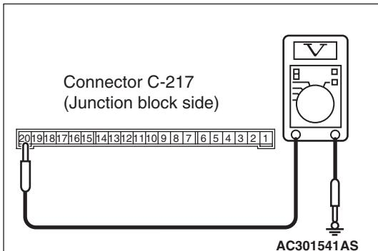
(2) Voltage between C-217 ETACS-ECU connector terminal No.20 and body earth.
