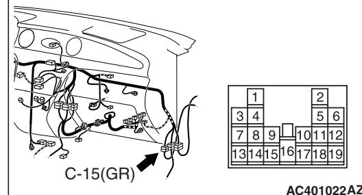
*Prior to the wiring harness inspection, check intermediate connector C-15, and repair if necessary.*
