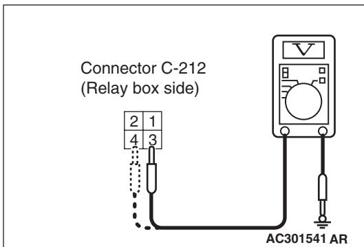
(2) Check the voltage between the rear fog lamp relay connector and body earth.
