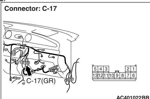
*Prior to the wiring harness inspection, check joint connector C-17, and repair if necessary.*
