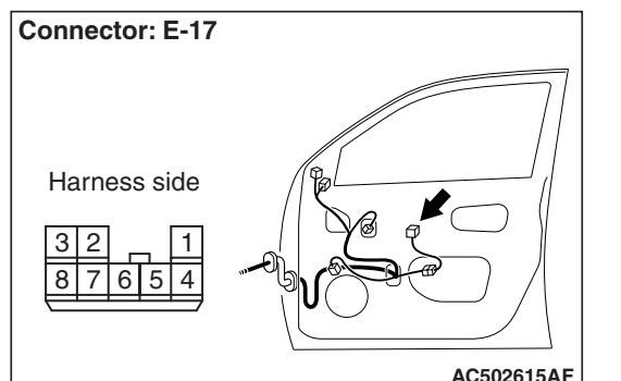
(1) Disconnect the connector, and measure at the wiring harness side.
