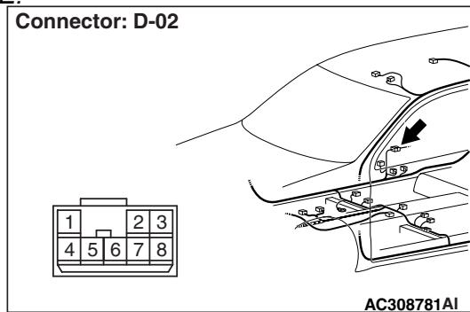
*Prior to the wiring harness inspection, check intermediate connectors E-27 and D-02, and repair if necessary.*
