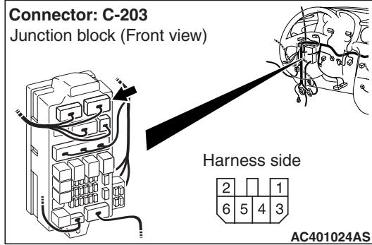
*Prior to the wiring harness inspection, check junction block connector C-203, and repair if necessary.*
