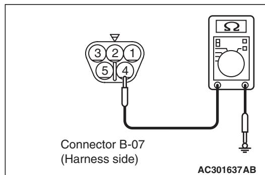
(4) Check the voltage between the B-07 windshield wiper motor connector terminal No.4 and body earth.
