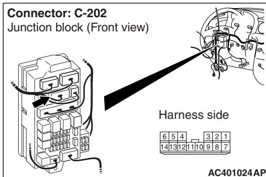
*Prior to the wiring harness inspection, check intermediate connector C-116 and junction block connector C-202, and repair if necessary.*
