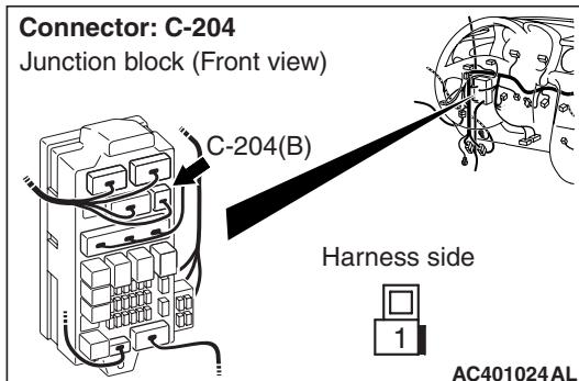
*Prior to the wiring harness inspection, check intermediate connector C-116 and junction block connector C-204, and repair if necessary.*
