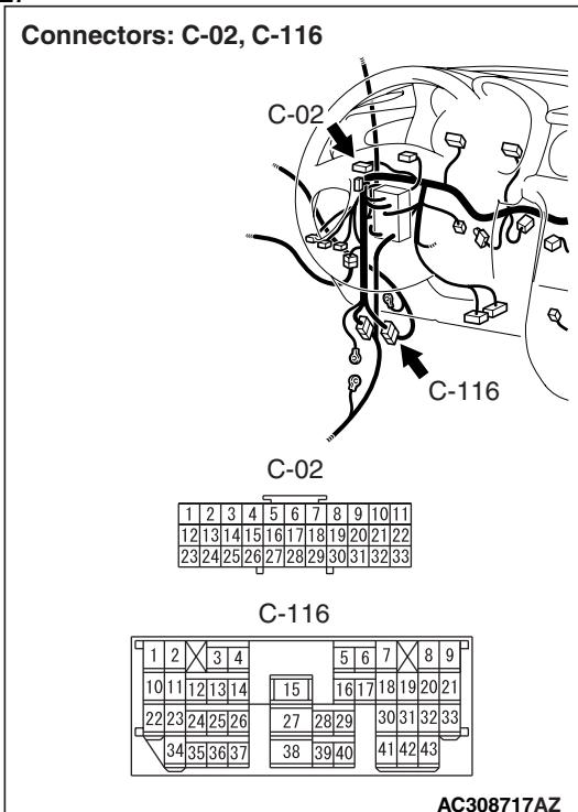
*Prior to the wiring harness inspection, check joint connector C-02 and intermediate connector C-116, and repair if necessary.*
