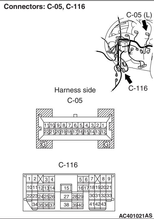
*NOTE: Prior to the wiring harness inspection, check intermediate connectors A-19, A-24 and C-116 <front fog lamp indicator lamp>, and repair if necessary.*
