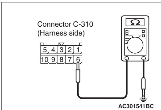
(2) Resistance between C-310 column switch connector terminal No.6 and body earth
