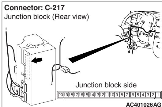
(1) Remove the ETACS-ECU, and measure at the junction block side.
