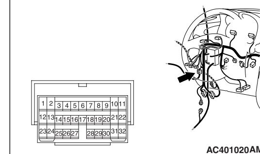
*Prior to the wiring harness inspection, check intermediate connectors C-118, E-12, and junction block connector C-203, and repair if necessary.*
