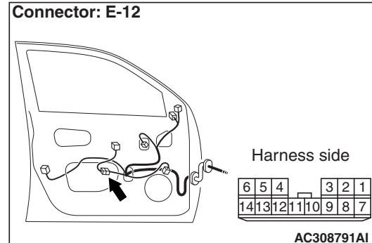
*Prior to the wiring harness inspection, check intermediate connectors C-118, E-12, and junction block connector C-203, and repair if necessary.*
