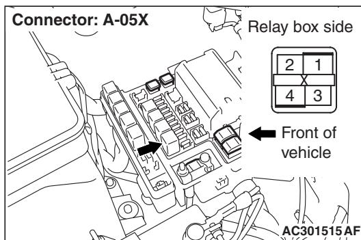
(1) Remove the front fog lamp relay, and measure at the relay box side.
