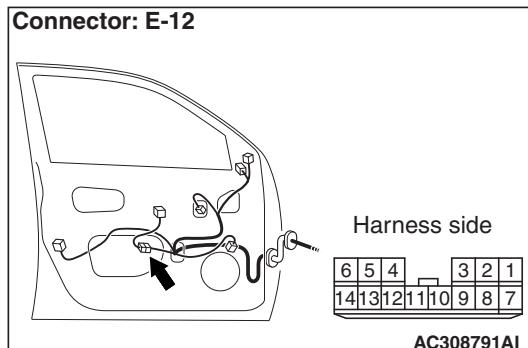
Prior to the wiring harness inspection, check intermediate connectors C-118, E-12 and joint connector C-02, and repair if necessary.
