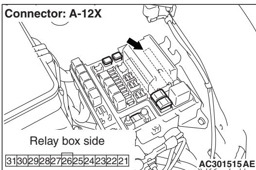
(1) Remove the front-ECU, and measure at the relay box side.
