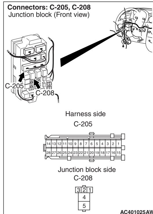
*NOTE: Prior to the wiring harness inspection, check junction block connector C-205, and repair if necessary.*
