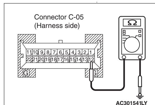
Resistance between C-05 <turn-signal indicator lamp (RH)> combination meter terminal No.12 and body earth
