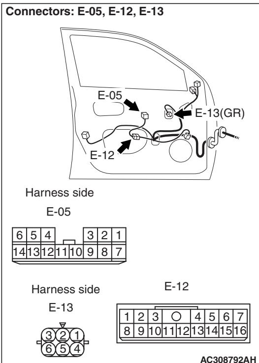
*NOTE: Prior to the wiring harness inspection, check intermediate connector E-12, and repair if necessary.*
