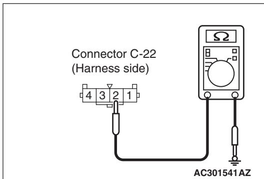
(2) Resistance between C-22 hazard warning lamp switch connector terminal No.2 and body earth
