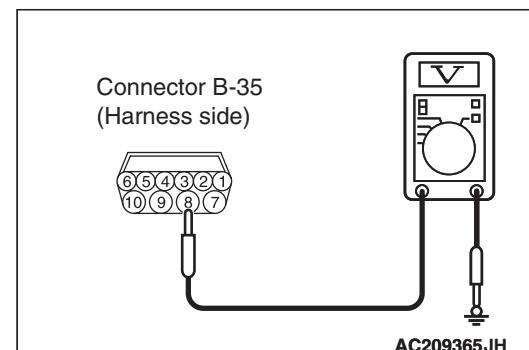
(3) Voltage between B-35 inhibitor switch connector terminal No.8 and body earth
