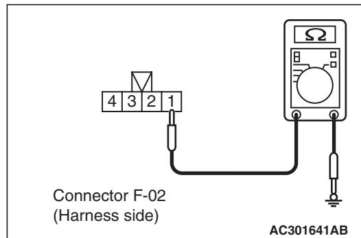
(2) Resistance between F-02 rear wiper motor connector terminal No.1 and body earth
