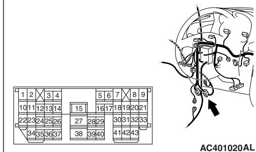
*Prior to the wiring harness inspection, check intermediate connectors C-116, and junction block connector C-203, and repair if necessary.*
