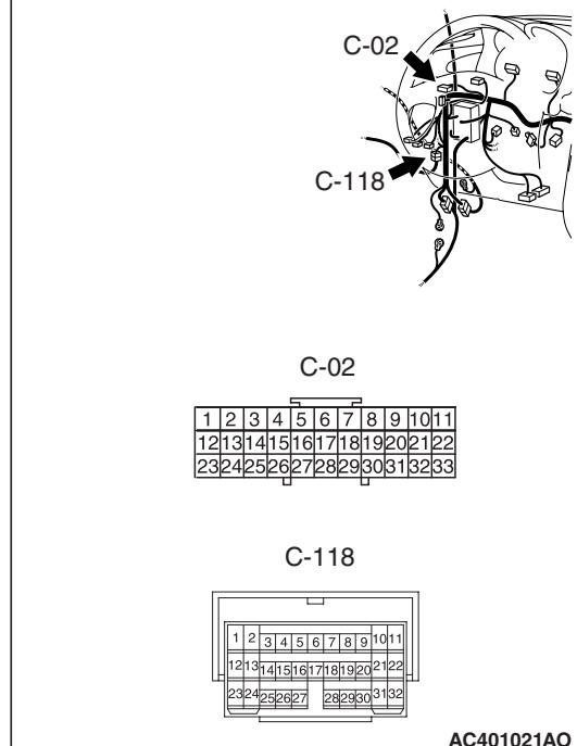
Prior to the wiring harness inspection, check intermediate connector C-116 and joint connector C-02, and repair if necessary.
