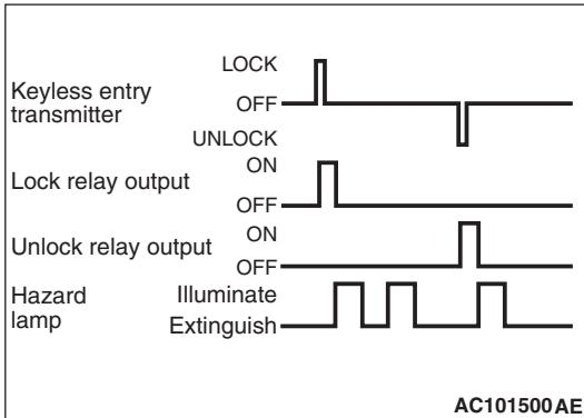
The hazard lamp answerback function that allows checking the lock/unlock state of the door easily even in the daytime is installed. When the lock signal from the keyless entry transmitter is received into ETACS-ECU, all doors (including the tailgate) are locked, and the hazard warning lamp blinks twice. When the unlock signal is received, all doors (including the tailgate) are unlocked, and the hazard warning lamp blinks once.
