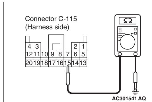
(2) Resistance between C-115 SRS-ECU connector terminal No.15 and body earth
