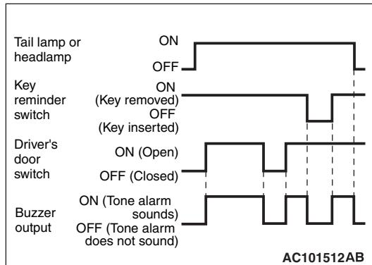
When the ignition key is removed and then the driver's door is opened with turning ON the tail lamp or the head lamp, the buzzer sounds continuously to alert the driver that the lamp is still ON. However, if the tail lamp or the head lamp is turned off by the headlamp automatic-shutdown function, the buzzer does not sound.
