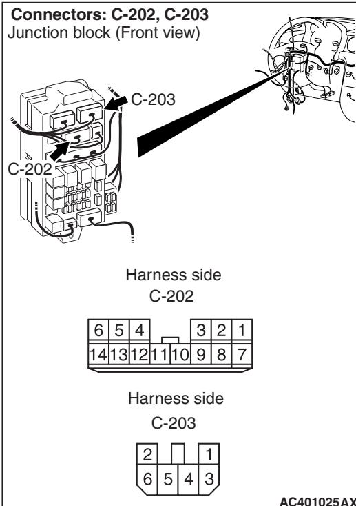
*Prior to the wiring harness inspection, check the junction connectors C-202, C-203, the intermediate connectors C-104, and repair if necessary.*
