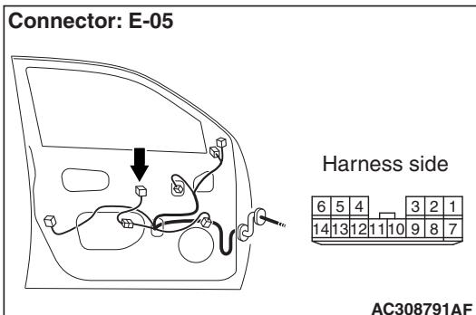
**Step 2. Check the wiring harness from each of A-12X front-ECU connector terminal No.30, C-310 column switch connector terminal No.3 and E-05 power window main switch connector terminal No.4 to C-219 ETACS-ECU connector terminal No.59.**
