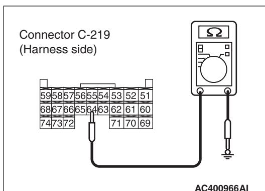
(2) Check the resistance between the ETACS-ECU connector and body earth.
