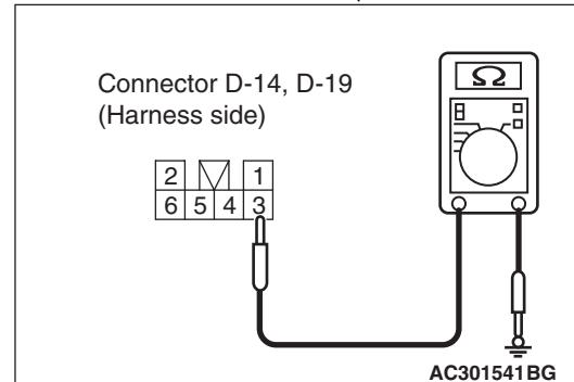
Resistance between D-14 <rear turn: RH> rear combination lamp connector terminal No.3 and body earth
