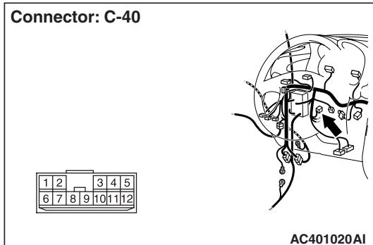
*Prior to the wiring harness inspection, check joint connector C-40, and repair if necessary.*
