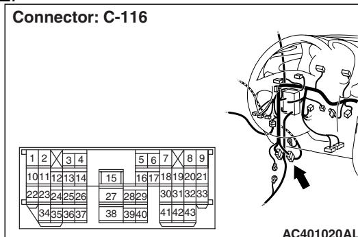
*Prior to the wiring harness inspection, check intermediate connectors C-116, junction block connectors C-204 and C-205, and repair if necessary.*
