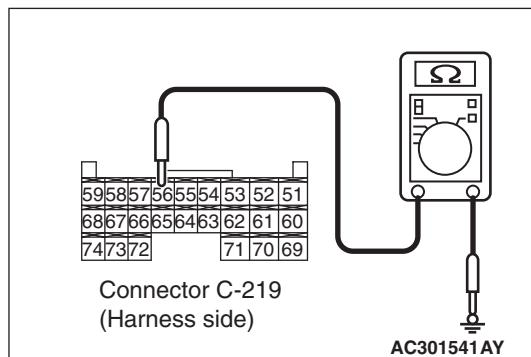
**Step 3. Connector check: C-219 ETACS-ECU connector**
