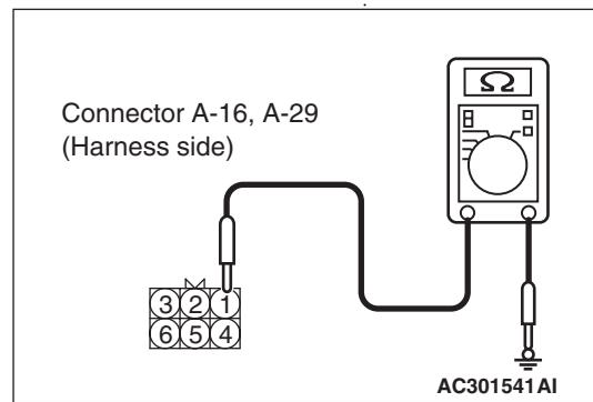
Resistance between A-16 <position LH> headlamp assembly connector terminal No.1 and body earth
