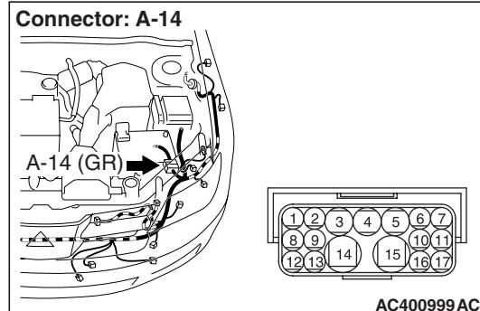
*Prior to the wiring harness inspection, check the intermediate connector A-14, and repair if necessary.*
