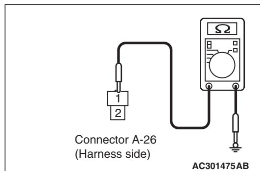
**(2) Continuity between A-26 windshield washer motor connector terminal No.1 and body earth**
