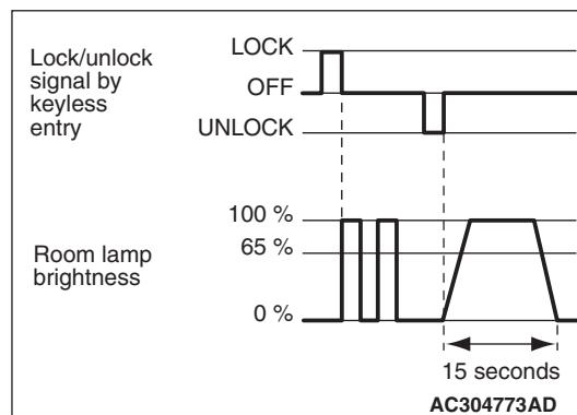
The room lamp blinks two times while locking the door for easy checking the keyless entry function. When the door is unlocked, the lamp lamps on for 15 seconds (100%), and turns off.
