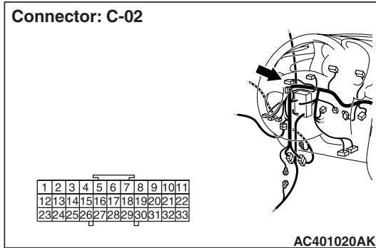
*Prior to the wiring harness inspection, check joint connector C-02, and repair if necessary.*
