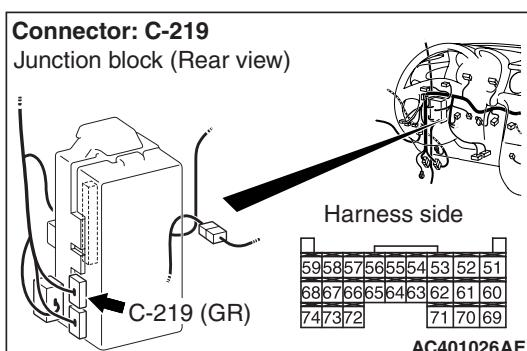
**(1) Disconnect the connector, and measure at the junction block side.**
