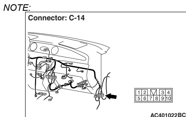
*Prior to the wiring harness inspection, check intermediate connector C-14 <side: RH>, and repair if necessary.*
