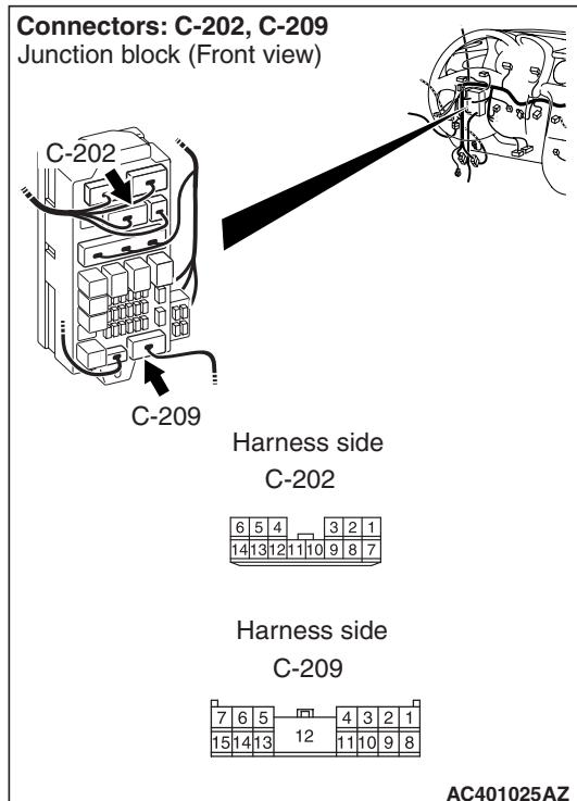
Prior to the wiring harness inspection, check joint connector C-01 <right tail lamp>, intermediate connector C-116 <tail lamp and licence plate lamp>, C-117 <left tail lamp and licence plate lamp>, D-31 <right tail lamp>, F-09 <licence plate lamp>, junction block connector C-202 <right tail lamp> and C-209 <right tail lamp>, and repair if necessary.
