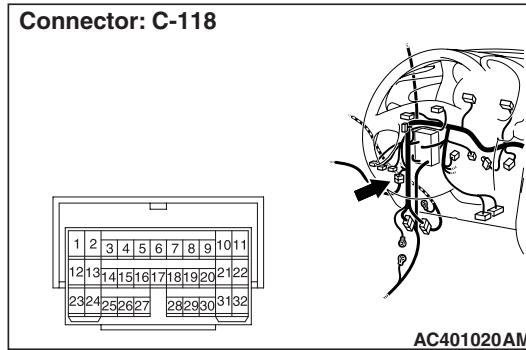
*Prior to the wiring harness inspection, check intermediate connectors C-118 and E-12, and repair if necessary.*
