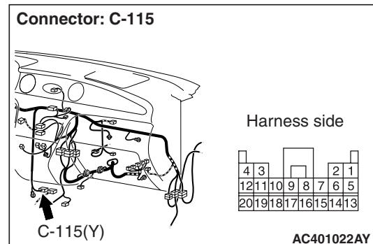
(1) Disconnect the connector, and measure at the wiring harness side.
