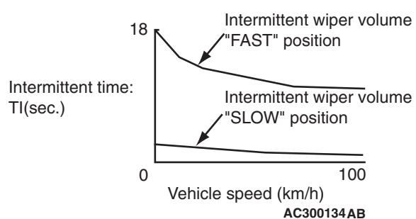
ETACS-ECU calculates the intermittent time TI from the vehicle speed calculated from the windshield intermittent wiper volume of the column switch and the vehicle speed signals (engine-ECU), and sends it to the front ECU as SWS data.
