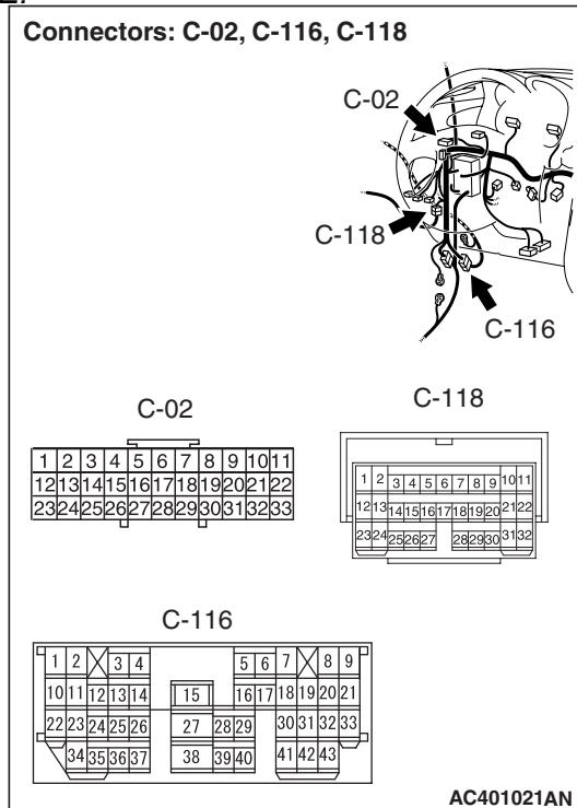
Prior to the wiring harness inspection, check joint connector C-02, intermediate connectors C-116, C-118 and E-12, and repair if necessary.
