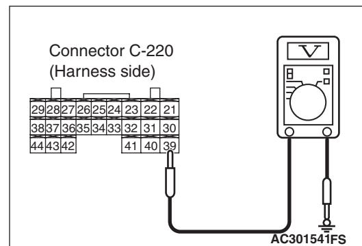
(4) Voltage between C-220 ETACS-ECU connector terminal No.39 and body earth
