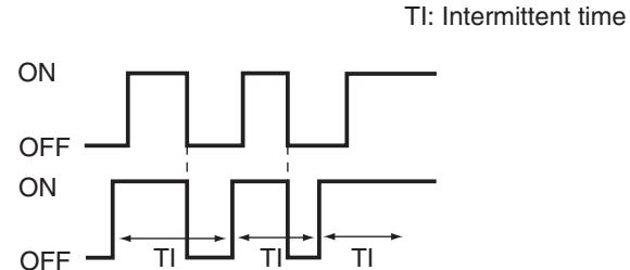
The front ECU determines the intermittent time TI from the input SWS data, and turns ON the windshield wiper drive signal. When the wiper comes to the stop position, the windshield wiper auto-stop signal is turned OFF, and the windshield wiper drive signal turns OFF.
