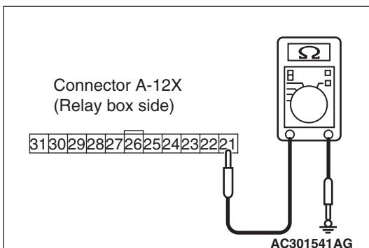
(2) Resistance between A-12X front-ECU connector terminal No.21 and body earth
