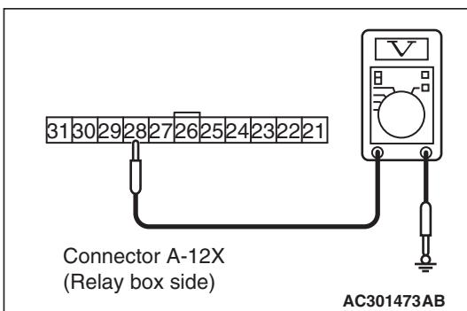
(3) Check the voltage between the A-12X front-ECU connector terminal No.28 and body earth.
