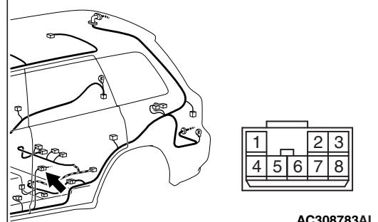
*Prior to the wiring harness inspection, check intermediate connector D-26 and junction block connector C-209, and repair if necessary.*
