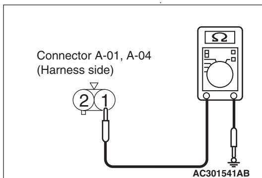
Resistance between A-01 <side: RH> side turn-signal lamp connector terminal No.1 and body earth
