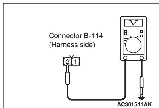
(3) Voltage between B-114 back-up lamp switch connector terminal No.2 and body earth
