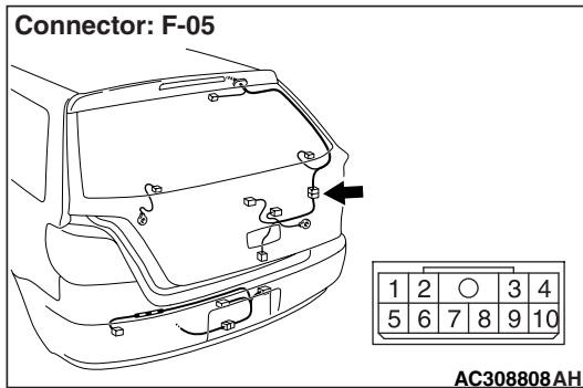
*Prior to the wiring harness inspection, check intermediate connector F-05 and junction block connectors C-203 and C-209, and repair if necessary.*
