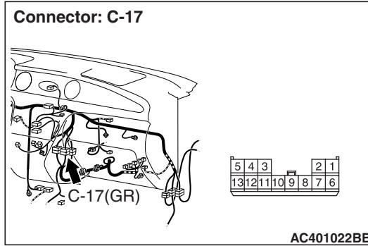
*Prior to the wiring harness inspection, check the joint connector C-17, and repair if necessary.*
