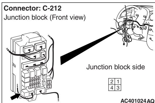
(1) Remove the rear fog lamp relay, and measure at the relay box side.
