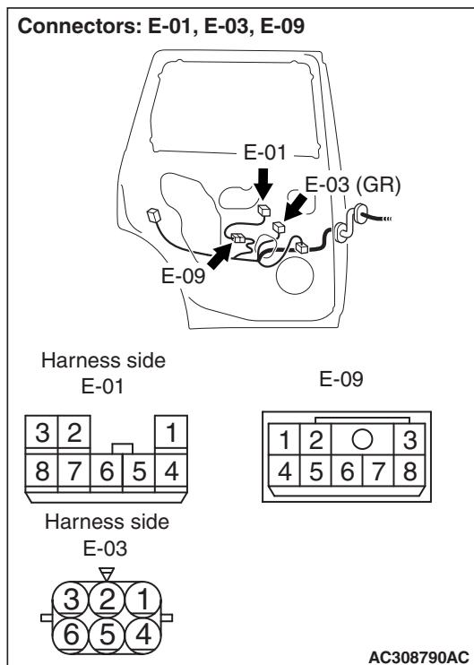
*NOTE: Prior to the wiring harness inspection, check intermediate connector E-09, and repair if necessary.*
