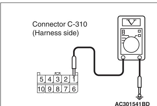
(2) Voltage between C-310 column switch connector terminal No.1 and body earth
