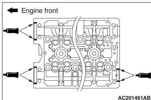
3. Apply sealant to the positions (6 areas) of the upper side of the cylinder head as shown in the illustration.
