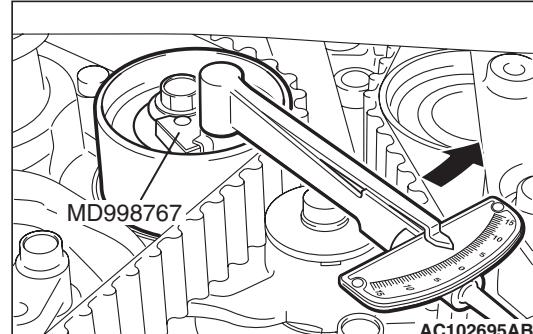
6. With special tool tensioner wrench (MD998767) and torque wrench, apply tension torque 3.5 N·m, and tighten the timing belt tensioner pulley mounting bolt to the specified torque.
