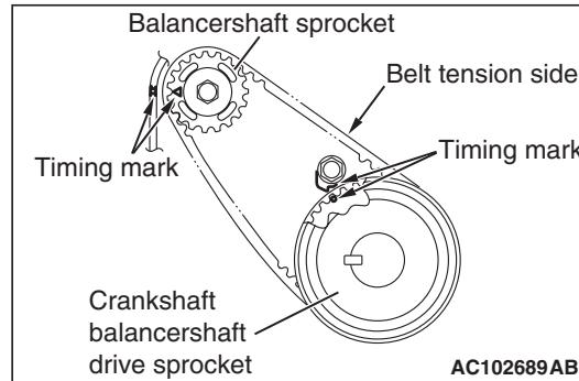
1. Ensure that the crankshaft balancershaft drive sprocket timing marks and balancershaft sprocket timing marks are aligned.
