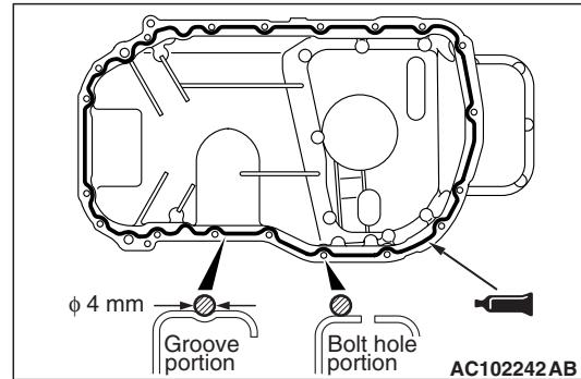
2. Apply a bead of the sealant to the mating surface of the engine upper oil pan as shown.
