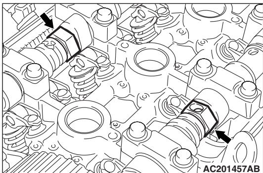
1. Hold the hexagon part of the camshaft with a wrench in the same manner as removal.
