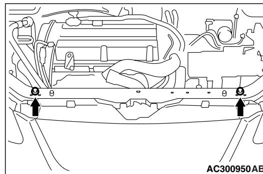
1. Pre-tighten the 2 bolts on the car to assemble the radiator support upper insulator to set the special tools engine hanger MB991895 or engine hanger MB991928.
