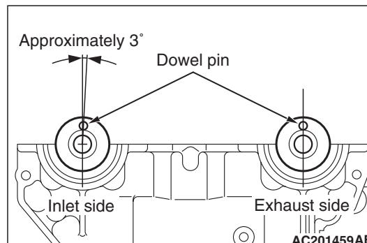
1. Set the dowel pin of the camshaft to the position as shown in the illustration.
