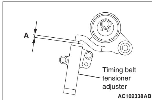
If the projection of timing belt tensioner adjuster rod is within the standard value, appropriate tension is applied.
