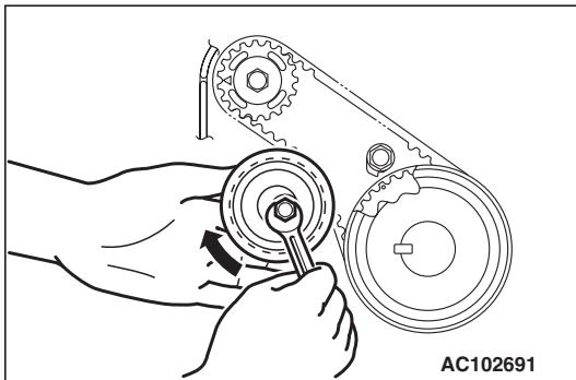
1. With your fingers, lift the balancer timing belt tensioner in the direction of the arrow. Apply pressure of  $3.0 \pm 0.4 \text{ N}\cdot\text{m}$  to the balancer timing belt. Tighten the assembling bolt to the specified torque. Then, fix the balancer timing belt tensioner.
