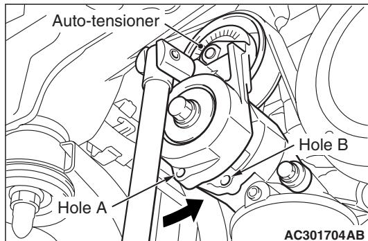
1. Securely insert the spindle handle or ratchet handle with a 12.7 mm insertion angle into the jig hole of the auto-tensioner.
