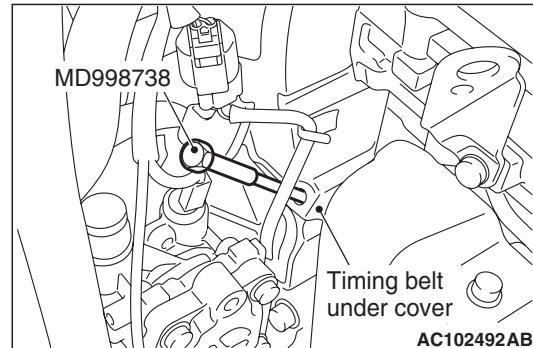
1. Set special tool adjusting bolt (MD998738) when removing the valve timing belt.
