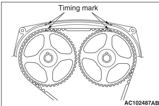
1. Turn the crankshaft clockwise, align each timing mark to set No.1 cylinder to TDC of its compression stroke.
