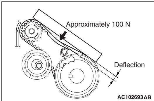
3. Apply a pressure of approximately 100N at the centre (arrow area) between the sprocket as shown, then inspect whether the belt deflection is within the standard value.
