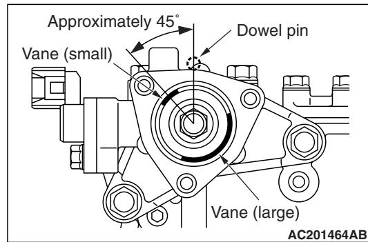
1. Set the dowel pin of the exhaust camshaft to the position (No.1 cylinder at compression TDC) as shown in the illustration.
