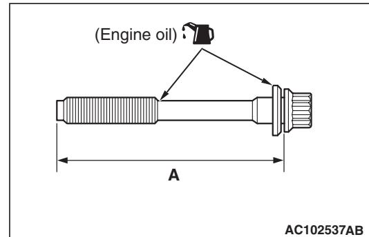
1. Check that the nominal length of each cylinder head bolt meets the limit. If it exceeds the limit, replace the bolt with a new one.
