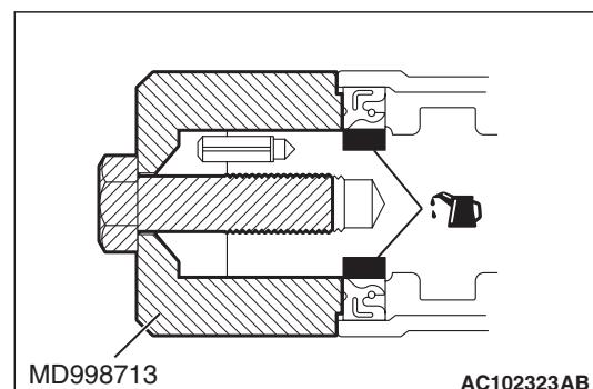
1. Apply engine oil to the entire inner diameter of the oil seal lip.
