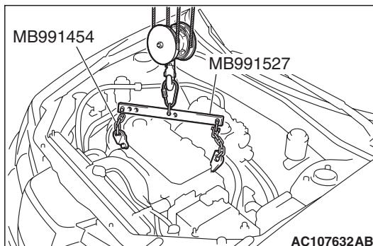
3. Hold the engine assembly with a chain block, etc.
