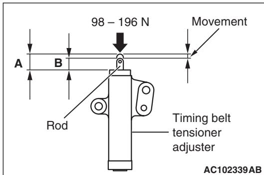
3. Hold the timing belt tensioner adjuster by hand, and press the top end of the rod onto the metal (e.g. cylinder block) under a pressure of 98 – 196 N to measure the movement of the rod.
