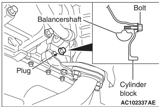
2. Adjust the timing mark of the engine oil pump sprocket. Unplug the cylinder block plug. Insert a bolt (M6 sectional width 10 mm, minor diameter 45 mm) from the plug hole and then check. If the bolt comes in contact with the balancer shaft turn the sprocket one rotation. Re-adjust the timing mark and then check to see that the bolt fits. Do not remove the bolt until the valve timing belt is assembled.
