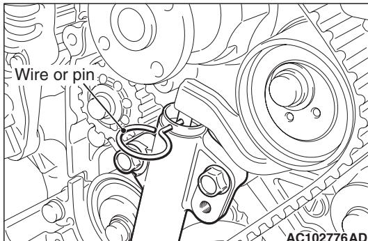
10. Insert wire or pin removed in Step 7 again, and ensure that it can be pulled out easily. When wire or pin can be easily removed, appropriate tension is applied on timing belt. In this case, remove wire or pin.
