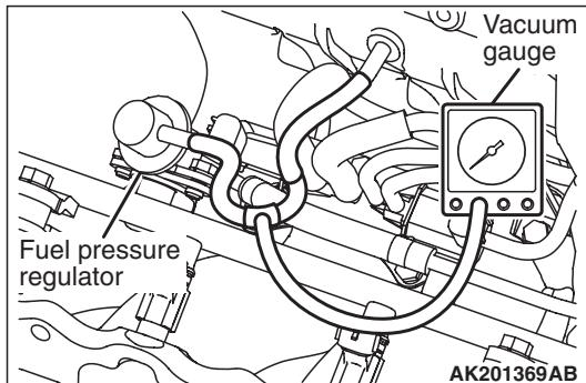
3. Attach a three-way joint to the vacuum hose between the fuel pressure regulator and the air intake plenum, and connect a vacuum gauge.
