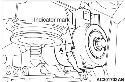
1. Make sure that the indicator mark is within the area marked with A in the illustration.
