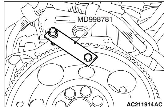
1. Use special tool flywheel stopper (MD998781) to secure the flywheel in the same manner as removal.
