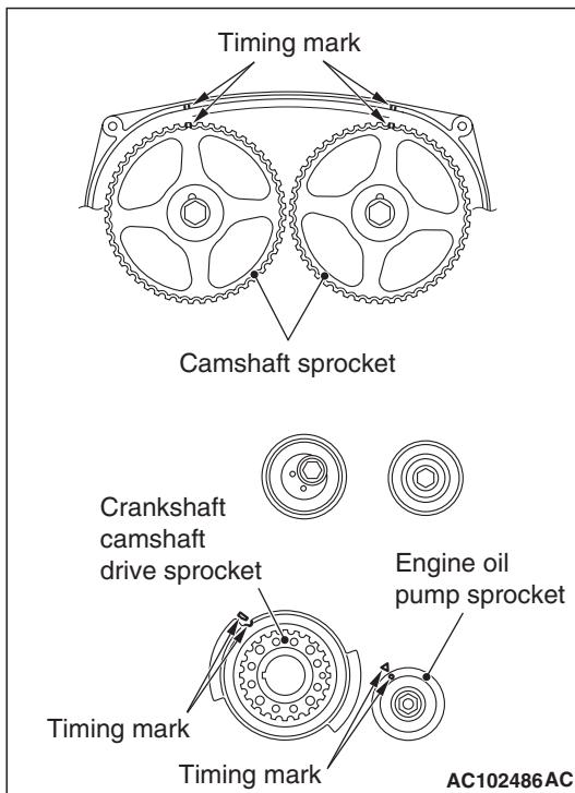
1. Align the timing marks on the camshaft sprocket, crankshaft camshaft drive sprocket and engine oil pump sprocket.
