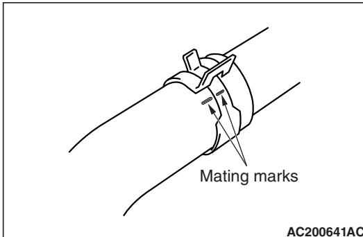
Make mating marks on the radiator hose and the hose clamp. Disconnect the radiator hose.
