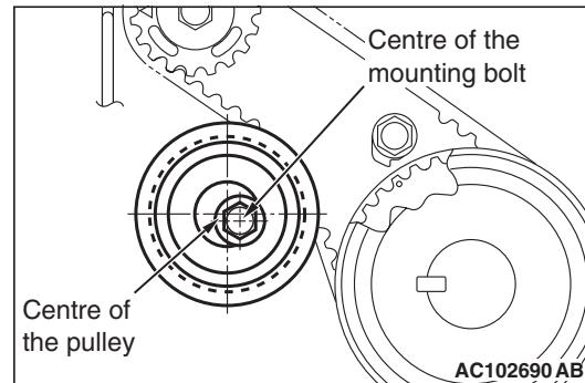
3. Assemble and temporarily fix the centre of the pulley of the balancer timing belt tensioner so that it is at the top left from the centre of the mounting bolt, and the pulley flange is at the front-side of the engine.
