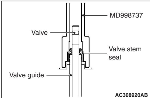
3. Use special tool to fill a new valve stem seal in the valve guide using the valve stem area as a guide.
