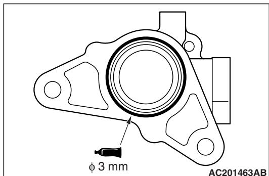
2. Apply the sealant to the camshaft position sensor support flange in a continuous bead as shown in the illustration.
