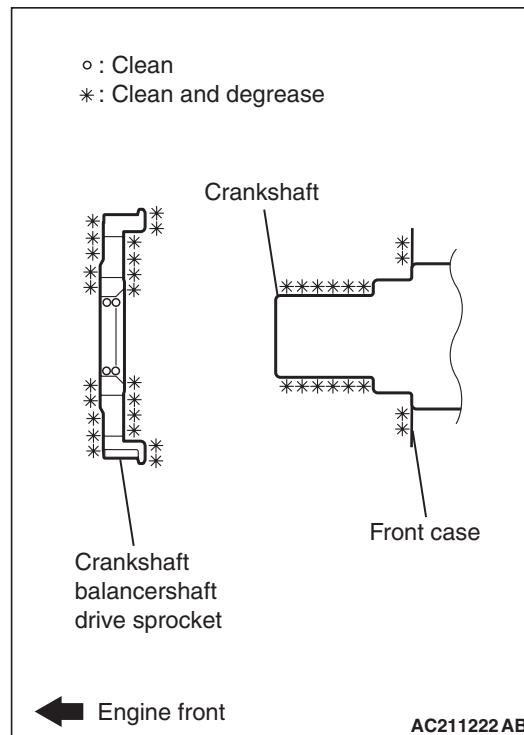
1. Clean or degrease the front case, the crankshaft and the crankshaft balancer shaft drive sprocket as shown.
