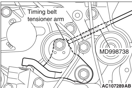
3. Screw in the special tool until it comes in contact with the timing belt tensioner arm.
