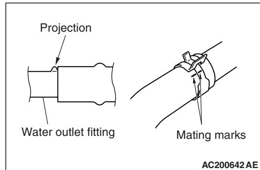
1. Insert each hose as far as the projection of the water outlet fitting.
