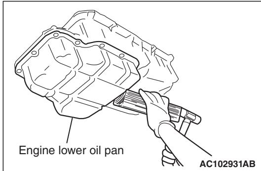
2. Apply a piece of wood to the lower oil pan and strike it with a hammer to remove the engine lower oil pan.
