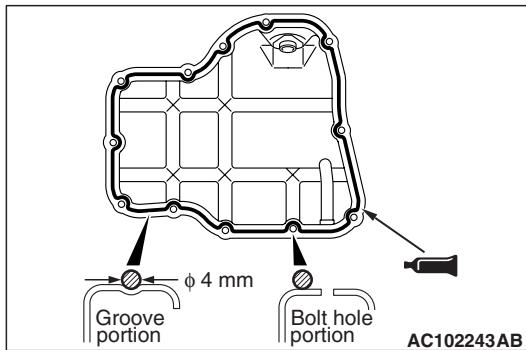
2. Apply a bead of the sealant to the mating surface of the engine lower oil pan as shown.
