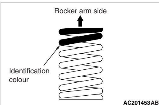
Install the valve springs with its identification colour painted end facing the rocker arm.
