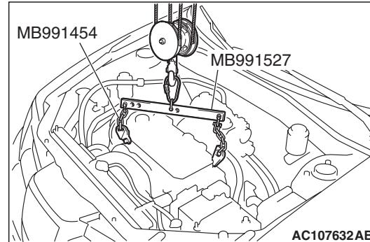
Install the engine assembly, being careful not to pinch the cables, hoses or wiring harness connectors.
