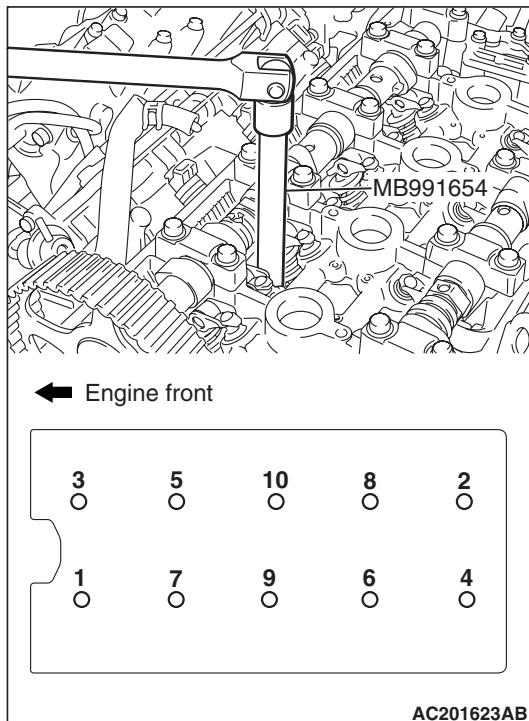
Using special tool cylinder head bolt wrench (MB991654), loosen the cylinder head bolts in two or three steps in the order of the numbers shown in the illustration.
