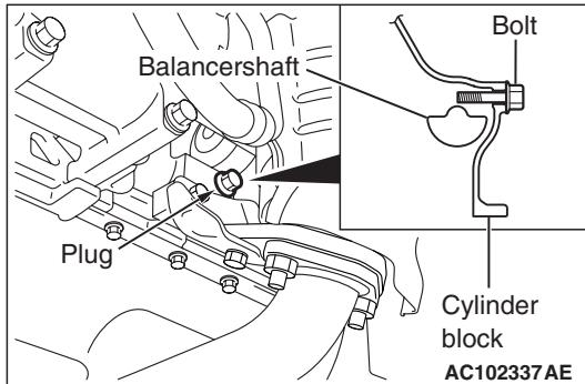
6. Remove the bolt inserted in Step 2 above, then assemble the cylinder block plug.
