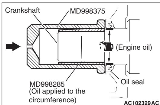
1. Apply a small amount of engine oil to the entire inner diameter of the oil seal lip.
