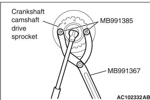
1. Use the following special tools to support the crankshaft camshaft drive sprocket.
