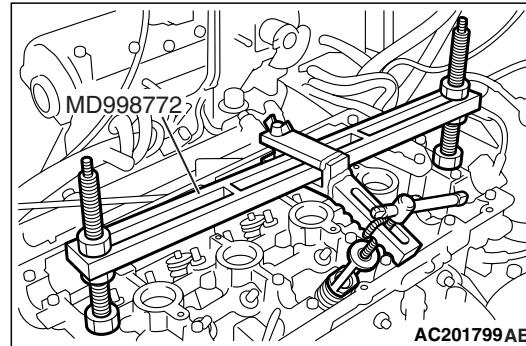
Use special tool valve spring compressor (MD998772) to compress the valve spring, remove the valve spring retainer locks.
