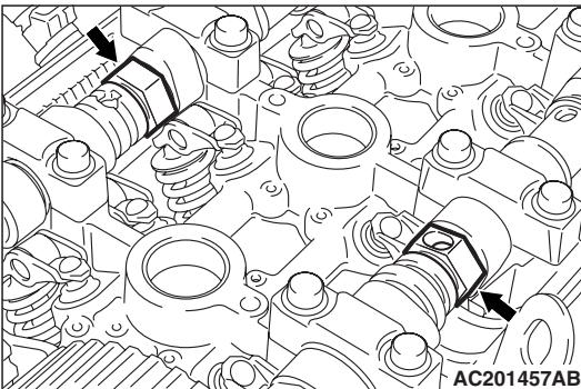
1. Hold the hexagon part of the camshaft with a wrench.
