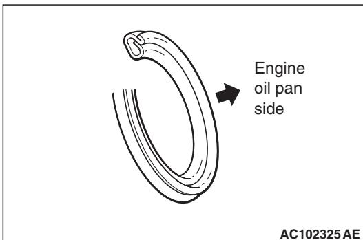
Replace the gasket with a new gasket. Install the new gasket in the direction shown in the illustration.
