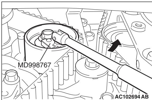
4. Turn the timing belt tensioner in the direction shown using special tool tensioner wrench (MD998767) to apply tension to the valve timing belt. Then pre-tighten the timing belt tensioner pulley.
