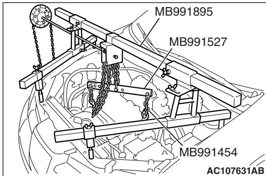
(1) <Special tool engine hanger (MB991895) is used>
