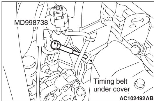
8. Remove the special tool adjusting bolt (MD998738), and install the rubber plug to the timing belt under cover.
