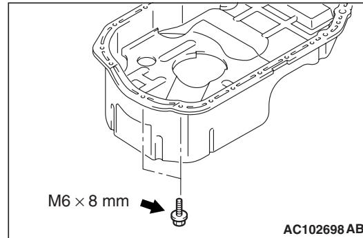
4. Tighten the engine oil pan mounting bolts to the specified torque. Be careful when installing, as the oil pan mounting bolts (indicated in the illustration) have different lengths from the other bolts.
