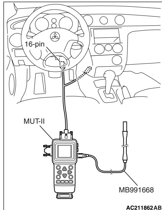
**To prevent damage to M.U.T.-II, always turn the ignition switch to the "LOCK" (OFF) position before connecting or disconnecting M.U.T.-II.**
