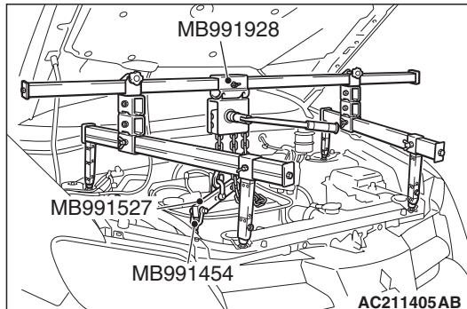
(2) <Special tool engine hanger (MB991928) is used>
