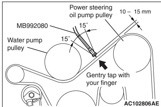
(5) Hold special tool MB992080 to the middle of the belt between the pulleys (at the place indicated by arrow) where it does not contact the belt (approximately 10 – 15 mm away from the rear surface of the belt) so that it is perpendicular to the belt (within an angle of  $\pm 15^\circ$ ).
