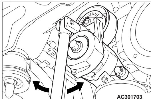
3. Securely insert the spindle handle or ratchet handle with a 12.7 mm insertion angle into the jig hole of the auto tensioner. Turn the auto-tensioner to the left and right to check and see that there is no threading.
