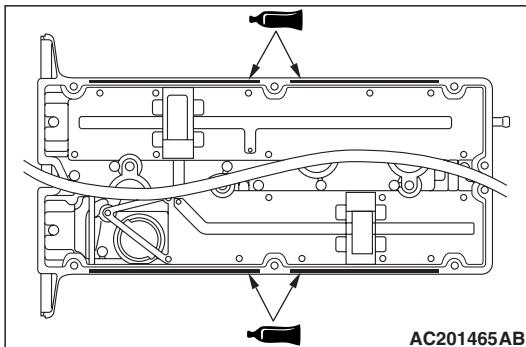
2. Apply sealant to the positions (4 areas) of the lower side of the rocker cover as shown in the illustration.
