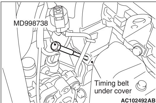
2. Remove the timing belt under cover rubber plug and then set the special tool adjusting bolt (MD998738).
