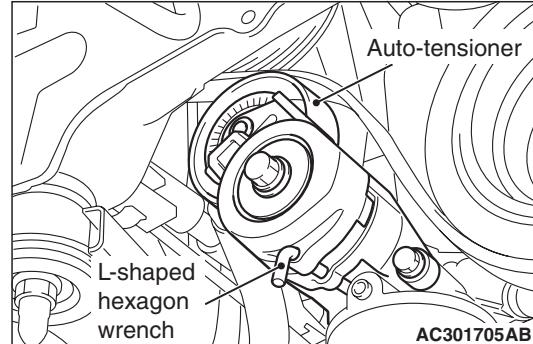
3. Insert an L-shaped hexagon wrench, etc. into the hole to fix and then remove the drive belt.
