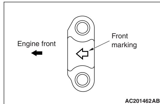
2. Since the shape of camshaft bearing caps No.2 – 5 is identical, check the identification marks so that the bearing cap No., inlet side, or exhaust side cannot be mistaken to install to the direction as shown in the illustration.
