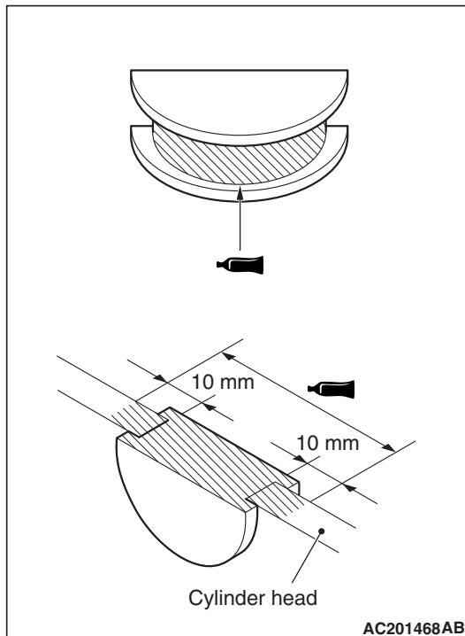
Apply sealant to the positions of the camshaft end seal as shown in the illustration and install to the cylinder head.
