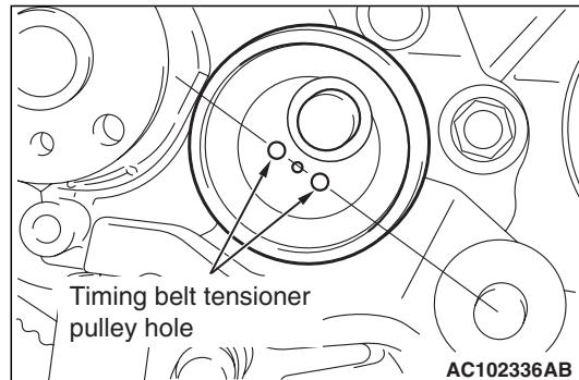
Temporarily tighten the timing belt tensioner pulley as shown.
