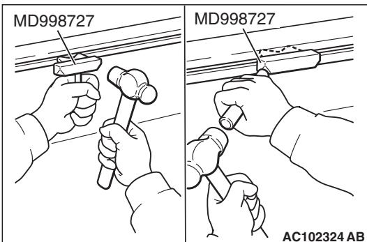
**Do not use special tool oil pan FIPG cutter (MD998727) in area A of the engine oil pan. Using the special tool in area A may cause deformation of the front case because the front case is made of aluminum.**
