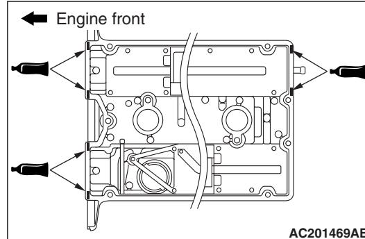
1. Apply sealant to the positions of the rocker cover gasket (6 areas) as shown in the illustration.
