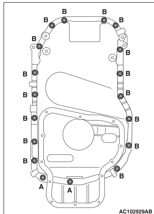
4. Insert the bolts to the engine upper oil pan as shown, and tighten them to the specified torque.
