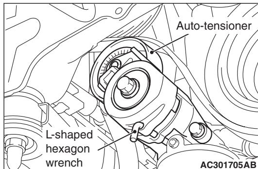
3. Insert an L-shaped hexagon wrench, etc. into the hole to fix and then remove the drive belt.
