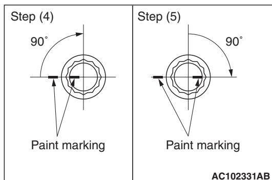
(4) Apply a paint mark to the heads of the cylinder head bolts and cylinder head, then tighten 90 degree angle as shown.
