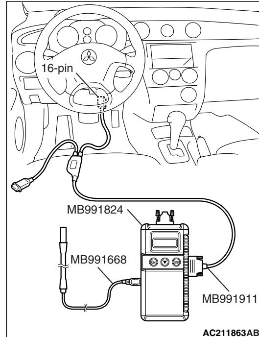
To prevent damage to special tool V.C.I. (MB991824), always turn the ignition switch to the "LOCK" (OFF) position before connecting or disconnecting special tool V.C.I. (MB991824).
