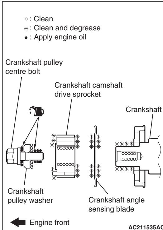
1. Clean or degrease the crankshaft, the crankshaft angle sensing blade, the crankshaft camshaft drive sprocket and crankshaft pulley washer as shown.
