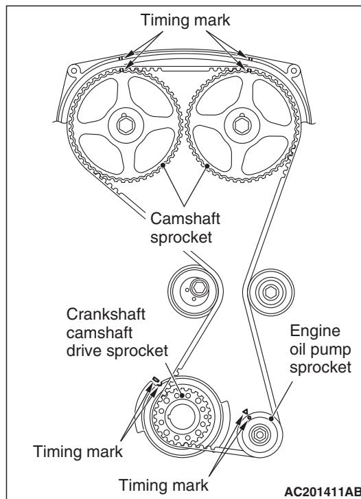
12. Check again that the timing marks on sprockets are aligned.
