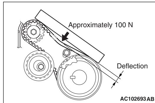
1. Apply a pressure of approximately 100 N at the centre (arrow area) between the sprocket as shown then inspect whether the deflection is within the standard value.
