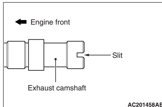
Do not install wrong camshaft at the side of inlet or exhaust. The exhaust camshaft has a slit at the rear surface.
