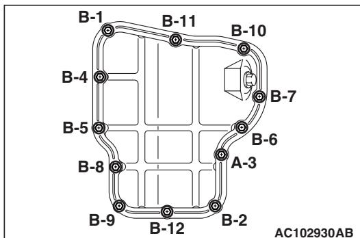
4. Insert the bolts to the engine lower oil pan as shown, and tighten them to the specified torque in the order shown.
