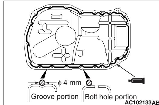
2. Apply a bead of the sealant to the cylinder block mating surface of the engine oil pan as shown.
