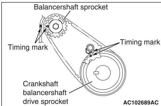
2. Turn the crankshaft clockwise two turns to set No.1 cylinder to TDC of its compression stroke and check that the sprocket timing marks are aligned.
