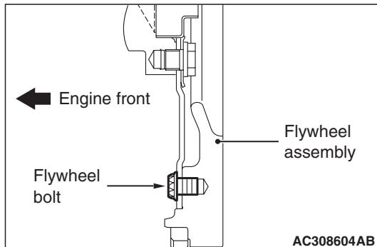
**Do not remove the flywheel bolt. If this bolt is removed, the flywheel assembly will become out of balance and damaged.**
