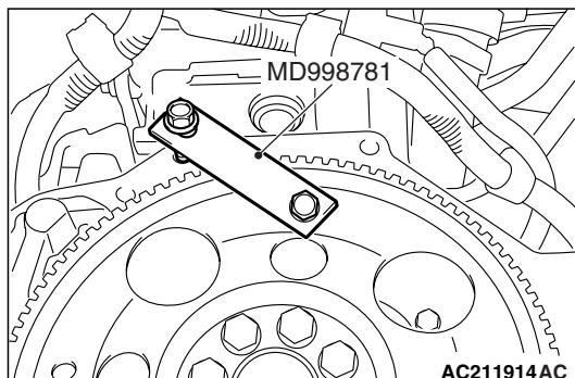
1. Use special tool flywheel stopper (MD998781) to secure the flywheel.
