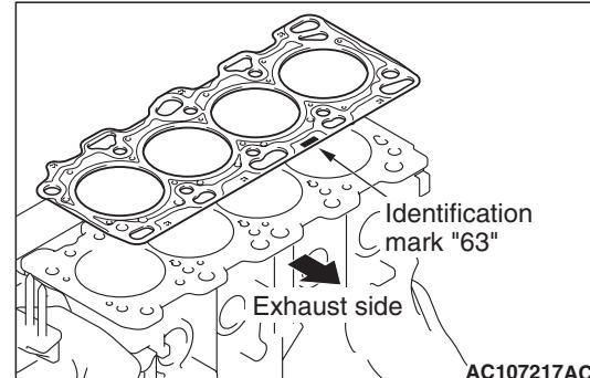
2. Assemble to the cylinder block so the cylinder head gasket identification mark "63" is at the top surface and on the exhaust side.
