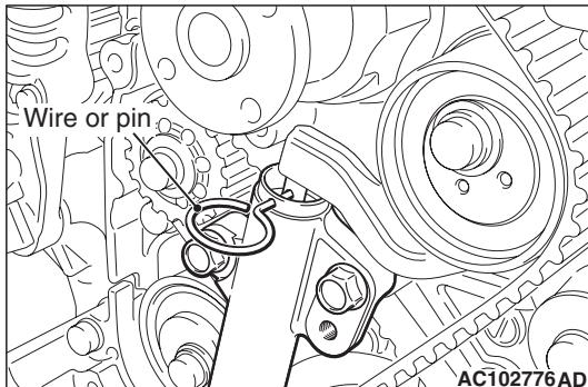
7. Remove wire or pin inserted to timing belt tensioner.
