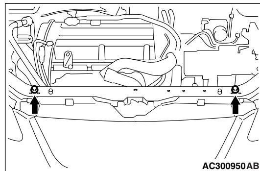
2. Remove from the car the 2 bolts, to assemble the radiator support upper insulator.
