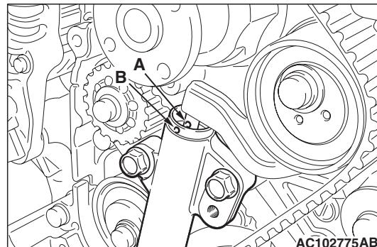
4. Gradually screw in the special tool. Then align the timing belt tensioner adjuster rod set hole A with the timing belt tensioner adjuster cylinder set hole B.
