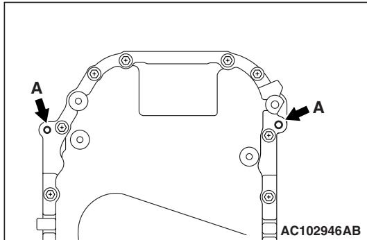
2. Screw in the bolt into bolt hole A in the location shown. Then lift the upper oil pan and remove it.
