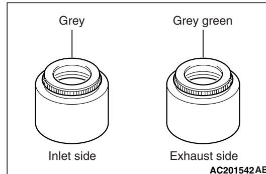
1. Check the valve stem seal colour to identify the inlet side or exhaust side.
