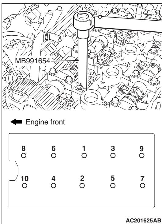
3. Use special tool cylinder head bolt wrench (MB991654) to tighten the cylinder head bolts as follows:
