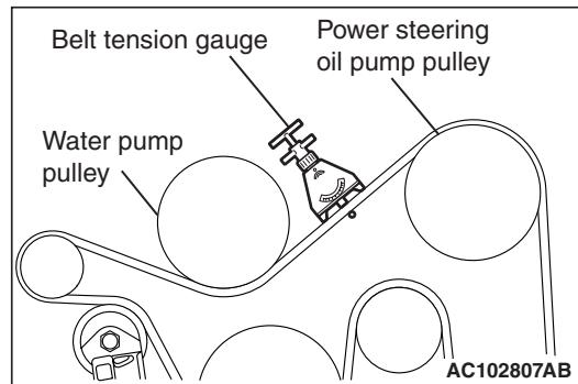
2. Use a belt tension gauge in the middle of the belt between the pulleys (at the place indicated by the arrow) to measure that the belt tension is within the standard value.
