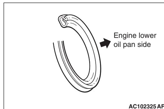
Replace the gasket with a new one. Install the new gasket in the direction shown in the illustration.
