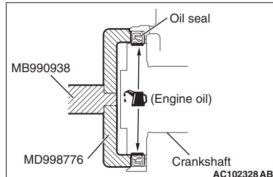
1. Apply a small amount of engine oil to the entire inner diameter of the oil seal lip.
