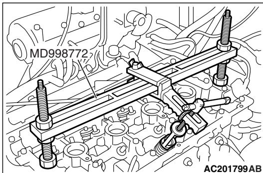
Use special tool valve spring compressor (MD998772) to compress the valve spring in the same manner as removal.
