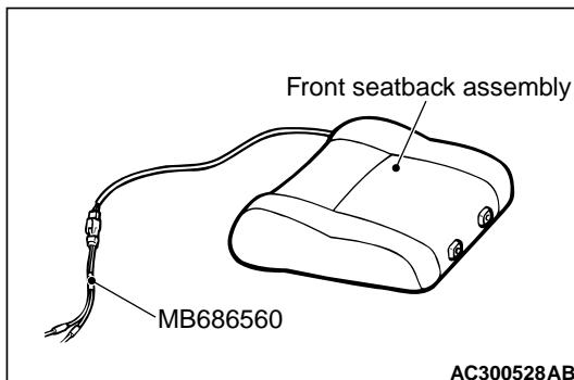
4. Place the front seatback assembly with its back contact with the earth.
