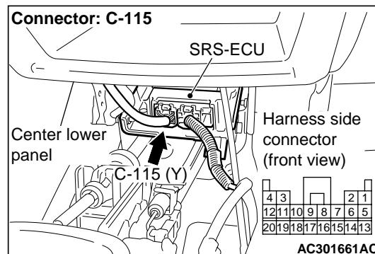
(2) Disconnect SRS-ECU connector C-115.
