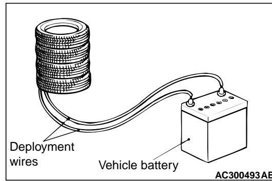
9. At a location as far away from the air bag module as possible, and from a shielded position, disconnect the two connected wires from each other, and connect them, to the two terminals of the battery (which has been removed from the vehicle) to deploy the air bag.
