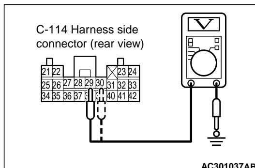
Do not insert a test probe into the terminal from its front side directly as the connector contact pressure may be weakened.
