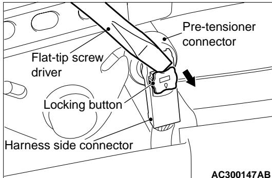
1. Use a flat-tipped screwdriver to pull out forward and unlock the locking button of the harness-side connector.
