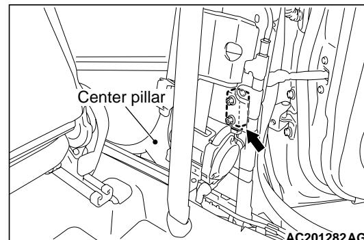
1. Check the centre pillar for deformation or rust.
