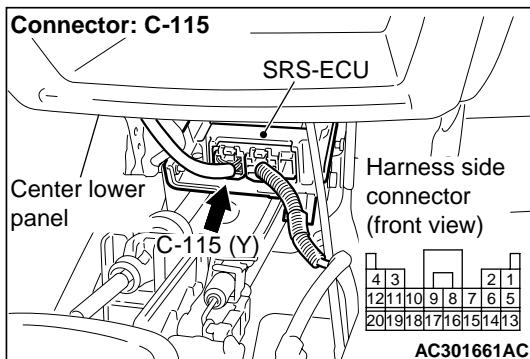
(1) Disconnect SRS-ECU connector C-115.
