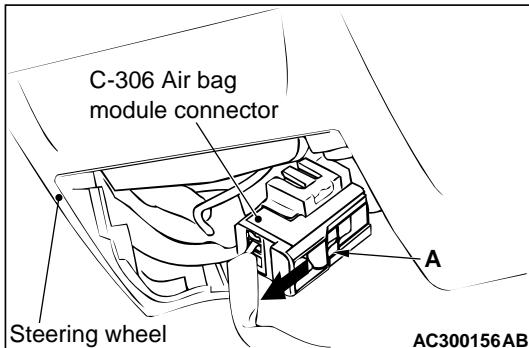
(2) By sliding the A section (in the figure) of air bag module connector C-306 in arrow direction, disconnect the connector.
