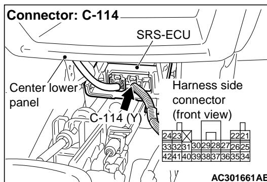
(1) Disconnect SRS-ECU connector C-114.
