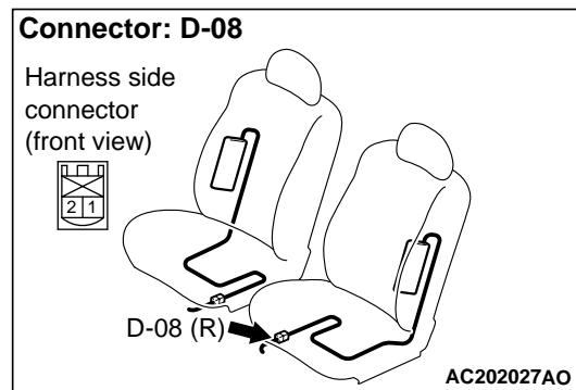
(2) Disconnect side air bag module (LH) connector D-08.
