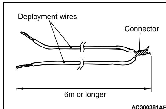
5. Obtain two suitable wires, which are 6 meters or longer, as deployment wires. Then connect the wires at one end to short.
