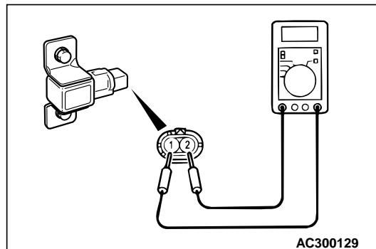
2. Measure the resistance between terminals and check whether it is within the standard value.
