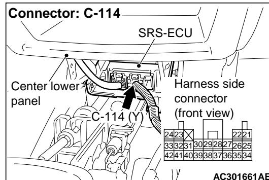
(1) Disconnect SRS-ECU connector C-114.
