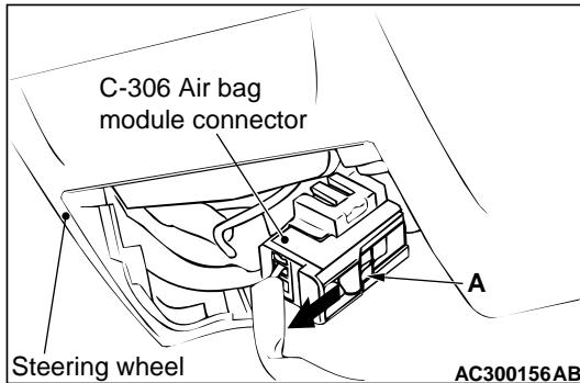
(2) By sliding the A section (in the figure) of air bag module connector C-306 in the arrow direction,
