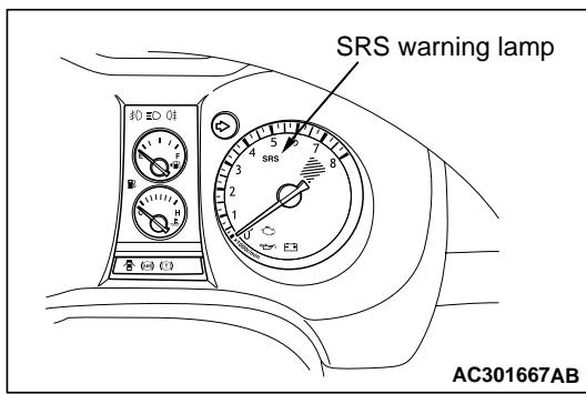
3. Does the SRS warning lamp illuminate for about 7 seconds, and then remain extinguished for at least 5 seconds after turning OFF?
