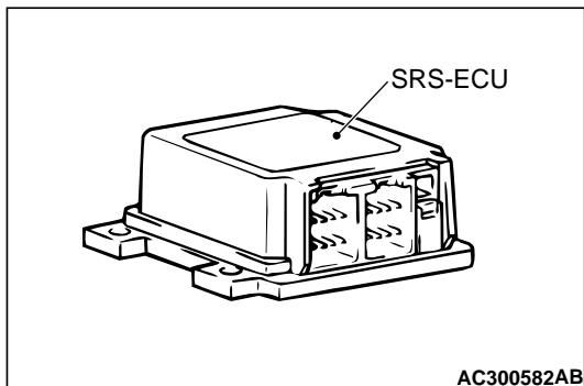
1. Check the SRS-ECU case and brackets for dents, cracks or deformation.
