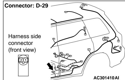
**To prevents the air bag from deploying unintentionally, disconnect the driver's seat belt pre-tensioner connector D-29 to short the squib circuit.**
