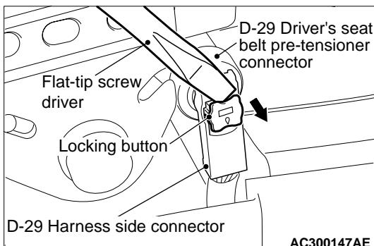
(2) Disconnect passenger's seat belt pre-tensioner connector D-29. Use a flat-tipped screwdriver to pull out the locking button at the harness side connector, and then disconnect the connector.
