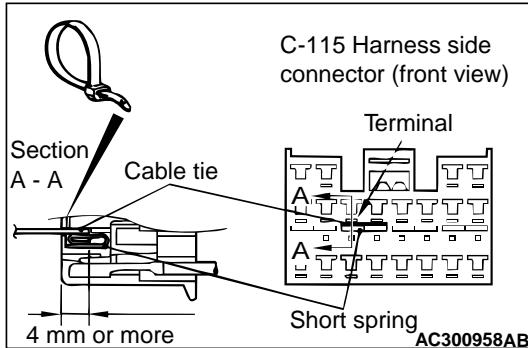
**Insert an insulator such as a cable tie to a depth of 4 mm or more, otherwise the short spring will not be released.**
