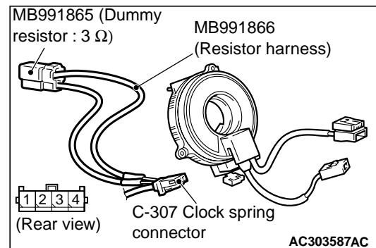
(3) Connect special tool dummy resistor (MB991865) to special tool resistor harness (MB991866).
