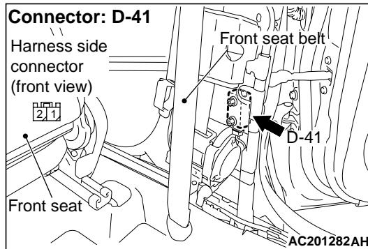
**NOTE:** If any harness wires between SRS-ECU connector C-114 and side impact sensor (RH) connector D-41 are damaged, repair or replace it. Then go to Step 3.
