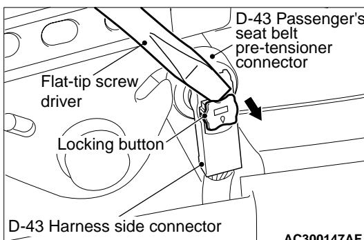
(2) Disconnect passenger's seat belt pre-tensioner connector D-43. Use a flat-tipped screwdriver to pull out the locking button at the harness side connector, and then disconnect the connector.
