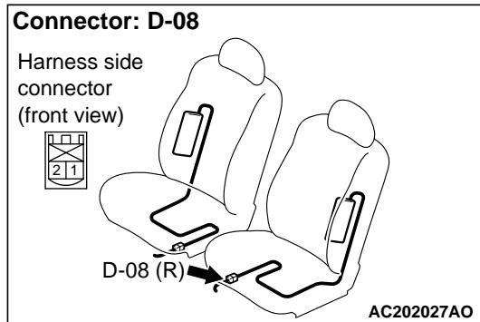
(2) Disconnect the side air bag module (LH) connector D-08.
