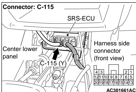
(1) Disconnect SRS-ECU connector C-115.
