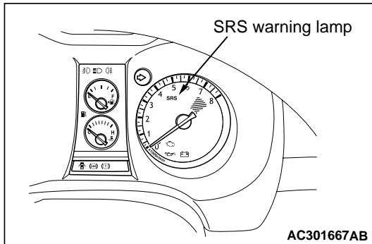
Turn the ignition key to the "ON" position. Does the SRS warning lamp illuminate for about 7 seconds, turn off and then remain extinguished for at least 5 seconds? If yes, SRS system is functioning properly. If no, consult page [P.52B-11](#).
