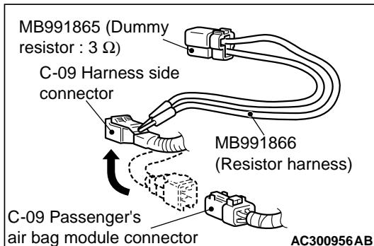
(3) Connect special tool dummy resistor (MB991865)
