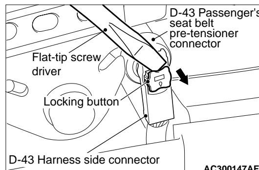
(2) Disconnect passenger's seat belt pre-tensioner connector D-43. Use a flat-tipped screwdriver to pull out the locking button at the harness side connector.
