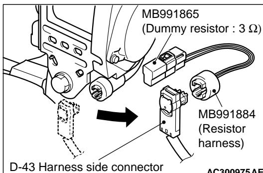
(3) Connect special tool dummy resistor (MB991865) to special tool resistor harness (MB991884).
