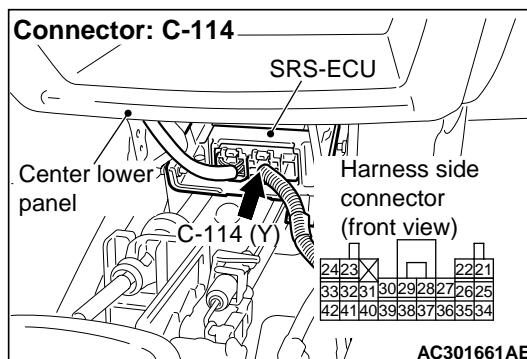
(1) Disconnect SRS-ECU connector C-114.
