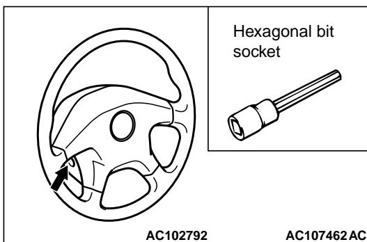
2. Insert the hexagonal bit socket into the arrow section in the figure. Completely loosen the bolt, and then remove the steering wheel air bag module assembly.
