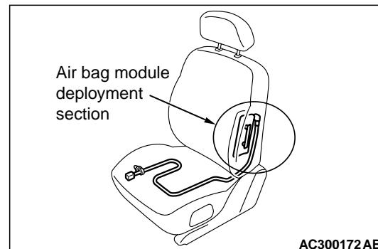
1. Check the side air bag module deployment section in the seat for dents and deformation.
