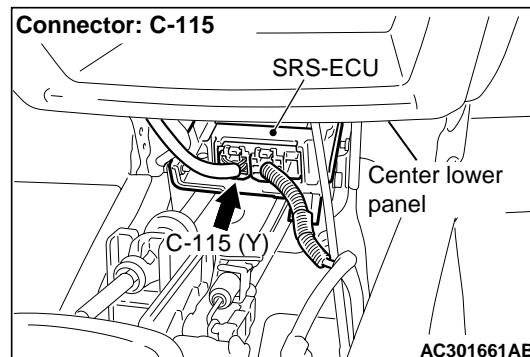
(1) Disconnect SRS-ECU connector C-115, and measure at the wiring harness side.
