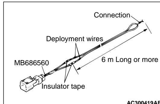
3. Connect deployment wires longer than 6 m to each special tool SRS air bag adapter harness (MB686560) and insulate the connections with plastic tape. Also, connect the deployment wires in the other ends to short, thereby preventing the passenger's air bag from accidental deployment caused by static etc.
