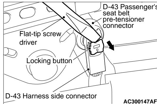
(2) Disconnect driver's seat belt pre-tensioner connector D-43. Use a flat-tipped screwdriver to pull out the locking button at the harness side
