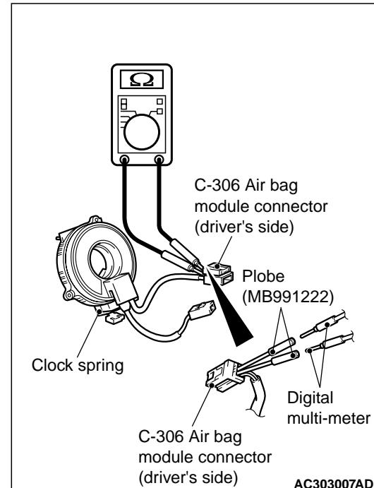
**Do not directly insert a probe, etc. into the terminal from the front of the connector.**
