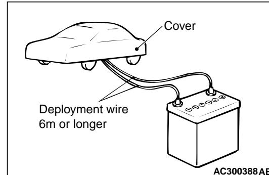
***If the glass is scratched, air bag deployment could cause it to crack and fly out of the vehicle, so always put a cover over the vehicle.***
