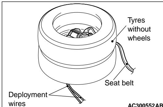
8. Pull the seat belt out the outside of the tyre, and then place one tyre without a wheel inside on top of the existing tyre.
