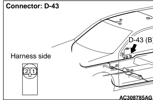
**To prevents the air bag from deploying unintentionally, disconnect the driver's seat belt pre-tensioner connector D-43 to short the squib circuit.**
