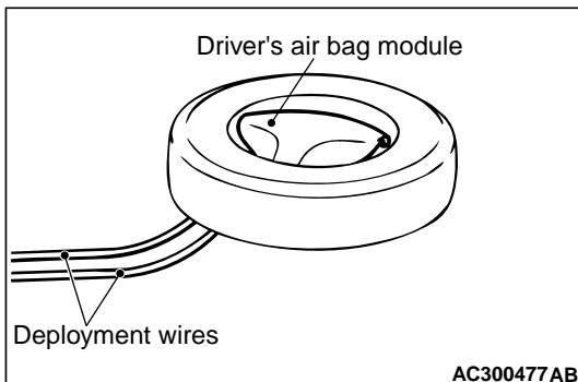
6. Install a nut to the bolt behind the driver's air bag module and tie thick wire there for securing.
