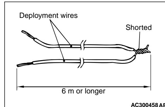
3. Obtain two suitable wires, which are 6 meters or longer, as deployment wires. Then connect the wires at one end to short.
