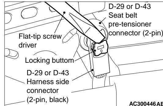
3. Use a flat-tipped screwdriver to unlock the locking button of the harness-side connector (2-pin, black) by drawing it toward you in two stages.
