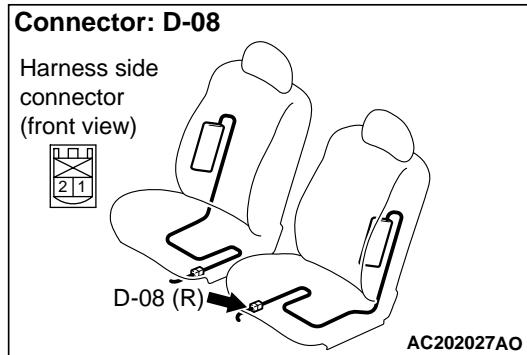
**To prevents the air bag from deploying unintentionally, disconnect the side air bag module (LH) connector D-08 to short the squib circuit.**
