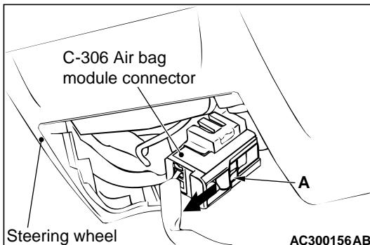
1. By sliding the A section (in the figure) of the air bag module connector in the arrow direction, disconnect the connector.
