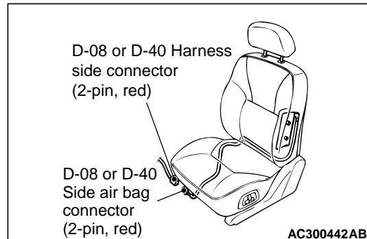
**The side air bag modules for both the driver's side and passenger's side should be deployed.**
