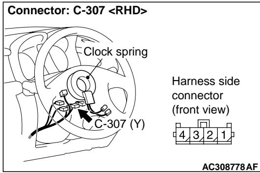
(1) Disconnect SRS-ECU connector C-115 and clock spring connector C-307.
