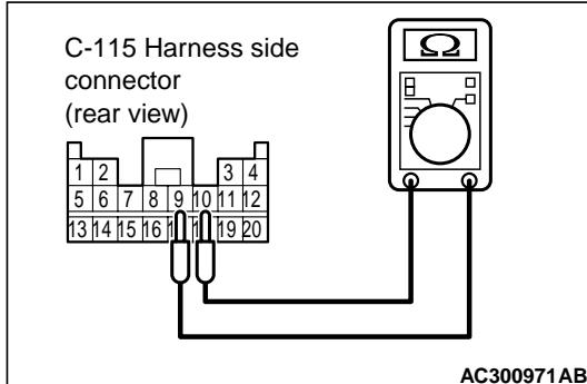
**Do not insert a test probe into the terminal from its front side directly as the connector contact pressure may be weakened.**
