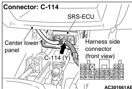
(1) Disconnect SRS-ECU connector C-114.
