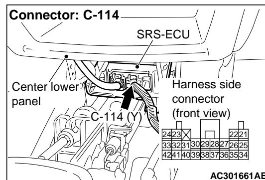
(1) Disconnect SRS-ECU connector C-114.
