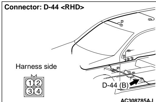
After inspecting intermediate connector D-31 <L.H. drive vehicles> or D-44 <R.H. drive vehicles> inspect the wiring harness. If the intermediate connector D-31 <L.H. drive vehicles> or D-44 <R.H. drive vehicles> is damaged, repair or replace it. Then go to Step 3. If any harness wires between SRS-ECU connector C-114 and side impact sensor (LH) connector D-27 are damaged, repair or replace it.
