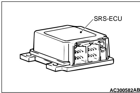
1. Check the SRS-ECU case and brackets for dents, cracks, deformation or rust.
