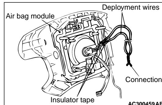
5. Using pliers, cut the driver's air bag module connector from the harnesses. Connect the deployment wires to each harness that has been cut and insulate the connections with plastic tape.
