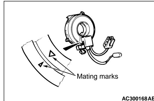
2. Align the mating marks of the clock spring.
