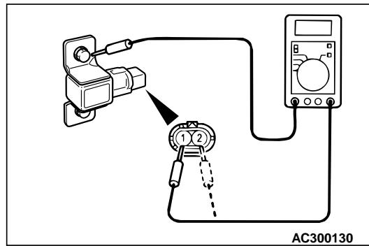
3. Check the continuity between the terminal and bracket. If there is a continuity, the insulation is malfunctioned, and replace the sensor with a new one.
