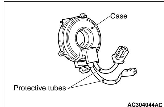
1. Check the clock spring connectors and protective tube for damage, and the terminals for deformation.
