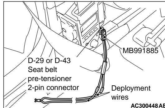
6. Connect the D-29 or D-43 seat belt pre-tensioner 2-pin connector (red) to special tool SRS air bag adapter harness (MB991885) and move the deployment harness out of the vehicle.
