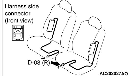
(2) Disconnect side air bag module (LH) connector D-08.
