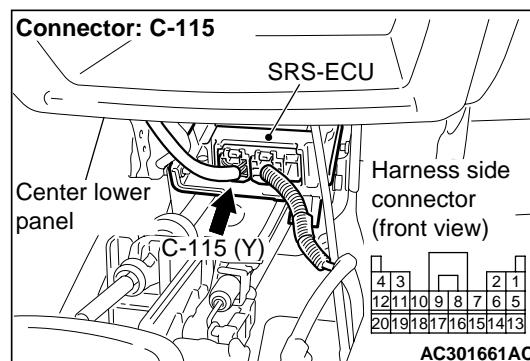
(2) Disconnect SRS-ECU connector C-115.
