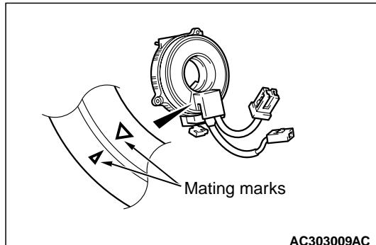
8. Align the mating marks of the clock spring and, after turning the vehicle's front wheels to straight-ahead position, install the clock spring to the column switch.
