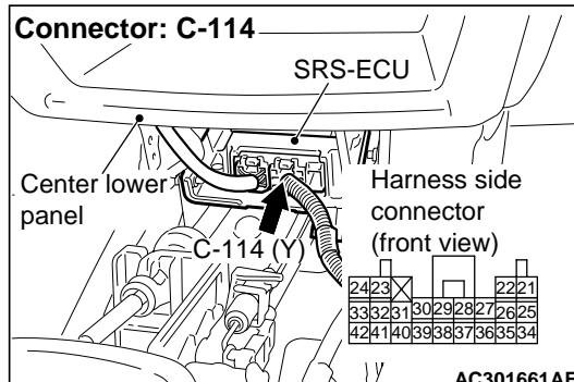
(1) Disconnect SRS-ECU connector C-114.
