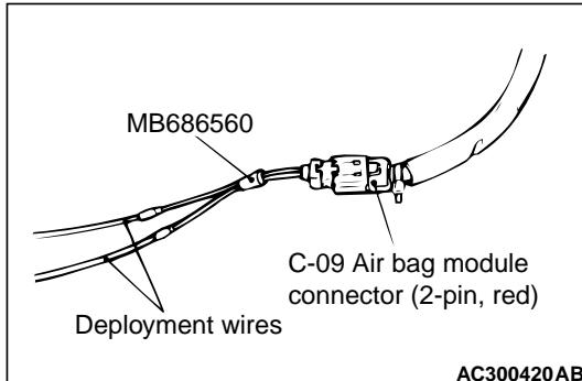
6. Connect the C-09 air bag module (front passenger's side) connector (2-pin, red) to special tool SRS air bag adapter harness (MB686560) and move the deployment wires out of the vehicle.
