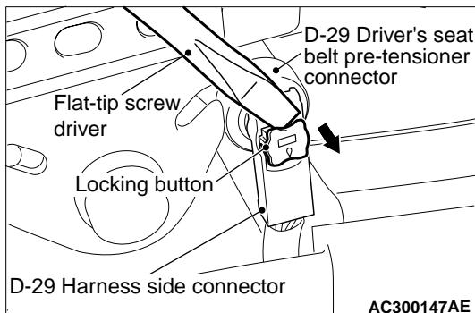
(2) Disconnect driver's seat belt pre-tensioner connector D-29. Use a flat-tipped screwdriver to pull out the locking button at the harness side connector, and then disconnect the connector.
