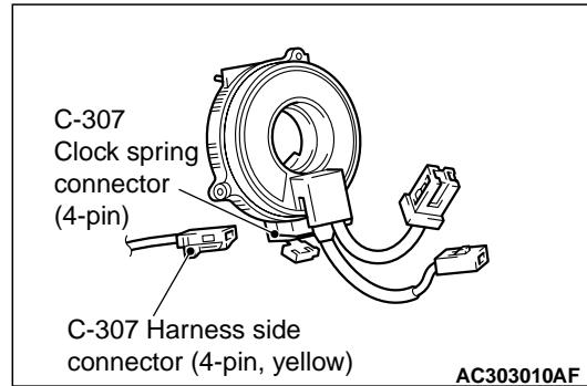
4. Remove the connection between the C-307 clock spring connector (4-pin) and the harness side connector (4-pin, yellow).
