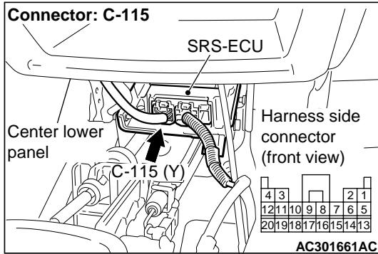
(1) Disconnect SRS-ECU connectors C-115.
