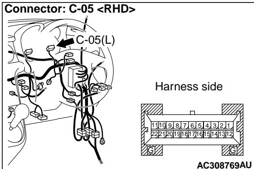
(2) Disconnect the combination meter connector C-05.
