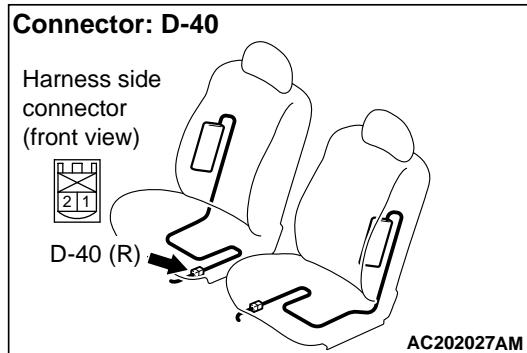
**To prevents the air bag from deploying unintentionally, disconnect the side air bag module (RH) connector D-40 to short the squib circuit.**
