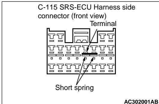
(2) Check the short spring for the warning lamp inside the harness side connector for improper contact or deformation.
