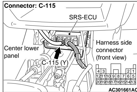
(1) Disconnect SRS-ECU connector C-115.
