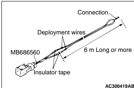
5. Connect deployment wires longer than 6 m to each special tool SRS air bag adapter harness (MB686560) and insulate the connections with plastic tape. Also, connect the deployment wires in the other ends to short, thereby preventing the passenger's air bag from accidental deployment caused by static etc.
