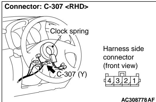
**To prevents the air bag from deploying unintentionally, disconnect the clock spring connector C-307 to short the squib circuit.**
