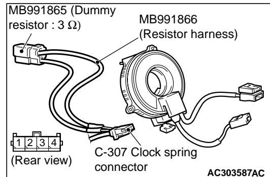
(2) Disconnect the clock spring connector C-307.
