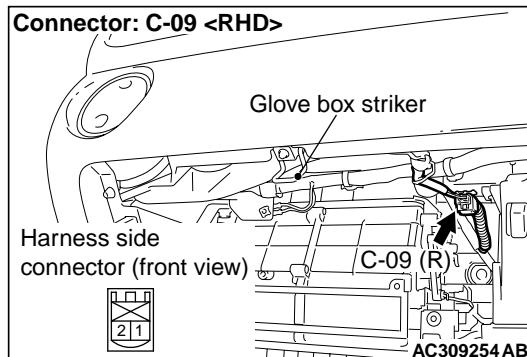
(1) Unclip passenger's air bag module connector C-09.
