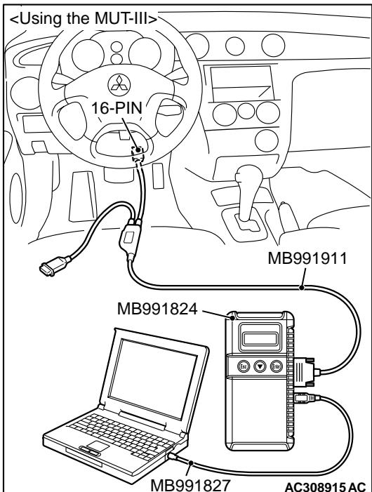
Refer to that the ignition switch is "LOCK" (OFF) when connecting or disconnecting MUT-II/III.
