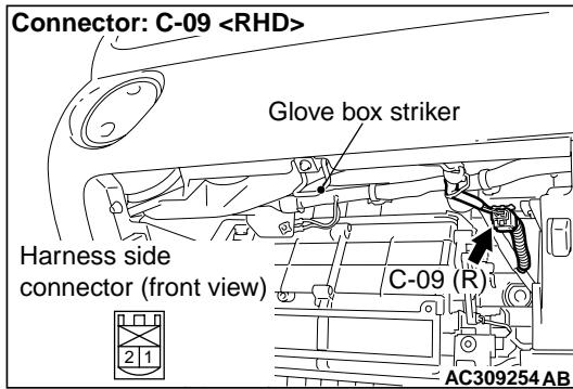
(2) Unclip passenger's air bag module connector C-09.
