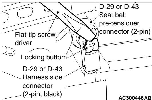
4. Execute the following steps to disconnect the connection between D-29 or D-43 seat belt pre-tensioner connector (2-pin) and harness side connector (2-pin, black).
