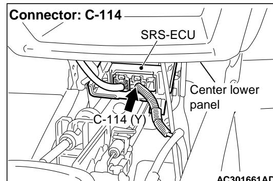
(1) Disconnect SRS-ECU connector C-114.
