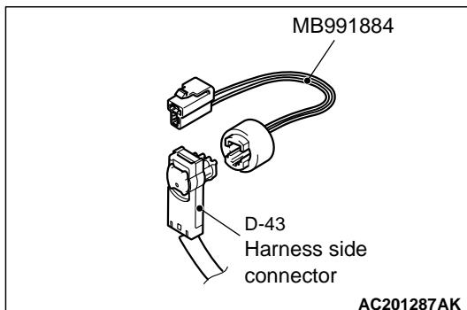
(2) Connect D-43 harness side connector to special tool resistor harness (MB991884).
