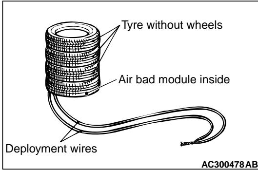
8. Place three old tyres without wheels on the tyre secured with the driver's air bag module.
