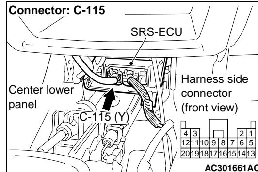
(1) Disconnect SRS-ECU connector C-115.
