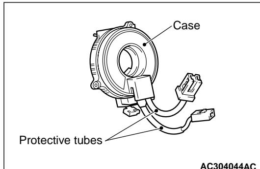
6. Check the clock spring connectors and protective tube for damage, and terminals for deformities.
