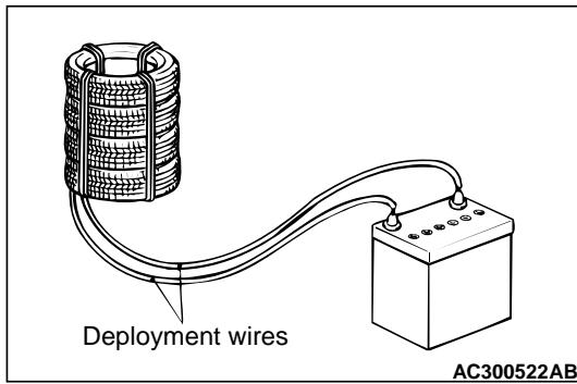
7. At a location as far away from the air bag module as possible, and from a shielded position, disconnect the two connected wires from each other, and connect them to the two terminals of the battery (which has been removed from the vehicle) to deploy the air bag.
