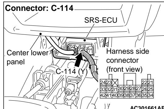
(1) Disconnect SRS-ECU connector C-114.
