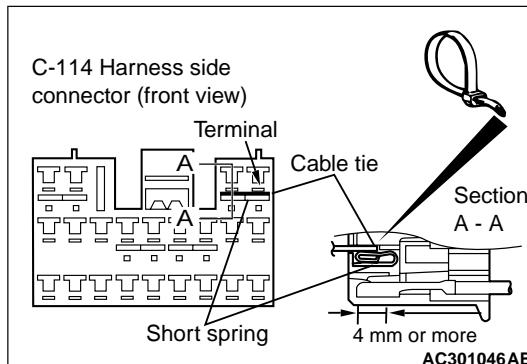
**Insert an insulator such as a cable tie to a depth of 4mm or more, otherwise the short spring will not be released.**
