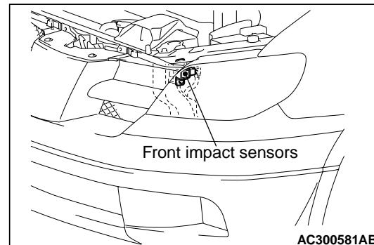
1. Check the front side member and front impact sensor for deformation or rust.
