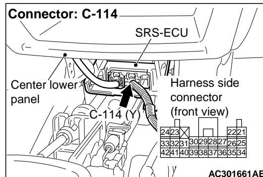
(1) Disconnect SRS-ECU connector C-114.
