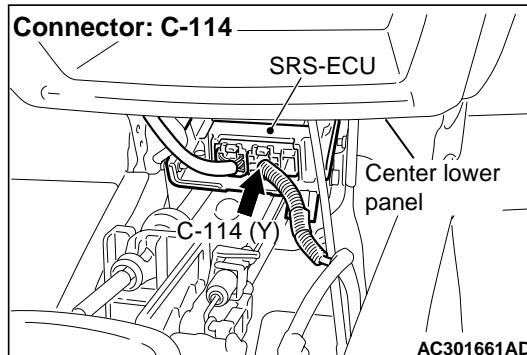
(1) Disconnect SRS-ECU connector C-114.
