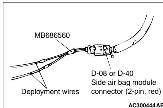
5. Connect the D-08 or D-40 side air bag module connector (2-pin, red) to special tool SRS air bag adapter harness (MB686560) and move the deployment wire out of the vehicle.
