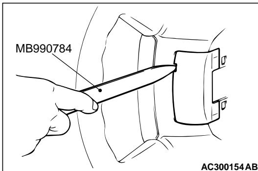
Insert the special tool ornament remover (MB990784) as shown in the illustration to remove the cover.
