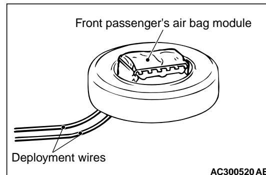
4. Connect the deployment wires to special tool SRS air bag adapter harness (MB686560), pass it beneath the tyre and wheel assembly, and connect it to the air bag module.
