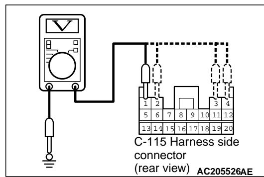
(6) Measure the voltage between terminal 1, 2, 3, 4 and body earth.
