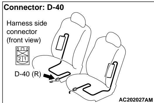
(1) Disconnect SRS-ECU connector C-114 and side air bag module (RH) connector D-40.
