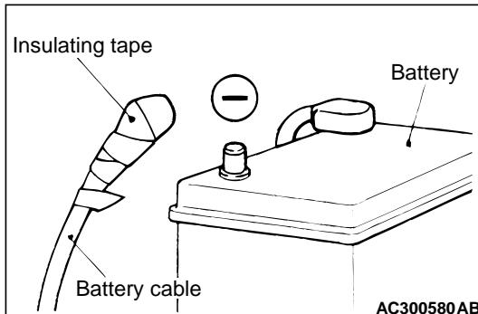
**Wait at least 60 seconds after disconnecting the battery cable before doing any further work (Refer to [P.52B-3](#)).**
