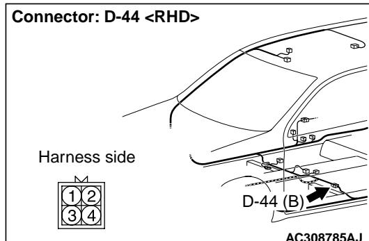
After inspecting intermediate connector D-31 <L.H. drive vehicles> or D-44 <R.H. drive vehicles> inspect the wiring harness. If the intermediate connector D-31 <L.H. drive vehicles> or D-44 <R.H. drive vehicles> is damaged, repair or replace it. Then go to Step 3.
