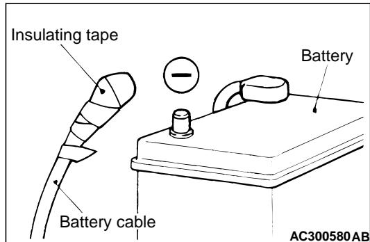
*After disconnecting the battery cable, wait 60 seconds or more before proceeding with the following work. In addition, insulate the negative battery terminal with a tape. The condenser inside the SRS-ECU is designed to retain enough voltage to deploy the air bag for a short time even after the battery has been disconnected, so serious injury may result from unintended air bag deployment if work is done on the SRS system immediately after the battery cables are disconnected.*
