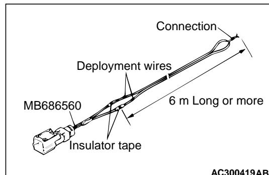
4. Connect deployment wires longer than 6 m to each special tool SRS air bag adapter harness (MB686560) and insulate the connections with plastic tape. Also, connect the deployment wires in the other ends to short, thereby preventing the passenger's air bag from accidental deployment caused by static etc.
