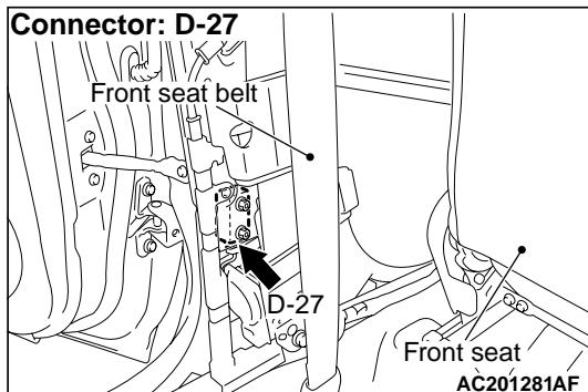
(2) Disconnect side impact sensor (LH) connector D-27, and measure at the wiring harness side.
