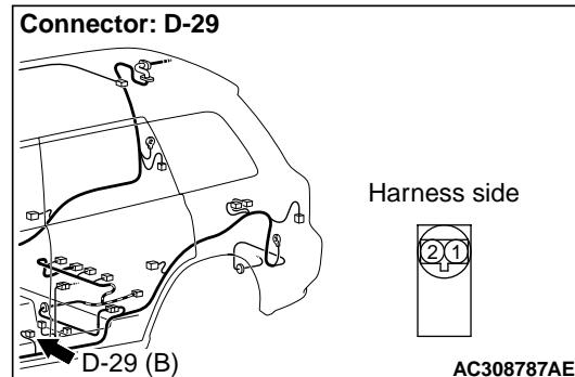
**To prevents the air bag from deploying unintentionally, disconnect the passenger's seat belt pre-tensioner connector D-29 to short the squib circuit.**
