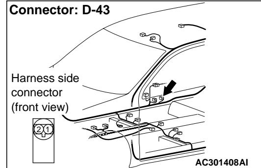
**To prevents the air bag from deploying unintentionally, disconnect the passenger's seat belt pre-tensioner connector D-43 to short the squib circuit.**
