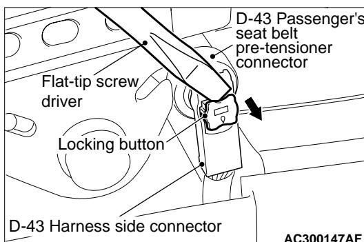
(2) Disconnect driver's seat belt pre-tensioner connector D-43. Use a flat-tipped screwdriver to pull out the locking button at the harness side connector, and then disconnect the connector.
