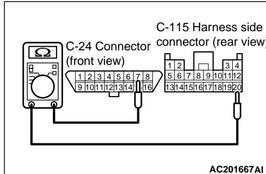
**Do not insert a test probe into the terminal 7 of the SRS-ECU connector C-115 its front side directly as the connector contact pressure may be weakened.**
