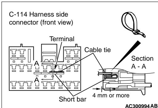
**Insert an insulator such as a cable tie to a depth of 4 mm or more, otherwise the short bar will not be released.**
