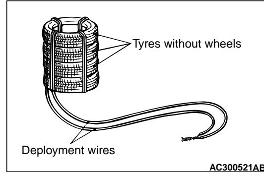
6. Place three old tyres without wheels on top of the tyre secured to the air bag module, and secure all tyres together with ropes (four locations).
