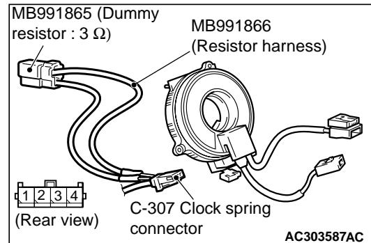
(2) Disconnect the clock spring connector C-307.
