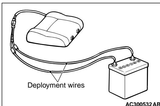
6. Disconnect the deployment wires as far from the front seatback assembly possible and connect the harnesses to the battery removed from the vehicle. Then, deploy.
