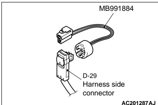
(2) Connect D-29 harness side connector to special tool resistor harness (MB991884).
