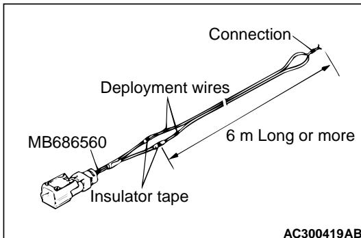
3. Connect deployment wires longer than 6 m to each special tool SRS air bag adapter harness (MB686560) and insulate the connections with plastic tape. Also, connect the deployment wires in the other ends to short, thereby preventing the passenger's air bag from accidental deployment caused by static etc.
