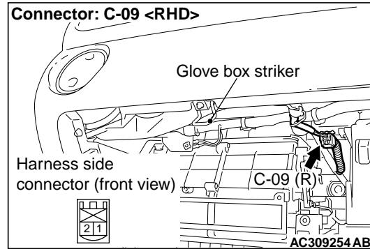
**To prevents the air bag from deploying unintentionally, disconnect the passenger's air bag module connector C-09 to short the squib circuit.**
