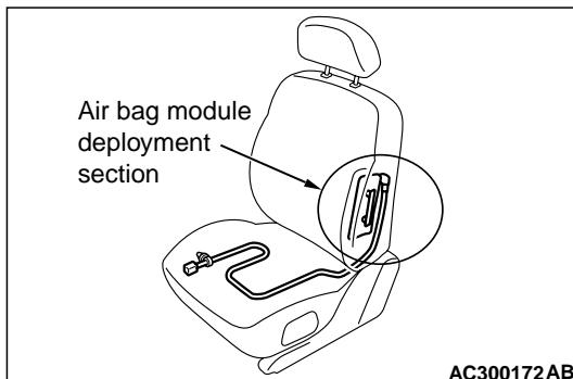
1. Check the air bag module deployment section for dents or deformation.
