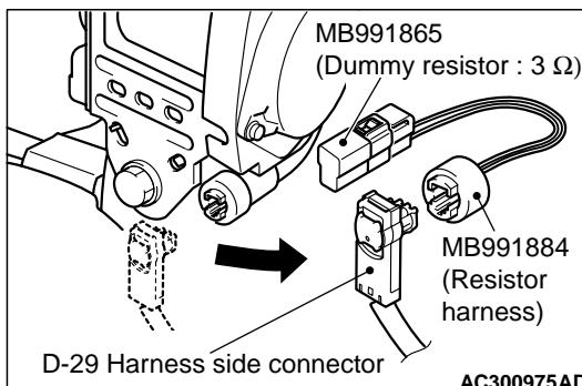
(3) Connect special tool dummy resistor (MB991865)
