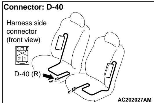
(2) Disconnect the side air bag module (RH) connector D-40.
