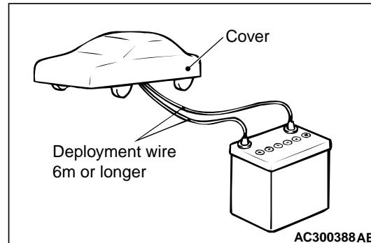
*If the glass is scratched, seat belt pre-tensioner operation could cause it to crack and fly out of the vehicle, so always put a cover over the vehicle.*
