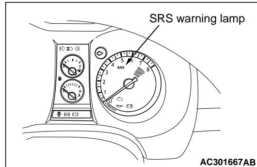
1. Check that the SRS warning lamp comes on when the ignition switch is turned ON.
