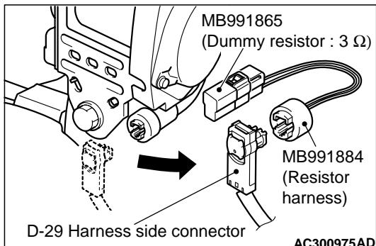
(3) Connect special tool dummy resistor (MB991865) to special tool resistor harness (MB991884).
