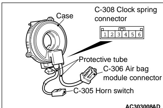
If any malfunction is found in the following inspections, replace the clock spring with a new one.
