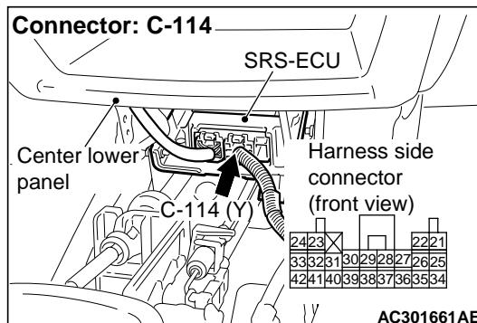
(1) Disconnect SRS-ECU connector C-114.
