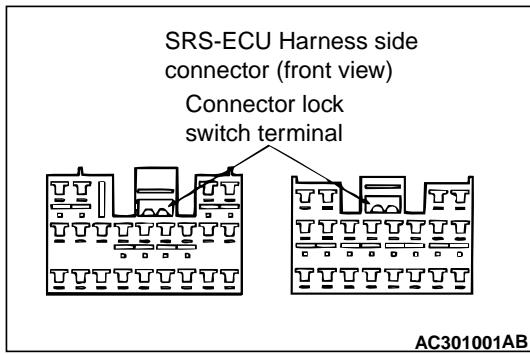
(2) Check the connector lock switch terminal inside
