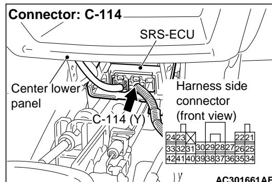
(1) Disconnect SRS-ECU connector C-114.
