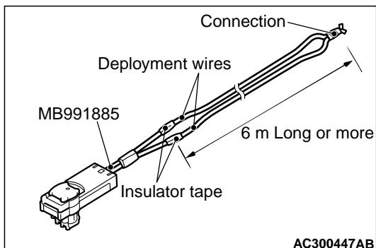
5. Connect deployment wires longer than 6 m to each special tool SRS air bag adapter harness (MB991885) and insulate the connections with plastic tape. Also, connect the deployment wires in the other ends to short, thereby preventing the passenger's air bag from accidental deployment caused by static etc.
