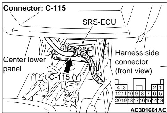
(2) Disconnect SRS-ECU connector C-115 and passenger's air bag module connector C-09.
