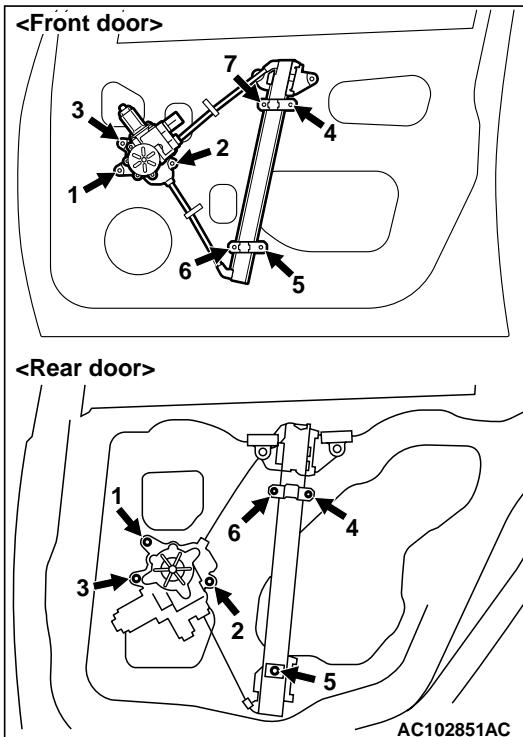
When installing the window regulator assembly, tighten the bolts to the specified torque in the order shown.
