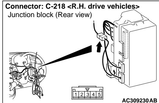
*Prior to the wiring harness inspection, check the junction block connectors C-203, C-210 and the intermediate connectors A-14, C-124, C-218 and repair if necessary. <R.H. drive vehicles>*
