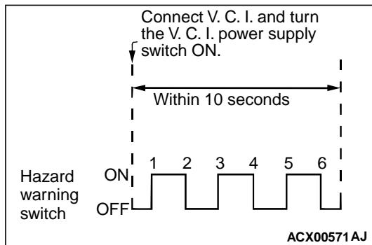
4. Within 10 seconds after turning the V.C.I. power switch to the "ON" position, press the hazard switch six times.
