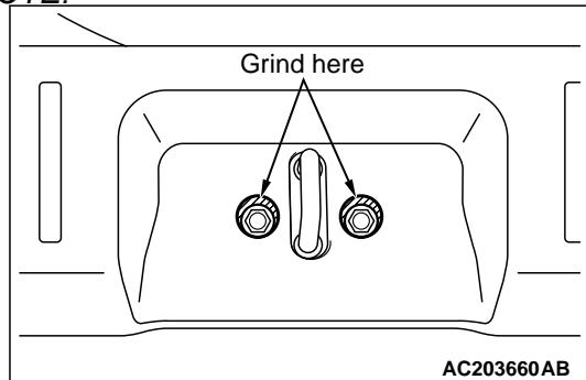
When the bolt head interferes with the rear end trim, rasp the interference area with a round file.
