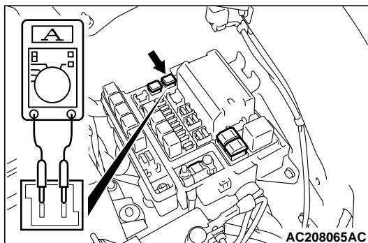
1. Remove the power window fuse and connect an ammeter as shown in the illustration.
