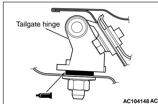
Apply the specified sealing agent to the tailgate hinge assembly surface to assemble the tailgate hinge.
