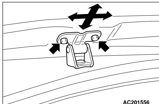
4. If uneven clearance is present between tailgate and body, reposition the hinge to adjust the clearance.
