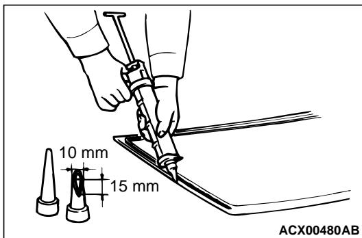
4. Fill a sealant gun with adhesive. Then apply the adhesive evenly around the windshield within 30 minutes after applying the primer.
