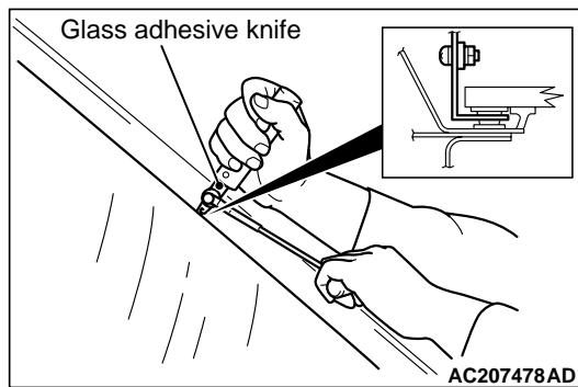
**Inserting the glass adhesive knife too deeply into windshield adhesive may damage windshield.**
