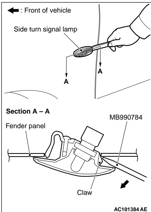
Use an appropriate tool such as special tool Ornament remover MB990784 to pry out the tab from the fender, and remove the side turn signal lamp.
