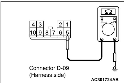
(2) Check the resistance between the sunroof motor assembly connector and body earth.
