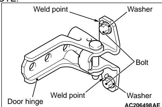
If the door hinge mounting bolt washers are welded, grind off the welding according to the procedure below beforehand.
