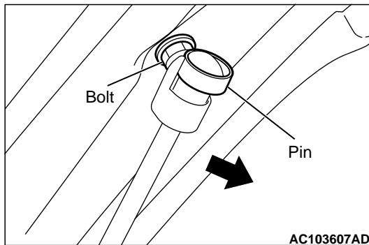
As shown in the Figure, slide the pin upward, then remove the tailgate gas spring in the direction of the arrow to unscrew the bolt.
