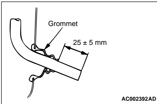
Install the grommet, and then position the drain pipe so that it protrudes from the grommet as shown in the illustration.
