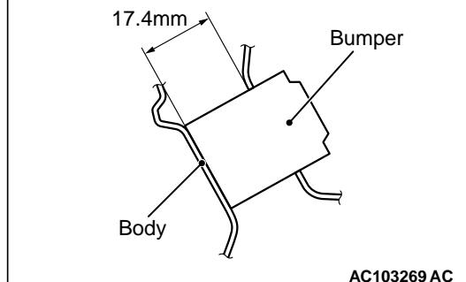
Turn the tailgate bumper using the arrow of the tailgate bumper as a guideline to adjust the height of the tailgate. The bumper height is altered by approximately 3mm by turning the tailgate bumper one rotation.
