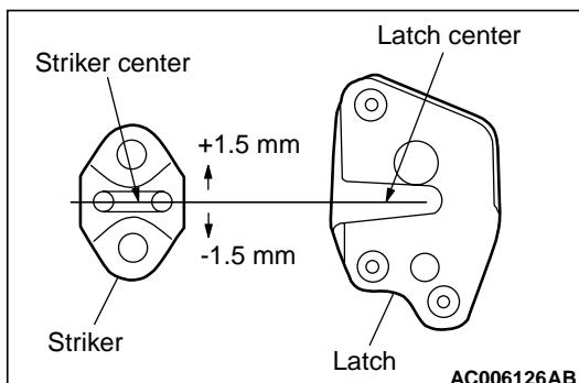
Assemble so the distance between the centre of the striker and centre of the latch is  $\pm 1.5\text{mm}$  or less.
