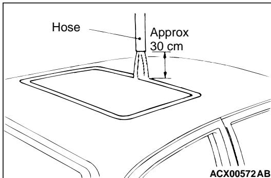
3. Hold the end of the hose approximately 30 cm above the roof and let the water run onto the weatherstrip for 5 minutes or more.
