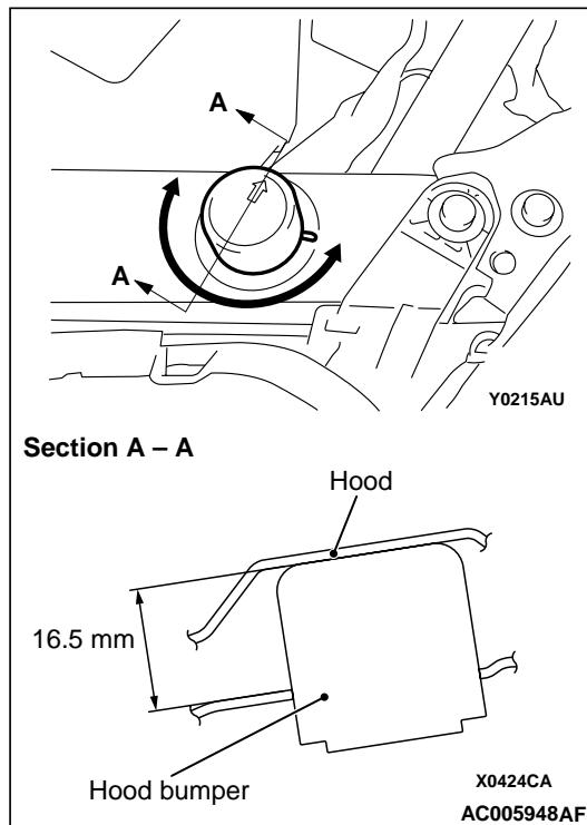
Rotate the hood bumper by using the arrow mark on the hood bumper as a guide to adjust the hood height. If the hood bumper is rotated just one turn, the hood height changes by approximately 3 mm.
