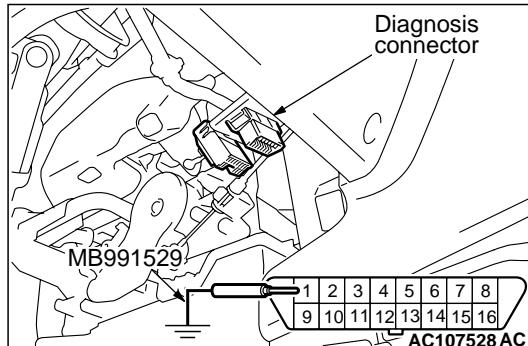
3. Connect the diagnosis connector to the special tool diagnosis code check harness MB991529.
