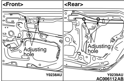
3. Loosen the door glass mounting screw via the adjusting hole with the door window glass fully closed, then lower the window glass a little.
