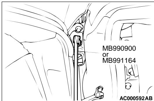
1. Use special tool door hinge adjusting wrench MB990900 or MB991164 to loosen the hinge mounting bolts on the body side, and then adjust the clearance around the door so that it is uniform on all sides.
