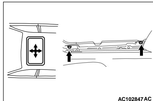
4. To adjust the roof lid glass in the front/back or left/right direction, loosen the nuts securing the roof lid glass assembly, then move the roof lid glass assembly to the front/back or left/right. Check to see that the space between the roof lid glass and body is even across the entire circumference.
