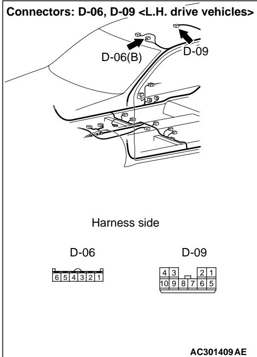
**STEP 6. Check the wiring harness between D-09 sunroof motor assembly connector terminal No.8 and D-06 sunroof switch connector terminal No.5.**
