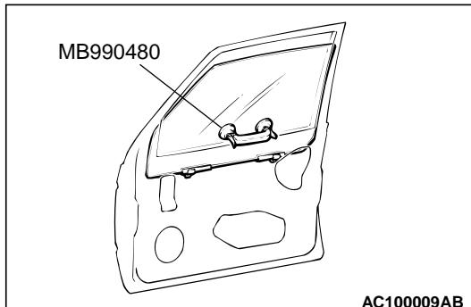
2. Lift the door window glass, and attach special tool window glass holder MB990480 to the glass as shown to prevent the glass from falling.
