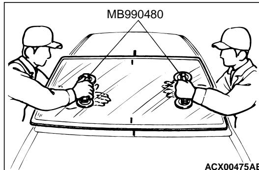
**5. Use special tool window glass holder MB990480 to remove the windshield.**
