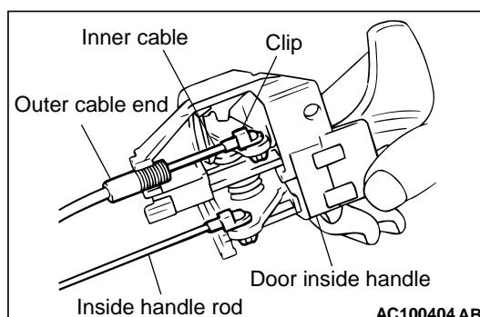
5. Adjust the door inside handle play with the outer cable end connecting the door inside handle and inside lock cable.
