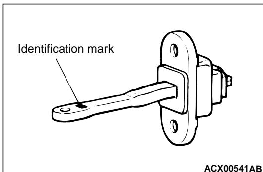
Install the door check so that the identification mark faces upwards.
