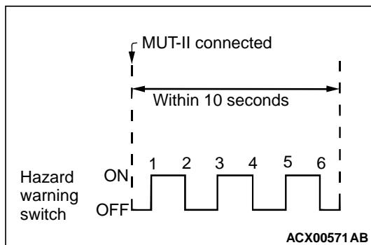
4. Press the hazard warning switch six times within 10 seconds.
