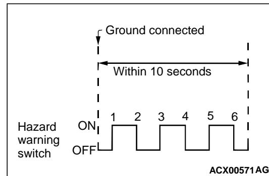
4. Press the hazard warning lamp switch six times within 10 seconds.
