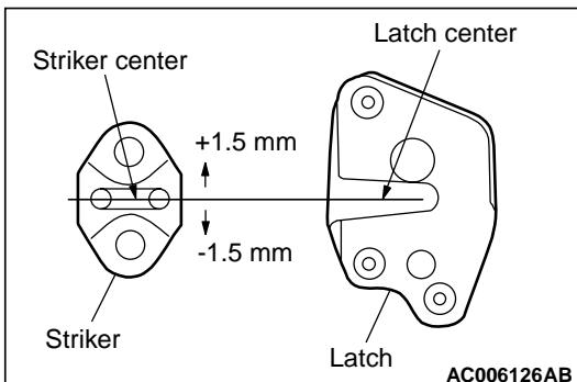
Align the centre of the striker and latch within  $\pm 1.5$  mm, and install.
