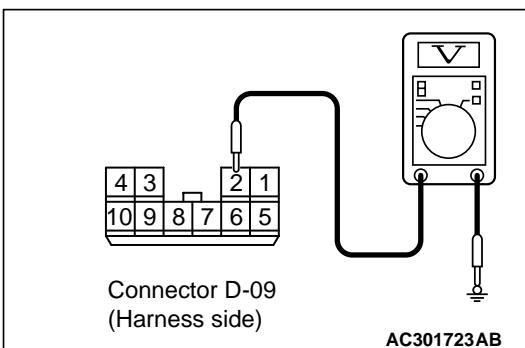
(2) Check the voltage between the sunroof motor
