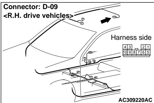
(1) Disconnect the sunroof motor assembly connector, and measure at the harness side.
