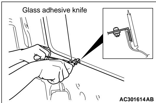
**Inserting the adhesive knife too deeply into windshield adhesive may damage quarter window glass.**
