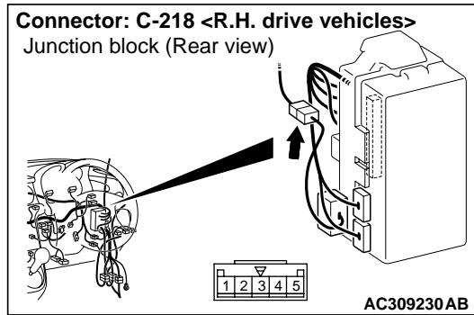
*Prior to the wiring harness inspection, check intermediate connector C-218, and repair if necessary.*
