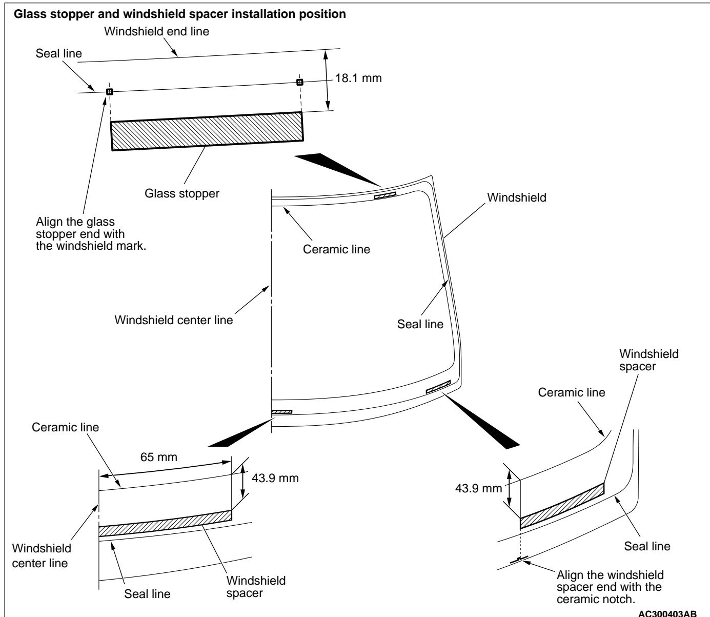
2. The inner side of the windshield is curved, therefore, make a point to assemble the glass stopper and windshield spacer without any lifting and assemble in the position shown.
