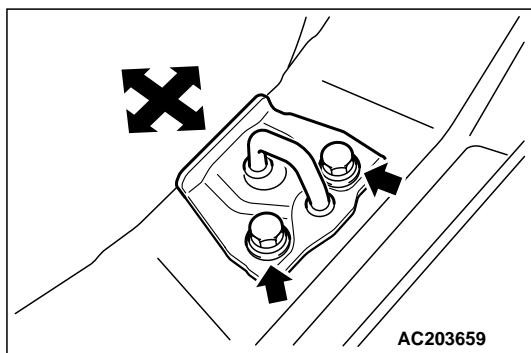
2. Move the replaced striker forward and backward or to the left and right to adjust, after bolt the striker temporarily.
