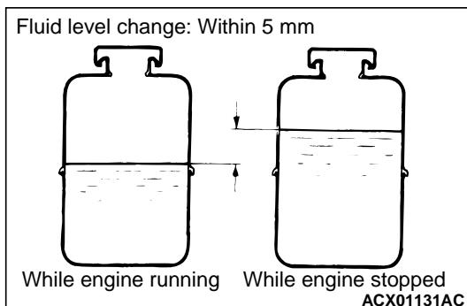
4. Check the fluid in the oil reservoir for foaming or milkiness. Check the difference of the fluid level when the engine is stopped, and while it is running. If the change of the fluid level is 5 mm or more, air bleeding should be done.
