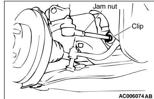
3. Loosen the jam nut, and unclip the bellows.
