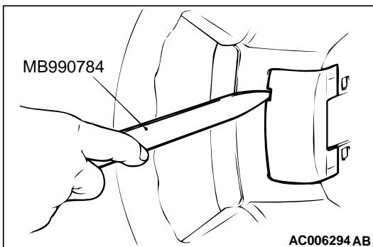
Insert special tool ornament remover (MB990784) at the indicated position to remove the cover.
