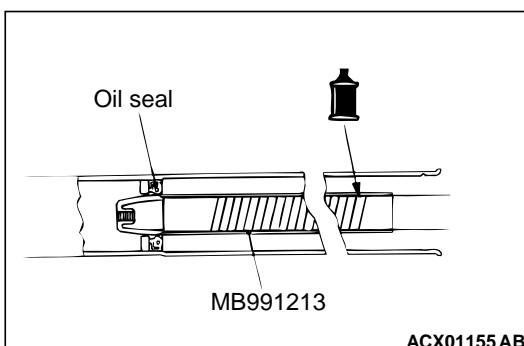
2. Cover rack serrations with special tool rack installer (MB991213).
