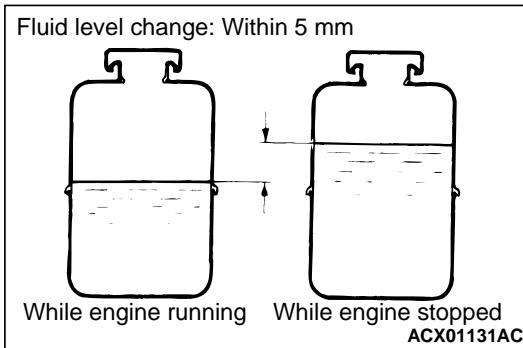
9. Confirm that the change in the fluid level is no more than 5 mm when the engine is stopped and when it is running.
