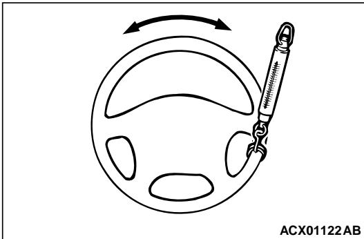
2. Measure the play on the steering wheel circumference before the wheels start to move when slightly moving the steering wheel in both directions.
