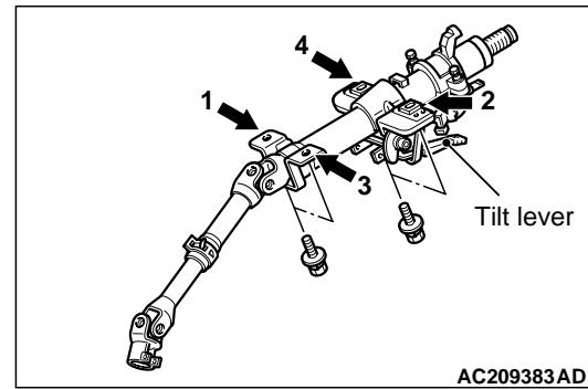
Ensure that the tilt lever is in the lock position, and install the steering column. Tighten the four bolts in the order shown by hand, and then tighten them to the specified torque in the order shown.
