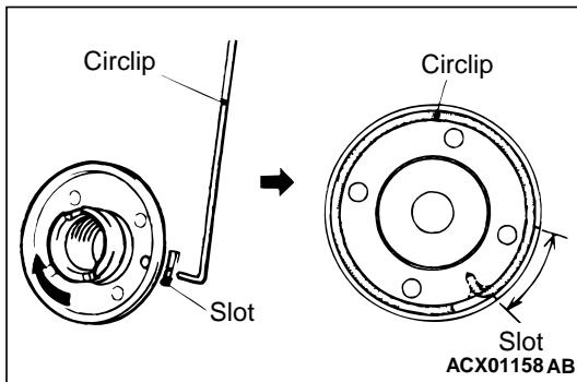
Insert the circlip to the rack stopper hole through cylinder hole. Turn the rack stopper clockwise and insert the circlip firmly.
