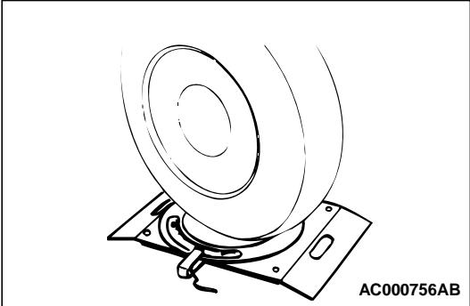
1. Place the front wheel on a turning radius gauge and measure the steering angle.
