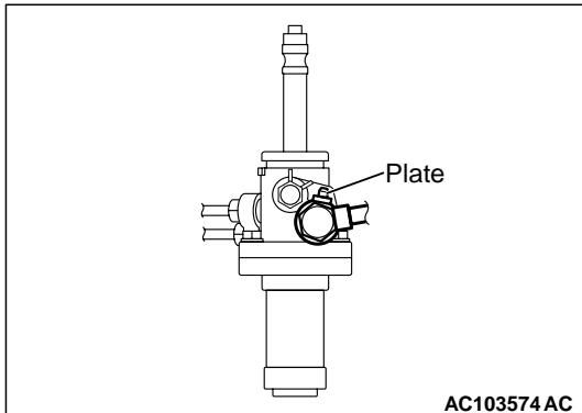
Install the pressure hose assembly so that its plate is positioned as shown in the illustration.
