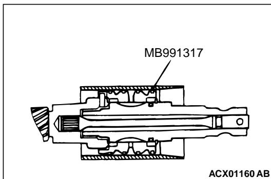
Because the seal rings expand after installation, tighten after installing by using special tool seal ring installer (MB991317) to compress the rings, or press down by hand.
