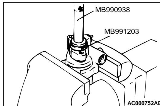
Use following special tool to install the oil seal.
