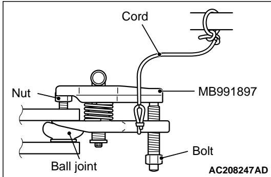
1. Install the special tool ball joint remover (MB991897) as shown in the figure.
