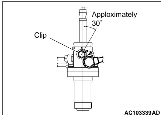
Install the return hose so that the clip is positioned as shown in the illustration.
