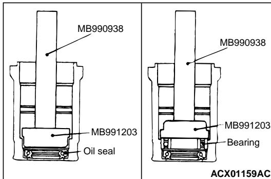
Apply a coating of ATF DEXRON III or DEXRON II to the outside of the upper oil seal/upper bearing. Using the following special tools, press the upper oil seal/upper bearing into the valve housing.
