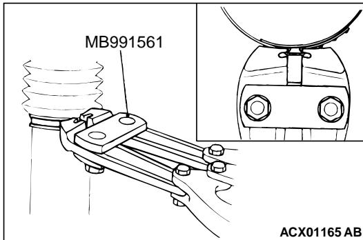
2. Use special tool boot band crimping tool (MB991561) to crimp the bellows band.
