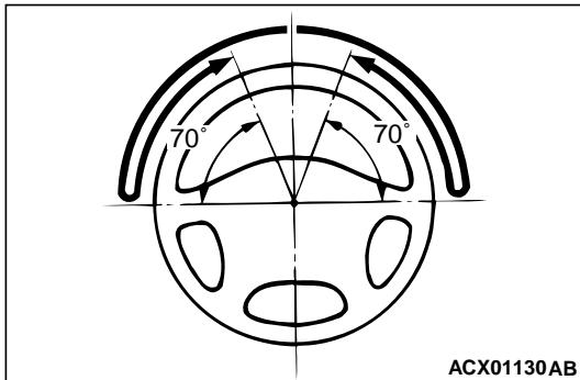
2. At a vehicle speed of approximately 35 km/h, turn the steering wheel 90°, hold a few seconds, then release. If the steering wheel then returns 70° or more, the return can be judged satisfactory.
