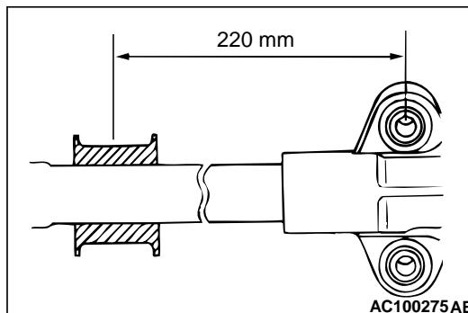
Install the gear mounting rubber to the rack housing so that the distance is as shown in the illustration.
