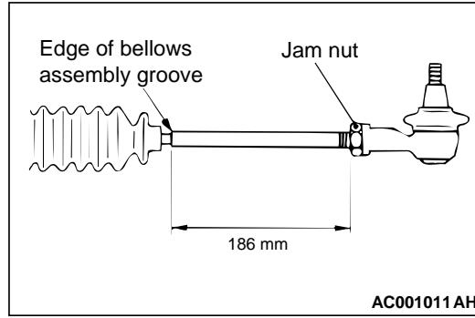
Screw in the tie rod end to achieve the right and left length as illustrated. Lock with the jam nut.
