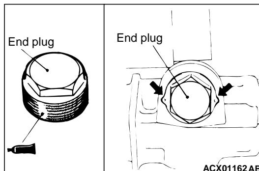
1. Apply specified sealant to the threaded part of the end plug.
