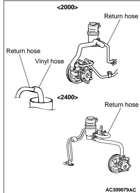
2. Disconnect the return hose connection, and then connect a vinyl hose to the return hose, and drain the fluid into a container.
