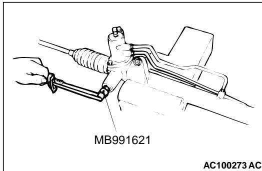
3. Use special tool rack support cover wrench (MB991621) to tighten the rack support cover to  $23 \pm 2 \text{ N}\cdot\text{m}$ .
