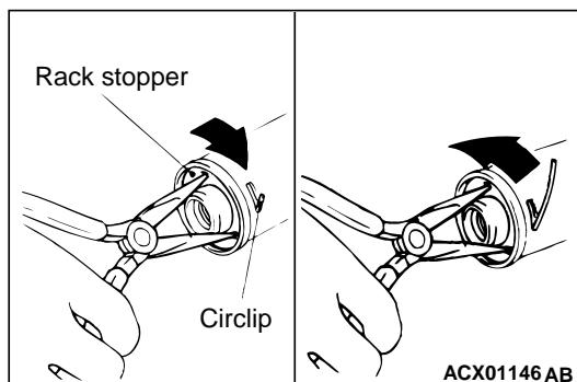
1. Turn the rack stopper clockwise until the end of the circlip comes out of the slot in the rack housing.
