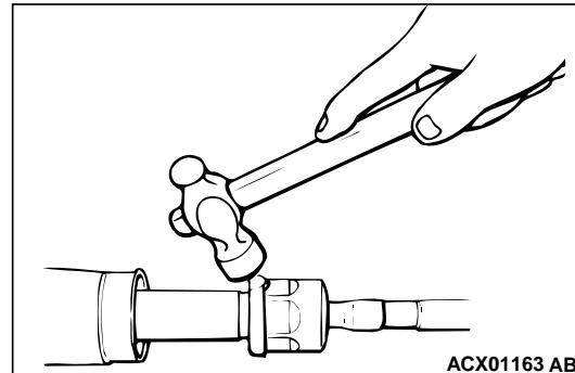
After installing the tie rod to the rack, fold tab washer end (two locations) to tie rod notch.
