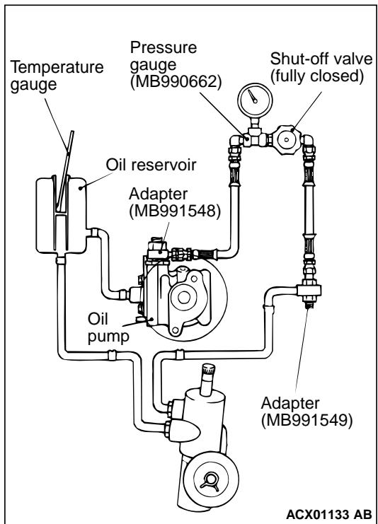
1. Disconnect the pressure hose from the oil pump, and then connect the following special tools.
