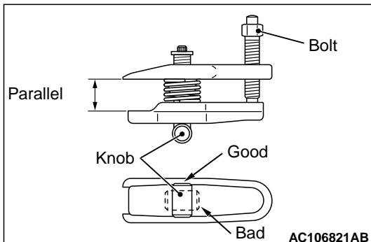
2. Turn the bolt and knob as necessary to make the jaws of the special tool parallel, tighten the bolt by hand and confirm that the jaws are still parallel.
