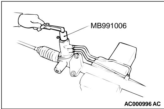
Using special tool preload socket (MB991006), rotate the pinion gear at the rate of one rotation in approximately 4 to 6 seconds to check the total pinion torque.
