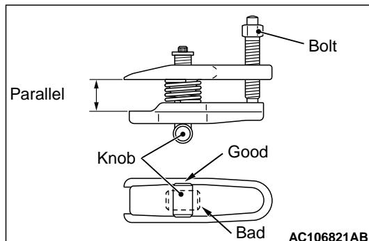
2. Turn the bolt and knob as necessary to make the jaws of special tool parallel, tighten the bolt by hand and confirm that the jaws are still parallel.
