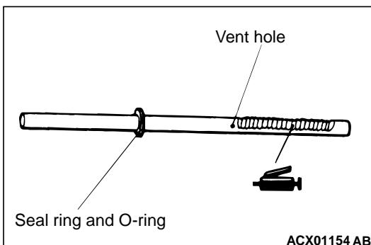
1. Apply a coating of repair kit grease to the rack teeth face.
