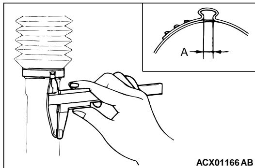
3. Check that crimped width (A) is within the standard value.
