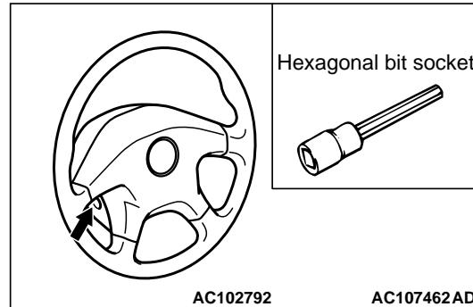
2. Loosen the bolt completely. Then, remove the steering wheel and air bag module assembly.
