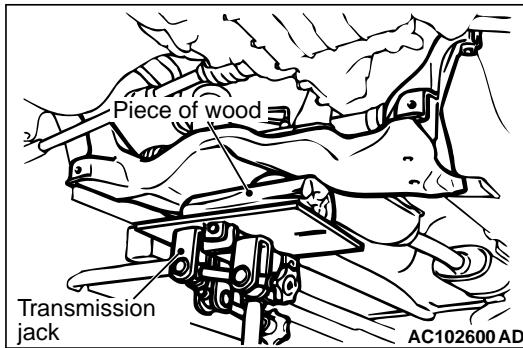
1. Use a transmission jack to hold the crossmember, and then remove the crossmember mounting nuts and bolts.
