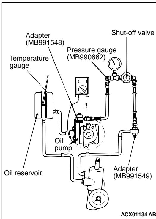
2. Bleed air, and then turn the steering wheel several times while the vehicle is not moving so that the temperature of the fluid rises to approximately 50 – 60°C.
