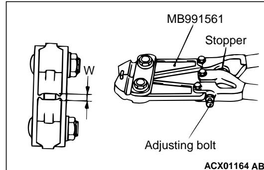
1. Turn the adjusting bolt of special tool boot band crimping tool (MB991561) to adjust the opening dimension (W) to the standard value.
