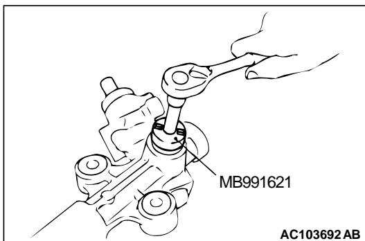
Using special tool rack support cover wrench (MB991621), remove the rack support cover from the steering gear.
