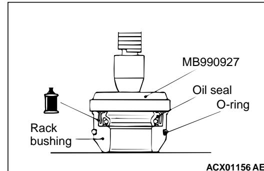
1. Apply ATF DEXRON III or DEXRON II to the outer surface of the oil seal. Using the special tool installer adapter (MB990927), press in the oil seal until it is flush with the bushing end face.
