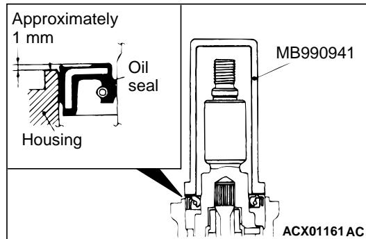
To eliminate a seal malfunction at the valve housing alignment surface, the upper surface of the oil seal should project outward approximately 1 mm from the housing edge surface.
