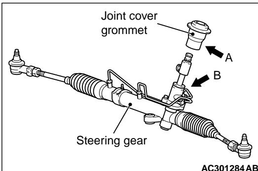
Align the joint cover grommet notch (arrow A) with the steering gear lug (arrow B), and then install the steering joint cover to the steering gear.
