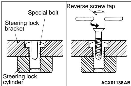
1. Drill in the special bolt a hole deep enough for the tap to stand.
