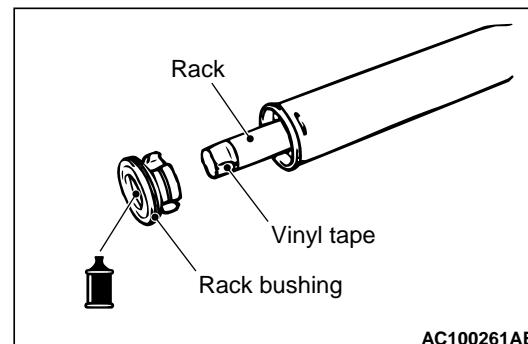
2. Apply ATF DEXRON III or DEXRON II to the oil seal inner surface and the O-ring.
