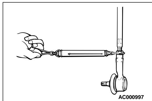
2. Measure the tie rod swing resistance [tie rod swing torque] with a spring balance.
