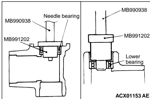
2. Press fit needle bearing with the following special tools.
