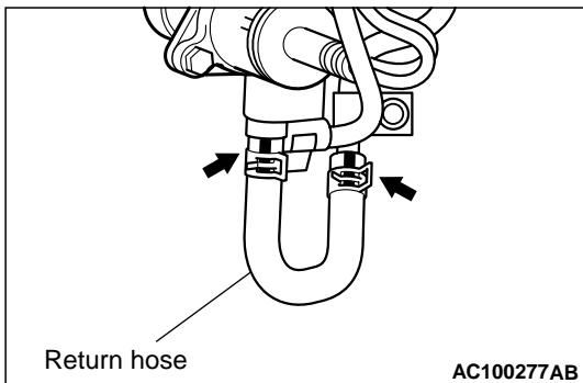
Install the return hose so that the marking is positioned as shown in the illustration.
