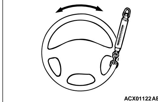
3. Attach a spring balance to the outer circumference of the steering wheel and measure the steering force required to turn the steering wheel from the straight ahead position to the left and right (within a range of 1.5 turns). Also check to be sure that there is no significant change in the required steering effort.
