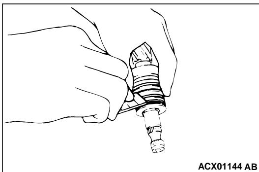
Cut the seal ring and remove it from the pinion and valve assembly or the rack.
