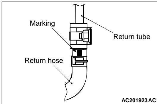
Install the return hose so that the markings are positioned as shown in the illustration.
