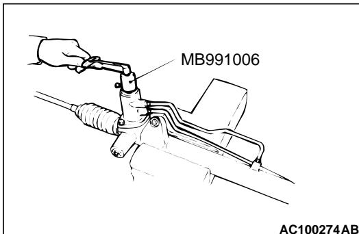
1. Using special tool preload socket (MB991006), rotate the pinion shaft at the rate of one rotation in four to six seconds to check the total pinion torque and the change in torque.
