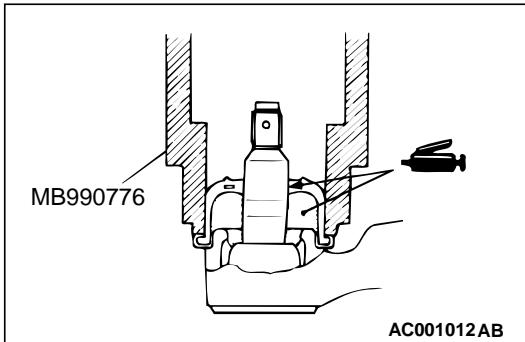
1. Apply specified grease to the lip and inside of the dust cover.
