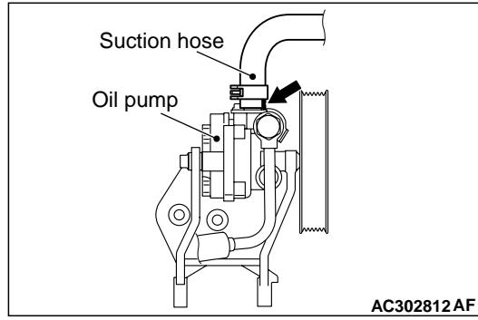
Install the suction hose so that the marking is positioned as shown in the illustration.
