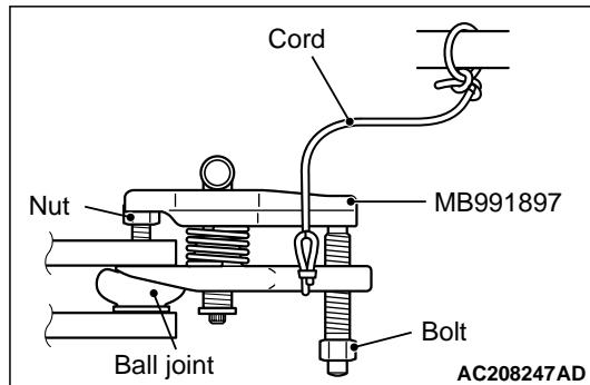
1. Install special tool ball joint remover (MB991897) as shown in the figure.
