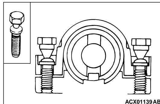
2. After checking that the lock works properly, tighten the special bolts until the head twists off.
