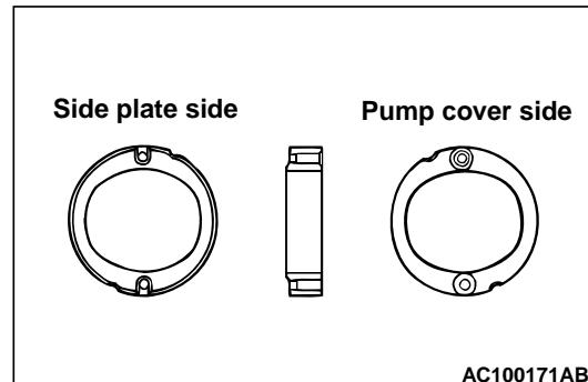
Install the cam ring as shown in the illustration.
