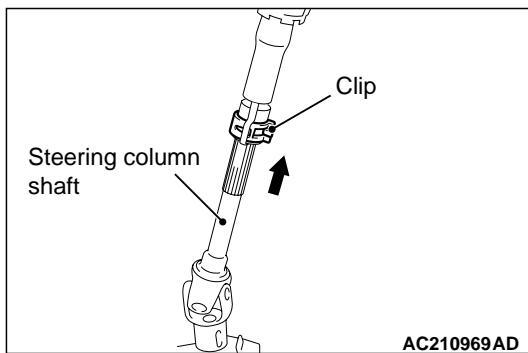
2. Pinch the steering column shaft clip with pliers, and pull up the shaft towards the direction shown to disengage the steering column shaft assembly.
