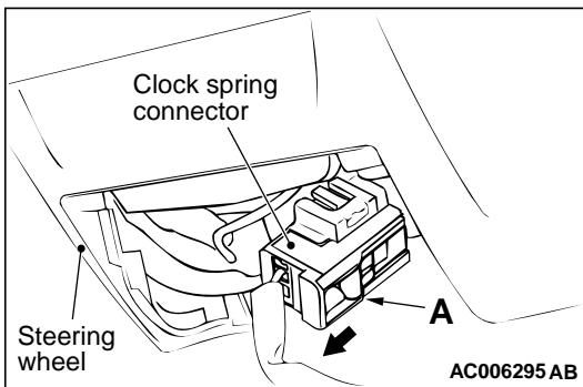
1. By sliding section A of the clock spring connector shown in the illustration in the arrow direction, disconnect the connector.
