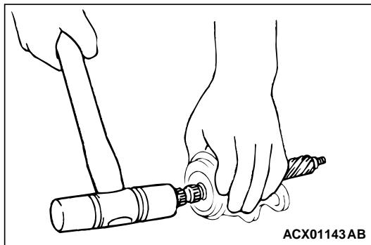
Using a plastic hammer, gently tap the pinion to remove it.
