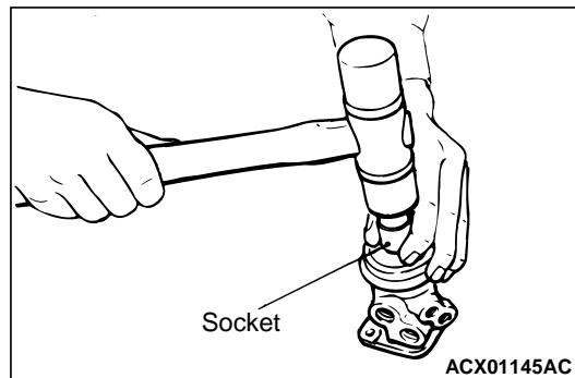
Using a socket, remove the oil seal and the ball bearing from the valve housing simultaneously.
