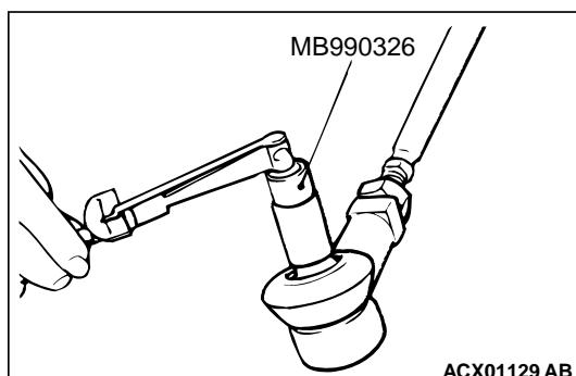
4. Move the ball joint stud several times and install the nut on the stud. Using special tool preload socket (MB990326), measure the ball joint starting torque.
