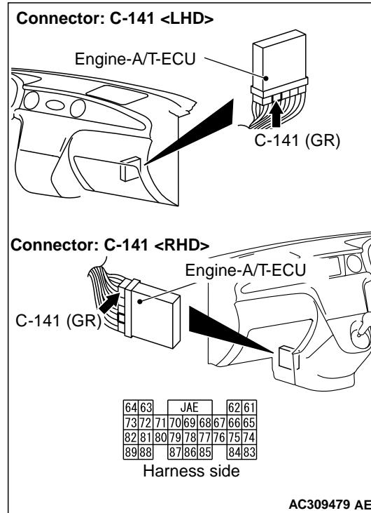
(3) Measure the voltage between engine-A/T-ECU connector C-141 terminal No.64 and earth.
