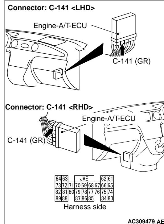
Check the output line for open circuit.
