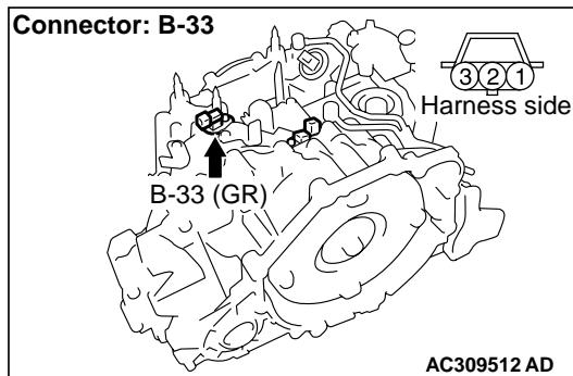
Disconnect the connector, and measure the resistance between terminal 1 and earth at the wiring harness side.
