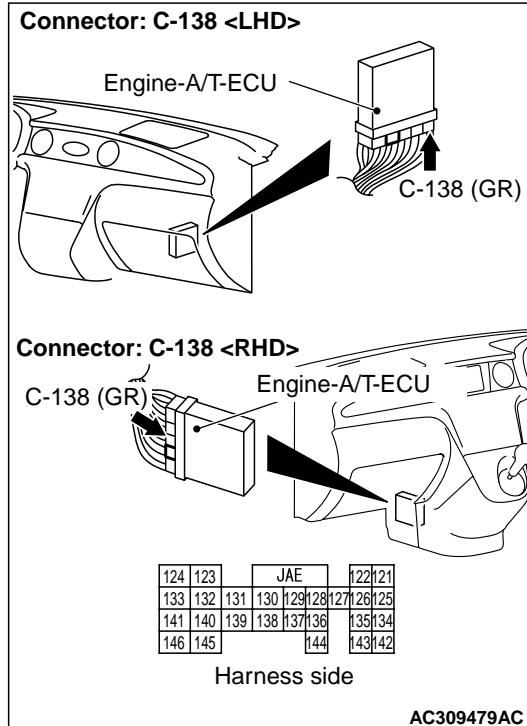
Check the power supply line for short or open circuit.
