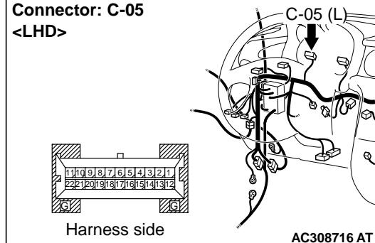
Check the output line for short circuit.
