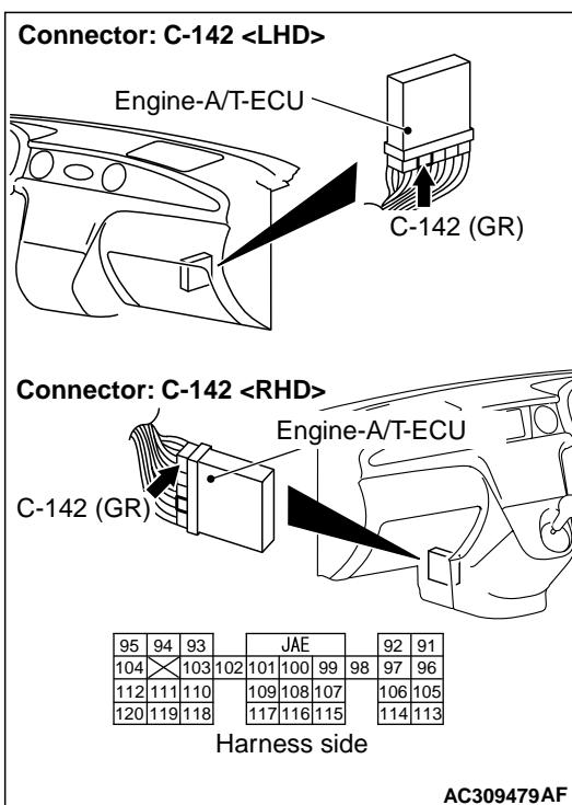
(3) Measure the voltage between engine-A/T-ECU connector C-142 terminal No.96 and earth.
