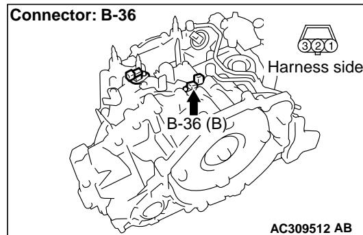
Disconnect the connector, and measure the resistance between terminal 1 and earth at the wiring harness side.
