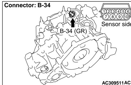
Disconnect the connector, and measure the resistance between terminal No.5 and No.9 at the solenoid valve side.
