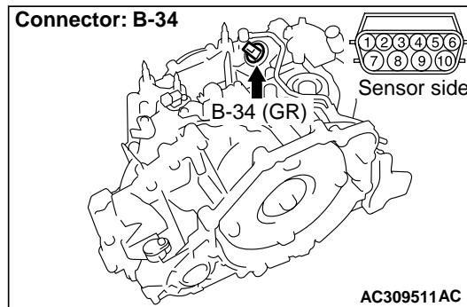
(1) Disconnect the connector, and measure the voltage between terminal 1 and earth at the wiring harness side.
