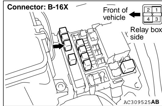
(2) Disconnect the A/T control relay, and measure the voltage between terminal No.3 and earth at the relay box side.
