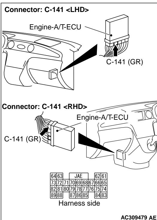
Check the output line for short-circuited or open circuit.
