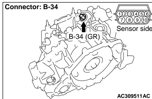
Disconnect the connector, and measure the resistance between terminal 1 and 2 at the sensor side.
