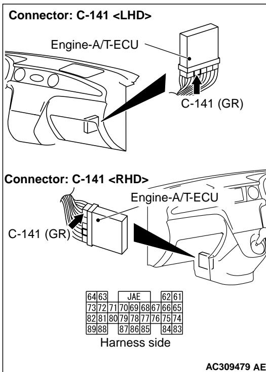
**STEP 21. Check the harness between shift switch assembly connector C-129 <RHD>, C-143 <LHD> terminal No.6 and engine-A/T-ECU connector C-141 terminal No.77.**
