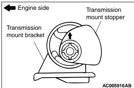
Install the transmission mount stopper so that the arrow mark points as shown in the illustration.
