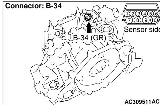
Disconnect the connector, and measure the resistance between terminal No.4 and No.9 at the solenoid valve side.
