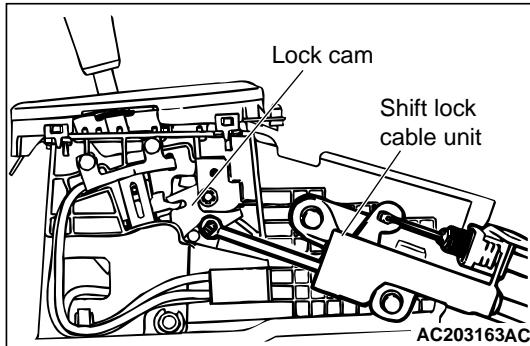
3. Install the shift lock cable unit rod to the selector lever assembly lock cam, and tighten the shift lock cable unit installation bolt to the specified torque.
