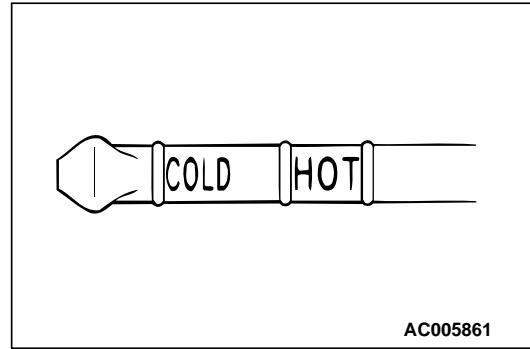
5. Check that the A/T fluid level is between the HOT marks on the oil level gauge. If the A/T fluid level is too low, add more A/T fluid until the level reaches between the HOT marks.
