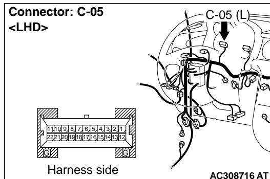
Disconnect the connector, and measure the resistance between terminal 12 and earth at the wiring harness side.
