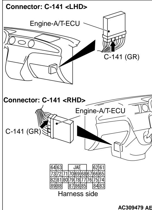
Check the output line for short circuit.
