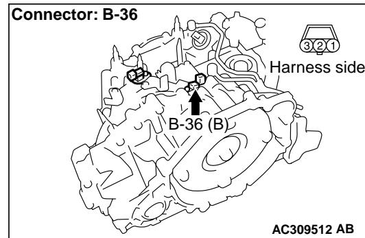
(1) Disconnect the connector, and measure the voltage between terminal 3 and earth at the wiring harness side.
