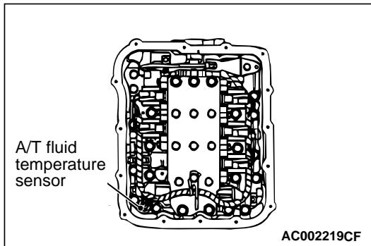
2. Remove the A/T fluid temperature sensor.
