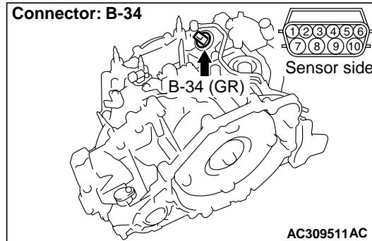
Disconnect the connector, and measure the resistance between terminal No.6 and No.10 at the solenoid valve side.
