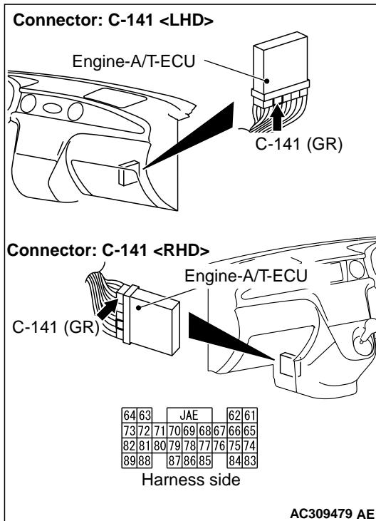
Check the output line for open circuit.
