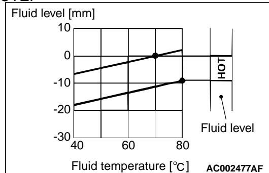
*Check the oil level referring to the characteristics chart shown at left if it takes some time until reaching the normal operation temperature of A/T fluid (70 – 80 °C.)*
