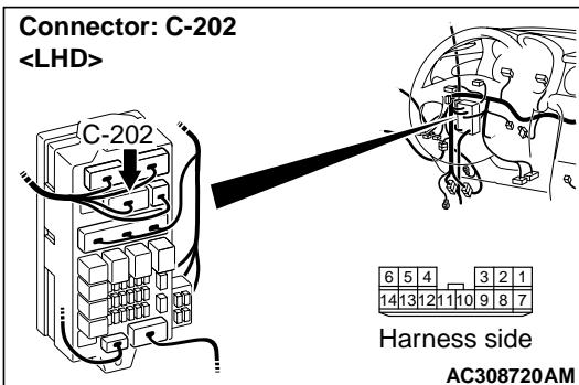
Check the power supply line for open circuit.
