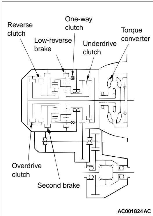
The purpose of this test is to measure the maximum engine speed when the torque converter stalls in D or R ranges in order to check the torque converter (Stator and one-way clutch operation) and the holding performance of the clutches and brakes which are built into the transmission.
