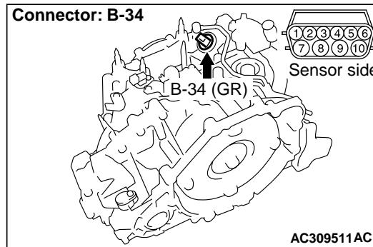
Disconnect the connector, and measure the resistance between terminal No.3 and No.9 at the solenoid valve side.
