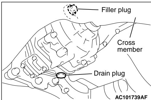
1. Remove the drain plug and discharge the oil.
