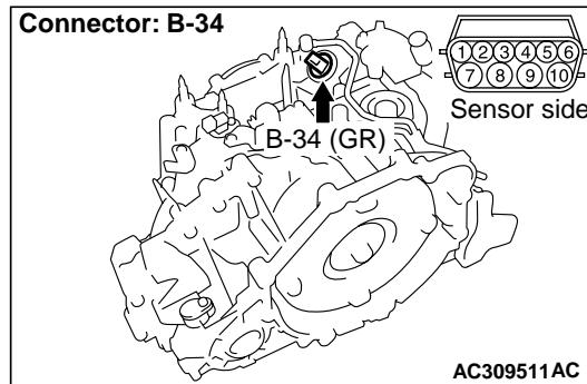
Disconnect the connector, and measure the resistance between terminal No.6 and No.10 at the solenoid valve side.
