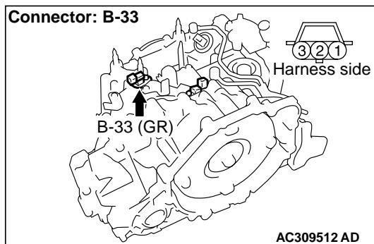
(1) Disconnect the connector, and measure the
