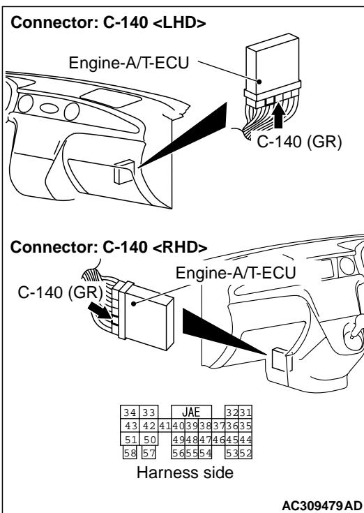
Check the output line for short or open circuit.
