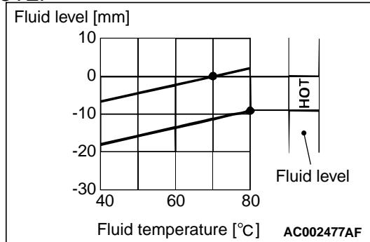
Check the oil level referring to the characteristics chart shown at left if it takes some time to reach the normal operation temperature of A/T fluid (70 – 80 °C).
