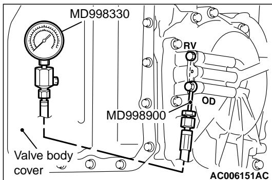
3. Connect the special tools (oil pressure gauge (3.0 MPa) [MD998330] and adapters [MD998332, MD998900]) to each pressure discharge port.
