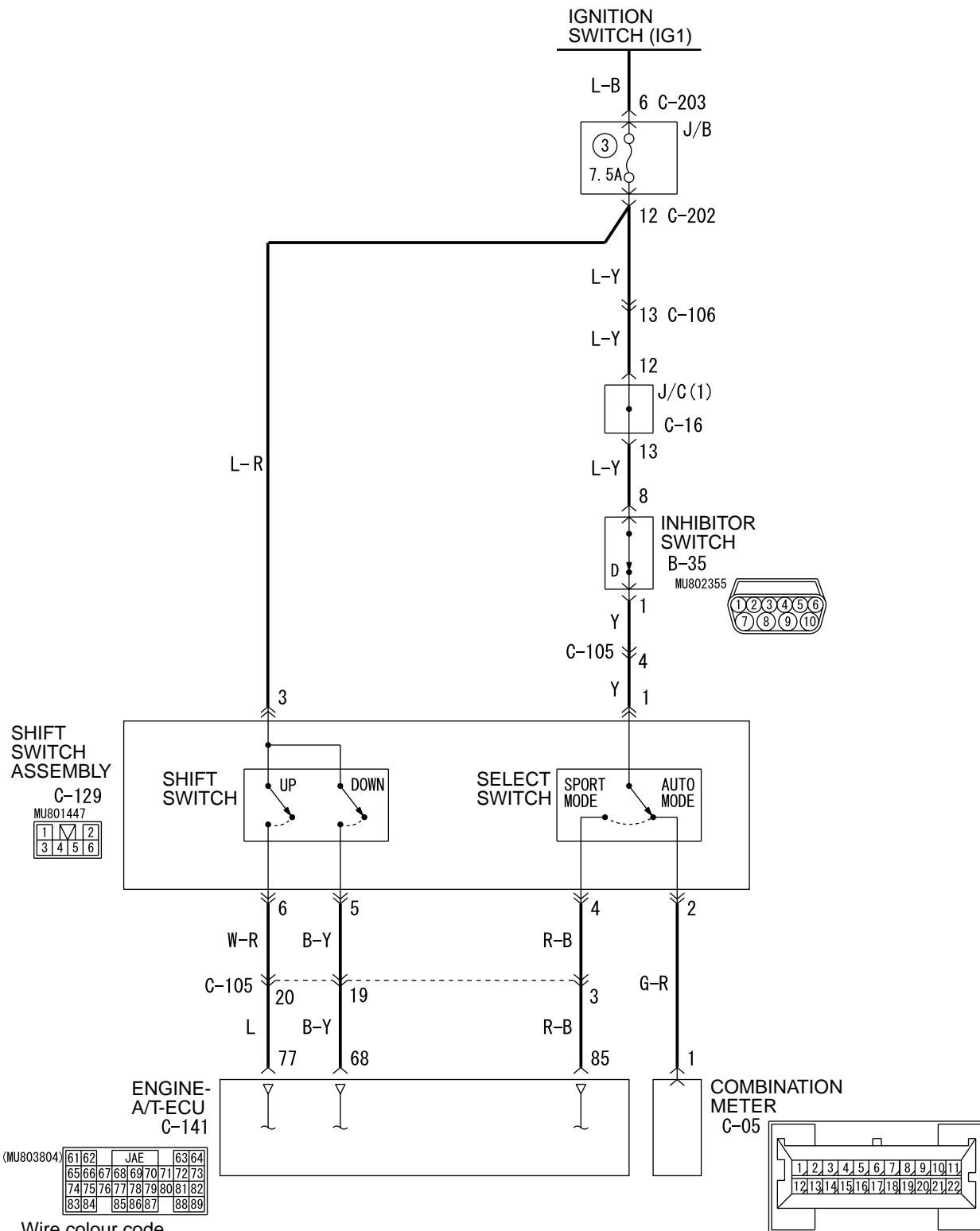
**Shift switch system circuit <LHD>**
