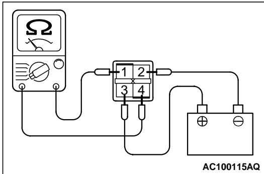
2. Use the jumper leads to connect A/T control relay terminal 2 to the negative battery terminal and terminal 3 to the positive battery terminal.
