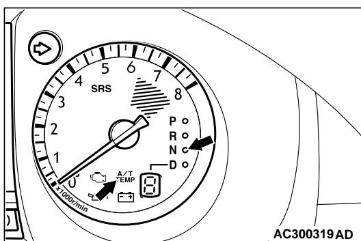
If there is a problem with any of the A/T system, the N range lamp will flash at a rate of approximately 1Hz.
