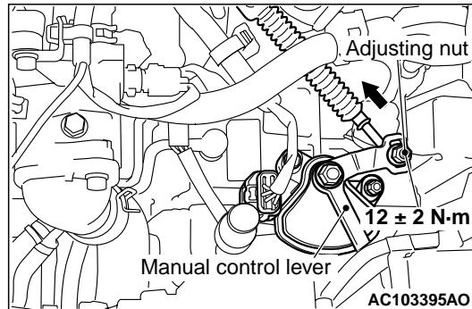
2. Place the cable stud into the manual control lever slot and install the nut loosely. Gently push the transmission control cable into the manual control lever slot until the cable is taut. Tighten the nut to the specified torque.
