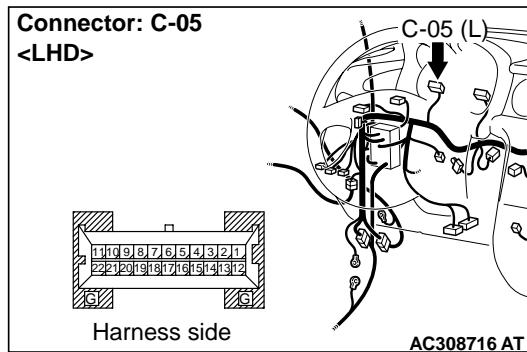
(1) Disconnect the connector, and measure the voltage between terminal 2 and earth at the wiring harness side.
