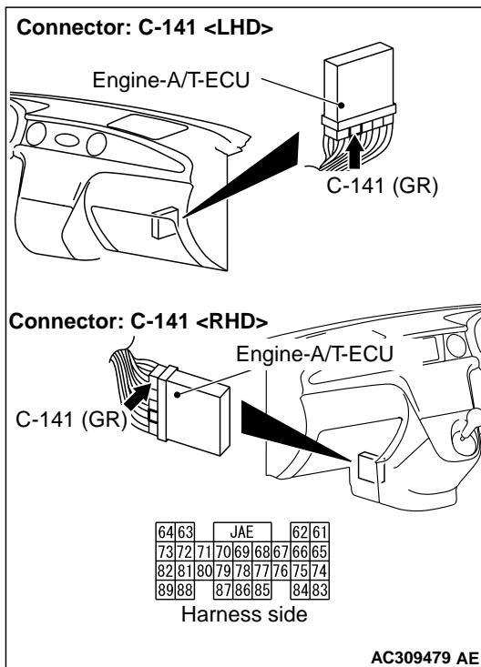
Check the output line for short circuit.
