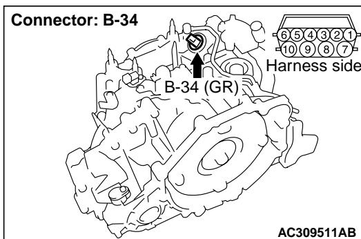
Disconnect the connector, and measure the resistance between terminal 2 and earth at the wiring harness side.
