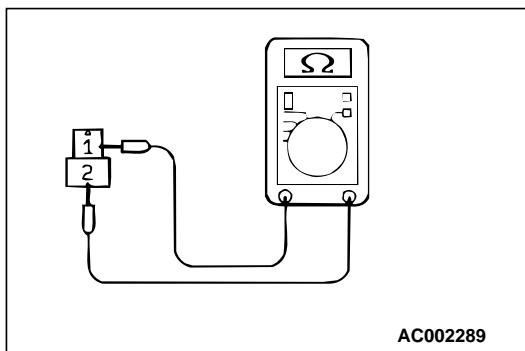
8. Measure the resistance between terminals 1 and 2 at each solenoid valve side.
