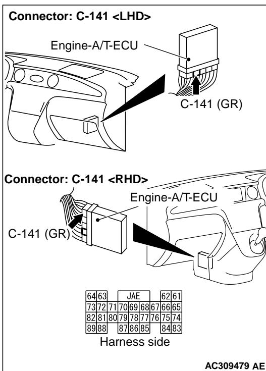
**STEP 24. Check the harness between shift switch assembly connector C-129 <RHD>, C-143 <LHD> terminal No.5 and engine-A/T-ECU connector C-141 terminal No.68.**
