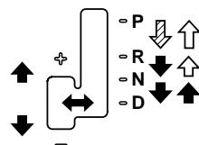
↗: Operation when the ignition switch is turned to a position other than LOCK (OFF), the brake pedal is depressed and the pushbutton is kept pressed.
