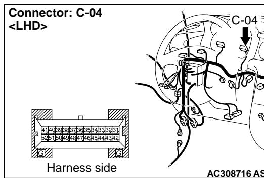
(2) Confirm the shift range by using the Actuator test on the MUT-II/III, and measure the voltage at the combination meter harness-side connector terminals.
