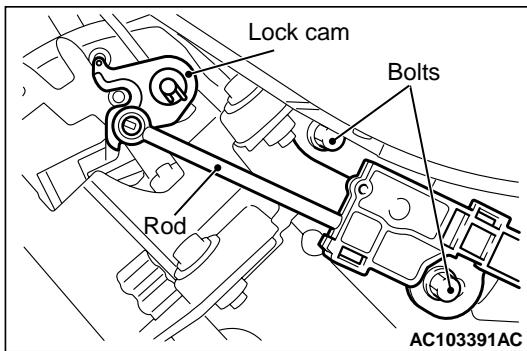
2. After installing the rod of the shift lock cable unit to the lock cam of the selector lever assembly, tighten the bolts of the shift lock cable unit to the specified torque.
