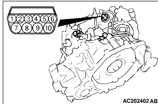
2. Disconnect the A/T control solenoid valve assembly connector.
