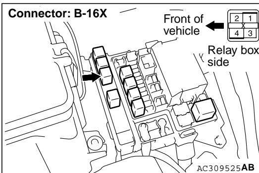
Disconnect the A/T control relay, and measure the voltage between terminal No.4 and earth at the relay box side.
