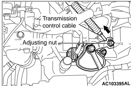
6. Gently push the transmission control cable in the direction as shown in the illustration at left, and tighten the adjusting nut the specified torque.
