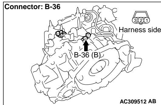
(1) Disconnect the connector, and measure the voltage between terminal 2 and earth at the wiring harness side.
