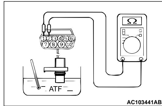
3. Measure the resistance between A/T control solenoid valve assembly connector terminals 1 and 2.
