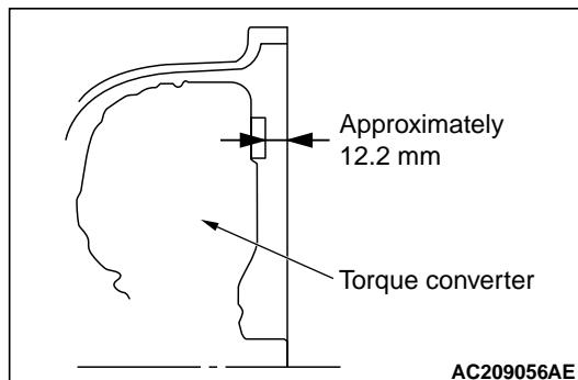
Engage the torque converter into the transmission side securely, and then assemble the transmission assembly on the engine.
