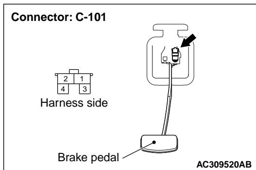
Check the power supply line for short or open circuit.
