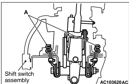
If the collision energy absorbing mechanism has already operated and the part A in the illustration is deformed, replace the selector lever assembly.
