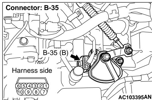
Check the output line for short-circuited or open circuit.
