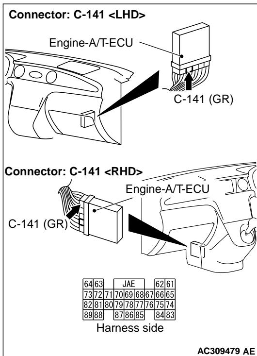
Check the output line for open circuit.
