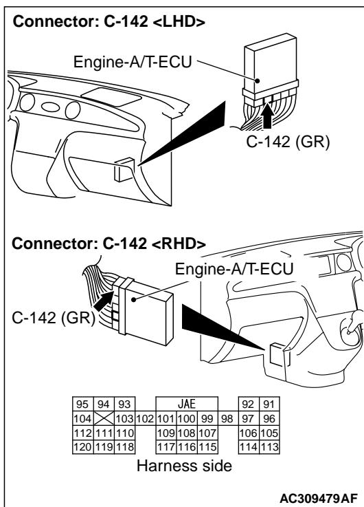
**STEP 13. Check the harness between A/T control solenoid valve assembly connector B-34 terminal No.1 and engine-A/T-ECU connector C-142 terminal No.119.**
