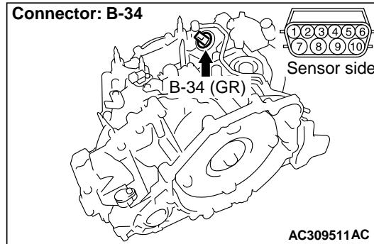
Disconnect the connector, and measure the resistance between terminal No.5 and No.9 at the solenoid valve side.
