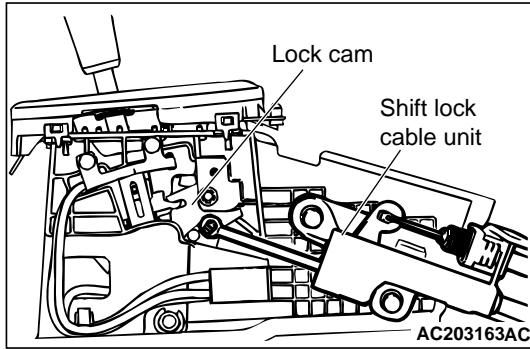
3. Install the shift lock cable unit rod to the selector lever assembly lock cam, and tighten the shift lock cable unit installation bolt to the specified torque.
