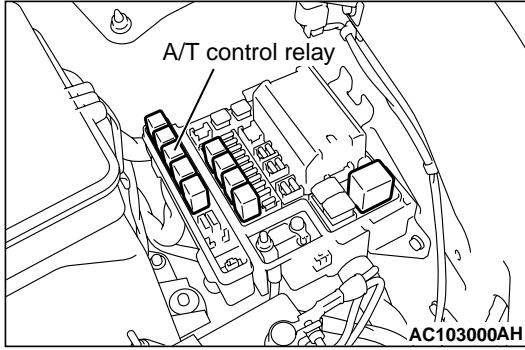
1. Remove the A/T control relay.
