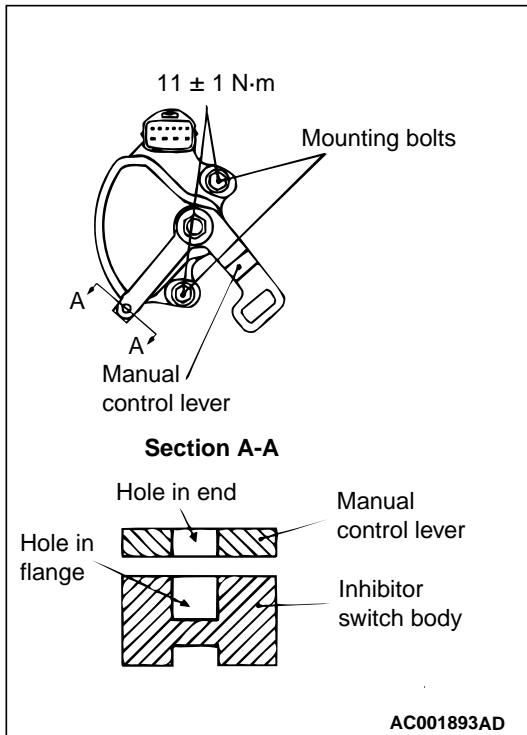
4. Loosen the inhibitor switch body mounting bolt, and then turn the inhibitor switch to adjust so that the hole at the end of the manual control lever and the hole in the inhibitor switch body flange (section A – A in the illustration at left) are aligned.
