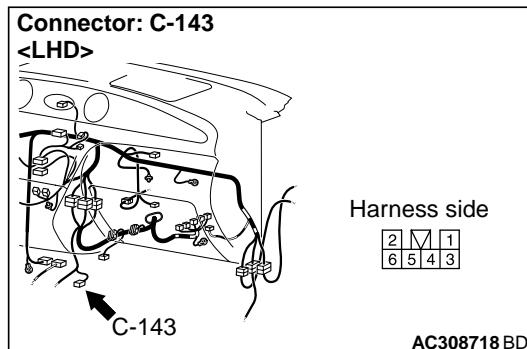
Check the output line for short circuit.
