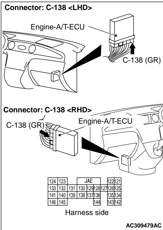
(3) Measure the voltage between engine-A/T-ECU connector C-138 terminal No.137 and earth.
