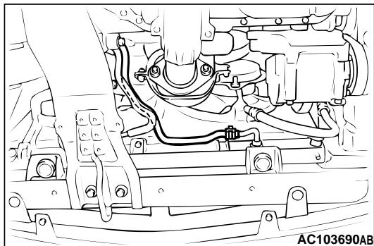
1. Remove the hose shown in the illustration which allows the A/T fluid to flow from the A/T fluid cooler (built into the radiator) to the transmission.
