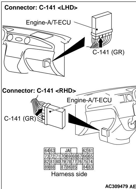
Check the earth line for open circuit.
