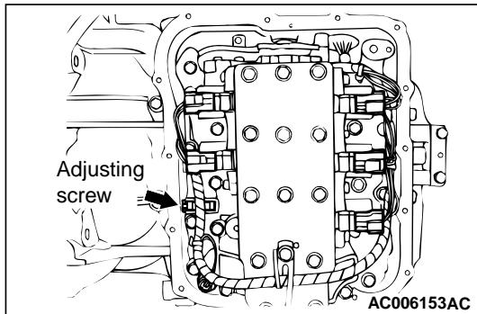
3. Turn the adjusting screw shown in the illustration to adjust the line pressure to the standard value. The pressure increases when the screw is turned counterclockwise.
