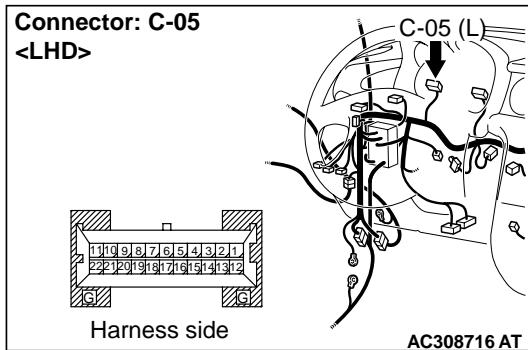
Check the earth line for open circuit or short-circuit.
