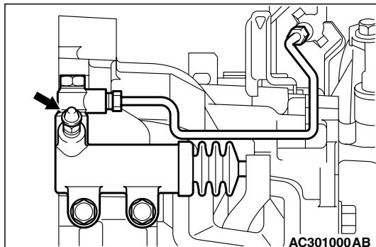
2. Connect a hose with a bottle to the bleeder screw.
