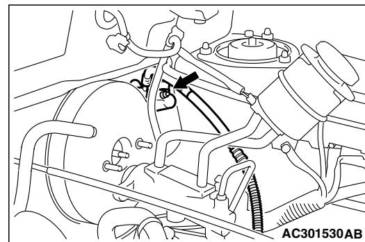
3. Connect a hose with a bottle to the bleeder screw.
