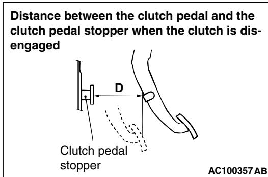
4. After completing the adjustments, confirm that the clutch pedal free play (measured at the face of the pedal pad) and the distance between the clutch pedal (the face of the pedal pad) and the clutch pedal stopper when the clutch is disengaged are within the standard value ranges.
