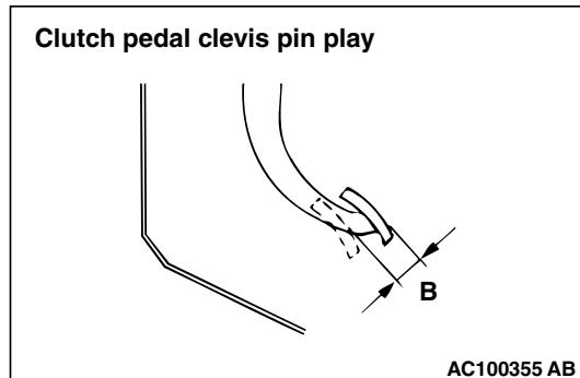
2. Measure the clutch pedal clevis pin play.
