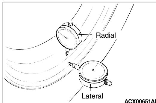
Jack up the vehicle so that the wheels are clear of the floor. While slowly turning the wheel, measure wheel runout with a dial indicator.
