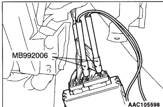
**Making an inspection with the connector attached (so the electrical circuit is complete)**
