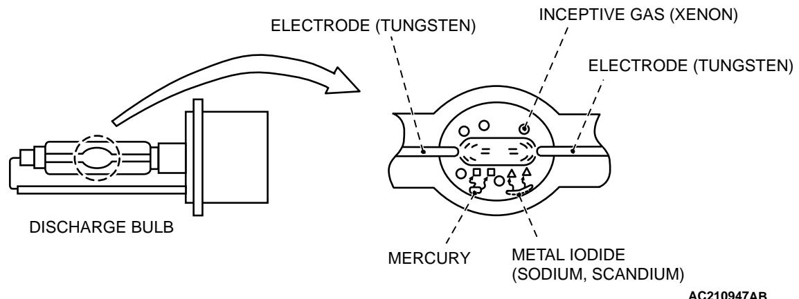
The HID headlight consists of the discharge bulb and controller that changes battery power supply into high-voltage AC.
