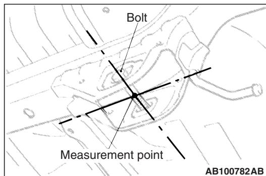
6. When measuring the suspension mounting arm, or link mounting position, use the suspension mounting bolt, etc. (Type B only)
