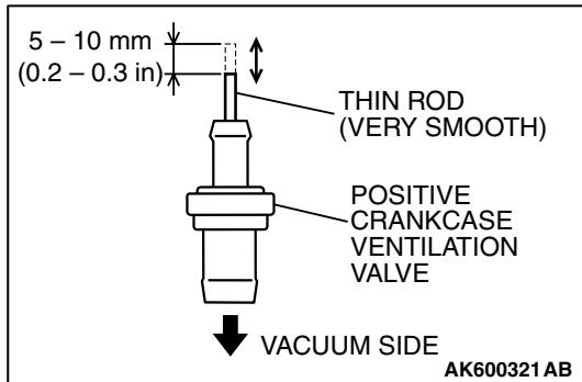
1. Hold the positive crankcase ventilation (PCV) valve with the vacuum side down. Insert a thin rod, and using light pressure, depress the end of the PCV valve spring by 5 – 10 mm (0.2 – 0.3 inch). Release pressure on the rod to see if the PCV valve spring will lift the rod to its original position.
