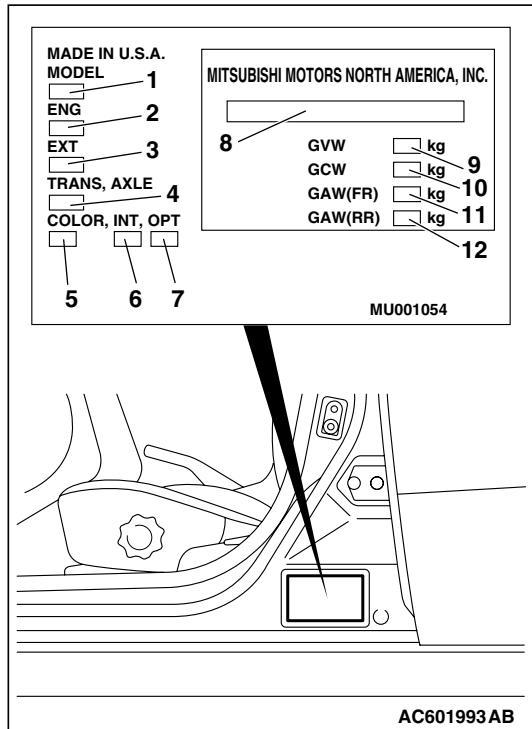
The vehicle information code plate is riveted to the face of the driver's door sill.
