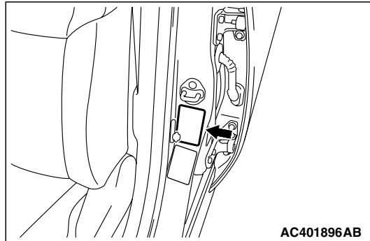
The tire and loading information placard is located on the inside sill of the driver's door.
