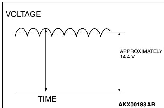
Rotation of the excited field coil generates AC voltage in the stator. This alternating current is rectified through diodes to DC voltage having a waveform shown in the illustration above. The average output voltage fluctuates slightly with the generator load condition.
