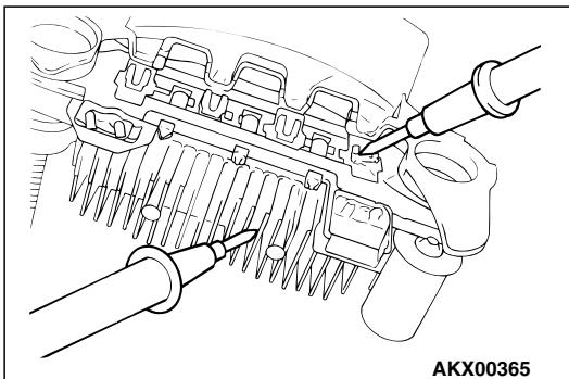
2. Check the continuity between the negative rectifier and the stator coil lead connection terminal with a tester. If there is continuity between the terminals, the diode is grounded, so replace the rectifier.
