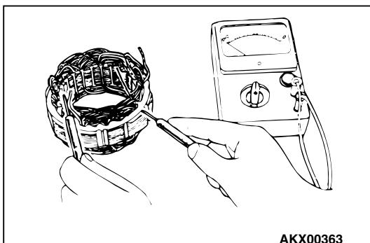
2. Check the continuity between the coil and the core. If there is continuity, replace the stator.
