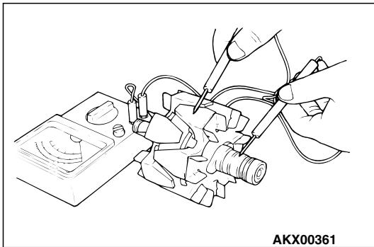
2. Check the continuity between the slip ring and the core. If there is continuity, replace the rotor.
