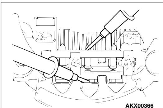
3. Check the continuity of the three diodes by connecting an ohmmeter to both ends of each diode. If there is continuity between the directions, or if there is no continuity, the diode is damaged, so replace the rectifier.
