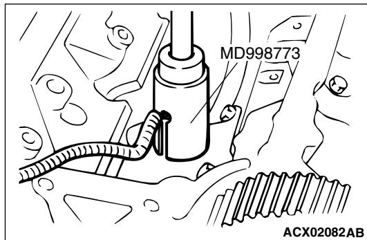
**INSTALLATION SERVICE POINTS****>>A<< KNOCK SENSOR INSTALLATION**
