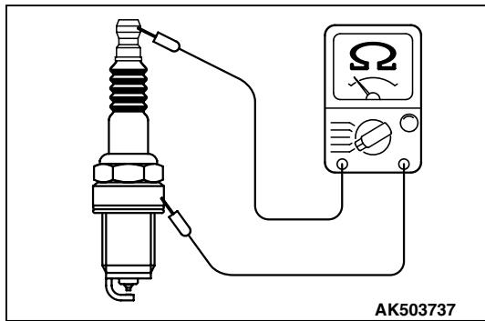
1. Measure the insulation resistance. If the insulation resistance of the spark plug is under the limited value, clean the plug within 20 seconds using a plug cleaner.
