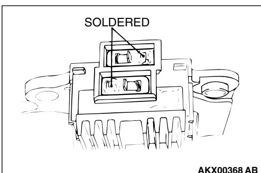
2. The brush can be removed by unsoldering the brush lead wire.
