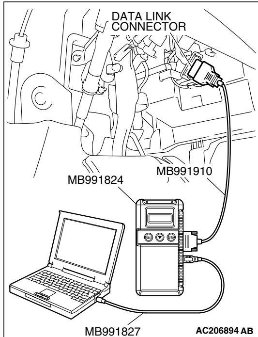
STEP 2. Using scan tool MB991958, check data list.
