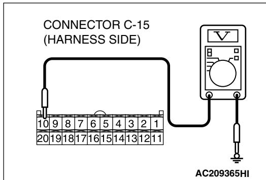
(4) Measure the voltage between A/C-ECU connector C-15 terminal No.10 and ground.
