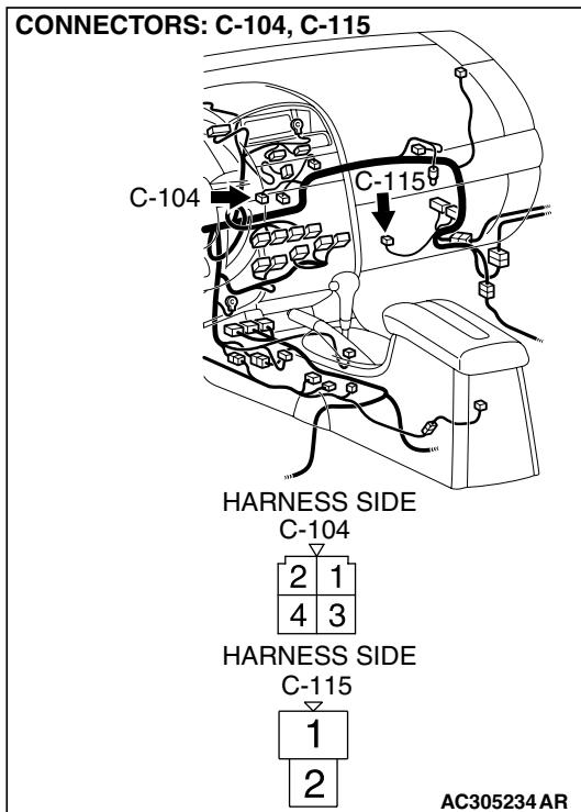
**STEP 5. Check the wiring harness between power transistor connector C-104 (terminal 4) and blower motor connector C-115 (terminal 2).**
