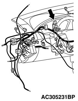
**NOTE:** Also check junction block connector C-211 and joint connector C-03 for loose, corroded, or damaged terminals, or terminals pushed back in the connector. If junction block connector C-211 and joint connector C-03 is damaged, repair or replace the connector as described in GROUP 00E, Harness Connector Inspection [P.00E-2](#).
