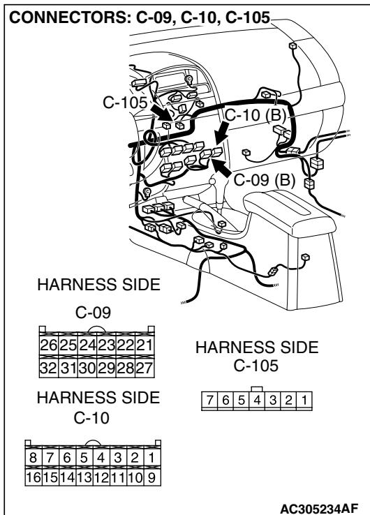
**STEP 5. Check the wiring harness between A/C-ECU connectors C-09 (terminal 32), C-10 (terminal 9) and air mixing damper control motor and potentiometer connector C-105 (terminals 2 and 1).**
