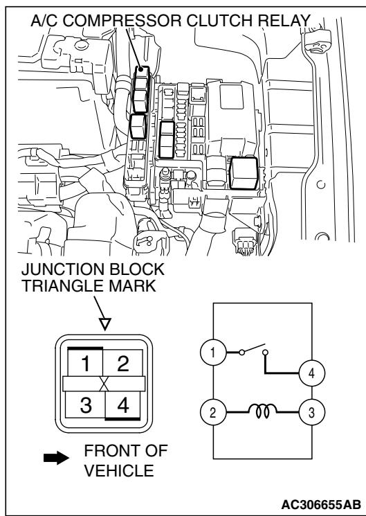
**STEP 6. Check the A/C compressor clutch relay continuity.**
