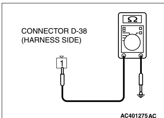
**STEP 14. Measure the resistance at defogger connector D-38.**
