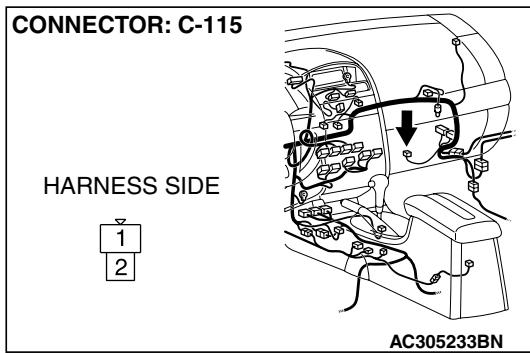
**STEP 13. Check the wiring harness between blower motor connector C-115 (terminal 1) and blower switch connector C-14 (terminal 5).**
