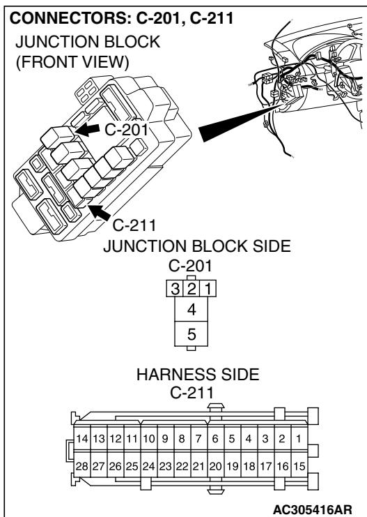
**STEP 12. Check the wiring harness between rear window defogger relay connector C-201 (terminal 4) and rear window defogger connector D-39 (terminal 1).**
