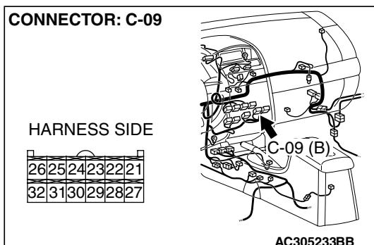
**STEP 15. Check A/C-ECU connector C-09 for loose, corroded or damaged terminals, or terminals pushed back in the connector.**
