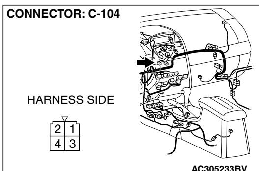
**STEP 14. Check the wiring harness between power transistor connector C-104 (terminal 2) and ground.**
