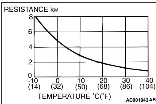
**STEP 20. Check the air thermo sensor.**
