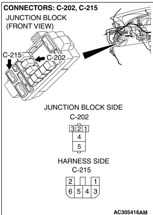
*NOTE: Also check junction block connector C-215 for loose, corroded, or damaged terminals, or terminals pushed back in the connector. If junction block connector C-215 is damaged, repair or replace the connector as described in GROUP 00E, Harness Connector Inspection [P.00E-2](#).*
