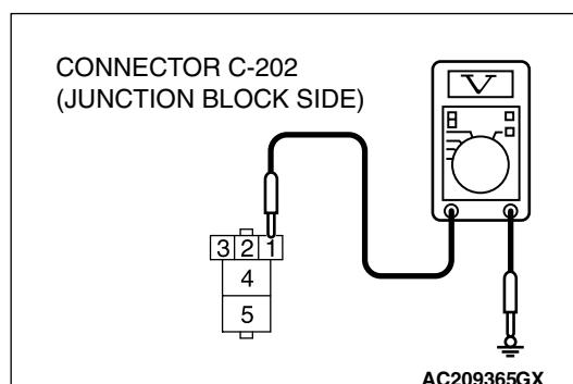
**STEP 5. Measure the voltage at blower relay connector C-202.**
