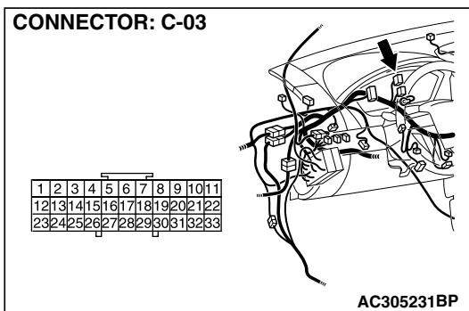
*NOTE: Also check joint connector C-03 for loose, corroded, or damaged terminals, or terminals pushed back in the connector. If joint connector C-03 is damaged, repair or replace the connector as described in GROUP 00E, Harness Connector Inspection [P.00E-2](#).*
