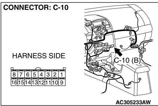
**STEP 2. Measure the voltage at A/C-ECU connector C-10.**
