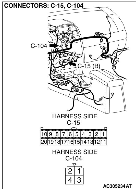
**STEP 7. Check the wiring harness between power transistor connector C-104 (terminals 1 and 3) and A/C-ECU connector C-15 (terminals 17 and 18).**
