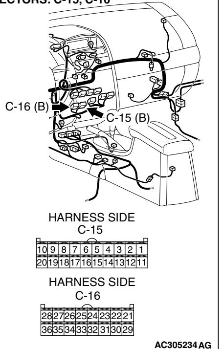
**STEP 6. Check the wiring harness between A/C-ECU connector C-15 (terminal 12), C-16 (terminals 34 and 26) and A/C pressure sensor connector A-30 (terminals 3, 1 and 2).**
