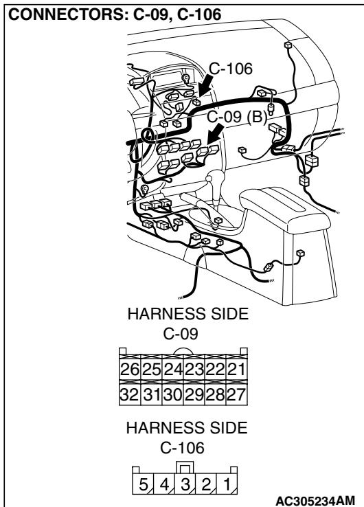
**STEP 7. Check the wiring harness between outside/inside air selection damper control motor connector C-106 (terminals 4 and 5) and A/C-ECU C-09 (terminals 28 and 29).**
