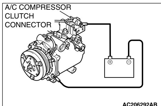
**STEP 19. Check the A/C compressor clutch operation.**
