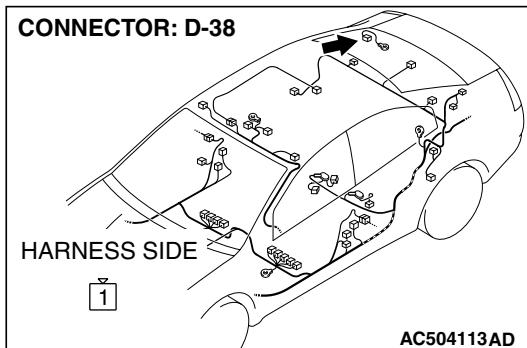
**STEP 13. Check defogger connector D-38 for loose, corroded or damaged terminals, or terminals pushed back in the connector.**
