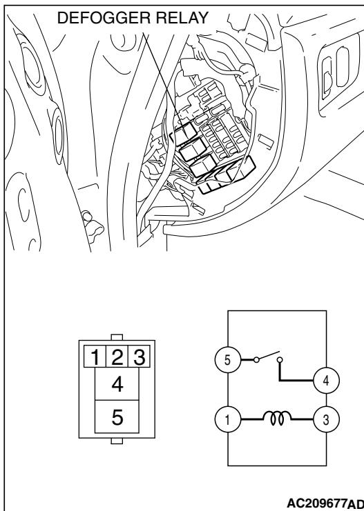
**STEP 3. Check the rear window defogger relay continuity.**
