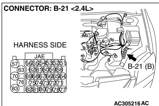
(2) Disconnect powertrain control module connector B-21 and ground harness side terminal No.81.
