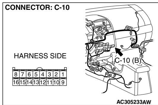
**STEP 9. Check the wiring harness between A/C-ECU connector C-10 (terminal 2) and the ground.**
