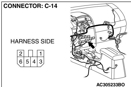
**STEP 5. Check blower switch connector C-14 for loose, corroded or damaged terminals, or terminals pushed back in the connector.**
