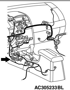
**NOTE:** Also check intermediate connectors A-13 and C-23 for loose, corroded, or damaged terminals, or terminals pushed back in the connector. If intermediate connector A-13 or C-23 is damaged, repair or replace the connector as described in GROUP 00E, Harness Connector Inspection [P.00E-2](#).
