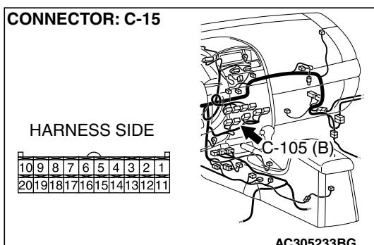
**STEP 15. Check A/C-ECU connector C-15 for loose, corroded or damaged terminals, or terminals pushed back in the connector.**
