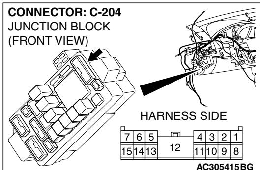
**STEP 17. Check the wiring harness between capacitor connector D-40 (terminal 1) and junction block connector C-204 (terminal 1).**
