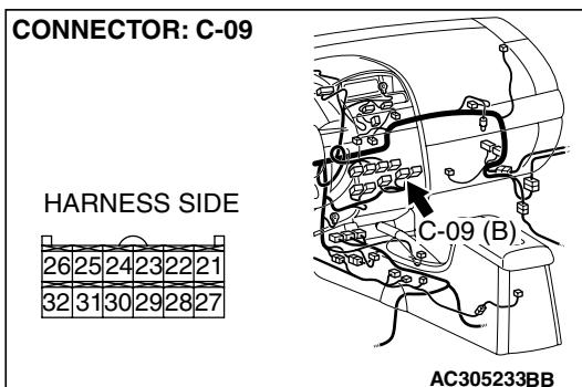
**STEP 16. Measure the voltage at A/C-ECU connector C-09.**
