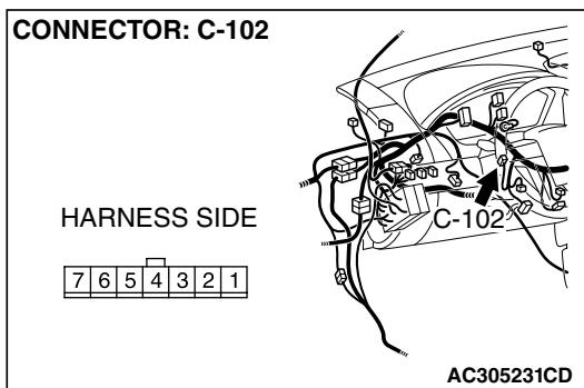
**STEP 5. Check the wiring harness between A/C-ECU connector C-09 (terminals 31 and 30) and mode selection damper control motor and potentiometer connector C-102 (terminals 1 and 2).**
