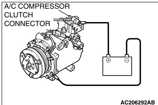
1. Disconnect the A/C compressor clutch connector to the A/C compressor clutch.
