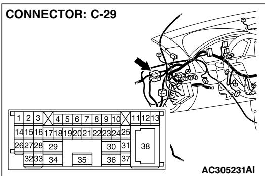
*NOTE: Also check intermediate connector C-29 for loose, corroded, or damaged terminals, or terminals pushed back in the connector. If intermediate connector C-29 is damaged, repair or replace the connector as described in GROUP 00E, Harness Connector Inspection [P.00E-2](#).*
