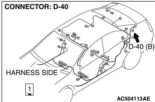
**STEP 16. Check capacitor connector D-40 for loose, corroded or damaged terminals, or terminals pushed back in the connector.**
