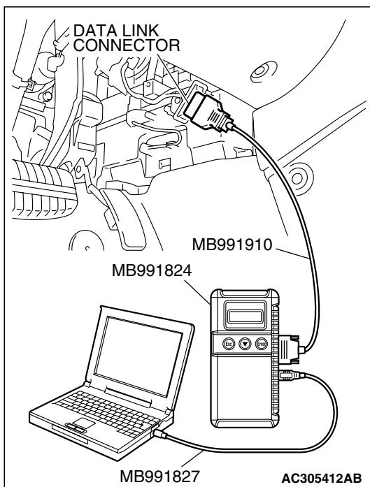
**STEP 3. Using scan tool MB991958, check for any diagnostic trouble code.**
