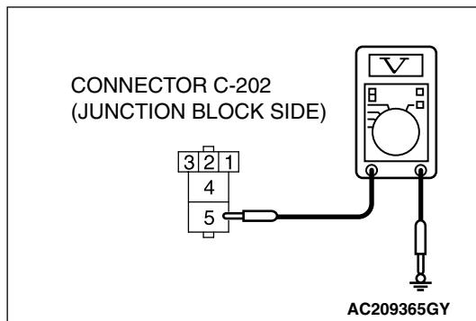
(2) Measure the voltage between terminal 5 and ground.
