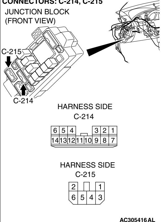
**NOTE:** Also check intermediate connector A-13, joint connector C-01, junction block connectors C-214 and C-215 for loose, corroded, or damaged terminals, or terminals pushed back in the connector. If intermediate connector A-13, joint connector C-01, junction block connector C-214 or C-215 is damaged, repair or replace the connector as described in GROUP 00E, Harness Connector Inspection [P.00E-2](#).
