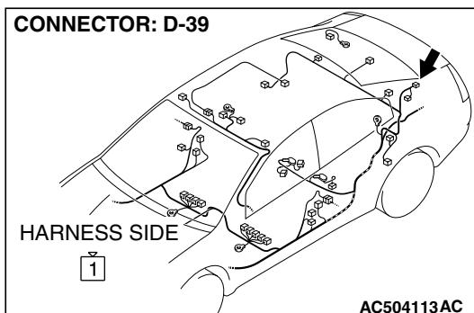
**STEP 4. Check rear window defogger connector D-39 for loose, corroded or damaged terminals, or terminals pushed back in the connector.**
