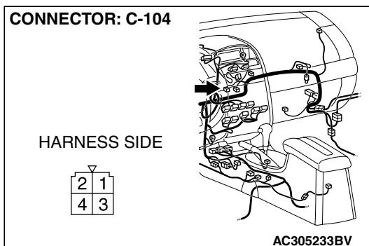
**STEP 12. Check blower power transistor connector C-104 for loose, corroded or damaged terminals, or terminals pushed back in the connector.**
