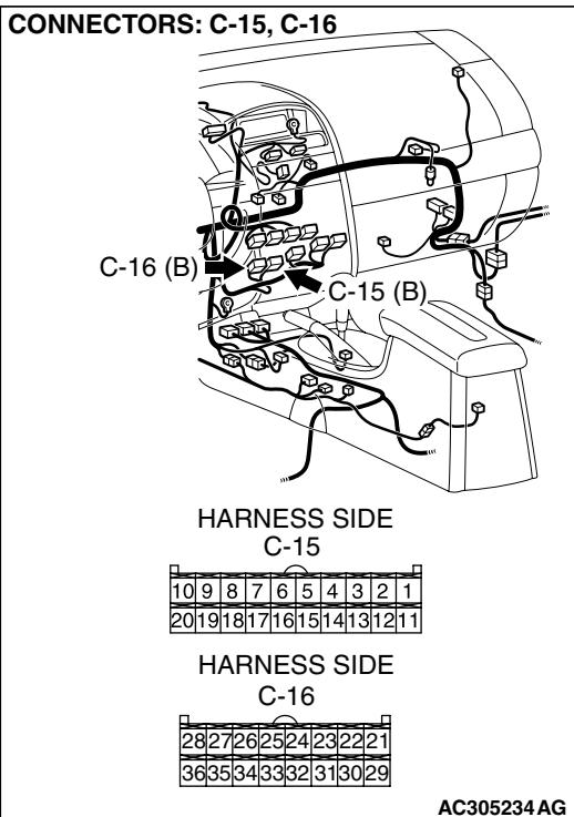
**STEP 6. Check A/C-ECU connectors C-15 and C-16 for loose, corroded or damaged terminals, or terminals pushed back in the connector.**
