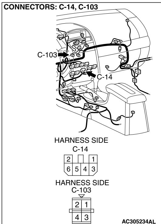
**STEP 7. Check the wiring harness blower switch connector C-14 (terminals 1, 6 and 2) and resistor connector C-103 (terminals 3, 1 and 4).****Q: Are the wiring harness between blower switch connector C-14 (terminals 1, 6 and 2) and resistor connector C-103 (terminals 3, 1 and 4) in good condition?**
