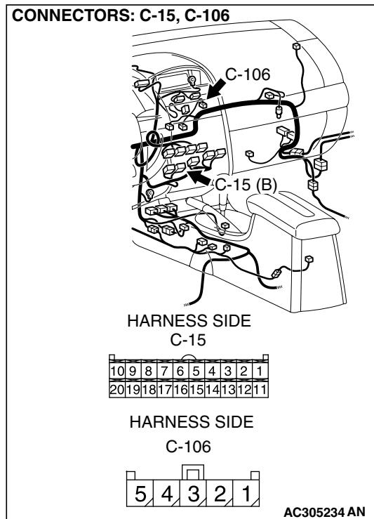
**STEP 7. Check the wiring harness between outside/inside air selection damper control motor connector C-106 (terminals 4 and 5) and A/C-ECU C-15 (terminals 5 and 6).**
