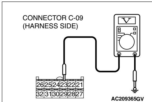
(4) Measure the voltage between A/C-ECU connector C-09 terminal No.23 and ground.
