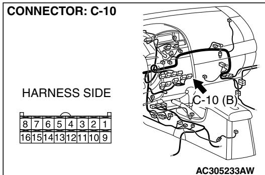
**STEP 5. Check A/C-ECU connector C-10 for loose, corroded or damaged terminals, or terminals pushed back in the connector.****Q: Is A/C-ECU connectors C-10 in good condition?**
