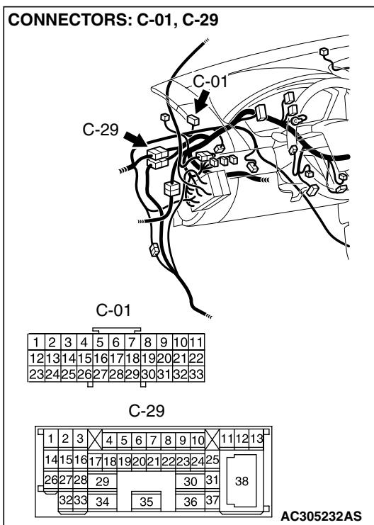
**NOTE:** Also check joint connector C-01 and intermediate connector C-29 for loose, corroded, or damaged terminals, or terminals pushed back in the connector. If joint connector C-01 or intermediate connector C-29 is damaged, repair or replace the connector as described in GROUP 00E, Harness Connector Inspection [P.00E-2](#).
