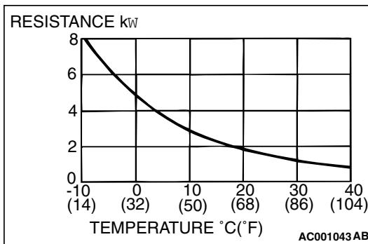
(2) Measure the resistance between connector terminals 1 and 2 under at least two different temperatures. The resistance values should generally match those in the graph.
