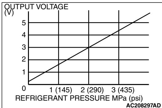
4. At this time, check to see that the voltage of A/C pressure sensor terminal No. 2 reflects the specifications of the figure.
