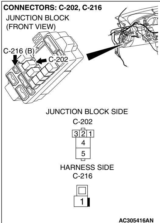
*NOTE: Also check intermediate connector C-29 and junction block connector C-216 for loose, corroded, or damaged terminals, or terminals pushed back in the connector. If intermediate connector C-29, junction block connector C-216 is damaged, repair or replace the connector as described in GROUP 00E, Harness Connector Inspection [P.00E-2](#).*
