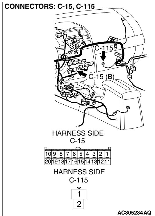
**STEP 1. Check blower motor connector C-115 and A/C-ECU connector C-15 for loose, corroded or damaged terminals, or terminals pushed back in the connector.**
