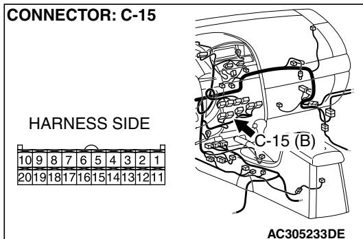
**STEP 10. Check A/C-ECU connector C-15 for loose, corroded or damaged terminals, or terminals pushed back in the connector.**
