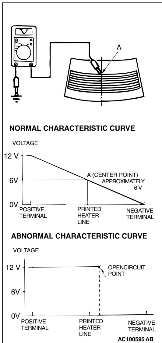
**STEP 18. Check the rear window defogger.**
