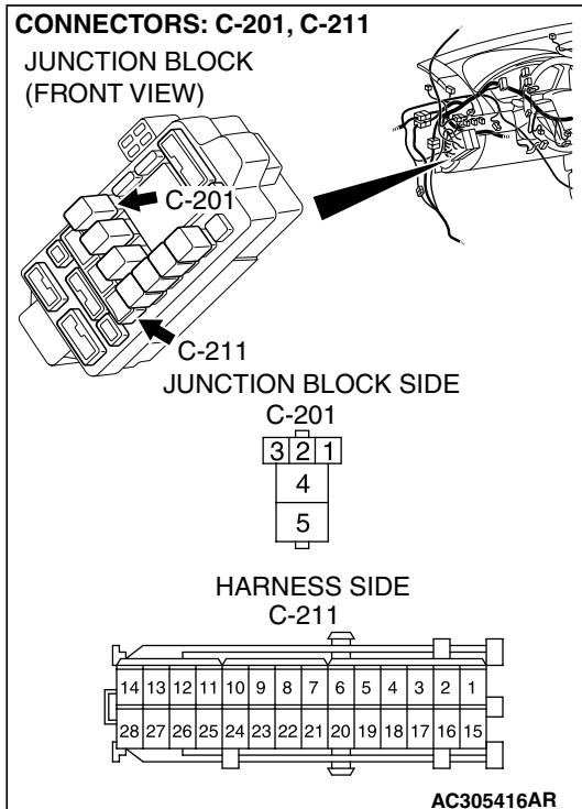
**NOTE:** Also check junction block connector C-211 for loose, corroded, or damaged terminals, or terminals pushed back in the connector. If junction block connector C-211 is damaged, repair or replace the connector as described in GROUP 00E, Harness Connector Inspection [P.00E-2](#).
