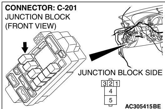
**STEP 2. Check rear window defogger relay connector C-201 for loose, corroded or damaged terminals, or terminals pushed back in the connector.**
