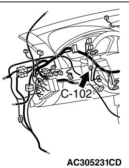
**STEP 5. Check the wiring harness between A/C-ECU connector C-15 (terminals 11 and 4) and mode selection damper control motor and potentiometer connector C-102 (terminals 1 and 2).**
