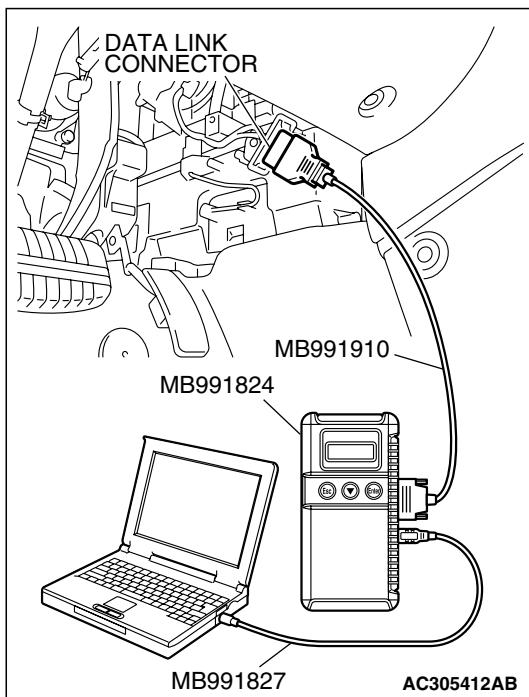
**STEP 2. Using scan tool MB991958, read the powertrain control module diagnostic trouble code.**
