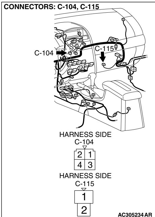
**STEP 15. Check the wiring harness between power transistor connector C-104 (terminal 4) and blower motor connector C-115 (terminal 2).**
