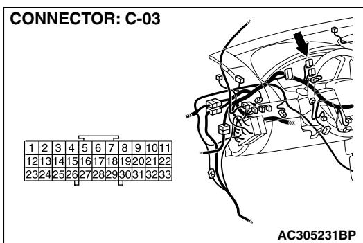
*NOTE: Also check intermediate connector C-23 and joint connector C-03 for loose, corroded, or damaged terminals, or terminals pushed back in the connector. If intermediate connector C-23 or joint connector C-03 is damaged, repair or replace the connector as described in GROUP 00E, Harness Connector Inspection [P.00E-2](#).*
