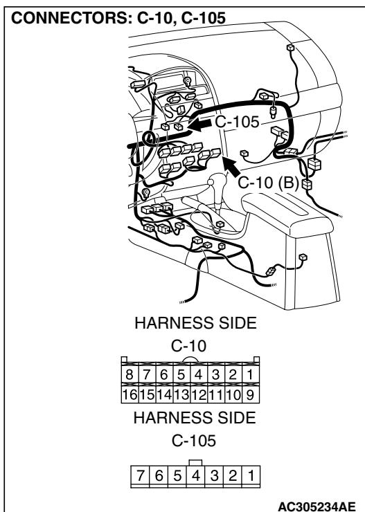
**STEP 5. Check the wiring harness between A/C-ECU connectors C-10 (terminals 15, 12 and 10) and air mixing damper control motor and potentiometer connector C-105 (terminals 5, 3 and 7).**
