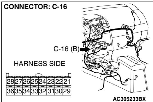
**STEP 2. Measure the voltage at A/C-ECU connector C-16.**
