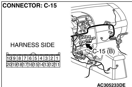
**STEP 11. Check the wiring harness between rear window defogger relay connector C-201 (terminal 3) and A/C-ECU connector C-15 (terminal 8).**
