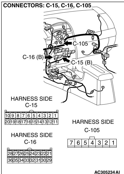
**STEP 5. Check the wiring harness between A/C-ECU connectors C-15 (terminals 16 and 20), C-16 (terminal 29) and air mixing damper control motor and potentiometer connector C-105 (terminals 5, 7 and 3).**
