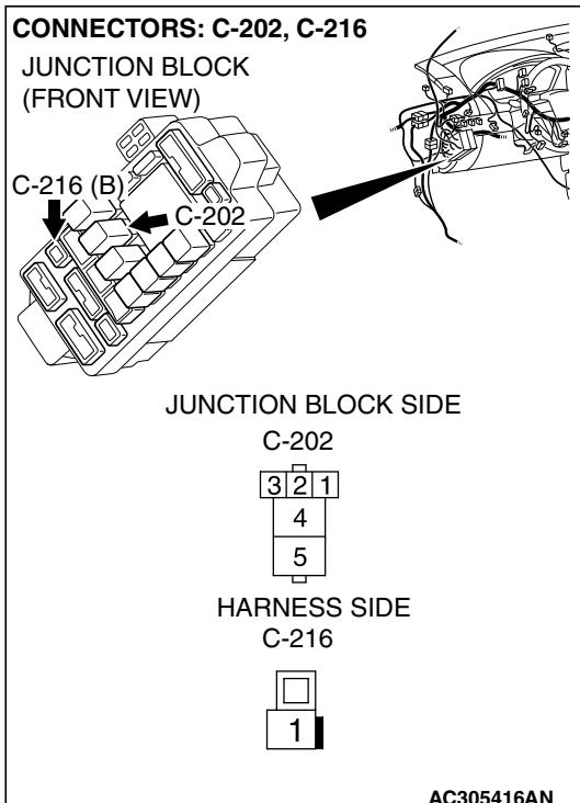
**NOTE:** Also check intermediate connector C-29 and junction block connector C-216 for loose, corroded, or damaged terminals, or terminals pushed back in the connector. If intermediate connector C-29, junction block connector C-216 is damaged, repair or replace the connector as described in GROUP 00E, Harness Connector Inspection [P.00E-2](#).
