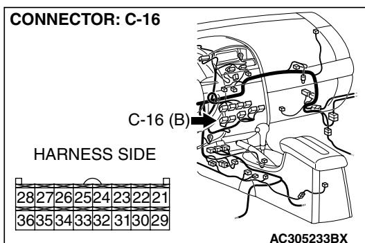
**STEP 8. Measure the resistance at A/C-ECU connector C-16.**
