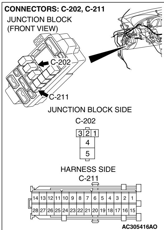
**STEP 9. Measure the resistance at blower relay connector C-202.**
