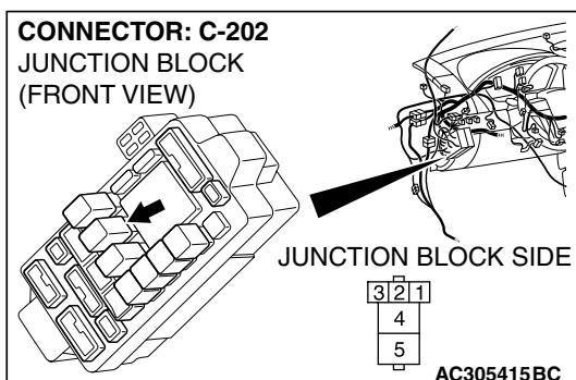
**STEP 7. Measure the voltage at blower relay connector C-202.**
