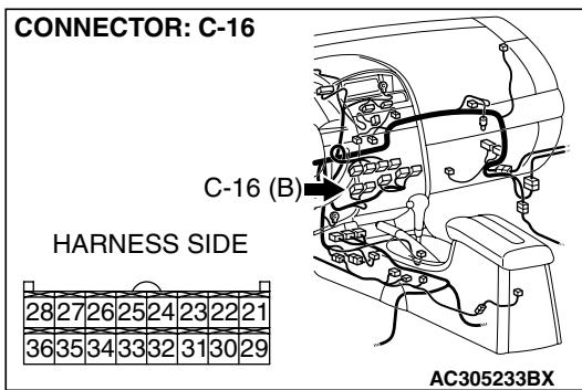
**STEP 4. Measure the voltage at A/C-ECU connector C-16.**
