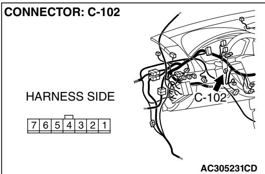
**STEP 5. Check the wiring harness between A/C-ECU connectors C-15 (terminals 16 and 20), C-16 (terminal 21) and mode selection damper control motor and potentiometer connector C-102 (terminals 5, 7 and 3).**
