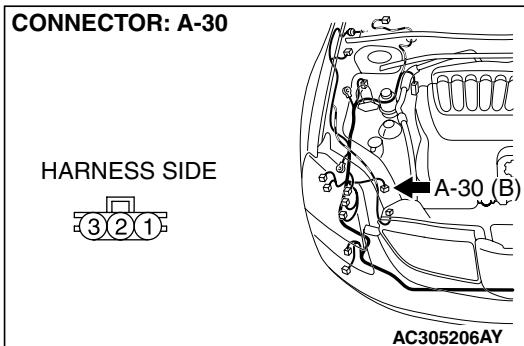
**STEP 3. Check A/C pressure sensor connector A-30 for loose, corroded or damaged terminals, or terminals pushed back in the connector.**
