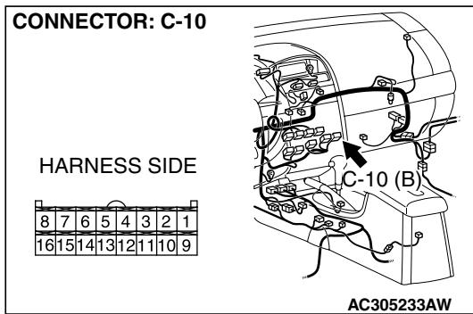
**STEP 5. Check the ambient air temperature sensor.**
