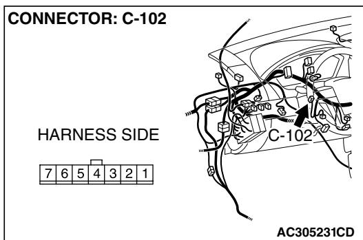
**STEP 5. Check the wiring harness between A/C-ECU connectors C-10 (terminals 15, 11 and 10) and mode selection damper control motor and potentiometer connector C-102 (terminals 5, 7 and 3).**
