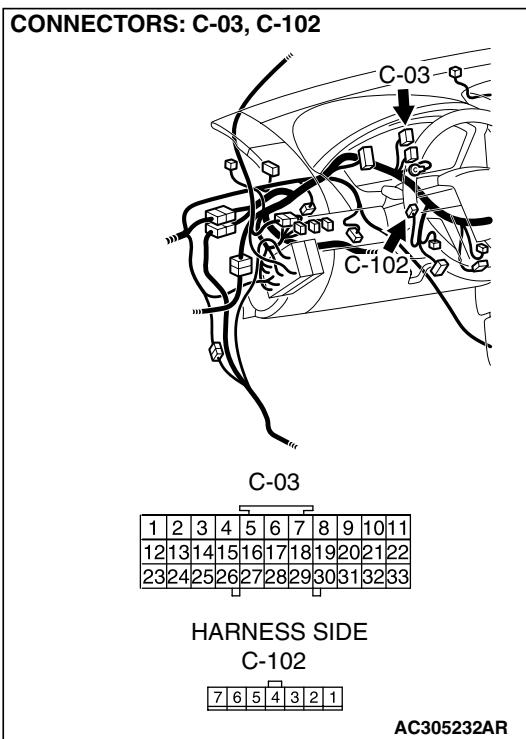
*NOTE: Also check joint connector C-03 for loose, corroded, or damaged terminals, or terminals pushed back in the connector. If joint connector C-03 is damaged, repair or replace the connector as described in GROUP 00E, Harness Connector Inspection [P.00E-2](#).*
