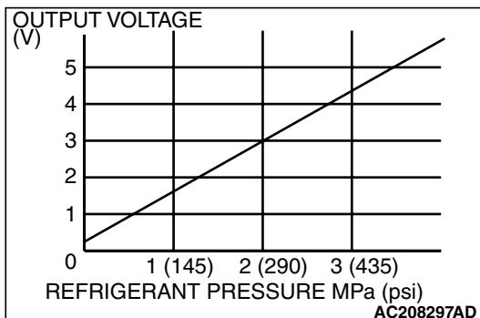
**STEP 22. Check the A/C pressure sensor operation.**
