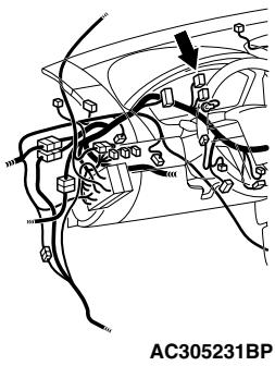
**NOTE:** Also check joint connector C-03, junction block connectors C-211 and C-215 for loose, corroded, or damaged terminals, or terminals pushed back in the connector. If joint connector C-03, junction block connector C-211 or C-215 is damaged, repair or replace the connector as described in GROUP 00E, Harness Connector Inspection [P.00E-2](#).
