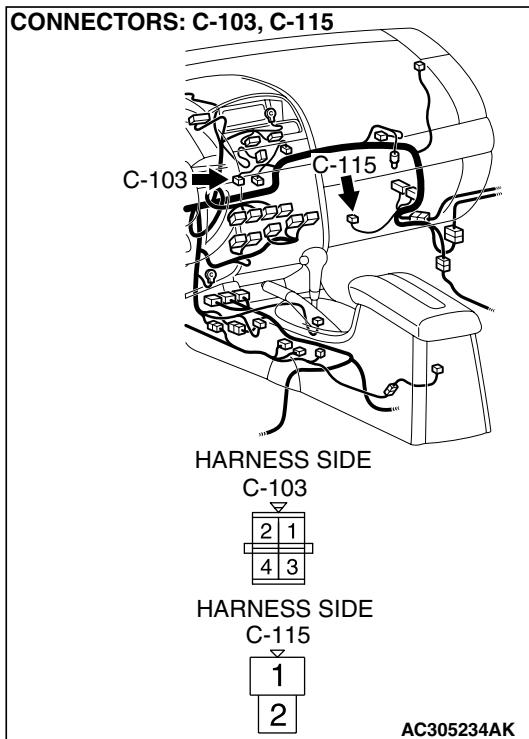
**STEP 4. Check the wiring harness blower switch connector C-115 (terminal 1) and resistor connector C-103 (terminal 2).**
