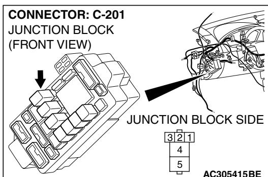
**STEP 6. Measure the voltage at rear window defogger relay connector C-201.**
