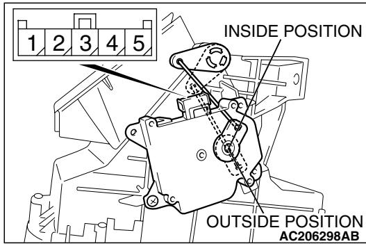
**STEP 5. Check the outside/inside air selection damper control motor.**
