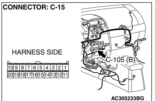
**STEP 16. Measure the voltage at A/C-ECU connector C-15.**
