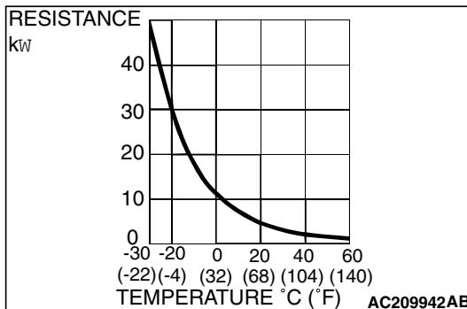
**STEP 21. Check the ambient air temperature sensor.**
