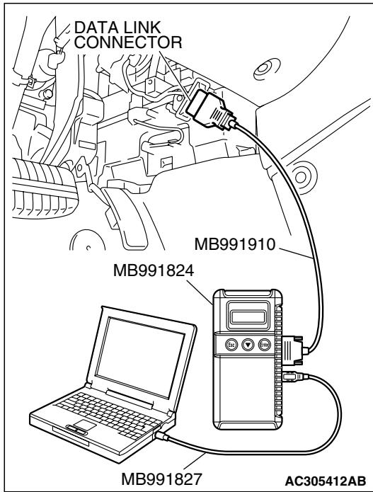
1. Connect the scan tool MB991958 to the data link connector.
