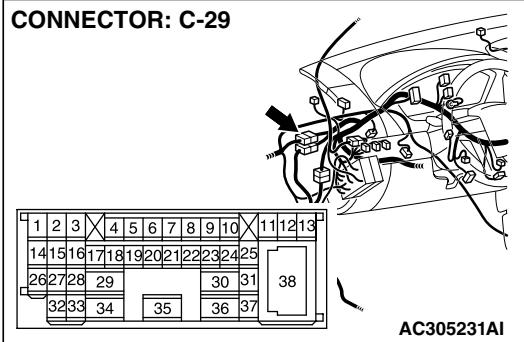
**NOTE:** Also check intermediate connector C-29 and junction block connector C-216 for loose, corroded, or damaged terminals, or terminals pushed back in the connector. If intermediate connector C-29 and junction block connector C-216 is damaged, repair or replace the connector as described in GROUP 00E, Harness Connector Inspection [P.00E-2](#).
