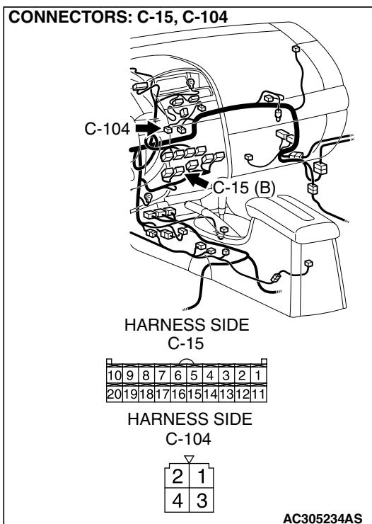
**STEP 16. Check the wiring harness between power transistor connector C-104 (terminals 1 and 3) and A/C-ECU connector C-15 (terminals 17 and 18).**
