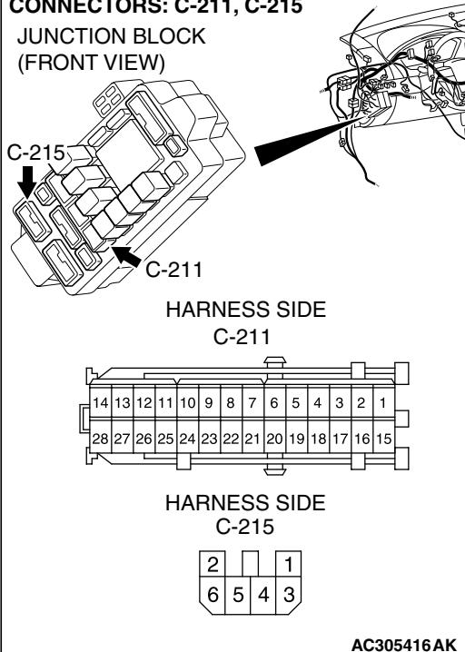
**NOTE:** Also check joint connector C-03, junction block connectors C-211 and C-215 for loose, corroded, or damaged terminals, or terminals pushed back in the connector. If intermediate connector C-03, junction block connector C-211 or C-215 is damaged, repair or replace the connector as described in GROUP 00E, Harness Connector Inspection [P.00E-2](#).
