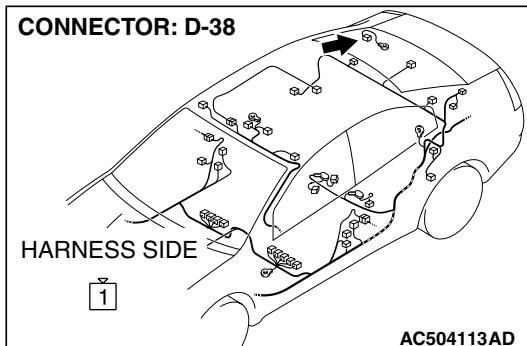
**STEP 15. Check the wiring harness between defogger connector D-38 (terminal 1) and the ground.**
