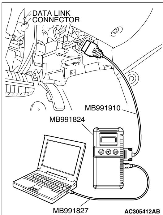
**DTC U1100: Powertrain Control Module Time-out (Related to Engine)****⚠ CAUTION**
