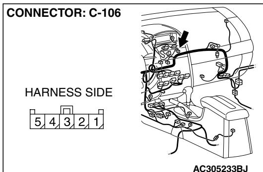
**STEP 3. Measure the voltage at outside/inside air selection damper control motor connector C-106.**
