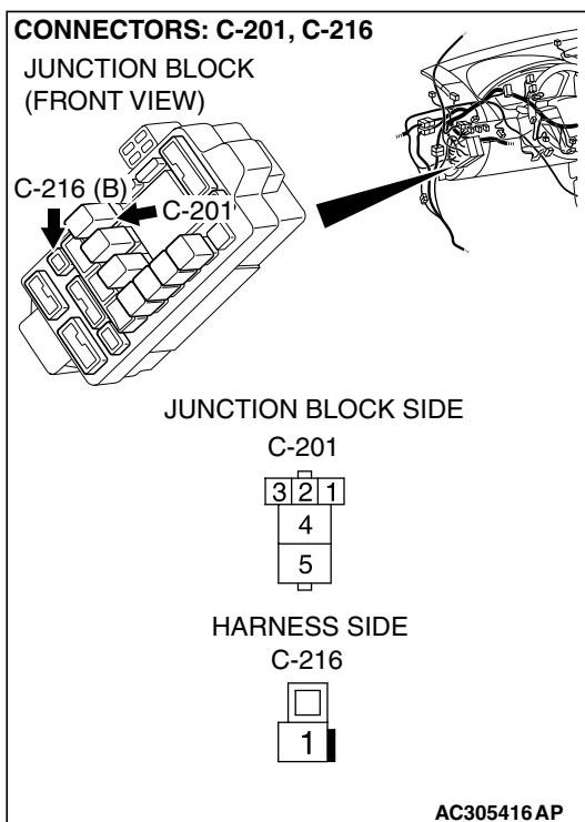
**STEP 7. Check the wiring harness between rear window defogger relay connector C-201 (terminal 5) and the fusible link (1).**
