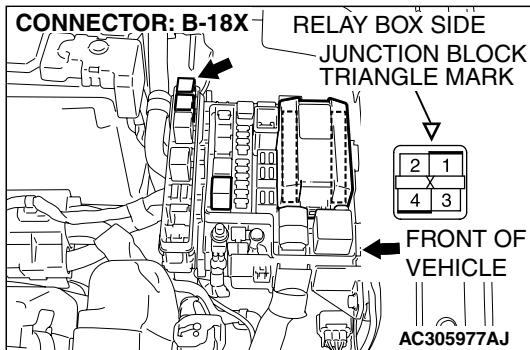
**STEP 14. Check the wiring harness between powertrain control module connector B-21 (terminal 81) and A/C compressor clutch relay connector B-18X (terminal 3).**
