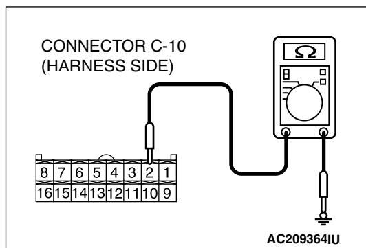
(2) Measure the resistance between terminal 2 and ground.
