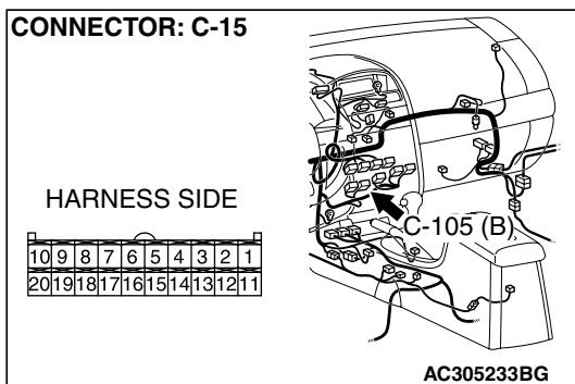
**STEP 6. Check A/C-ECU connector C-15 for loose, corroded or damaged terminals, or terminals pushed back in the connector.**
