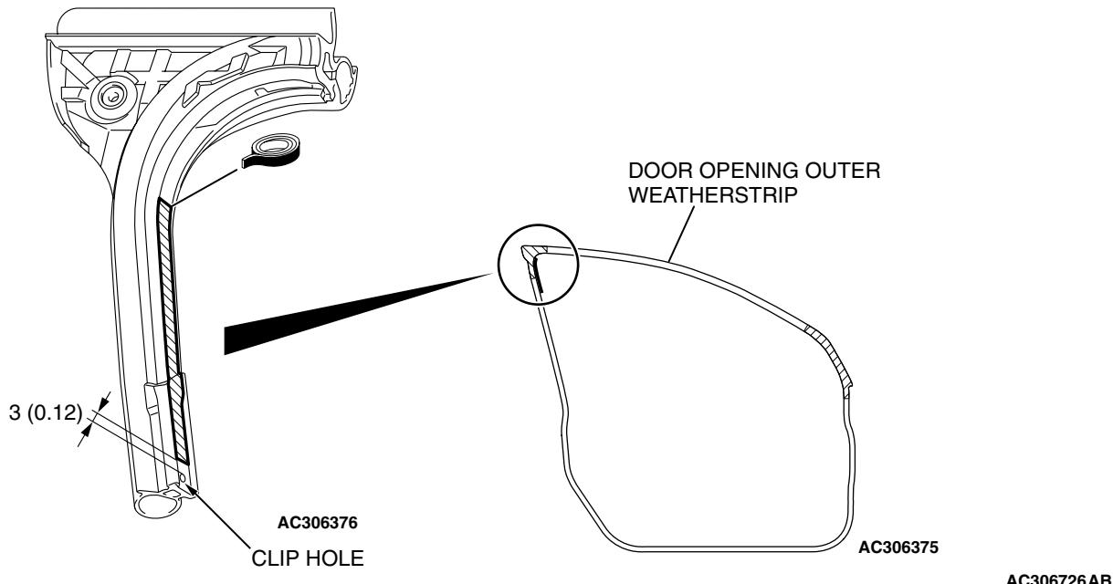
**ADHESIVE TAPE: DOUBLE-SIDED TAPE [ 7 mm (0.28 in) WIDTH, 85 mm (3.35 in) LENGTH AND 0.8 mm (0.031 in) THICKNESS ]**
