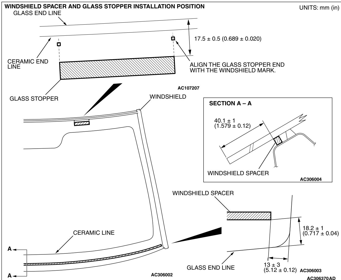
2. Install the windshield spacer and glass stoppers to the specified positions so that there are no adrift or warped surfaces inside the windshield.
