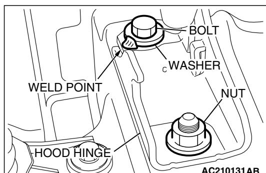
If the hood hinge mounting bolt washers are welded, grind off the welding according to the procedure below beforehand.
