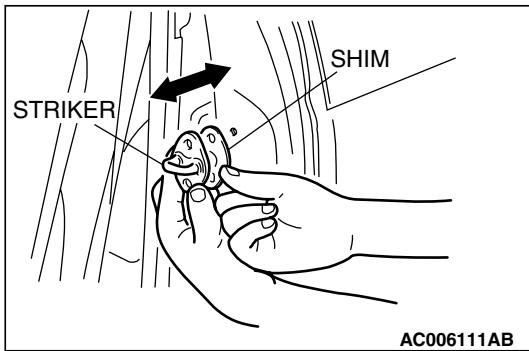
(3) Adjustment by using shims (forward and rearward)
