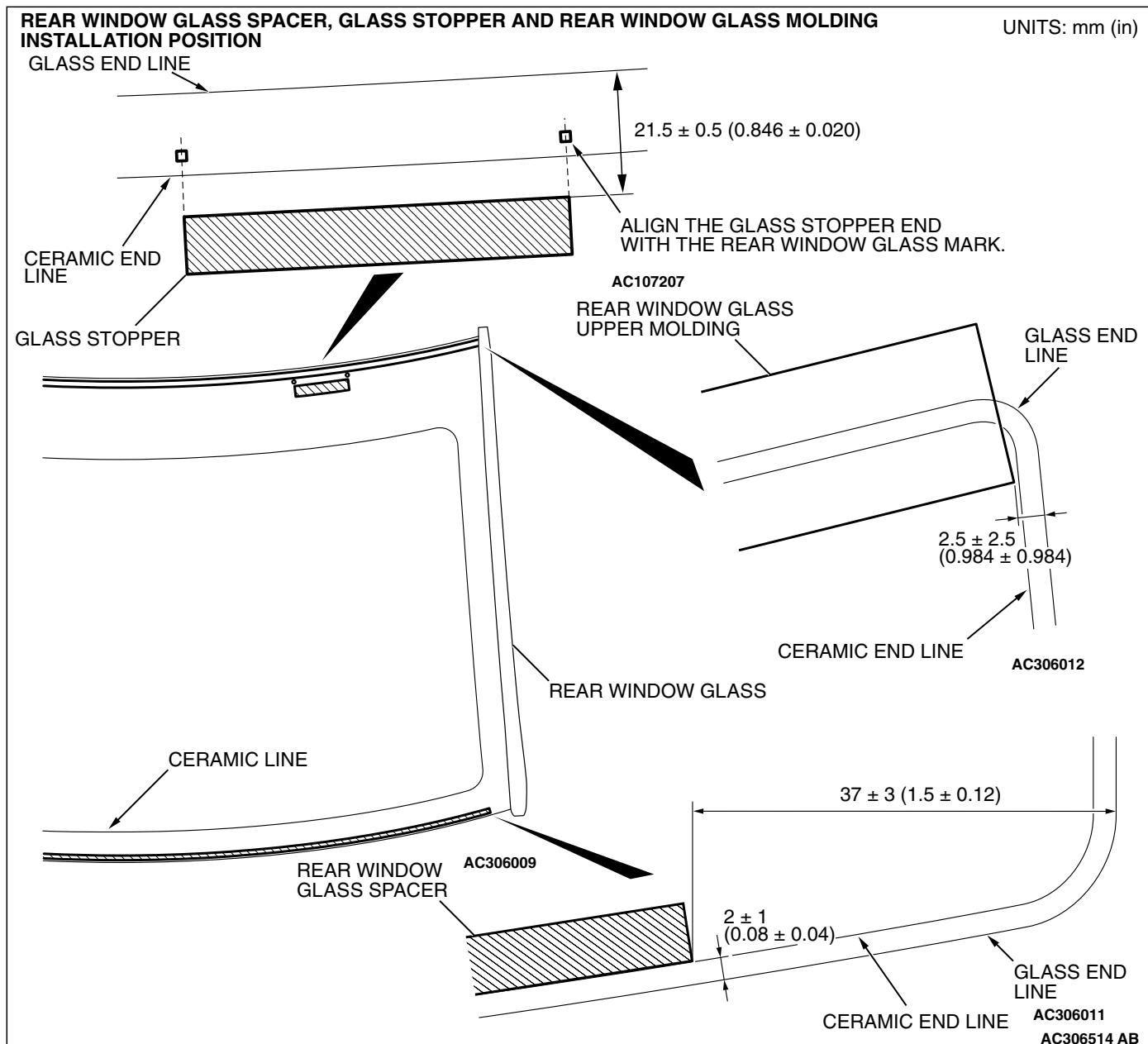
2. Install the rear window spacer and glass stopper to the specified positions so that there are no adrift or bent surfaces inside the rear window glass.
