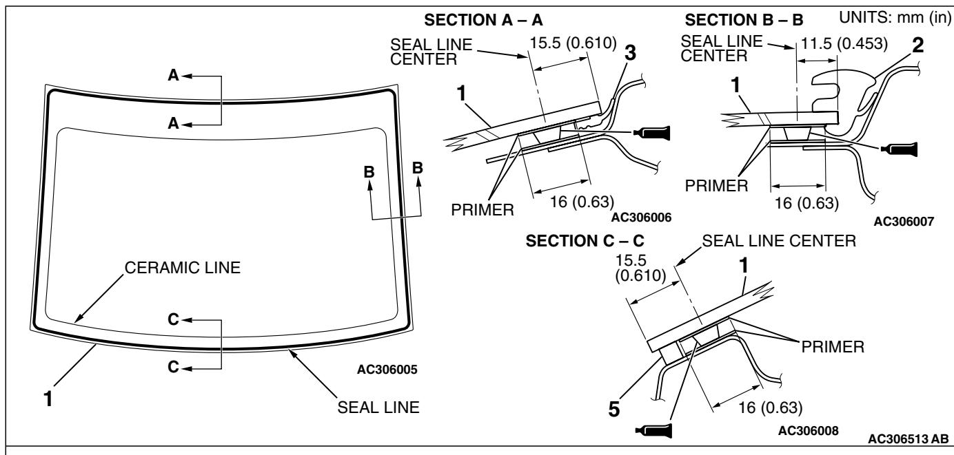
**ADHESIVE: 3M™ AAD PART NO. 8609 SUPER FAST URETHANE AND 3M™ AAD PART NO. 8608 SUPER FAST URETHANE PRIMER OR EQUIVALENT**
