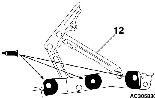
ADHESIVE: 3M™ AAD PART NO.8531 HEAVY DRIP CHECK SEALER, 3M™ AAD PART NO.8646 AUTOMOTIVE JOINT AND SEAM SEALER OR EQUIVALENT
