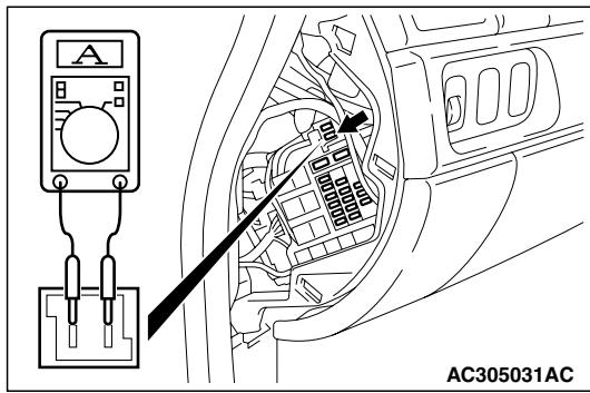
1. Remove the fuse of the sunroof, then connect the circuit tester as shown in the Figure.
