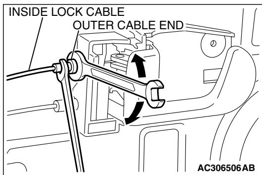
3. If not within the standard value, adjust the inside handle lock knob stroke with the outer cable end connecting the inside handle lock knob and inside lock cable.
