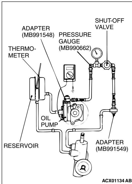
1. Disconnect the pressure hose from the oil pump, and then connect the special tools MB991548, MB990662 and MB991549.
