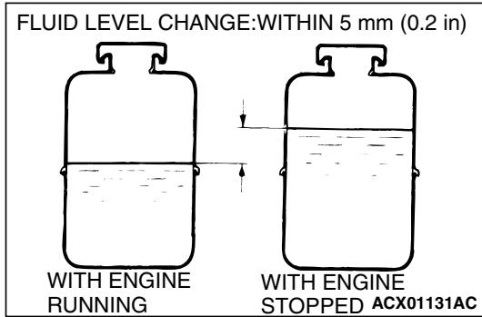
9. Confirm that the change in the fluid level is no more than 5 mm (0.2 inch) when the engine is stopped.
