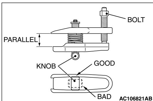
2. Turn the bolt and knob as necessary to make the jaws of special tool MB991897 parallel, tighten the bolt by hand and confirm that the jaws are still parallel.
