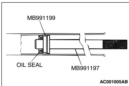
>>C<< STEERING GEAR PINION SHAFT UPPER BEARING (NEEDLE ROLLER BEARING)/STEERING GEAR PINION BEARING (BALL BEARING) INSTALLATION
