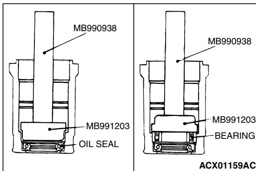
>>H<< OIL SEAL/SPECIAL BEARING INSTALLATION
