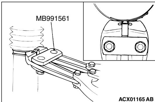
**>>O<< STEERING GEAR BAND (BELLOWS BAND)
