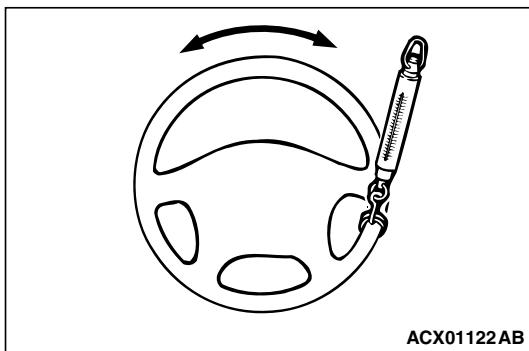
3. Attach a spring scale to the outer circumference of the steering wheel and measure the steering force required to turn the steering wheel from the straight ahead position to the left and right (within a range of 1.5 turns). Also check to be sure that there is no significant change in the required steering effort.
