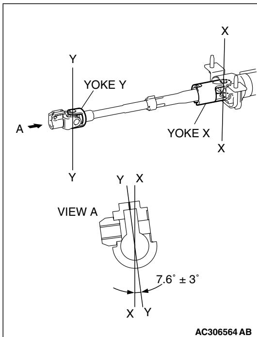
*NOTE: If the steering column shaft is removed accidentally, remove the steering column shaft assembly and be sure to insert the steering column shaft into the steering column as shown in the figure.*
