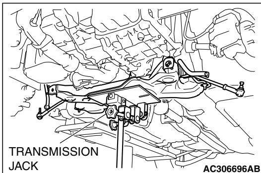
2. Use a transmission jack to hold the crossmember, and then remove the crossmember mounting nuts and bolts.
