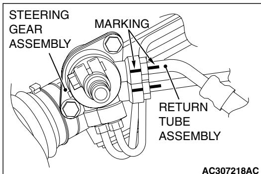
**>>C<< RETURN TUBE ASSEMBLY INSTALLATION**
