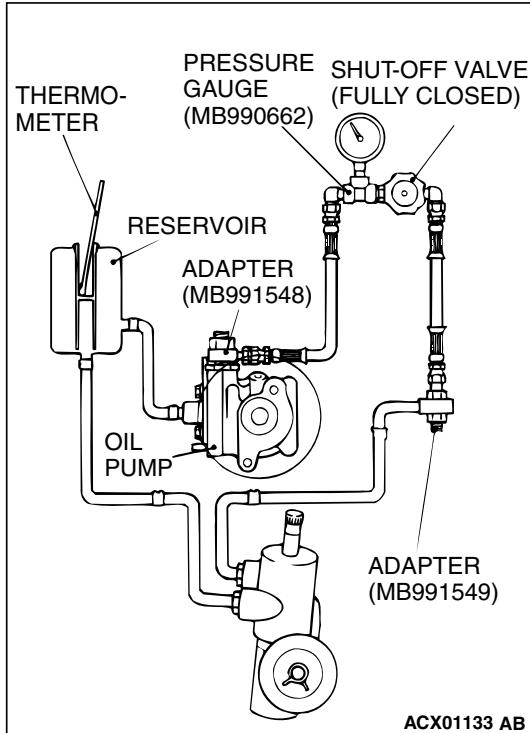
8. Turn the steering wheel all the way to the left or right; then check the retention hydraulic pressure.
