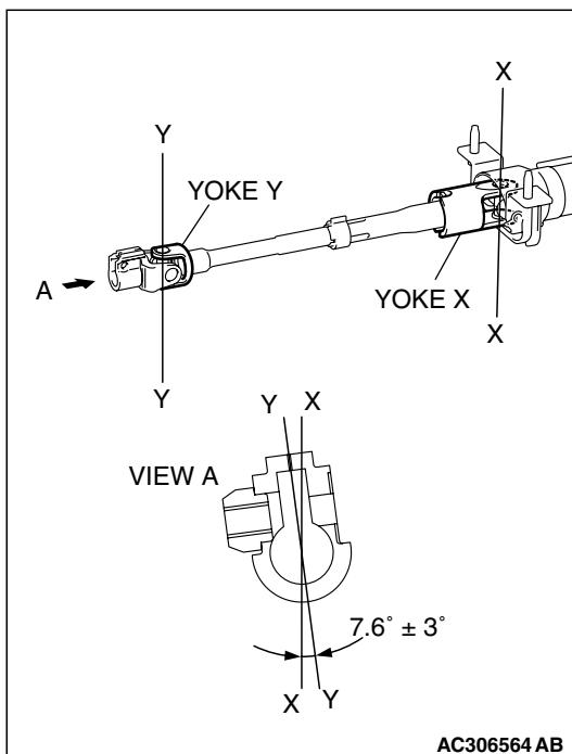
*NOTE: If the steering column shaft is removed accidentally, remove the steering column shaft assembly and be sure to insert the steering column shaft into the steering column as shown in the figure.*
