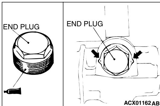
1. Apply 3M™ AAD Part number 8661, 8663, 8672, 8678, 8679 or equivalent to the threaded part of the end plug.
