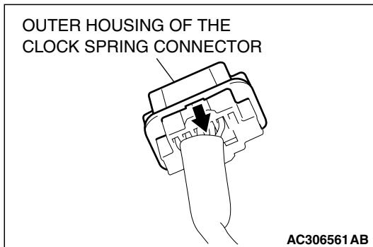
**<<B>> STEERING WHEEL ASSEMBLY REMOVAL**
