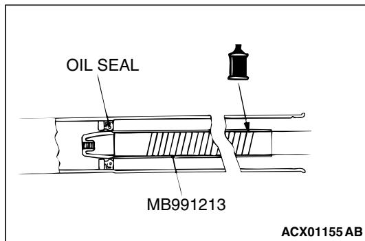
2. Cover the rack serrations with special tool MB991213.
