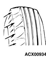
ACX00934 | Lack of rotation of tires or worn or out-of-alignment suspension                                                 | Rotate the tires, and check the front suspension alignment.                                  | Refer to GROUP 33, On-vehicle service – Front wheel alignment check and adjustment <a href="#">P.33-6</a> . |   |
