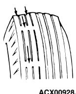
ACX00928AB | Excessive camber<br>
