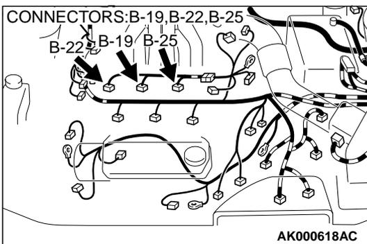
**STEP 11. Check connector B-19 or B-22 or B-25 at right bank injector for damage.**
