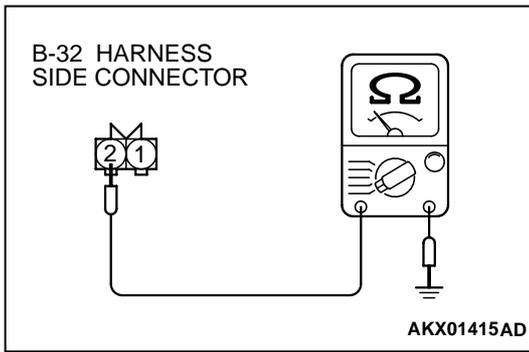
**STEP 2 Check the continuity at knock sensor harness side connector B-32.**
