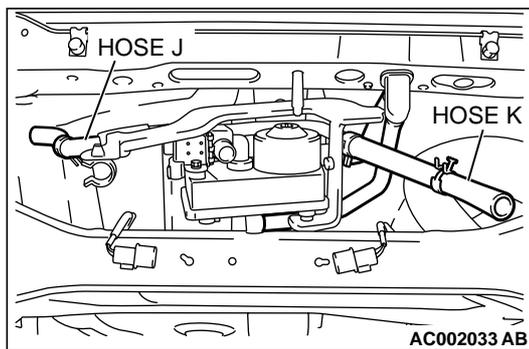
**STEP 15. Check for leaks in the evaporator line from hose J to hose K.**
