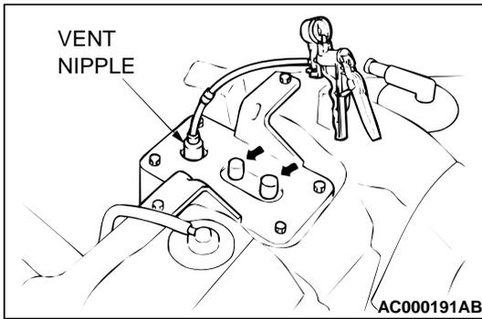
**STEP 23. Check for clogging in the evaporative emission canister.**
