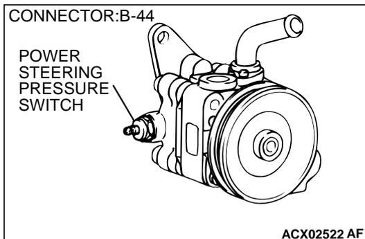
**STEP 4. Using scan tool MB991502, check data list item 27: Power Steering Pressure Switch.**
