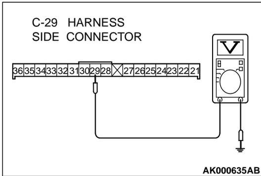
**STEP 4. Check the power supply voltage at combination meter harness side connector C-29.**
