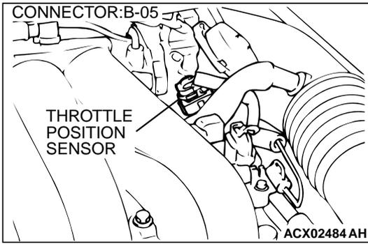
**STEP 2. Check connector B-05 at throttle position sensor for damage.**
