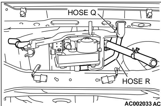
**STEP 22. Check for clogging in the evaporator lines Q and hose R.**
