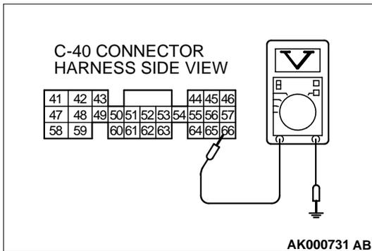
**STEP 3. Check the backup power supply voltage at PCM connector C-40 by backprobing.**
