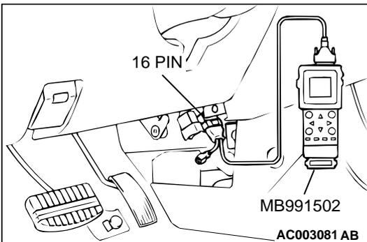
**STEP 4. Using scan tool MB991502, check data list item 25: Barometric Pressure Sensor.**
