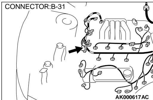
**STEP 12. Check for harness damage between right bank heated oxygen sensor (rear) connector B-31 terminal 2 and PCM connector C-40 terminal 57.**
