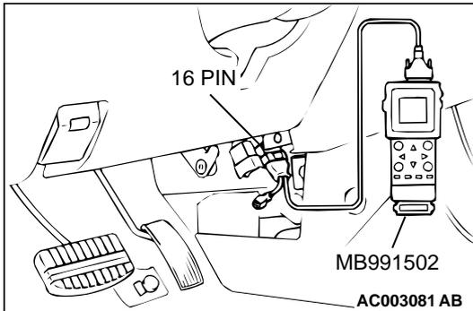
**STEP 3. Using scan tool MB991502, check actuator test.**
