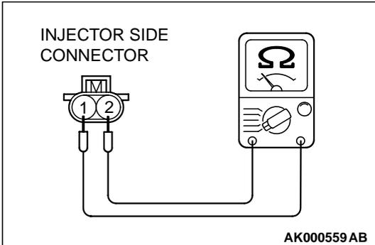
**STEP 3. Check the injector.**
