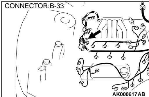
**STEP 12. Check for harness damage between right bank heated oxygen sensor (front) connector B-33 terminal 2 and PCM connector C-40 terminal 57.**
