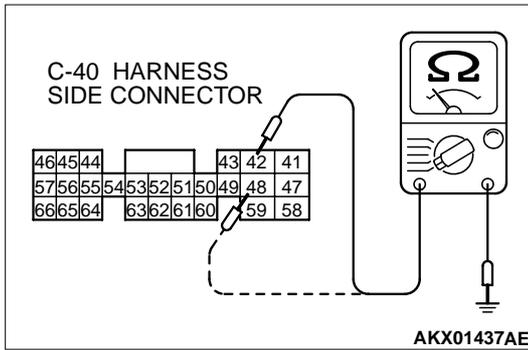
**STEP 7. Check the continuity at PCM harness side connector C-40.**
