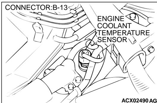
**STEP 5. Check for open circuit between engine coolant temperature sensor connector B-13 terminal 1 and PCM connector C-40 terminal 44.**
