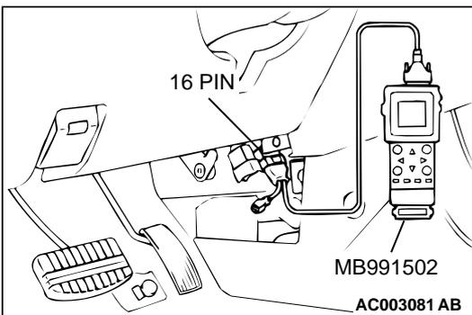
**DTC P0705: Transmission Range Sensor Circuit Malfunction (PRNDL Input)**
