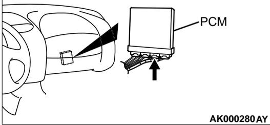
**STEP 11. Check connector C-41 at PCM for damage.**
