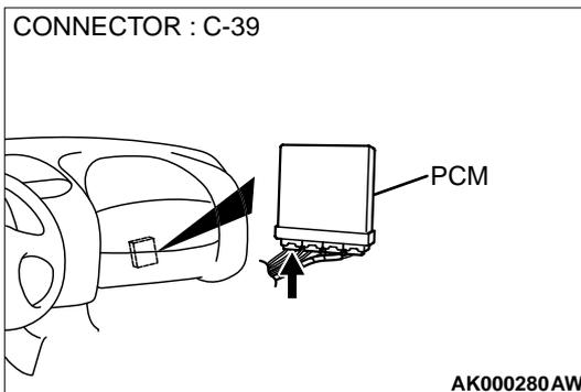
**STEP 12. Check for harness damage between right bank injector connector and PCM connector.**
