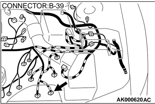
**STEP 5. Check for open circuit and short circuit to ground and harness damage between park/neutral position switch connector B-39 terminal 9 and PCM connector C-40 terminal 58.**
