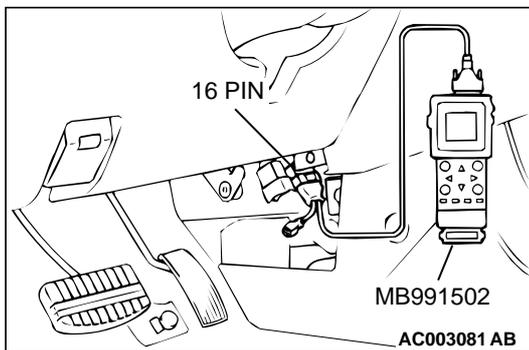
**STEP 4. Using scan tool MB991502, check data list item 11: Heated Oxygen Sensor Bank 2, Sensor 1 (left front).**
