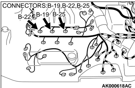
**STEP 9. Check connector B-19, B-22, B-25 at right bank injector for damage.**
