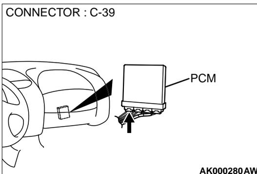
**STEP 8. Check connector C-39 at PCM for damage.**
