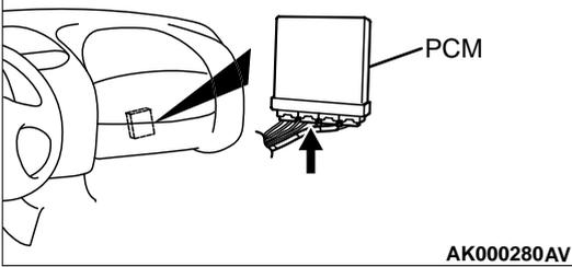
**STEP 7. Check connector C-115 at PCM for damage.**
