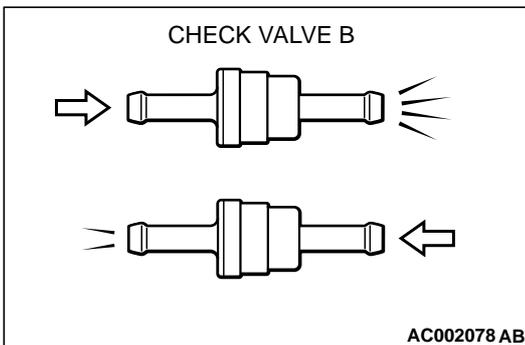
**STEP 29. Check the check valve B.**
