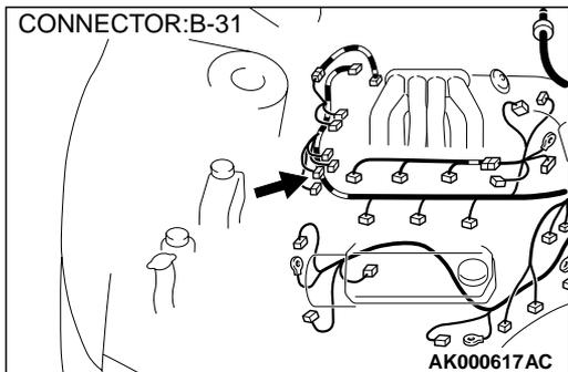
**STEP 10. Check for open circuit and harness damage between right bank heated oxygen sensor (rear) connector B-31 terminal 2 and PCM connector C-40 terminal 57.**
