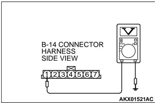
**STEP 5. Check the sensor supply voltage at barometric pressure sensor connector B-14 by backprobing**
