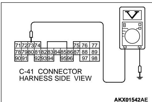
**STEP 4. Check connector B-29 at left bank heated oxygen sensor (rear) and connector C-41 at PCM for damage.**
