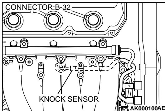
**STEP 4. Check for open circuit, short circuit to ground and harness damage between knock sensor connector B-32 terminal 1 and PCM connector C-41 terminal 90.**
