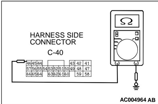
**STEP 13. Check the sensor power supply line for short circuit to ground at PCM connector C-40.**
