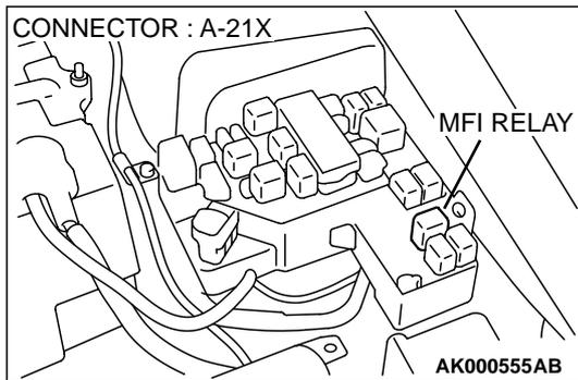
**STEP 14. Check connector A-21X at the MFI relay for damage.**
