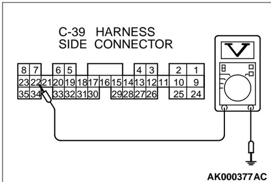
**STEP 6. Check the power supply voltage PCM connector C-39.**
