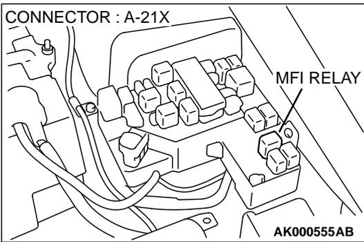
**STEP 10. Check for harness damage between MFI relay connector A-21X terminal 1 and evaporative emission purge solenoid connector B-04 terminal 2.**
