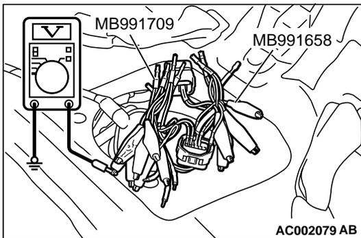
**STEP 4. Check the ground circuit voltage at intermediate connector D-15.**
