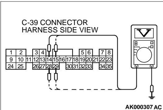
**STEP 7. Check the power supply voltage at PCM connector C-39 by backprobing**
