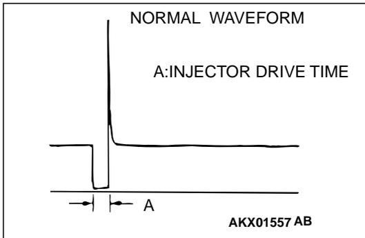
**STEP 11. Using the oscilloscope, check the injector.**
