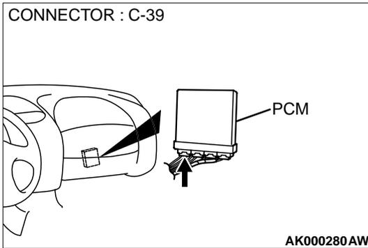
**STEP 12. Check the connector C-39 at the PCM for damage.**
