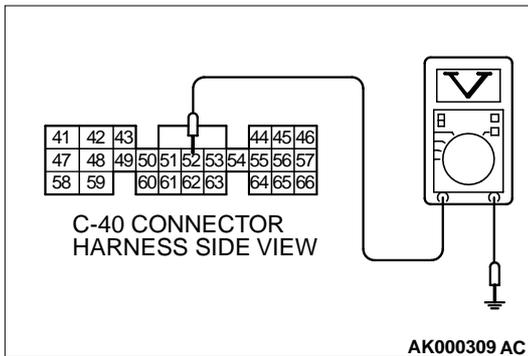
**STEP 7. Check the power supply voltage at PCM connector C-40 by backprobing**
