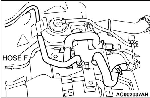
**STEP 26. Check for clogging in the evaporator line from hose F.**
