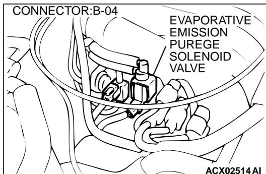
**STEP 8. Check for open circuit and short circuit to ground between evaporative emission purge solenoid connector B-04 terminal 1 and PCM connector C-39 terminal 34.**
