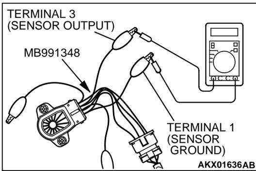
4. If not within the standard value range, adjust by loosening throttle position sensor mounting bolts and turning the throttle position sensor body. After adjusting, tighten the bolts securely.
