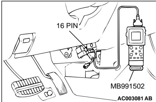
**STEP 1. Using scan tool MB991502, check data list item 59: Heated Oxygen Sensor Bank 2, Sensor 2 (left rear).**
