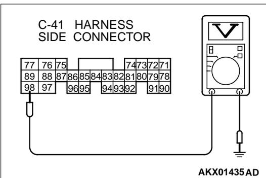
**STEP 5. Check the ignition switch-IG signal voltage at PCM harness side connector C-41.**
