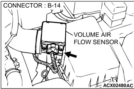
**STEP 4. Check connector B-14 at the volume air flow sensor for damage.**
