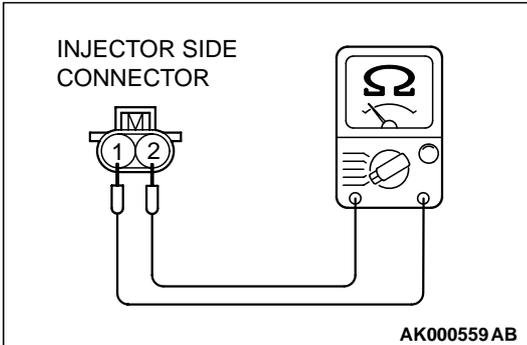
**STEP 5. Check the left bank injector.**
