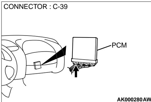
**STEP 10. Check for open circuit and short circuit to ground and harness damage between injector intermediate connector and PCM connector.**
