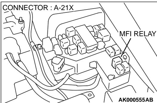
**STEP 8. Check for harness damage between MFI relay connector A-21X terminal 1 and injector intermediate connector B-26 terminal 1.**
