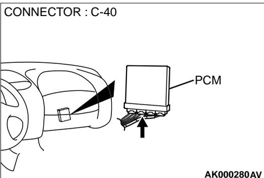
**STEP 10. Check for short circuit to ground between power steering pressure switch connector B-44 terminal 1 and PCM connector C-40 terminal 52.**
