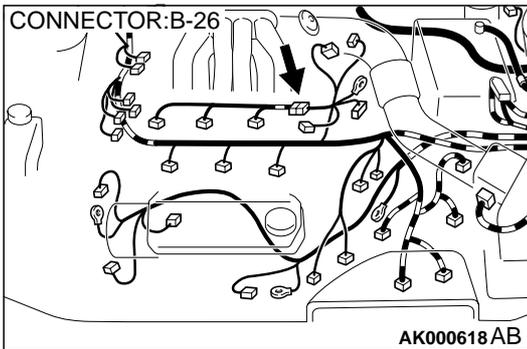
**STEP 6. Check the right bank injector resistance at intermediate connector B-26.**
