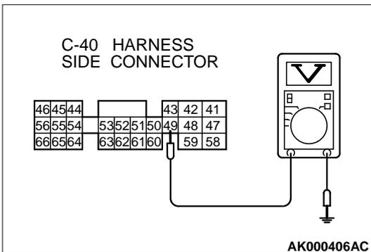
**STEP 8. Check the power supply voltage at PCM harness side connector C-40.**
