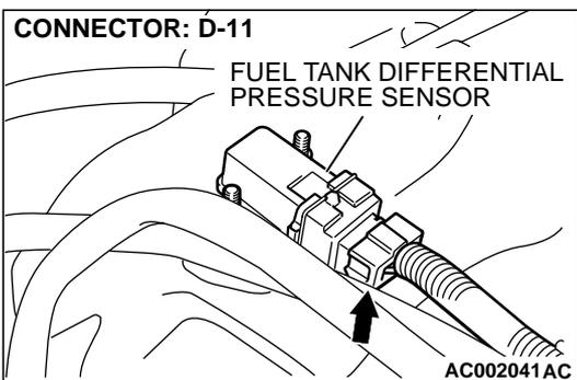
**STEP 17. Check the harness between fuel tank differential pressure sensor connector D-11 and intermediate connector D-15 for open circuit or damage.**
