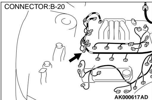
**STEP 17. Check for harness damage between crankshaft position sensor connector B-20 terminal 2 and PCM connector C-40 terminal 45.**
