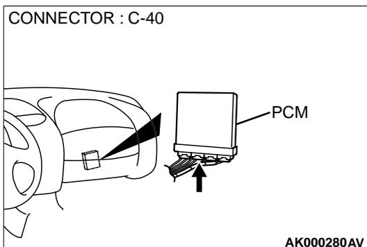
**STEP 5. Check connector C-40 at PCM for damage.**
