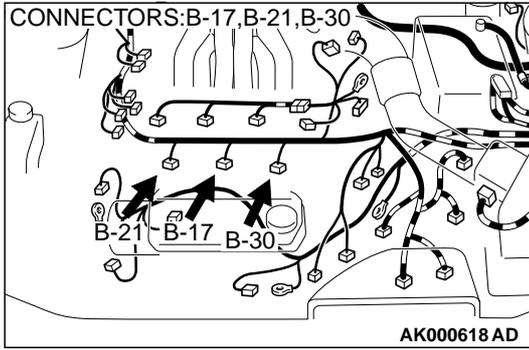
**STEP 8. Check the left bank injector.**
