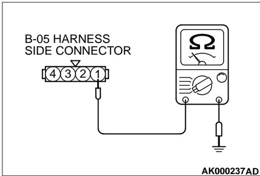
**STEP 5. Check the continuity at throttle position sensor harness side connector B-05**
