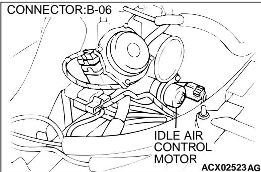
**STEP 13. Check for harness damage between idle air control motor connector B-06 and PCM connector C-39.**
