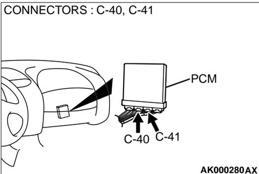
**STEP 8. Check the throttle position sensor.**
