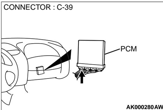
**STEP 8. connector C-39 at PCM for damage.**
