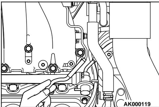
9. Disconnect the vacuum hose (blue stripe) from the fuel pressure regulator and measure fuel pressure with the hose end closed with your finger.
