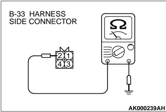
**STEP 8. Check the continuity at right bank heated oxygen sensor (front) harness side connector B-33.**
