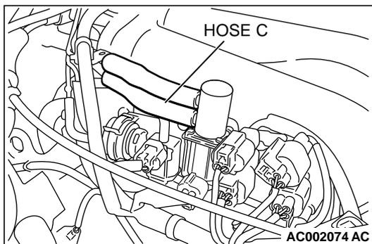
**STEP 25. Check for clogging in the evaporator line hose C to hose E.**
