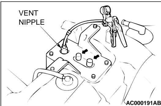
**STEP 25. Check for clogging in the evaporative emission canister.**
