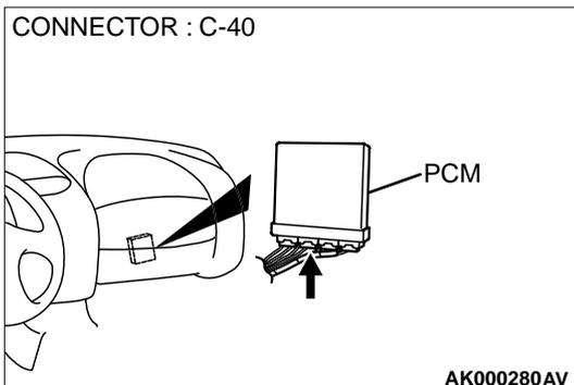
**STEP 9. Check connector C-40 at PCM for damage.**
