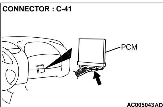
**STEP 18. Check PCM connector C-41 for damage.**
