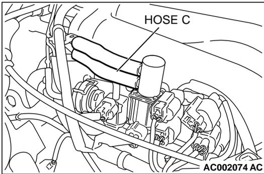
**STEP 9. Check for leaks in the evaporator line hose C to hose E.**
