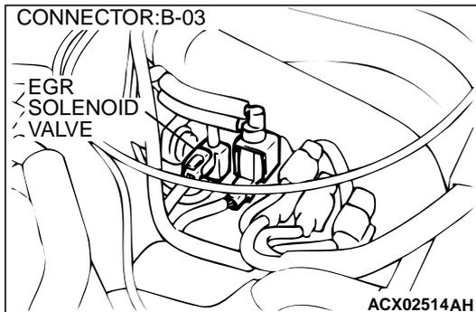
**STEP 8. Check for open circuit and short circuit to ground between EGR solenoid connector B-03 terminal 2 and PCM connector C-39 terminal 6.**
