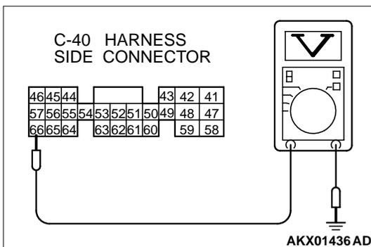
**STEP 4. Check the backup power supply voltage at PCM harness side connector C-40.**
