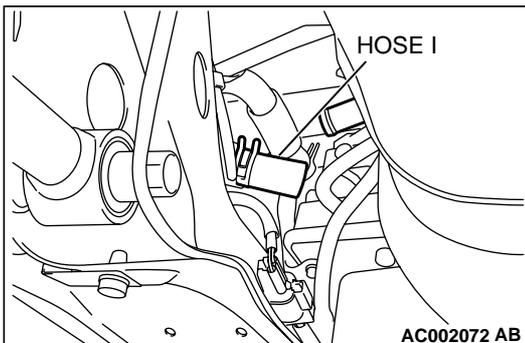
**STEP 23. Check for clogging in the evaporator lines I.**
