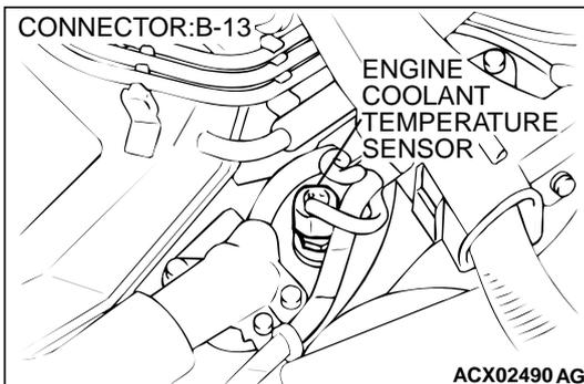
**STEP 6. Check the sensor supply voltage at engine coolant temperature sensor harness side connector B-13.**
