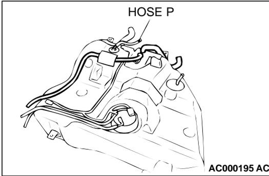
**STEP 31. Check for clogging in the evaporator line from hose P.**
