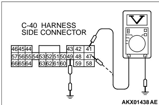
**STEP 9. Check the power supply voltage at PCM harness side connector C-40.**
