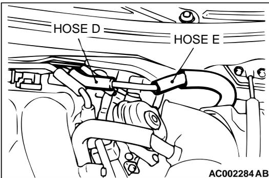
**STEP 5. Check for leaks in the evaporator line hose C to hose E.**
