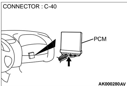
**STEP 6. Check connector C-40 at PCM for damage.**
