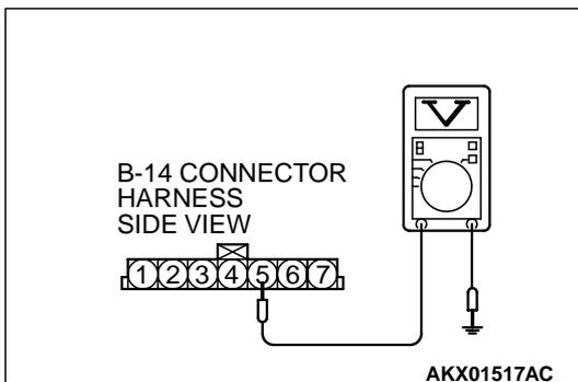
**STEP 7. Check the ground voltage at barometric pressure sensor connector B-14 by backprobing.**
