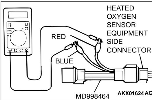
**STEP 3. Check the power supply voltage at right bank heated oxygen sensor (front) harness side connector B-33.**
