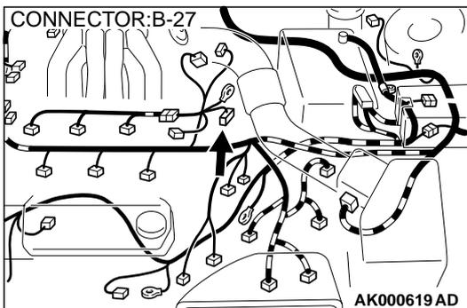
**STEP 16. Check for harness damage between camshaft position sensor connector B-22 terminal 5 and PCM connector C-115 terminal 56.**
