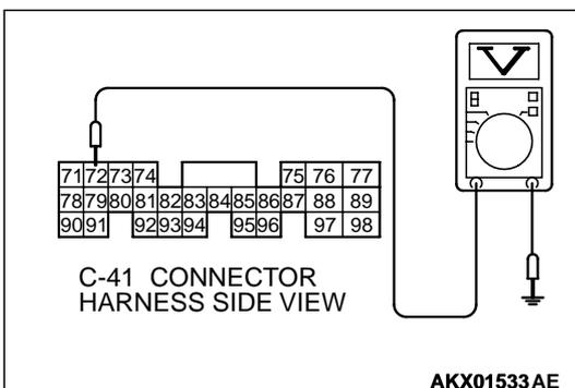
**STEP 4. Check connector B-33 at right bank heated oxygen sensor (front) and connector C-41 at PCM for damage.**
