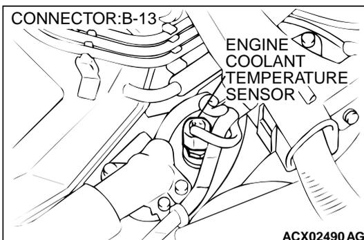
**STEP 4. Using scan tool MB991502, check data list item 21: Engine Coolant Temperature Sensor.**
