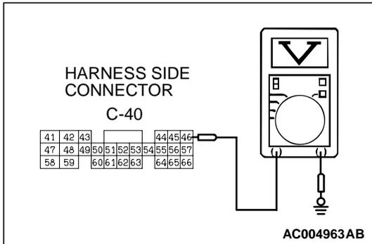
**STEP 11. Check the 5-volt supply circuit voltage at PCM connector C-40.**
