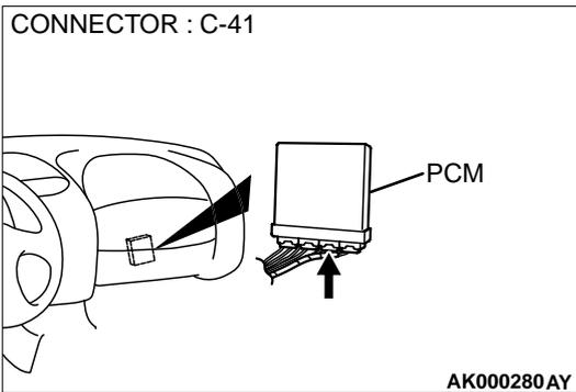
**STEP 9. Check for harness damage between left bank injector connector and PCM connector.**
