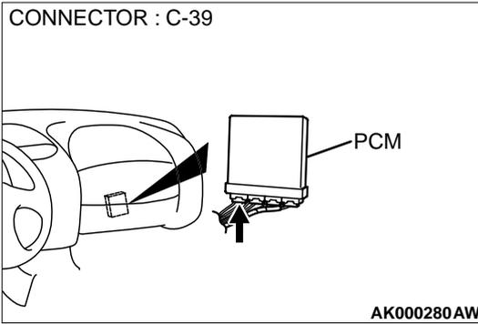
**STEP 13. Check connector C-39 for damage.**
