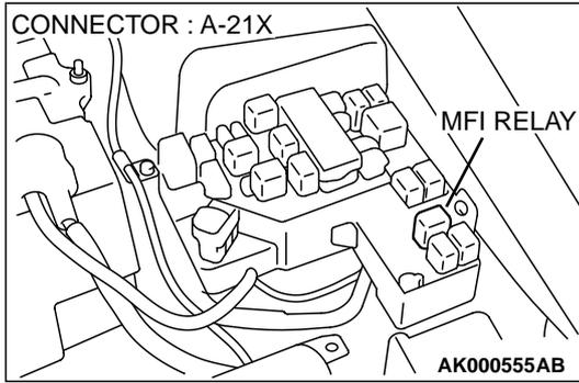
**STEP 6. Check connector A-21X at MFI relay for damage.**
