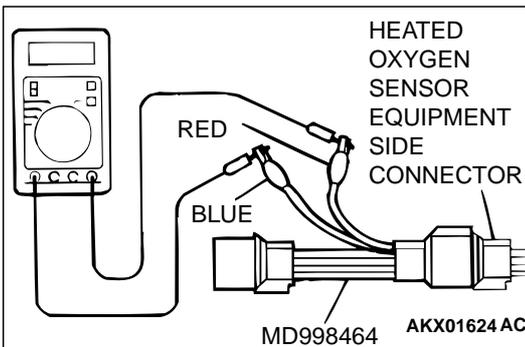
**STEP 3. Check the power supply voltage at left bank heated oxygen sensor (front) harness side connector B-28.**
