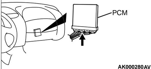
**STEP 13. Check for short circuit to ground and harness damage between right bank heated oxygen sensor (front) connector B-33 terminal 4 and PCM connector C-41 terminal 72.**
