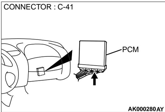
**STEP 12. Check for short circuit to ground between throttle position sensor connector and auto-cruise control-ECU.**
