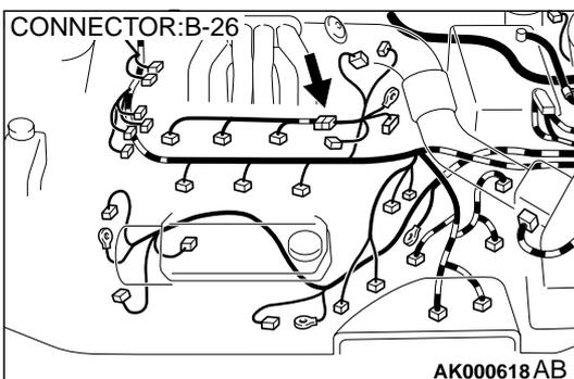
**STEP 12. Check connector B-26 at injector intermediate connector for damage.**
