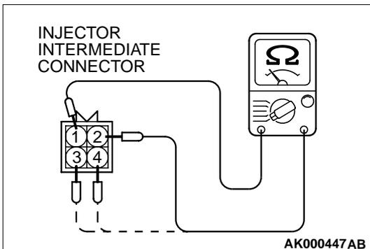
**STEP 7. Check the right bank injector resistance at injector intermediate connector B-26.**
