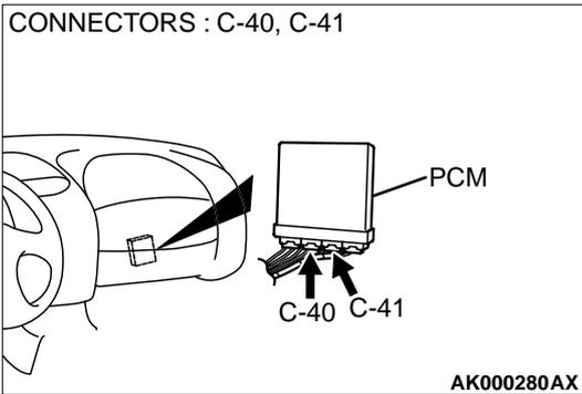
**STEP 4. Check connector C-40 and C-41 at PCM for damage.**
