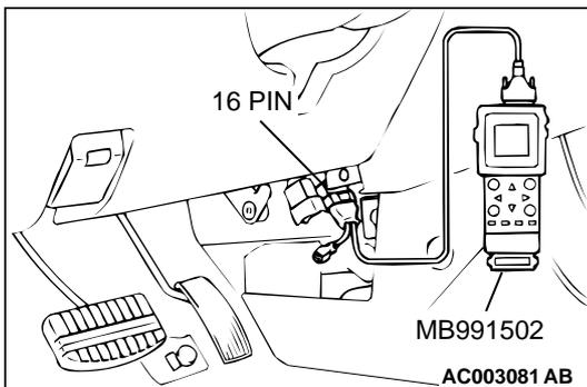
**STEP 6. Using scan tool MB991502, check data list item 25: Barometric Pressure Sensor.**
