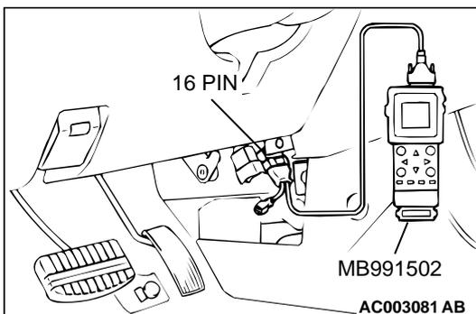
**STEP 5. Using scan tool MB991502, check data list item 45: Idle Air Control Position.**
