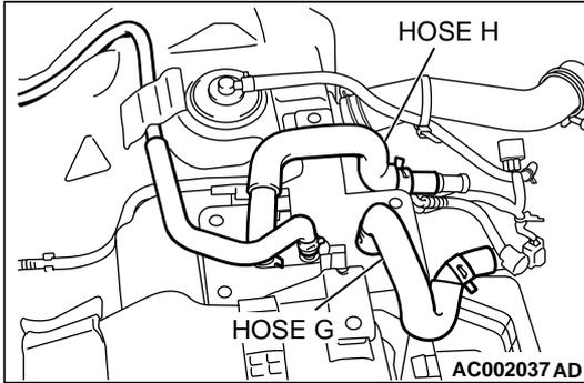
**STEP 24. Check for clogging in the evaporator line from hose G and hose H.**
