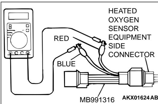
**STEP 3. Check the power supply voltage at left bank heated oxygen sensor (rear) harness side connector B-29.**
