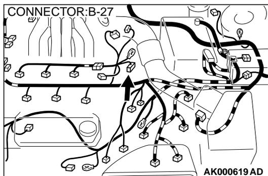
**STEP 7. Check for open circuit between distributor connector B-27 terminal 3 and PCM connector C-39 terminal 11.**
