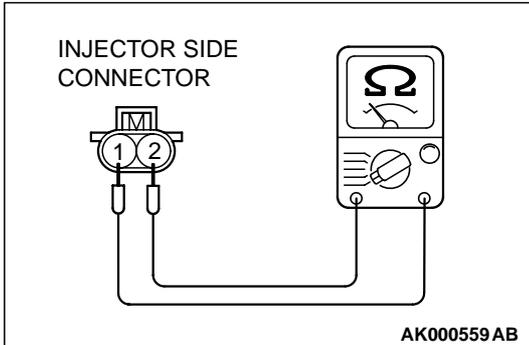
**STEP 5. Check the injector.**
