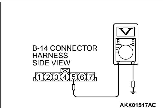
**STEP 12. Check the ground voltage at barometric pressure sensor connector B-14 by backprobing.**
