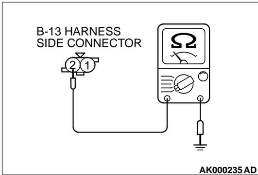
**STEP 6. Check the continuity at engine coolant temperature sensor harness side connector B-13.**
