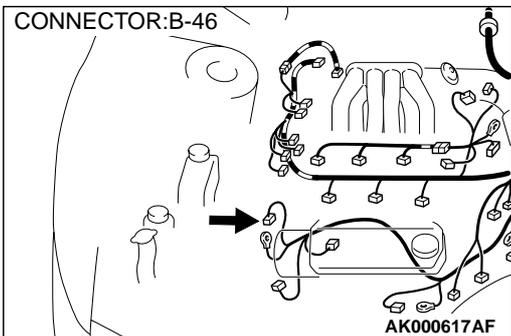
**STEP 6. Check the voltage at generator harness side connector B-46.**
