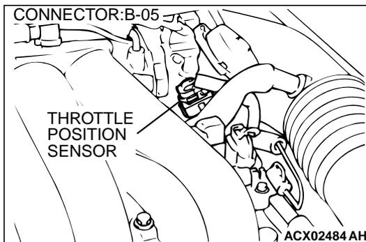
**STEP 6. Check for harness damage between throttle position sensor connector B-05 terminal 4 and PCM connector C-40 terminal 46.**
