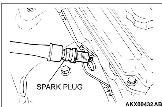
**STEP 4. Check the ignition coil spark**
