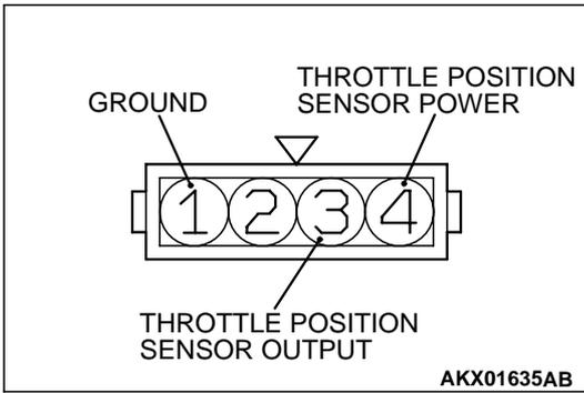
3. Connect an ohmmeter between terminals 1 (ground) and 3 (output), or between terminals 3 (output) and 4 (power). Then, make sure that the resistance changes smoothly when the throttle valve is slowly moved to the fully open position.
