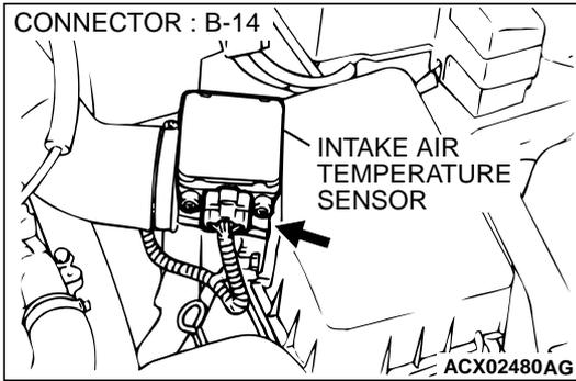
**STEP 15. Check the intake air temperature sensor.**
