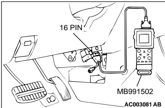
**STEP 3. Using scan tool MB991502, check data list.**
