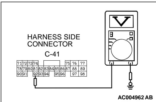
**STEP 10. Check the output circuit voltage at PCM connector C-41.**
