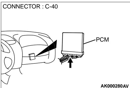
**STEP 8. Check connector C-40 at PCM for damage.**
