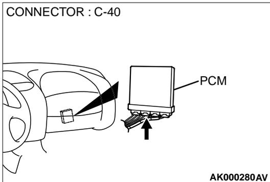
**STEP 10. Check connector C-40 at PCM for damage.**
