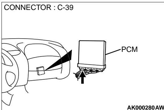
**STEP 10. Check for harness damage between injector connector and PCM connector.**
