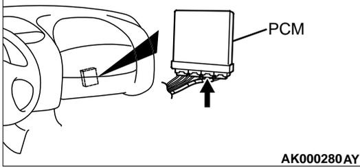
**STEP 11. Check connector C-40 at PCM for damage.**
