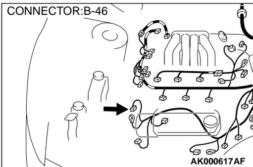
**STEP 8. Check for open circuit and short circuit to ground between generator connector B-46 terminal 4 and PCM connector C-40 terminal 54.**
