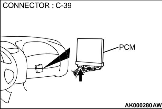
**STEP 9. Check connector C-39 at PCM for damage.**
