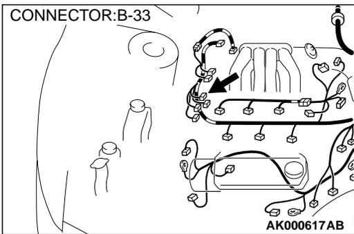
**STEP 10. Check for harness damage between right bank heated oxygen sensor (front) connector B-33 terminal 3 and PCM connector C-39 terminal 4.**
