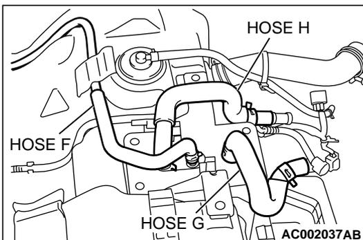
**STEP 11. Check for leaks in the evaporative emission canister.**
