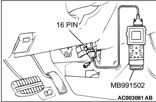
**STEP 8. Using scan tool MB991502, check actuator test.**
