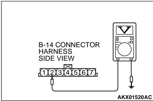
**STEP 2. Check the sensor output voltage at barometric pressure sensor connector B-14 by backprobing.**
