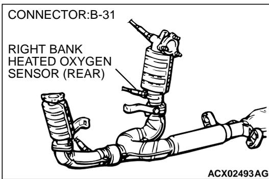
**STEP 2. Check the right bank heated oxygen sensor (rear).**
