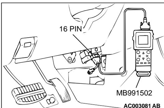
**STEP 5. Check the ignition timing.**
