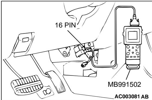
**STEP 2. Using scan tool MB991502, check actuator test.**
