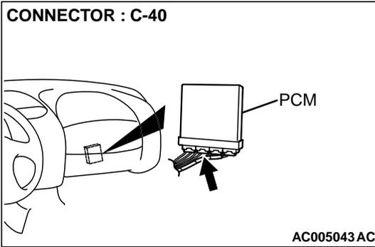
**STEP 16. Check PCM connector C-40 for damage.**
