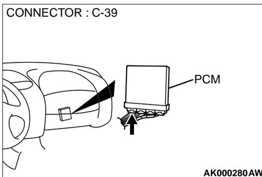
**STEP 5. Check connector C-39 at PCM for damage.**
