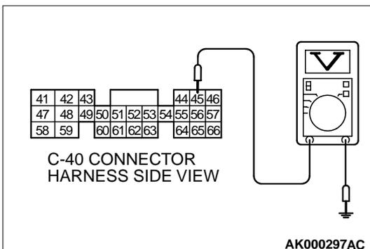
**STEP 7. Check the sensor supply voltage at PCM connector C-40 by backprobing**
