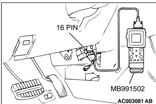
**STEP 7. Using scan tool MB991502, read the diagnostic trouble code (DTC).**
