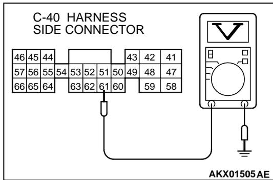
**INSPECTION PROCEDURE 28: Fans (radlator fan, A/C condenser fan) are inoperative**
