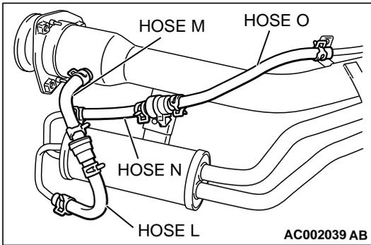
**STEP 12. Check for leaks in the evaporator line hose I, L, M, N and hose O.**
