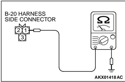
**STEP 13. Check the continuity at crankshaft position sensor harness side connector B-20.**
