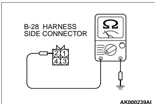
**STEP 8. Check the continuity at left bank heated oxygen sensor (front) harness side connector B-28.**
