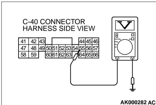
**STEP 3. Check the sensor output voltage at PCM connector C-40 by backprobing.**
