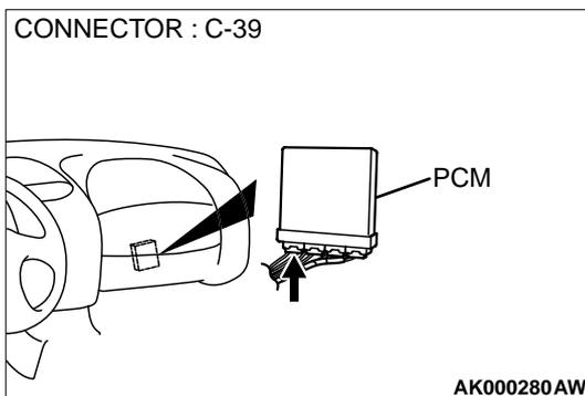
**STEP 14. Check connector C-39 at PCM for damage.**
