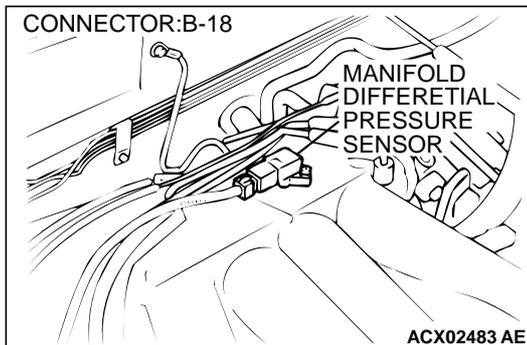
**STEP 3. Check the sensor supply voltage at manifold differential pressure sensor harness side connector B-18.**
