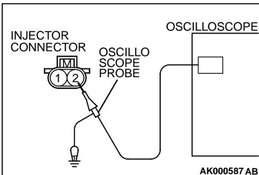
1. Disconnect the injector connector, and connect the test harness special tool (MB991348) in between. (All terminals should be connected.)
