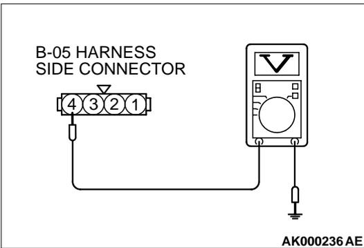
**STEP 3. Check the sensor supply voltage at throttle position sensor harness side connector B-05.**
