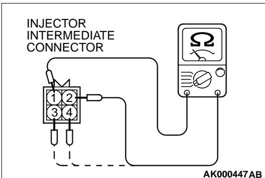
**STEP 8. Check the right bank injector resistance at injector intermediate connector B-26.**
