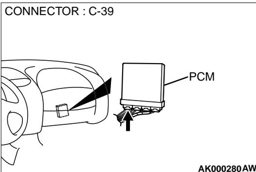
**STEP 11. Check for harness damage between EGR solenoid connector B-03 terminal 2 and PCM connector C-39 terminal 6.**
