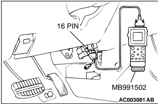
4. Connect scan tool MB991502 to the data link connector.
