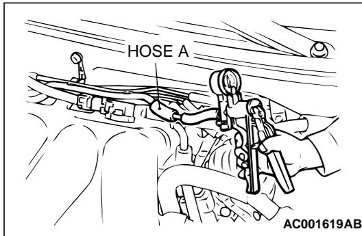
**STEP 2. Check for leaks in the evaporator line hose A and hose B.**
