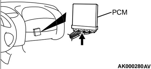
**STEP 8. Check connector C-115 at PCM for damage.**
