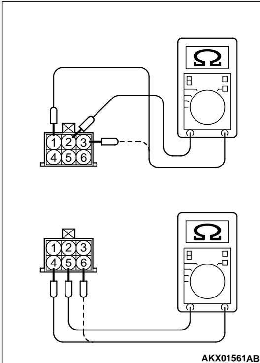
**STEP 4. Check the idle air control motor coil resistance.**
