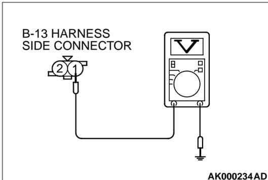
**STEP 3. Check the sensor supply voltage at engine coolant temperature sensor harness side connector B-13.**
