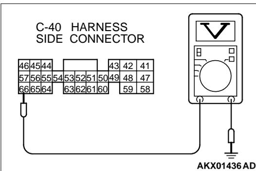
**STEP 6. Check the backup power supply voltage at PCM harness side connector C-40.**
