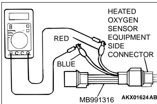
**STEP 3. Check the power supply voltage at right bank heated oxygen sensor (rear) harness side connector B-31.**
