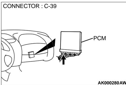
**STEP 2. Check the output voltage at PCM harness side connector C-39.**
