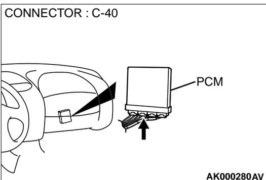
**STEP 11. Check for open circuit and harness damage between volume air flow sensor connector B-14 terminal 5 and PCM connector C-40 terminal 57.**
