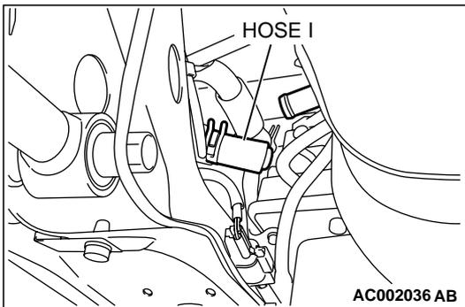
**STEP 7. Pressure test for evaporator line from hose C to hose P.**
