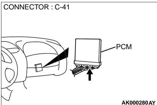
**STEP 3. Check for open circuit, short circuit to ground and harness damage between data link connector C-23 terminal 7 and PCM connector C-41 terminal 85.**
