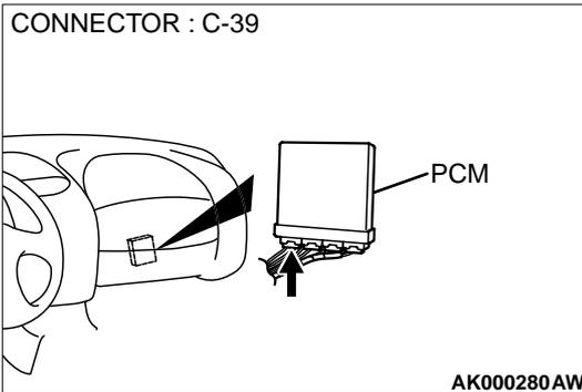
**STEP 4. Check for short circuit to ground between volume air flow sensor connector B-14 terminal 7 and PCM connector C-39 terminal 19.**
