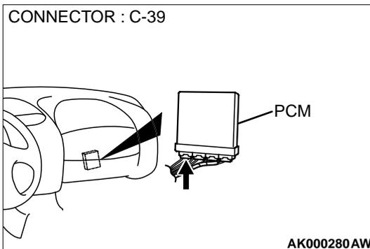
**STEP 7. Check connector C-39 at PCM for damage.**
