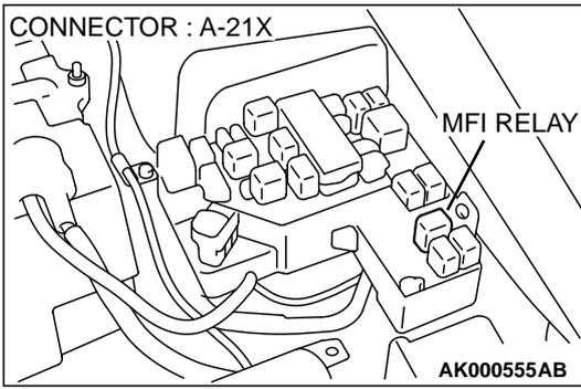
**STEP 4. Check connector A-21X at the MFI relay for damage.**
