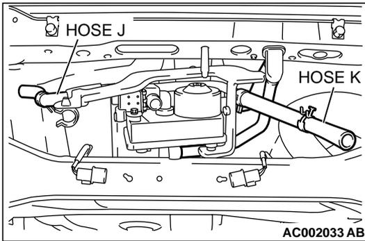
**STEP 19. Check for leaks in the evaporator line from hose J to hose K.**
