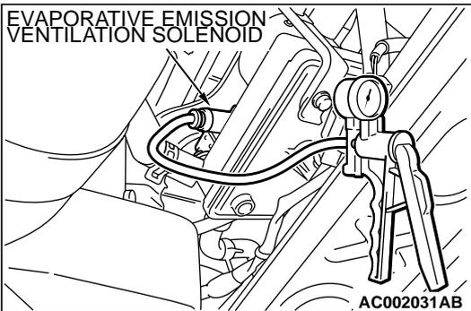
**STEP 3. Check the evaporative emission ventilation solenoid valve using the scan tool MB991502. (Actuator test item 29.)**
