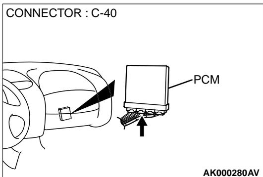
**STEP 15. Check connector C-40 at PCM for damage.**
