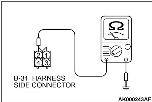
**STEP 8. Check the continuity at right bank heated oxygen sensor (rear) harness side connector B-31.**
