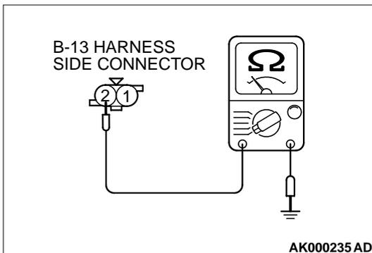
**STEP 8. Check the continuity at engine coolant temperature sensor harness side connector B-13.**
