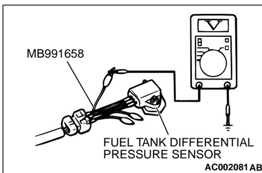
**STEP 7. Check the ground circuit voltage at fuel tank differential pressure sensor connector D-11.**
