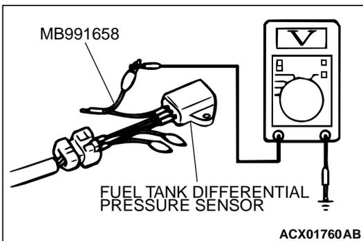
**STEP 9. Check the output voltage at fuel tank differential pressure sensor connector D-11.**
