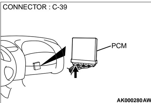
**STEP 6. Check connector C-39 at PCM for damage.**
