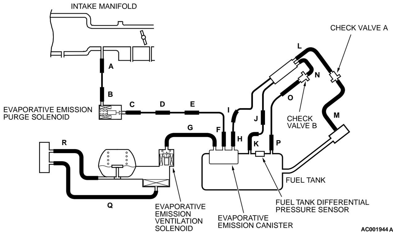
Fuel Tank Differential Pressure Sensor Circuit
