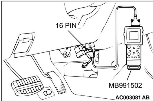
**STEP 1. Using scan tool MB991502, read the immobilizer diagnostic trouble code (DTC).**
