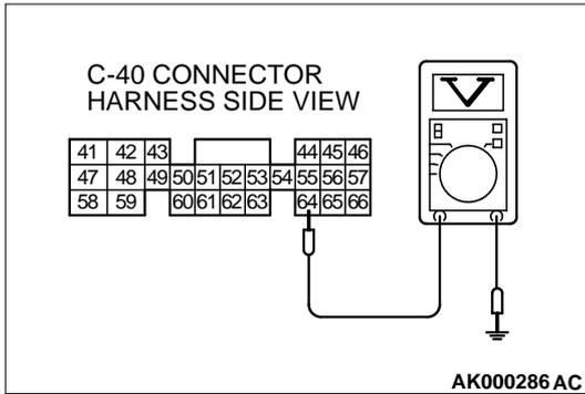
**STEP 8. Check the sensor supply voltage at PCM connector C-40 by backprobing.**
