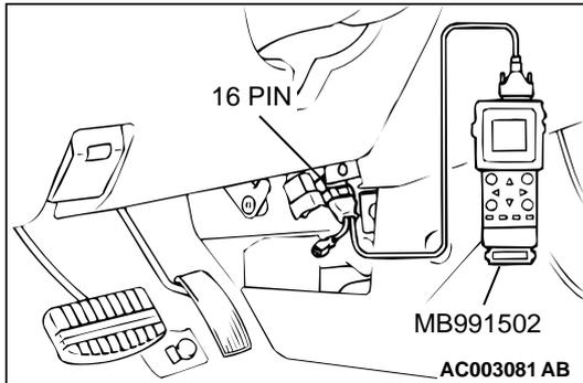
**STEP 1. Using scan tool MB991502, check data list item 39: Heated Oxygen Sensor Bank 1, Sensor 1 (right front).**
