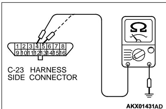
INSPECTION PROCEDURE 2: Scan Tool Communication with PCM Is Not Possible.
