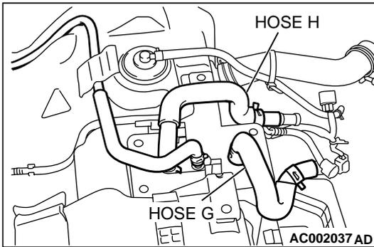
**STEP 22. Check for clogging in the evaporator line from hose H and G.**
