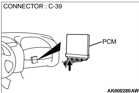
**STEP 10. Check connector C-39 at PCM for damage.**
