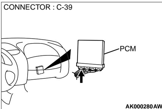
**STEP 7. Check for open circuit and harness damage between volume air flow sensor connector B-14 terminal 7 and PCM connector C-39 terminal 19.**
