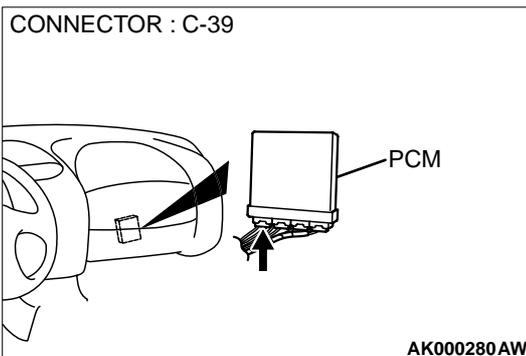
**STEP 7. Check for open circuit or short circuit to ground between right bank heated oxygen sensor (rear) connector B-31 terminal 3 and PCM connector C-39 terminal 27.**
