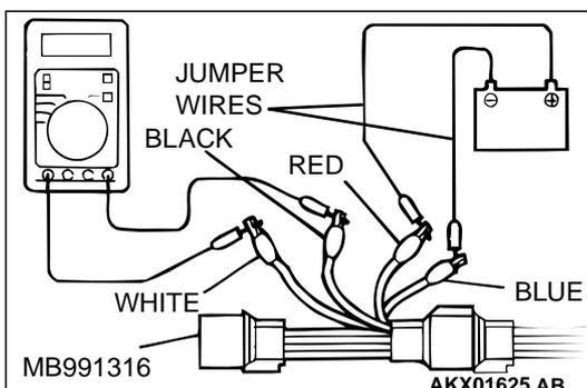
**STEP 14. Check the right bank heated oxygen sensor (rear).**
