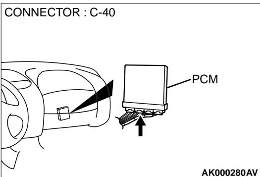
**STEP 11. Check connector C-40 at PCM for damage.**
