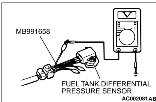
**STEP 5. Check the output circuit voltage at fuel tank differential pressure connector D-11.**
