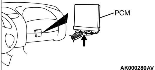
**STEP 13. Check for short circuit to ground and harness damage between right bank heated oxygen sensor (rear) connector B-31 terminal 4 and PCM connector C-41 terminal 74.**
