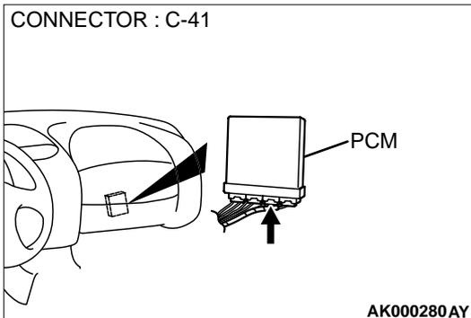
**STEP 11. Check for harness damage between right bank injector connector and PCM connector.**
