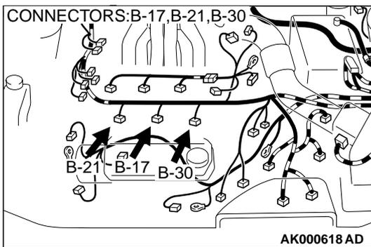
**STEP 13. Check connector B-17, B-21, B-30 at left bank injector for damage.**
