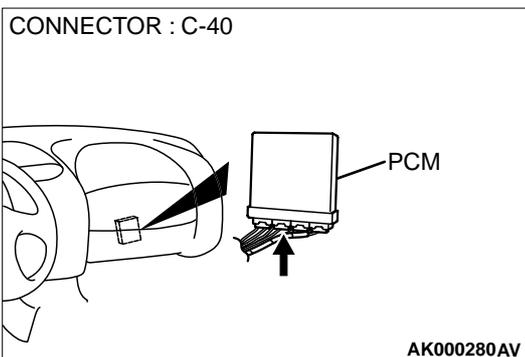
**STEP 17. Check for harness damage between intake air temperature sensor connector B-14 terminal 5 and PCM connector C-40 terminal 57.**
