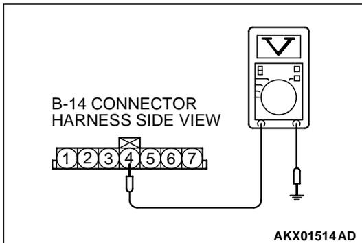
**STEP 3. Check the power supply voltage at volume air flow sensor harness side connector B-14.**
