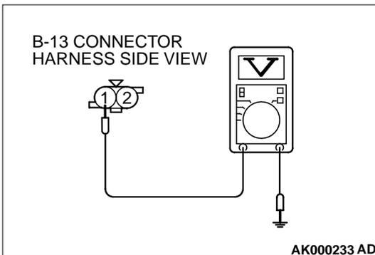
**STEP 3. Check connector B-13 at the engine coolant temperature sensor for damage.**
