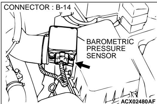
**STEP 17. Check for short circuit to ground and harness damage between barometric pressure sensor connector B-14 terminal 2 and PCM connector C-40 terminal 55.**
