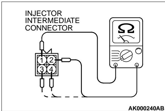
**STEP 8. Check the right bank injector resistance at intermediate connector B-26.**
