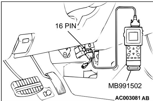
**DTC P0710 : Transmission Fluid Temperature Sensor Circuit Malfunction**
