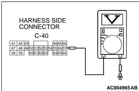
**STEP 15. Check the ground circuit voltage at PCM connector C-40.**
