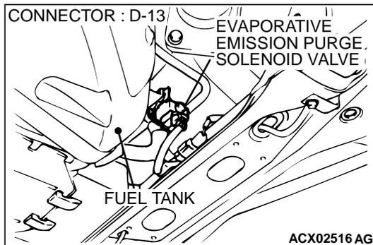
**STEP 8. Check for open circuit and short circuit to ground between evaporative emission ventilation solenoid connector D-13 terminal 1 and PCM connector C-39 terminal 35.**
