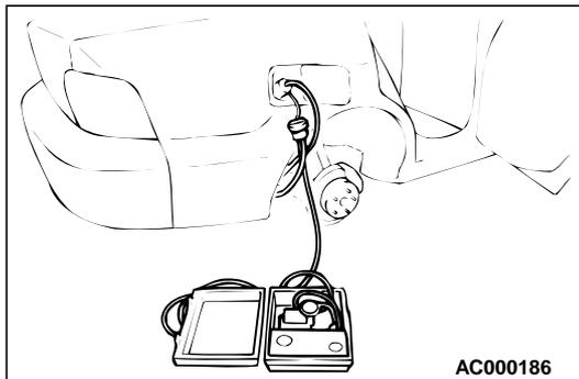
**STEP 2. Pressure test for evaporator line from hose C to hose P.**
