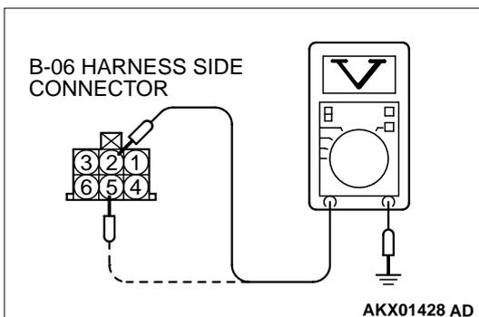
**STEP 5. Check the power supply voltage at idle air control motor harness side connector B-06.**
