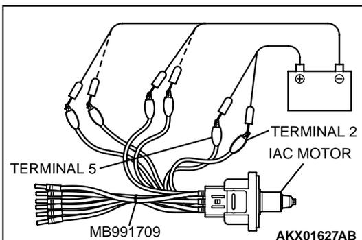
**STEP 11. Check the idle air control motor operation using special tool MB991709.**
