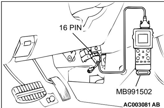
**STEP 9. Using scan tool MB991502, check data list item 39: Right Bank Heated oxygen sensor (front).**
