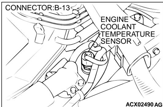
**STEP 8. Check for open circuit between engine coolant temperature sensor connector B-13 terminal 2 and PCM connector C-40 terminal 57.**
