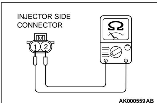
**STEP 8. Check connector B-17, B-19, B-21, B-22, B-25, B-30 at injector and connector B-26 at injector intermediate connector for damage.**
