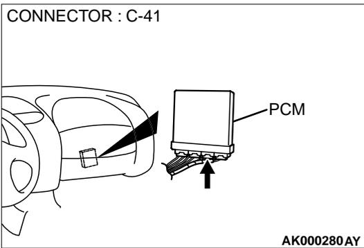
**STEP 4. Check connector B-28 at left bank heated oxygen sensor (front) and connector C-41 at PCM for damage.**
