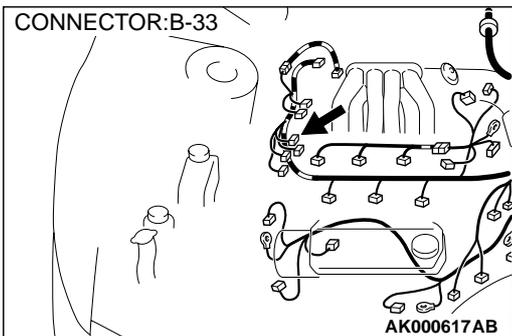
**STEP 10. Check for harness damage between right bank heated oxygen sensor (rear) connector B-31 terminal 3 and PCM connector C-39 terminal 27.**
