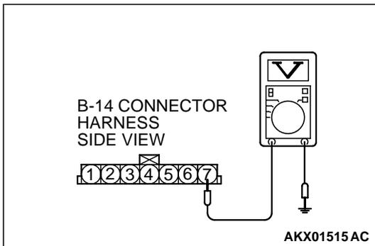
**STEP 3. Check connector B-14 at volume air flow sensor and connector C-39 at PCM for damage.**
