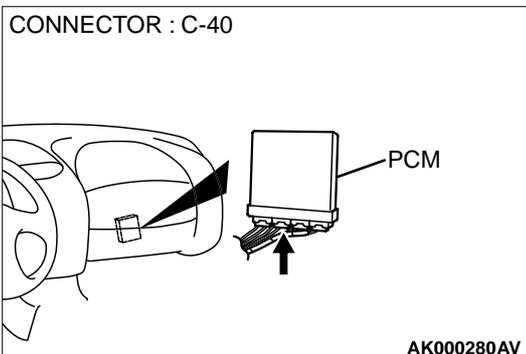
**STEP 10. Check for harness damage between generator connector B-46 terminal 4 and PCM connector C-40 terminal 54.**
