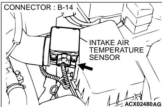
**STEP 6. Check the intake air temperature sensor.**
