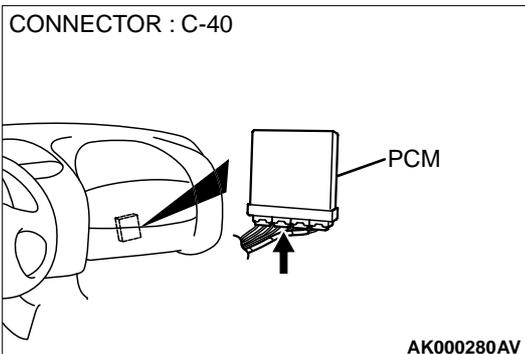
**STEP 11. Check for open circuit and short circuit to ground and harness damage between manifold differential pressure sensor connector B-18 terminal 1 and PCM connector C-41 terminal 91.**
