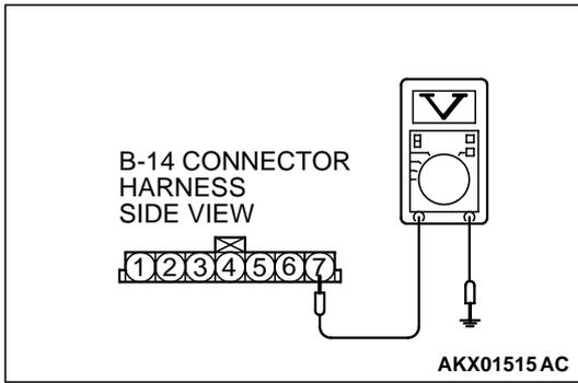
**STEP 5. Check the reset signal voltage at volume air flow sensor connector B-14 by backprobing.**
