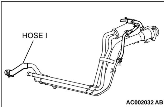
**STEP 27. Check for clogging in the evaporator line hose I, L, M, N and hose O.**
