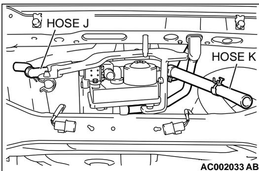
**STEP 30. Check for clogging in the evaporator line from hose J to hose K.**
