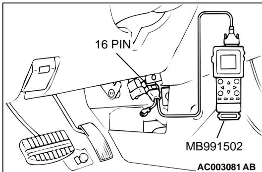
**STEP 3. Using scan tool MB991502, check data list item 82<bank 1> and 84 <bank 2>: Short – Term Fuel Compensation (trim) Bank 1.**
