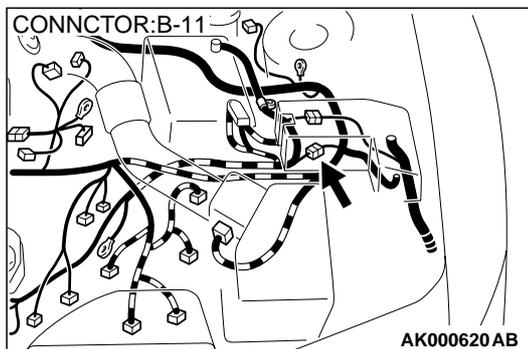
**STEP 4. Check connector B-11 at generator intermediate connector for damage.**
