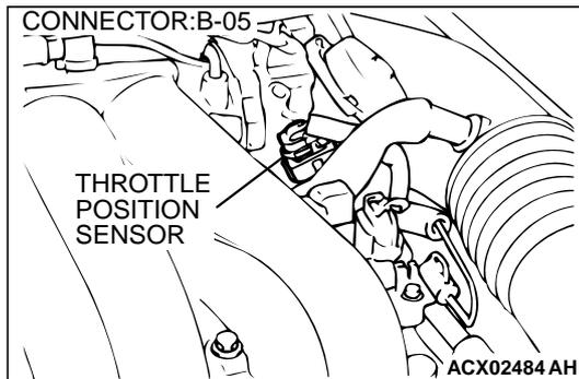
**STEP 7. Check for open circuit and harness damage between throttle position sensor connector B-05 terminal 1 and PCM connector C-40 terminal 57.**
