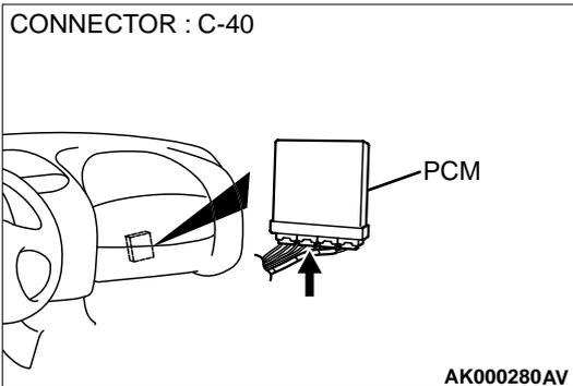
**STEP 14. Check for harness damage between barometric pressure sensor connector B-14 terminal 5 and PCM connector C-40 terminal 57.**
