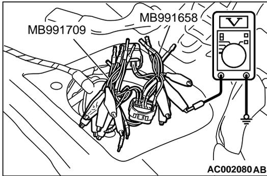
**STEP 3. Check the 5-volt supply circuit voltage at intermediate connector D-15.**
