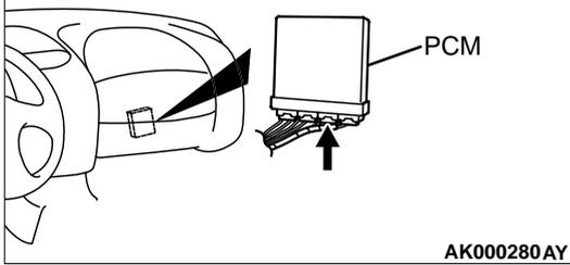
**STEP 5. Check connector C-41 at PCM for damage.**
