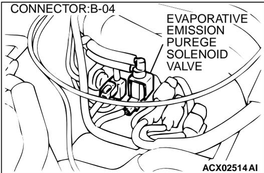
**STEP 11. Check for harness damage between evaporative emission purge solenoid connector B-04 terminal 1 and PCM connector C-39 terminal 34.**
