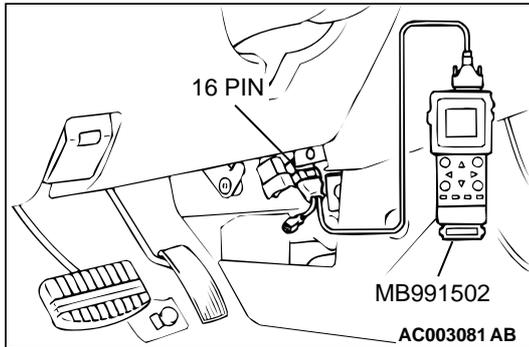
**STEP 2. Using scan tool MB991502, check data list item 81 <bank 1> and 83 <bank 2>: Long – Term Fuel Compensation (trim).**
