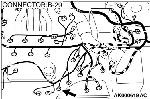
**STEP 10. Check for harness damage between left bank heated oxygen sensor (rear) connector B-29 terminal 3 and PCM connector C-39 terminal 26.**
