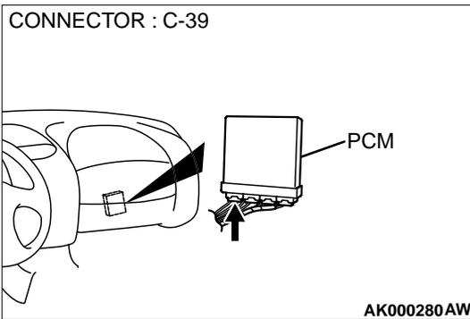
**STEP 11. Check for harness damage between evaporative emission ventilation solenoid connector D-13 terminal 1 and PCM connector C-39 terminal 35.**
