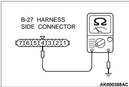
**STEP 5. Check the continuity at distributor harness side connector B-27.**
