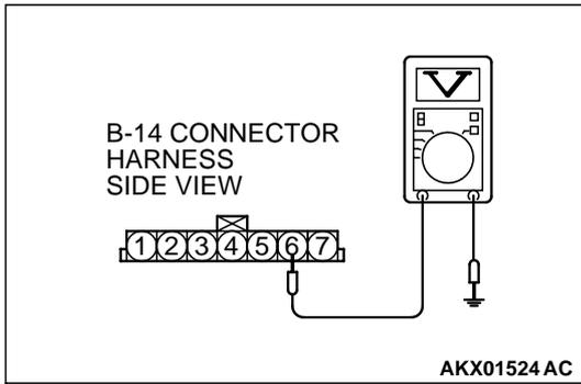
**STEP 2. Check the sensor output voltage at intake air temperature sensor connector B-14 by backprobing.**
