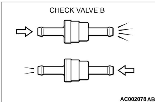
**STEP 14. Check the check valve B.**
