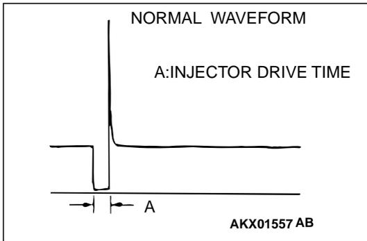
**STEP 9. Using the oscilloscope, check the injector.**
