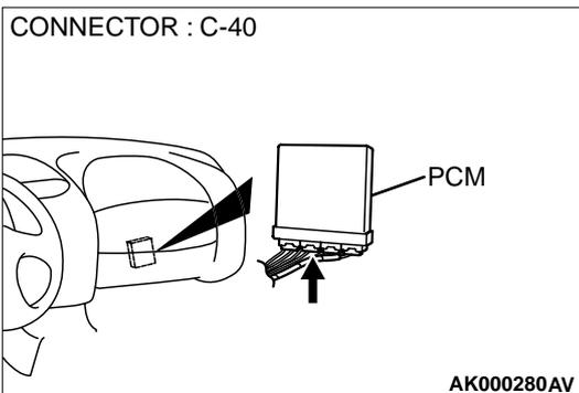
**STEP 12. Check connector C-40 at PCM for damage.**
