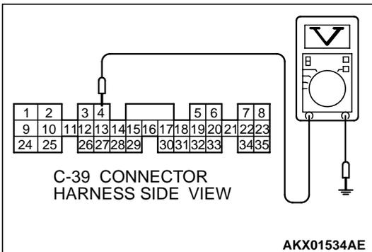
**STEP 5. Check the power supply voltage at PCM connector C-39 by backprobing.**
