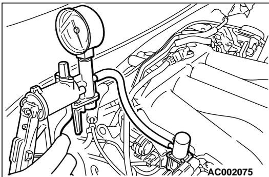
**STEP 3. Check the evaporative emission purge solenoid valve using the scan tool MB991502. (Actuator test item 08)**
