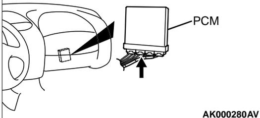
**STEP 7. Check for harness damage between throttle position sensor connector B-05 terminal 3 and PCM connector C-41 terminal 78.**
