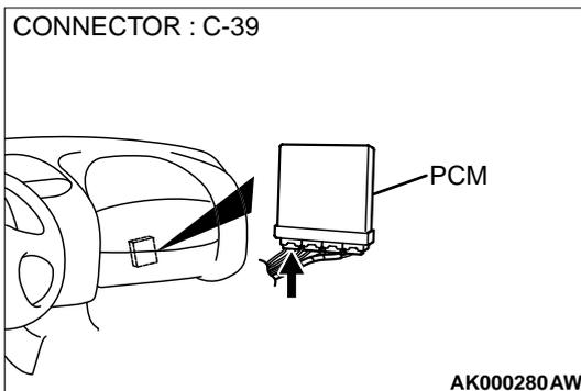
**STEP 10. Check for harness damage between left bank injector connector and PCM connector.**
