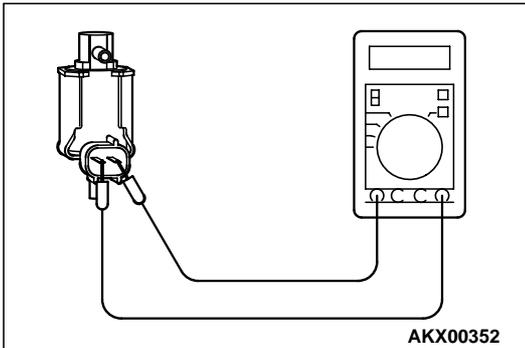
**STEP 4. Check the power supply voltage at EGR solenoid harness side connector B-03.**
