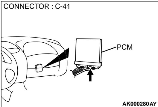
**STEP 2. Check for open circuit, short circuit to ground and harness damage between data link connector C-23 terminal 1 and PCM connector C-41 terminal 84.**
