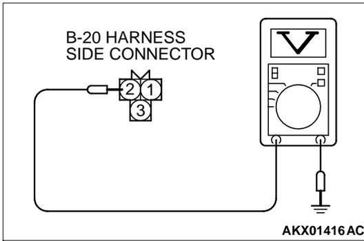
**STEP 6. Check the sensor supply voltage at crankshaft position sensor harness side connector B-20.**
