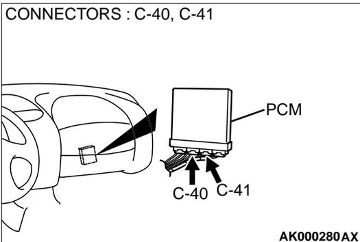
**STEP 10. Check connector C-40, C-41 at PCM for damage.**
