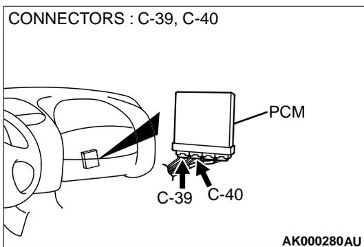
**STEP 6. Check connector C-39, C-40 at PCM for damage.**
