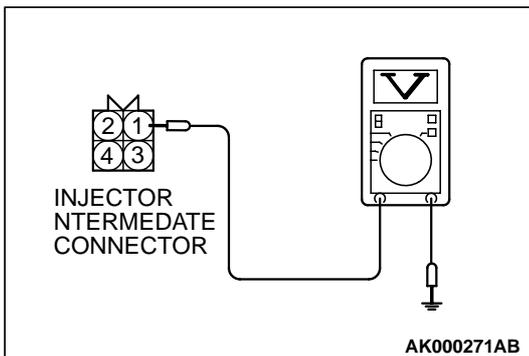
**STEP 6. Check the power supply voltage at injector intermediate connector B-26.**
