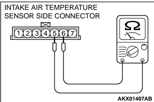
**STEP 7. Check the sensor supply voltage at intake air temperature sensor harness side connector B-14.**
