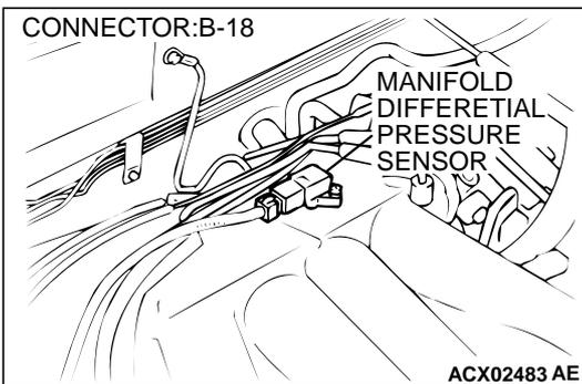
**STEP 8. Check for open circuit and harness damage between manifold differential pressure sensor connector B-18 terminal 2 and PCM connector C-40 terminal 57.**
