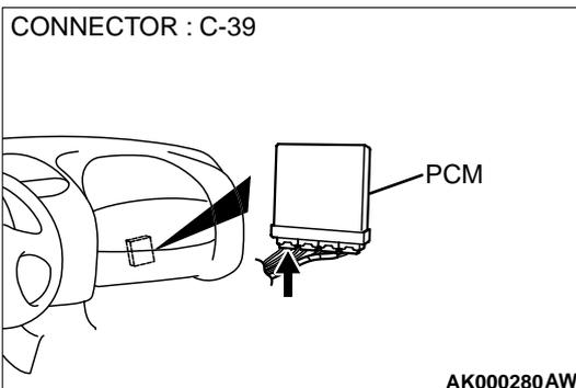
**STEP 5. Check for open circuit and short circuit to ground and harness damage between generator connector B-46 terminal 1 and PCM connector C-39 terminal 8.**
