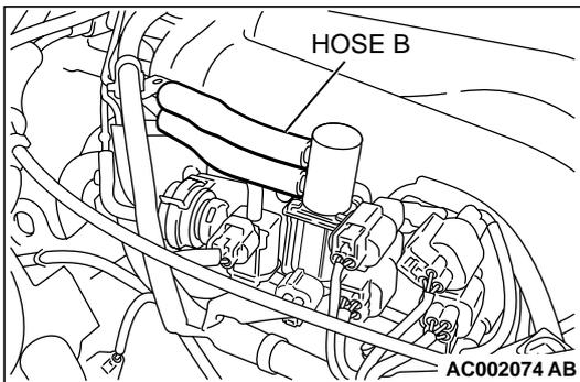
**STEP 6. Check the evaporative emission ventilation solenoid using the scan tool MB991502. (Actuator test item 29)**
