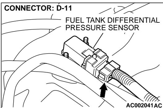
**STEP 8. Check fuel tank differential pressure sensor connector D-11 for damage.**
