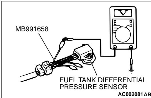
**STEP 5. Check the output circuit voltage at fuel tank differential pressure connector D-11.**
