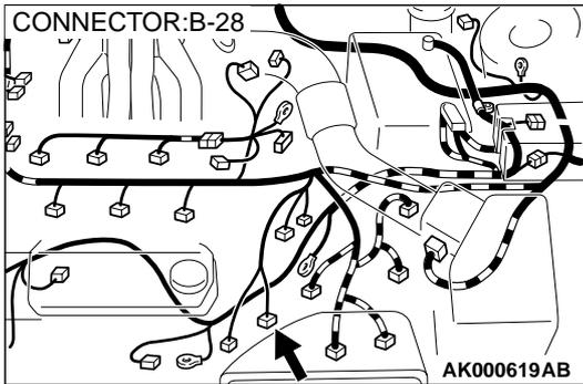
**STEP 10. Check for harness damage between left bank heated oxygen sensor (front) connector B-28 terminal 3 and PCM connector C-39 terminal 3.**
