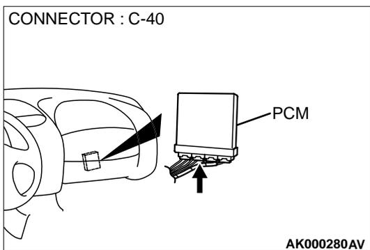
**STEP 7. Check connector C-40 at PCM for damage.**
