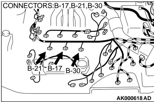
**STEP 8. Check the left bank injector.**
