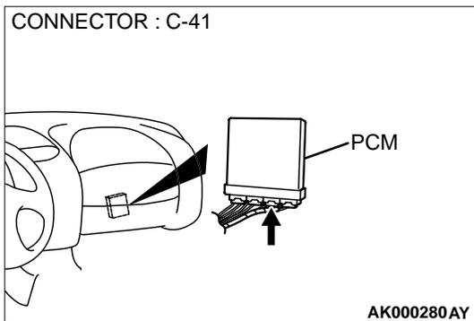
**STEP 3. Check connector C-41 at PCM for damage.**
