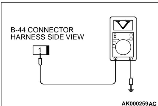
**STEP 3. Check connector B-44 at power steering pressure switch for damage.**
