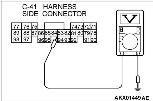
**STEP 3. Check the circuit at PCM connector C-41.**
