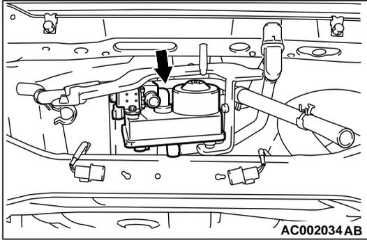
**STEP 21. Check the vent valve module for clogging.**
