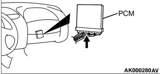
**STEP 4. Check connector C-40 at PCM for damage.**
