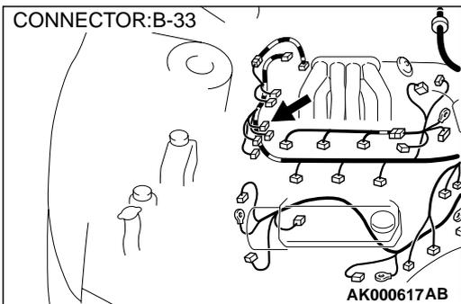
**STEP 10. Check for open circuit and harness damage between right bank heated oxygen sensor (front) connector B-33 terminal 2 and PCM connector C-40 terminal 57.**
