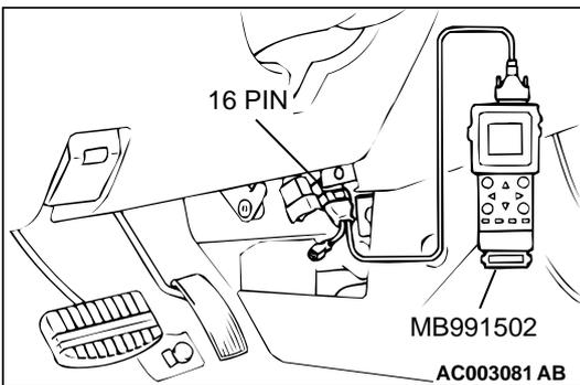
**STEP 6. Using scan tool MB991502, check data list item 44: Ignition Coils and Ignition Power Transistor.**
