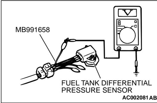
**STEP 6. Check the 5-volt supply circuit voltage at fuel tank differential pressure sensor connector D-11.**
