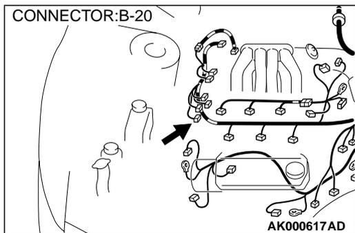
**STEP 4. Using scan tool MB991502, check data list item 22: Crankshaft Position Sensor.**
