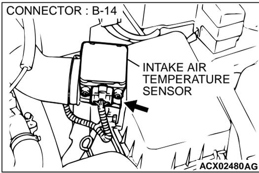
**STEP 5. Check connector B-14 at intake air temperature sensor for damage.**
