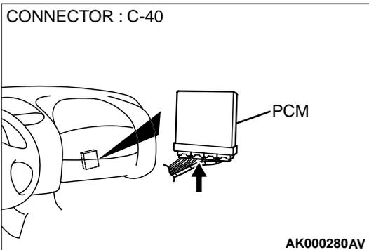
**STEP 4. Check connector C-40 at PCM for damage.**
