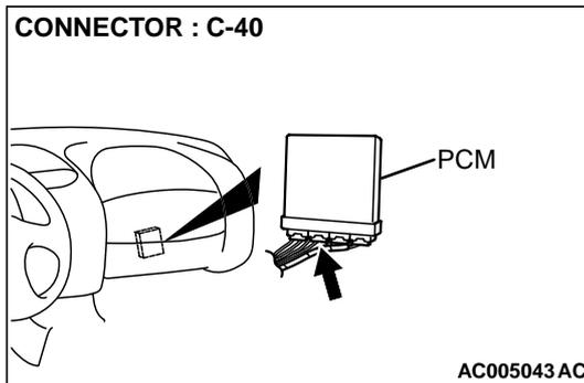
**STEP 12. Check PCM connector C-40 for damage.**
