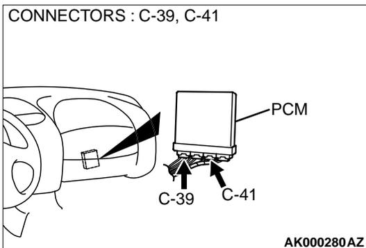
**STEP 2. Check the circuit at PCM connector C-39.**
