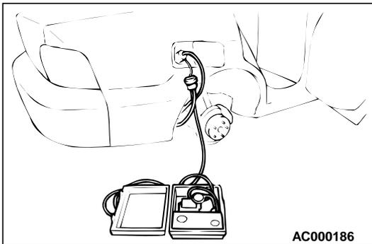
**STEP 2. Check the output circuit voltage at intermediate connector D-15.**
