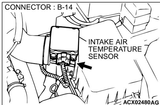
**STEP 4. Using scan tool MB991502, check data list item 13: Intake Air Temperature Sensor.**
