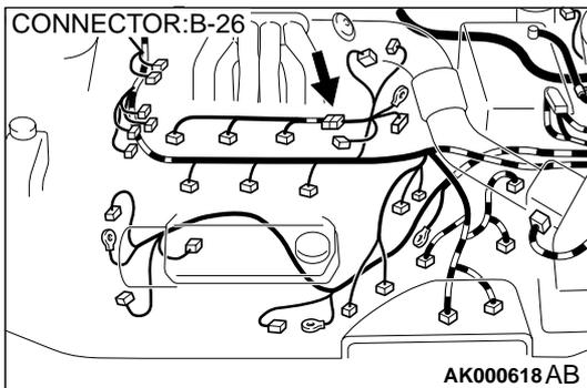
**STEP 9. Check the right bank injector resistance at injector intermediate connector B-26.**
