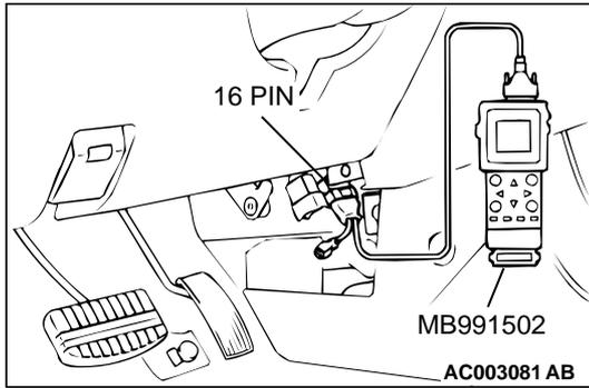
**STEP 5. Using scan tool MB991502, check actuator test.**
