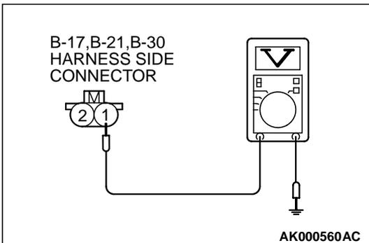
**STEP 4. Check the power supply voltage at injector connector.**
