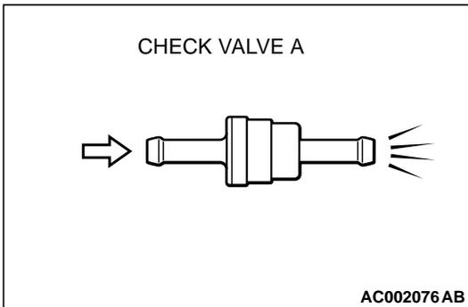
**STEP 13. Check the check valve A.**
