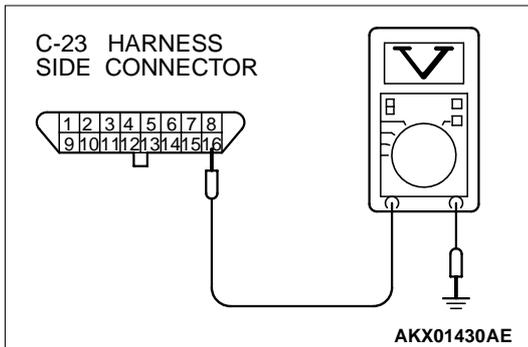
**STEP 2. Check the continuity at data link connector C-23.**
