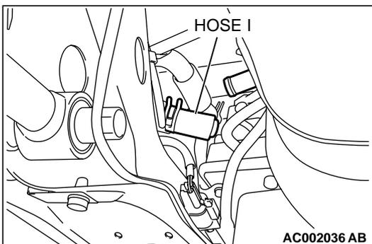
**STEP 4. Pressure test for evaporator line from hose I to hose P.**
