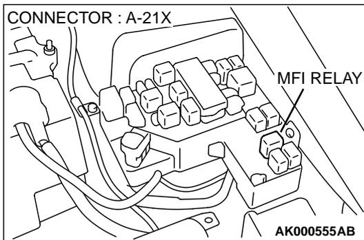
**STEP 11. Check connector A-21X at MFI relay for damage.**
