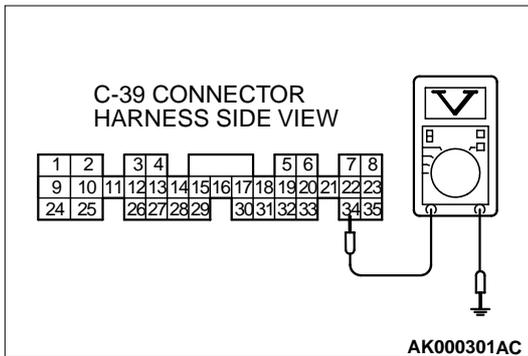
**STEP 6. Check the power supply voltage at PCM connector C-39 by backprobing**
