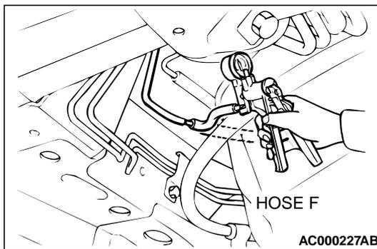
**STEP 24. Check for clogging in the evaporator line hose F.**
