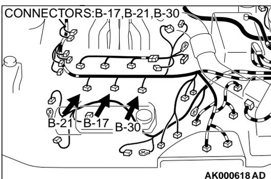
**STEP 4. Check the left bank heated oxygen sensor (front).**
