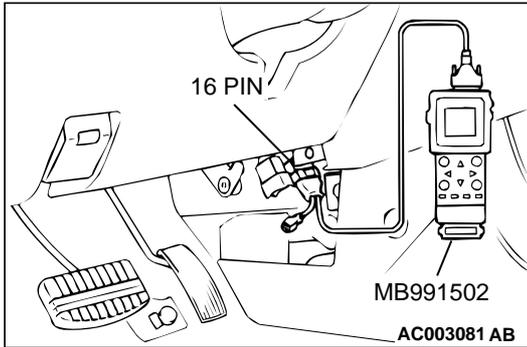
**INSPECTION PROCEDURE 18: Poor acceleration.**
