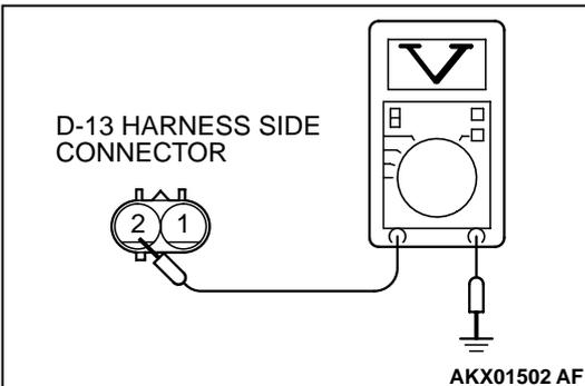
**STEP 4. Check the power supply voltage at evaporative emission ventilation solenoid harness side connector D-13.**
