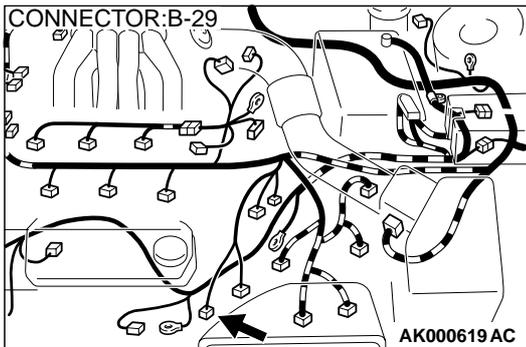
**STEP 8. Check the continuity at left bank heated oxygen sensor (rear) harness side connector B-29.**
