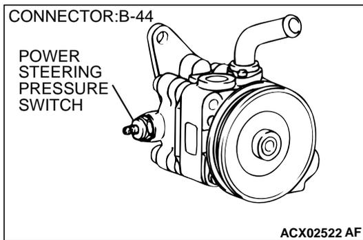
**STEP 6. Check the power supply voltage at power steering pressure switch harness side connector B-44.**
