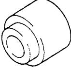
B990800                                | MB990800                             | Ball joint remover and installer         | Ball joint dust cover installation   |
