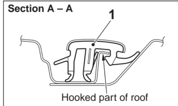
← : Roof drip moulding attaching locations to the hooked parts of roof.
