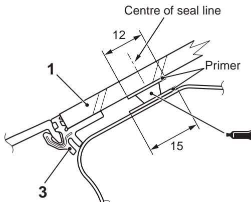
Adhesive: 3M ATD Part No. 8609 Super Fast Urethane Auto Glass Sealant or equivalent and
