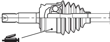
Grease: repair kit grease
