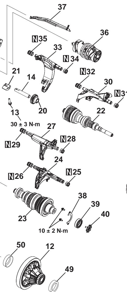
Apply gear oil to all moving parts before installation.
