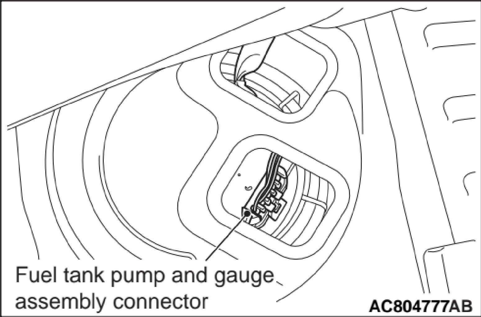
Fuel tank pump and gauge
