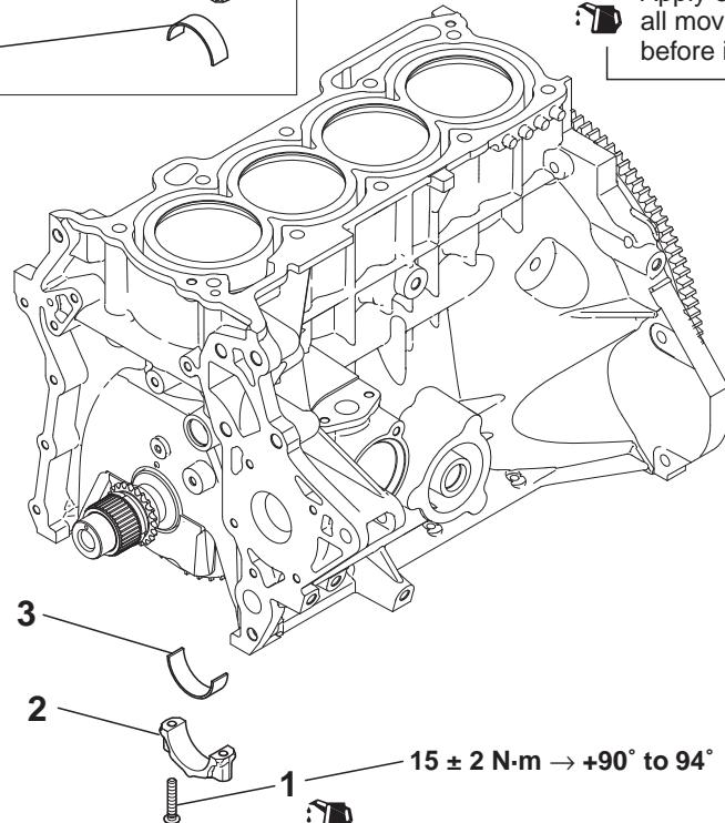
$15 \pm 2 \text{ N}\cdot\text{m} \rightarrow +90^\circ \text{ to } 94^\circ$
