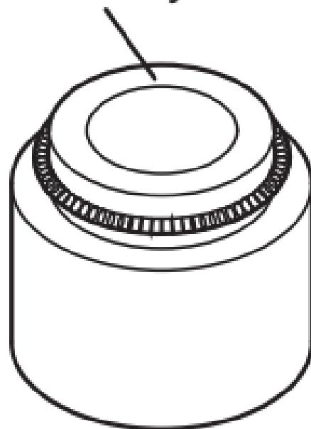
Exhaust valve stem seal
