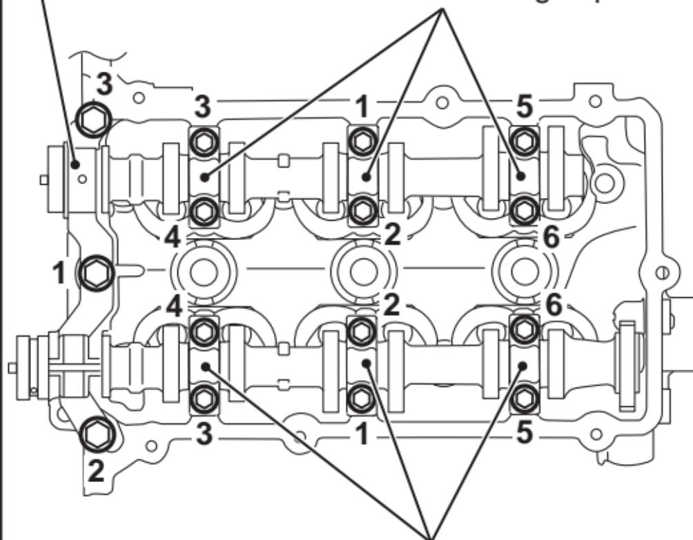
Camshaft bearing cap
