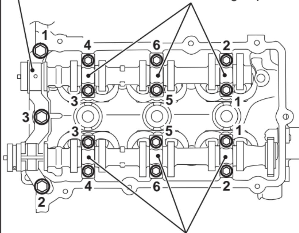
Camshaft bearing cap
