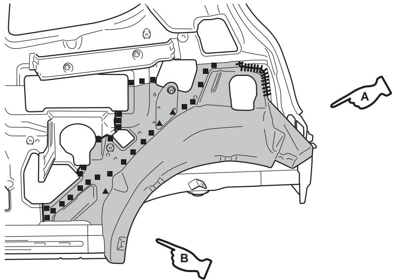
(With the quarter outer panel and fuel filler neck bracket removed)
