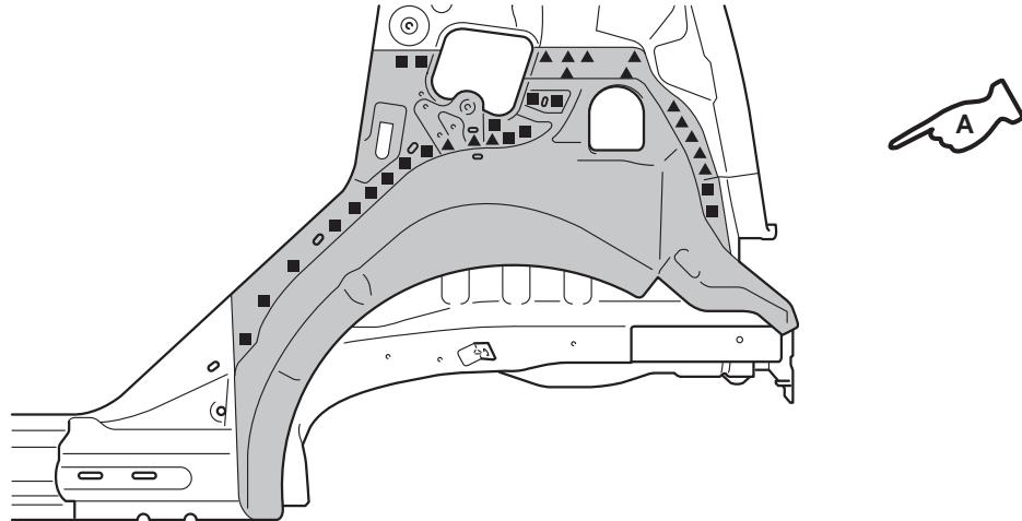
(With the quarter outer panel and fuel filler neck bracket removed)
