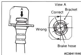
2. Twist the brake hose towards the lesser torsion between the brake hose and bracket as shown and secure it to the bracket.
