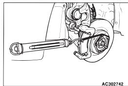
1. In order to measure the brake drag torque, measure the hub torque with the pads removed by the following procedure.
