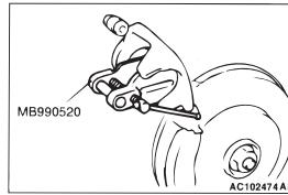
3. Clean the piston and insert into cylinder with special tool disc brake piston expander (MB990520).
