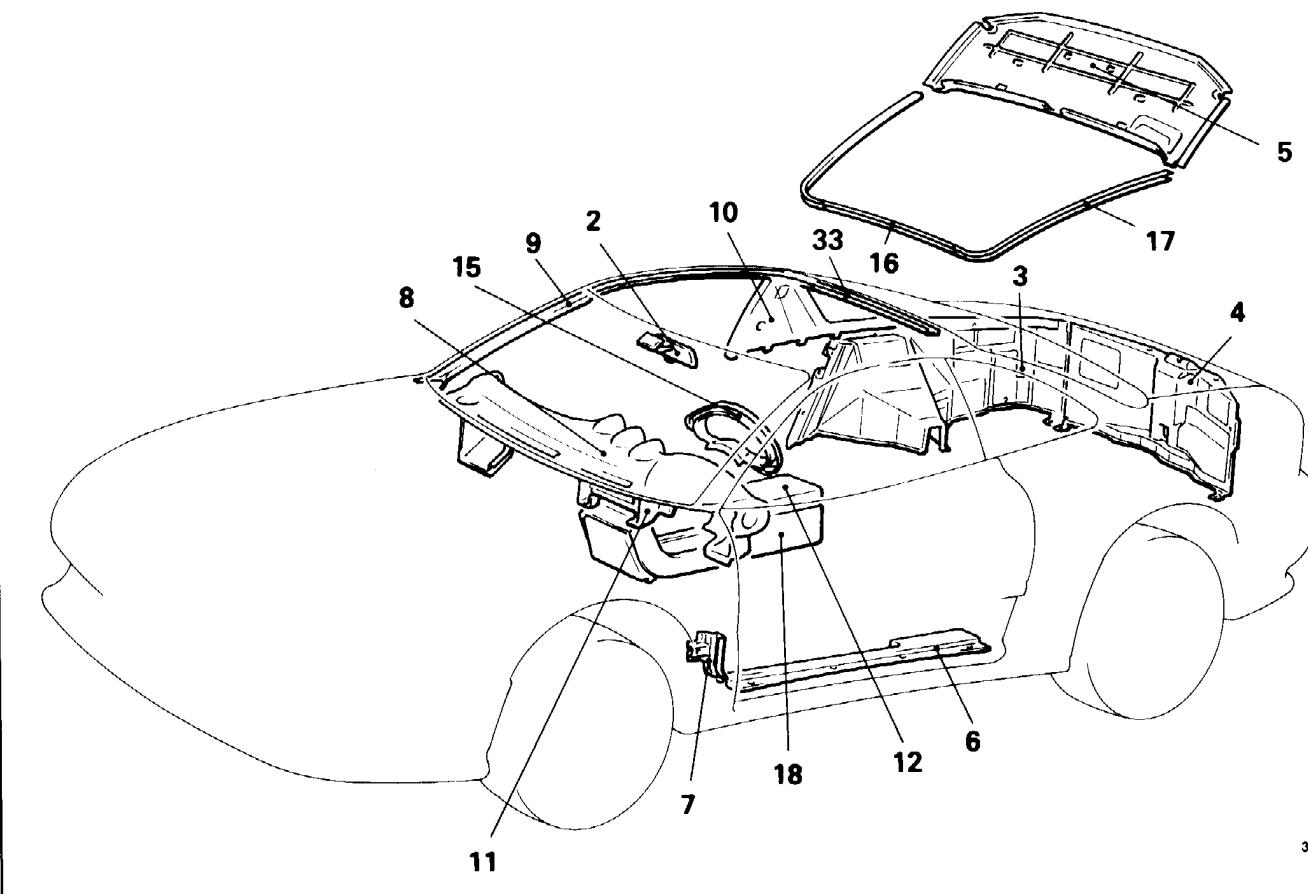
**SYNTHETIC-RESIN PARTS – Location of Synthetic-resin Parts**
