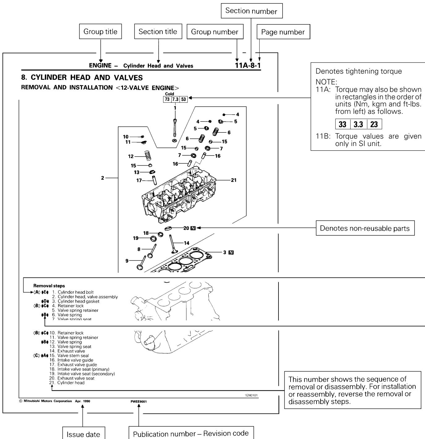
Operating procedures, cautions, etc. on removal, installation, disassembly and reassembly are described.
