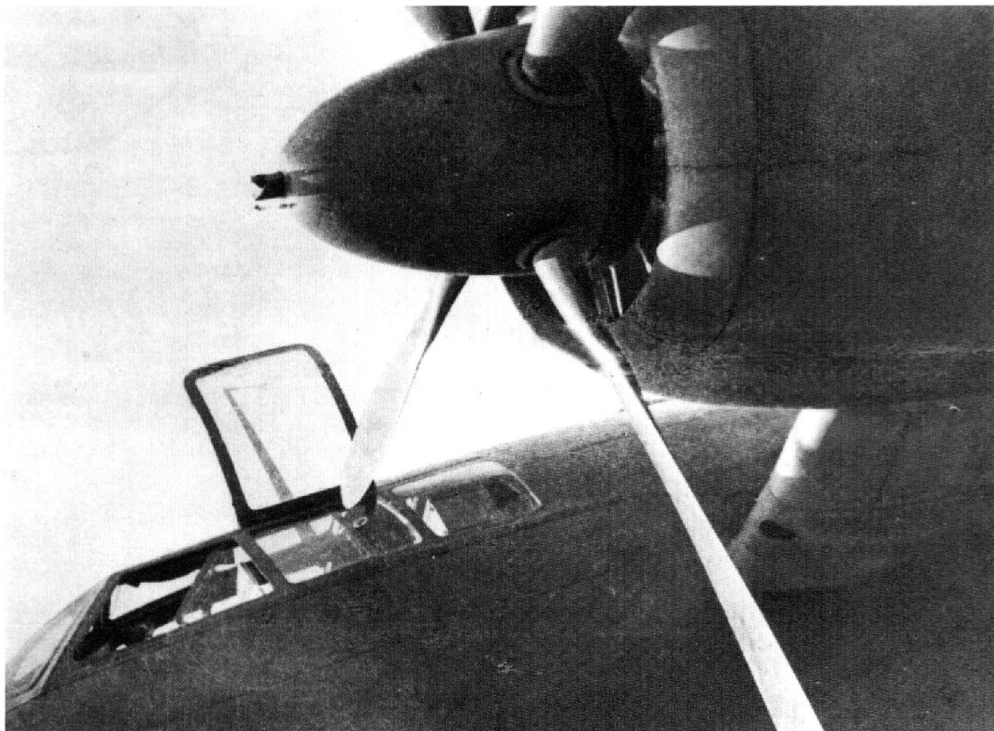
Power plants for all Hiryu production models were the powerful 18-cyl. 1,900 h.p. Mitsubishi Ha.104 Type 4 radial. Mannosuke Toda.
