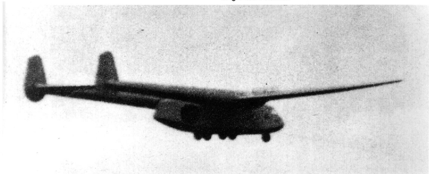
The Kokusai Ku.7 could be towed by the Nakajima Ki.49 Donryu or the Mitsubishi Ki.67-la Hiryu, although the Mitsubishi bomber was preferred due to its greater power and faster tow speed. Hideya Ando.
