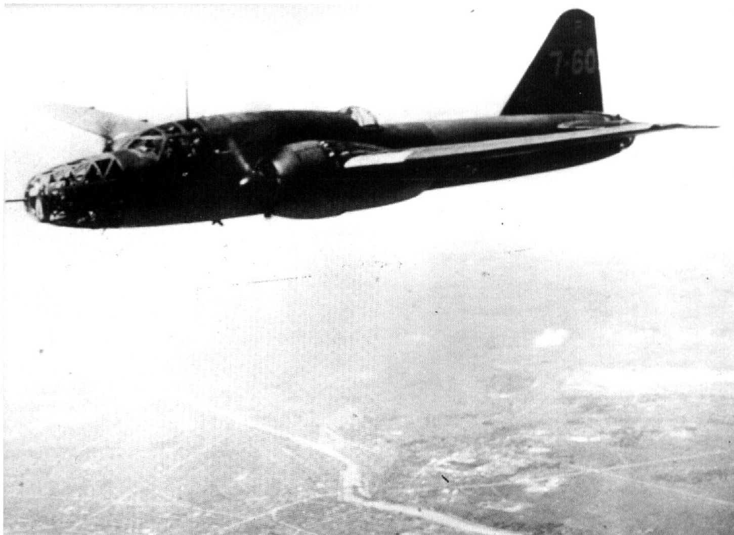
Hiryu torpedo bombers of the 7th Air Regiment carried their unit number on the fin. Mounting shackles to carry the torpedo below the fuselage can be seen on the underside of aircraft 7-60 of the 3rd company. Mannosuke Toda.
