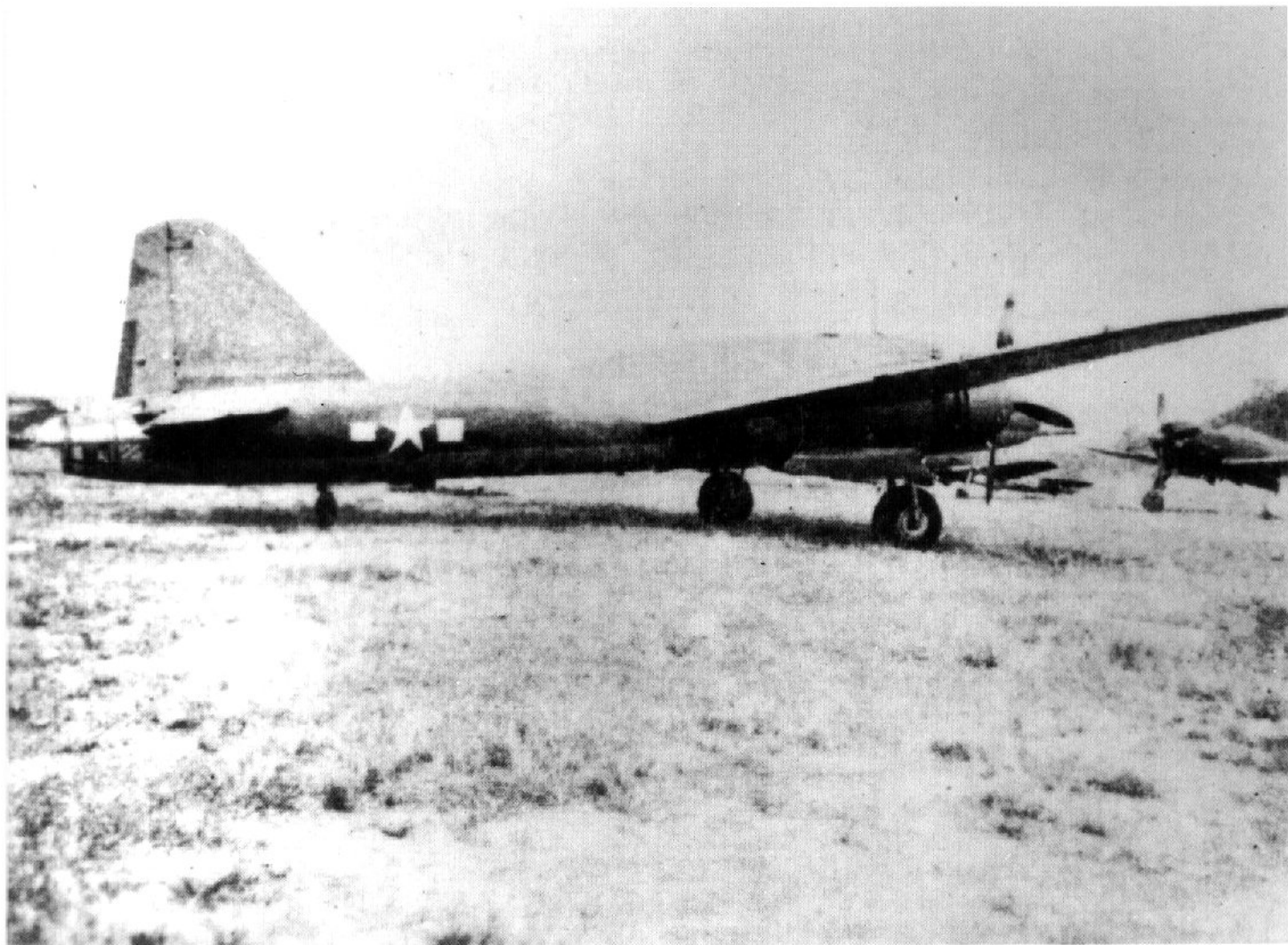
Production of the Ki.109 was 22 aircraft, experimental and operational. They were never able to intercept the B-29 due to poor climb and low ceilings. U. S. markings applied for test, but never pursued. Aircraft destroyed in Japan. USAF.
