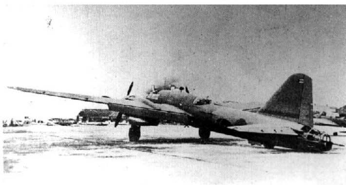
Radar "whiskers" were also on the fuselage, just forward of the side gun positions. Sekai no Kokuki.
