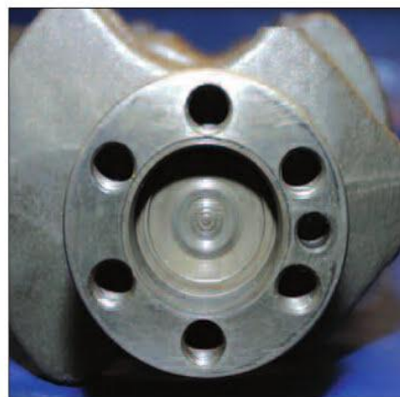
The 6-bolt and 7-bolt 4G63t engines take their names for the number of bolts holding the flywheel to the end of the crankshaft. There are hundreds of detail changes between the two engines; about all they share is bore and stroke, a head bolt pattern, and bellhousing bolt pattern.
