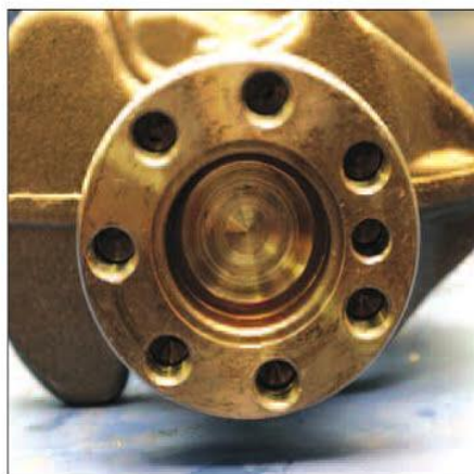
The 6-bolt and 7-bolt 4G63t engines take their names for the number of bolts holding the flywheel to the end of the crankshaft. There are hundreds of detail changes between the two engines; about all they share is bore and stroke, a head bolt pattern, and bellhousing bolt pattern.
