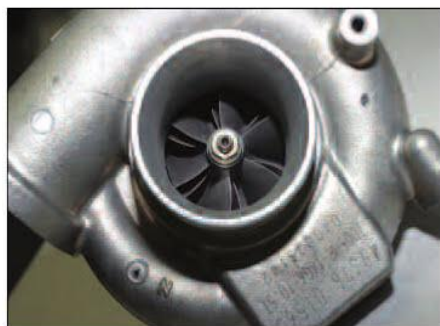
The Evo VIII has a unique, reverse-spinning variant of the 16G turbo. Its MHI code is 49178-01560. Notice how the compressor blades are folded over to the left, opposite the blades on the Evo III 16G shown above.
