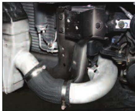
The Evo has a generous-sized intercooler, but the stock intercooler core is compromised to fit easily within the bumper. In addition, it is somewhat restrictive at high power levels.
