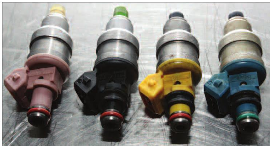
These are some of the most common stock 4G63t injectors. From left to right, the pink injector is a 560-cc/min unit from an Evo VIII or IX, the black one is a 450-cc/min 2g DSM injector, the yellow is a 510-cc/min from an Evo III or Japanese Galant with a big turbo, and the blue one is 450-cc/min from a 1g manual transmission car.
