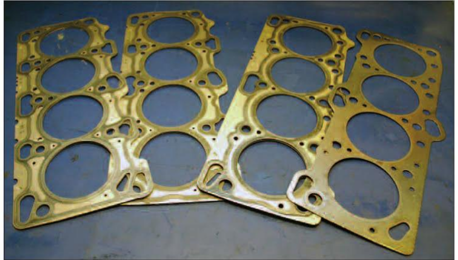
One look at this comparison of the various head gaskets and it's pretty clear that all of the 4G63t engines share the same head bolt pattern and most of the same oil and coolant passages. From left to right, the gaskets are Evo IX MLS, Evo VIII MLS, 2g MLS, and 1g composite.
