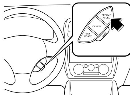
Your vehicle has a tap-up feature that allows you to increase your current speed in increments of 1.6 km/h (1 mph) by a momentary tap of the RESUME/ACCEL button. Multiple taps will increase your vehicle speed 1.6 km/h (1 mph) for each tap.
