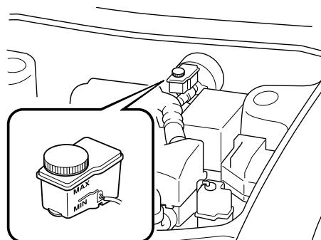
**Owner Maintenance****▼ Adding Brake/Clutch Fluid****⚠ WARNING****Spilled Brake Fluid:**
