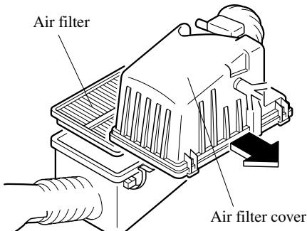
3. Wipe inside the air cleaner housing with a damp cloth.
