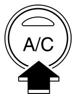
Push the switch to turn the air conditioner on. An indicator light on the switch will illuminate when the fan control dial is on.
