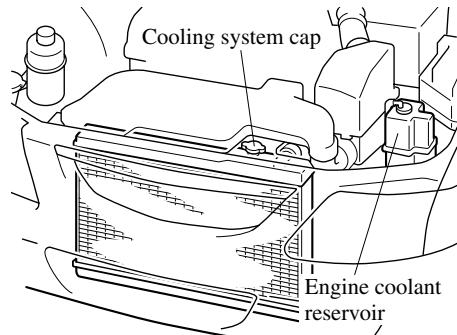
If you find no problems, the engine is cool, and no leaks are obvious, carefully add coolant as required (page 8-12).
