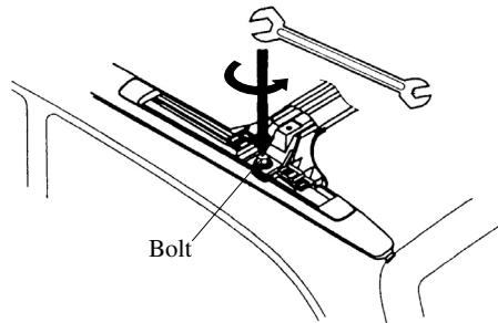
3. Tighten the bolt at both ends of the rear cross bar alternately and evenly.
