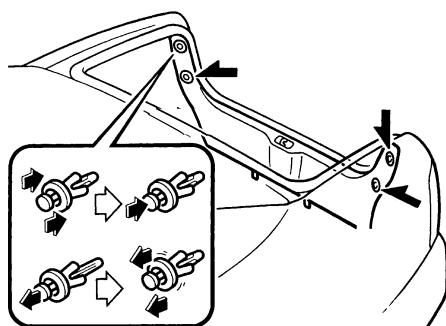
2. Remove the inside cover's plastic retainers and partially open the inside cover.
