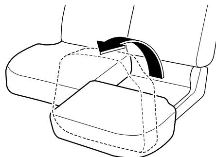
5. Pull the lock release up and fold each seatback forward.
