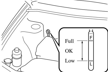
5. Pull it out again and examine the level. It's OK between L and F. But if it's near at or below L, add enough oil to bring the level to F.
