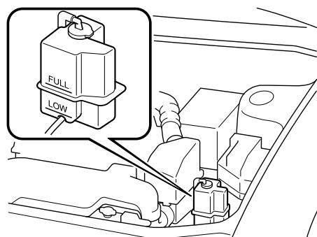
If it's at or near LOW, add enough coolant to the coolant reservoir to provide freezing and corrosion protection and to bring the level to FULL.
