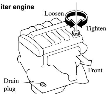
1. Warm up the engine for a few minutes and turn it off. Remove the oil-filler cap.
