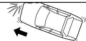
Side impacts involving trees or poles can cause severe cosmetic damage but may not have enough impact force to activate a side air bag.
