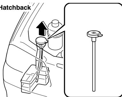
To inspect the washer fluid level in the front reservoir, pull off the cap. Then, holding your thumb over the hole in the center of the cap, lift it straight up. There should be fluid in the straw. Add fluid if necessary.
