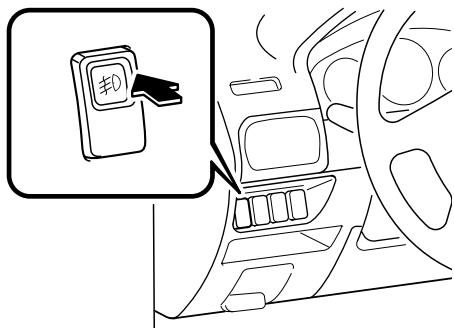
To turn on the fog lights, first turn on the headlight switch. Then press the fog light switch.
