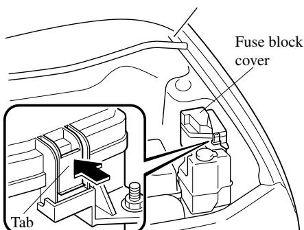
3. If a fuse is blown, replace it with a new one **of the same rating**.
