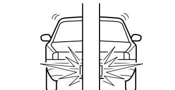
Frontal offset impact to the vehicle may not provide the stopping force necessary for air bag deployment.
