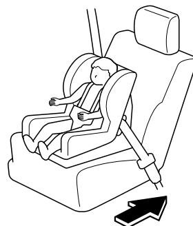
2. Secure the child-restraint system with the lap portion of the lap/shoulder belt. See the instructions on the child-restraint system for belt routing instructions.
