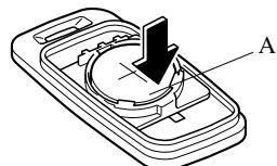
3. Install a new battery (CR2025 or the equivalent) into the front portion of the holder with the positive pole (+) facing up. Press on the B portion of the battery to set the battery.
