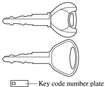
A code number is stamped on the plate attached to the key set; detach this plate and store it in a safe place (not in the vehicle) for use if you need to make a replacement key.
