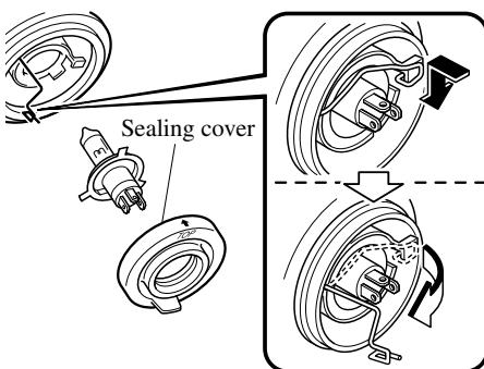
6. Swing the retaining spring out and away to free the headlight bulb.
