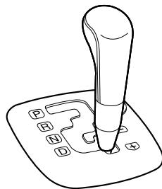
To return to automatic shift mode, shift the lever from M to D.
