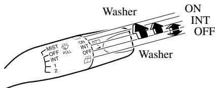
Turn the wiper on by turning the knob.
