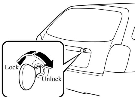
To unlock the liftgate with the key, insert the key and turn it clockwise.
