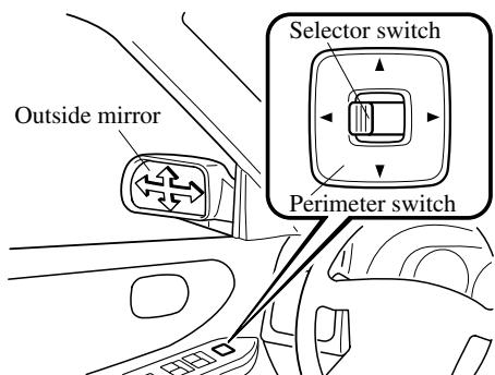
After adjusting the mirror, lock the control by moving the selector switch to the middle position.
