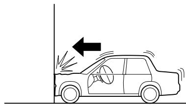
Frontal impact within about a 30 degree range from head-on to the vehicle.
