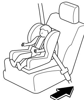
2. Secure the child-restraint system with the lap portion of the lap/shoulder belt. See the manufacturer's instructions on the child-restraint system for belt routing instructions.
