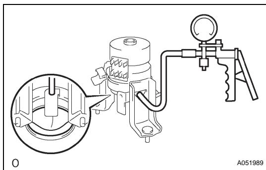
(a) Disconnect the vacuum hose from the front engine mount insulator.
