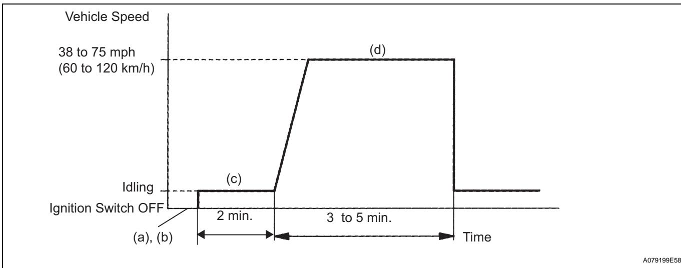
(b) Switch the intelligent tester from the normal mode to the check mode (See page [ES-29](#) Step (b).
