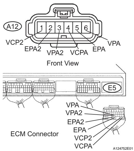
(a) Disconnect the A12 accelerator pedal position sensor connector.
