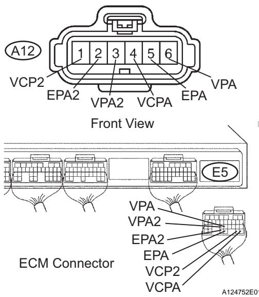
(a) Disconnect the A12 accelerator pedal position sensor connector.
