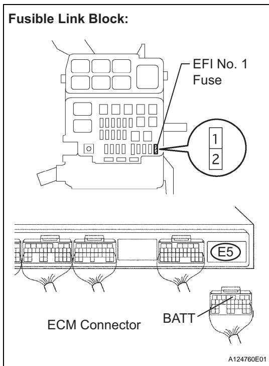
(a) Check the wire harness between the EFI No. 1 fuse and ECM.
