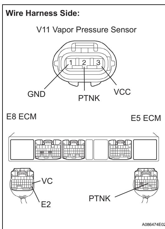
(a) Disconnect the V11 vapor pressure sensor connector.
