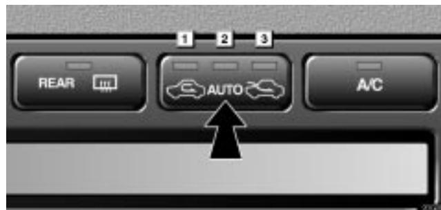
Each time you push the air intake control button, the mode changes in order from the RECIRCULATED AIR mode to AUTOMATIC mode to OUTSIDE AIR mode, then back to the RECIRCULATED AIR mode. Each indicator light shows which mode is now selected.
