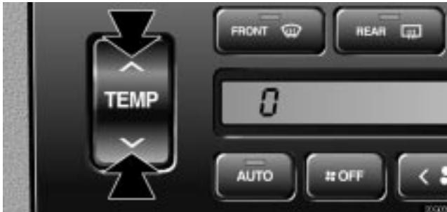
Each time you push the "TEMP" button, the sensitivity changes from "+3" down to "-3". If you do not operate any button for a few seconds or if you push the button other than the air intake control button and driver side temperature control button, the previous display returns.
