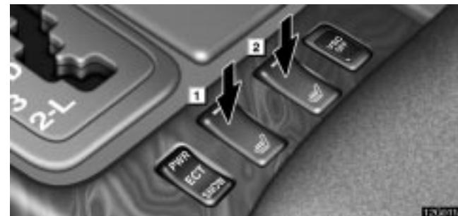
► **1 For driver's seat 2 For front passenger's seat**
