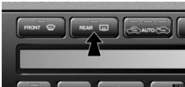
To turn the electric rear window defogger on, push the switch.
