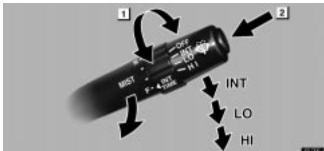
► 1 Interval adjuster 2 Washer on
