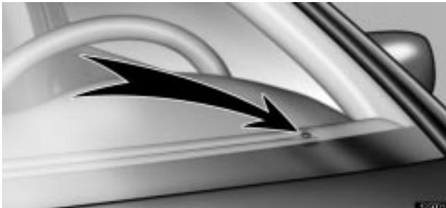
The automatic light control sensor is on top of the driver's side instrument panel.
