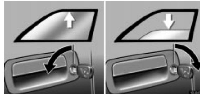
**Insert the ignition key into the key hole on the driver's side.**
