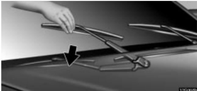
To return the windshield wipers to retracted position, push the connection of the wiper arm and wiper blade downward.
