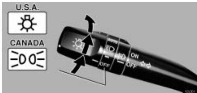
**To turn the lights on, twist the knob on the end of the lever.**
