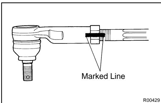
(1) Draw a line on the RH and LH tie rod and rack ends where it can easily be seen.
