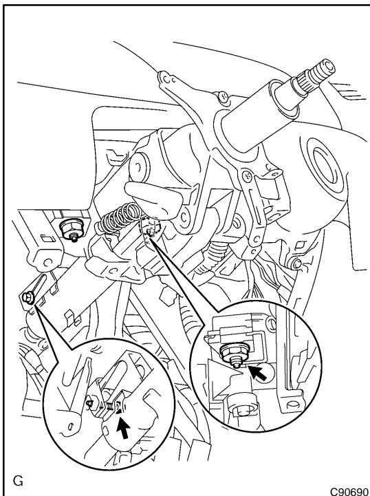
(c) Remove the 2 nuts, bolt and steering column assy from the instrument panel reinforcement assy.
