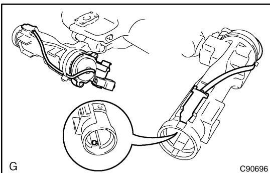
**26. REMOVE UN-LOCK WARNING SWITCH ASSY**
