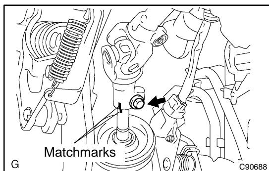
**19. REMOVE STEERING COLUMN HOLE COVER SUB-ASSY NO.2**
