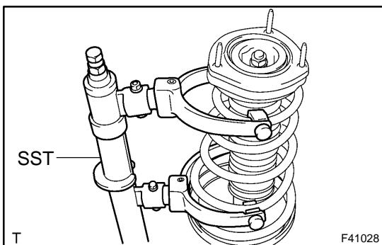
(b) Using SST, compress the coil spring.
