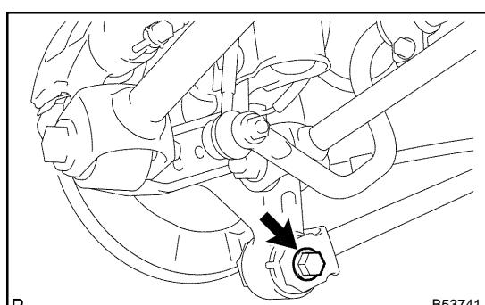
(c) Remove the bolt, nut and strut rod from rear axle carrier.
