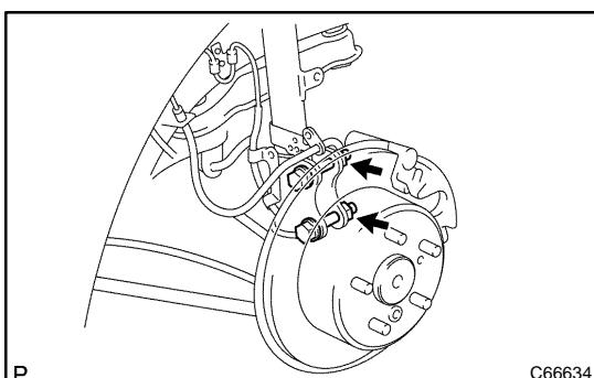
(b) Install the shock absorber with the coil spring, 2 bolts and nuts.
