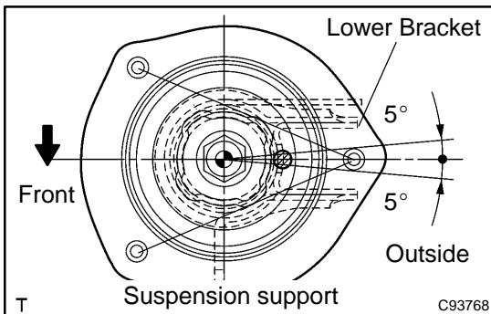
(e) Align the suspension support with the shock absorber lower bracket, as shown in the illustration.
