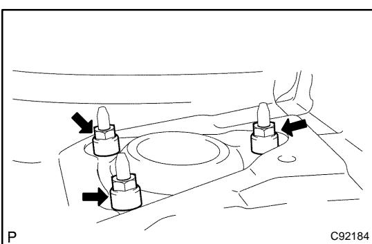
(f) Remove the 3 nuts of the suspension support.
