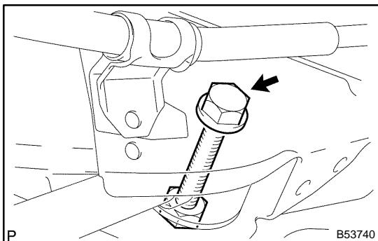
(b) Connect the strut rod (inner side) with the bolt.
