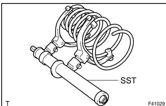
(c) Using SST, compress the coil spring.
