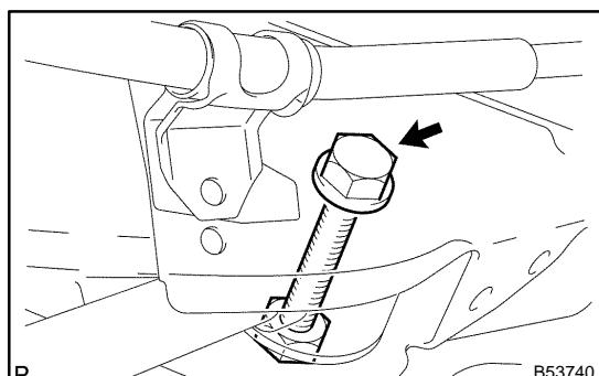
(b) Remove the bolt, nut and disconnect the strut rod (front side).
