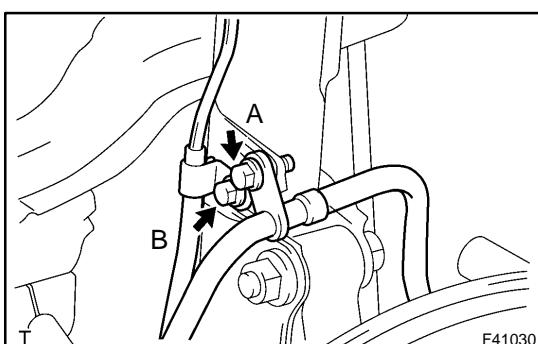
(c) Install the flexible hose and ABS speed sensor wire harness with the 2 bolts.
