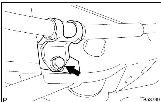
(b) Install the parking brake cable with the bolt and nut.
