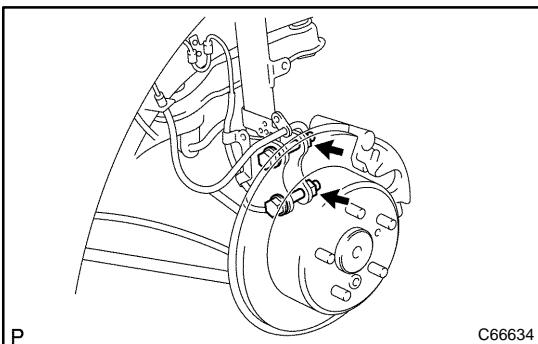
(b) Loosen the 2 bolts on the lower side of the shock absorber.
