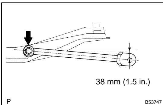
(b) Set the suspension arm in the position in the illustration and fully tighten the bolt.
