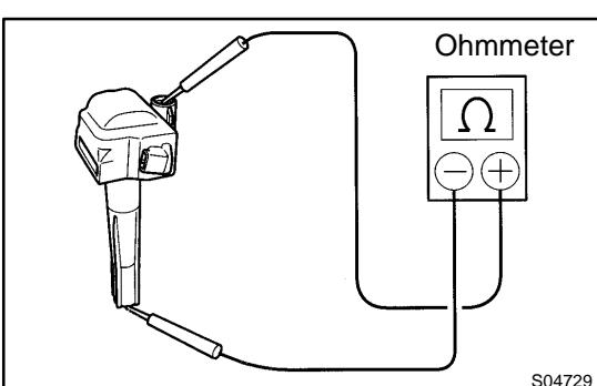
(d) Using an ohmmeter, measure the secondary coil resistance between the positive (+) and high-tension terminal.
