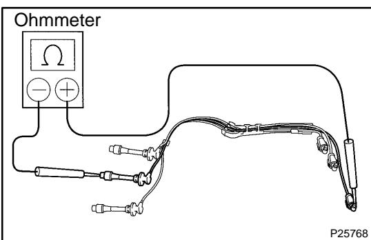
(e) Using an ohmmeter, measure the resistance.
