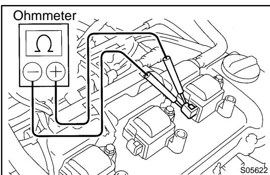
(c) Using an ohmmeter, measure the primary coil resistance between the positive (+) and negative (−) terminals.
