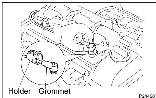
(g) Connect the high-tension cords to the ignition coils.
