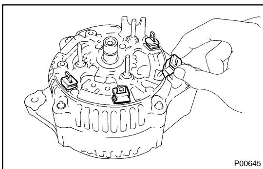
(b) Install the 4 rubber insulators on the lead wires.
