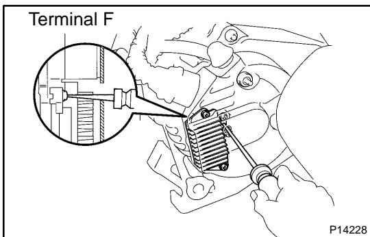
If the voltmeter reading is more than standard voltage, replace the voltage regulator.
