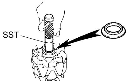
(e) Using SST, push in the bearing cover (outside).
