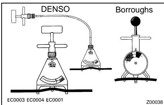
(b) Using a belt tension gauge, measure the belt tension.
