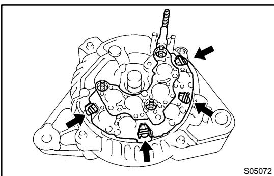
(c) Install the rectifier holder with the 4 screws.
