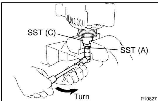
(e) To loosen the pulley nut, turn SST (A) in the direction shown in the illustration.
