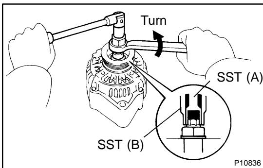
(h) Turn SST (B), and remove SST (A and B).
