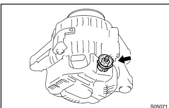
(b) Install the terminal insulator with the nut.
