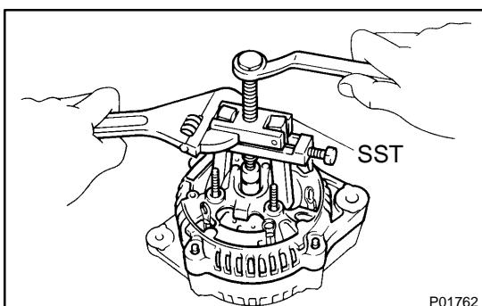
(b) Using SST, remove the rectifier end frame.
